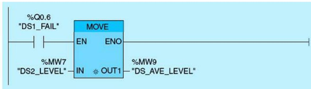
**Figure 9.19** Downstream average level update using sensor 2.
