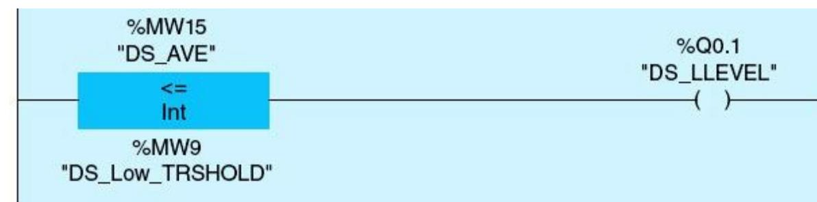
**Figure 4.36** Downstream waterlevel below or equal to the high limit.
