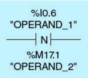
**Figure 3.37** Scan operand for a negative signal edge.
