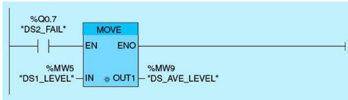
**Figure 9.18** Downstream average level update using sensor 1.
