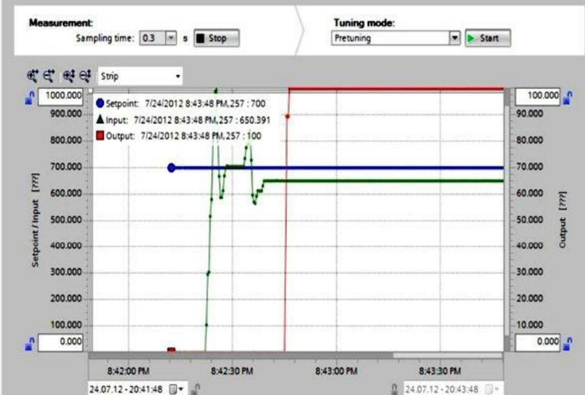
Figure 8.44 Displaying and monitoring process variables.
