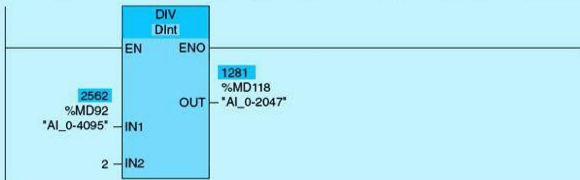
The output count is normalized and scaled to produce the standard analog output signal (0-10V/0-27648).
