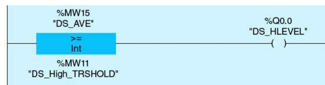
Figure 4.35 Downstream water level above or equal to the high limit.
