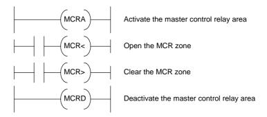
Figure 7.25 Siemens representation of master control relays
