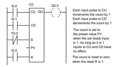
Figure 10.10 Up and down counting with a Siemens PLC
