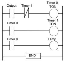
Figure 9.15 Flashing light
