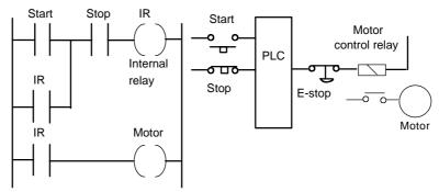
Figure 13.9 A safer emergency stop system
