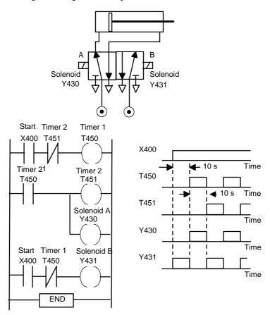
Figure 14.8 Cyclic movement of a piston
