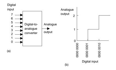
Figure 4.10 (a) DAC function, (b) digital-to-analogue conversion
