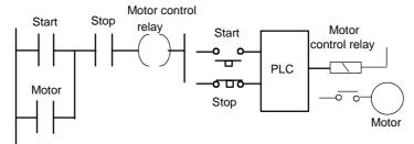
Figure 13.7 A safer stop system
