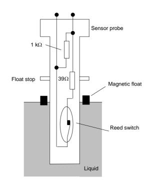
Figure 2.41 *Liquid level monitoring*
