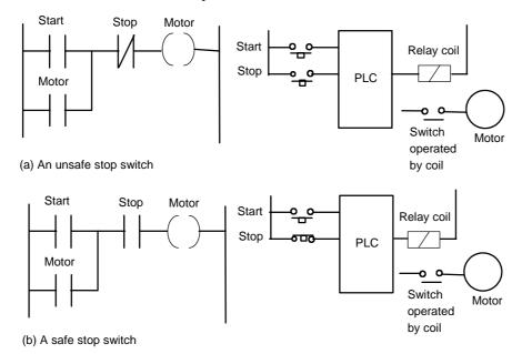
Figure 5.40 Motor stop switch location
