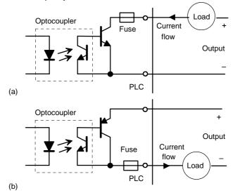
Figure 4.8 Basic forms of transistor output: (a) current sinking, (b) current sourcing
