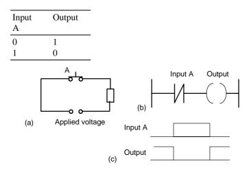
Figure 5.11 (a) NOT circuit, (b) NOT logic with a ladder rung, (c) high output when no input to A
