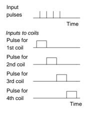
Figure 2.37 Input and outputs of the drive system
