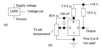
Figure 2.12 (a) LM35, (b) LM3911N circuit for on-off control
