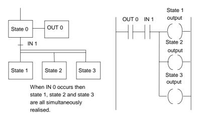
Figure 6.16 Parallel branching states 1, 2 and 3 occur simultaneously when transition IN 1 occurs.
