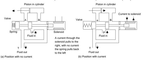
Figure 2.24 An example of a solenoid operated valve
