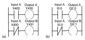
Figure 6.7 Toggle circuit: (a) Mitsubishi, (b) Siemens
