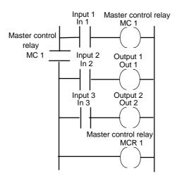
Figure 7.22 Principle of use of a master control relay
