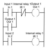
Figure 7.5 Resetting latch
