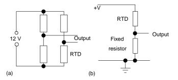
Figure 2.11 (a) Wheatstone bridge, (b) potential divider circuits
