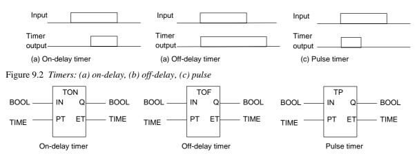
Figure 9.3 IEC 1131-1 standards. BOOL indicates a Boolean input/output, i.e. on/off. IN is the input. Q is the output. ET is the elapsed time output. PT is the input used to specify the time.
