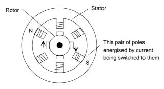
Figure 2.36 The principle of the variable reluctance stepper motor
