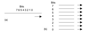
Figure 4.19 (a) Serial communication, (b) parallel communication
