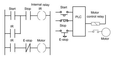
Figure 13.8 An unsafe emergency stop system
