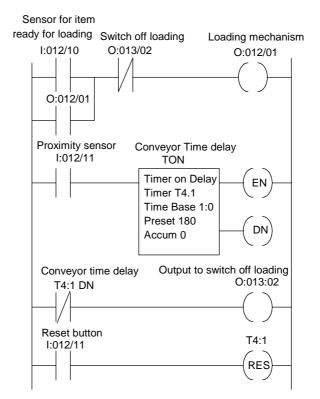
Figure 14.17 Conveyor belt time delays
