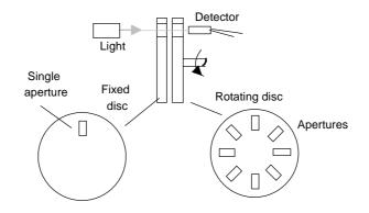
Figure 2.8 Basic form of an incremental encoder
