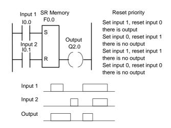
Figure 7.16 SET and RESET, with reset priority
