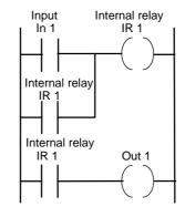
Figure 7.8 Battery-backed relay program
