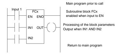
Figure 8.6 Call to subroutine block with Siemens PLC
