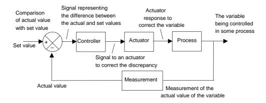
Figure 12.10 Closed loop control
