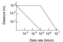
Figure 4.22 Transmission with RS232 and RS422
