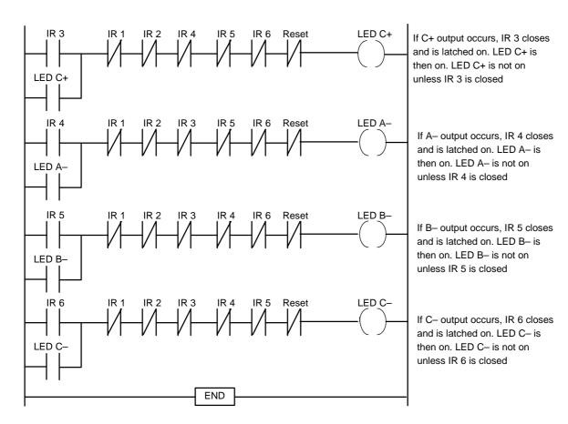
Figure 13.19 Diagnostic program for last cylinder action
