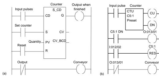
Figure 10.4 (a) Siemens, (b) Allen-Bradley counting program
