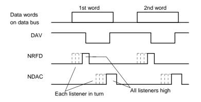
Figure 4.25 Handshaking sequence
