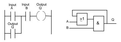
Figure 5.30 Ladder diagram and equivalent function block diagram
