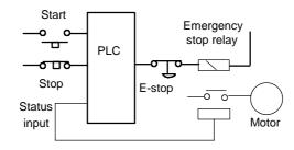
Figure 13.10 Emergency stop relay providing feedback of status
