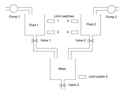
Figure 14.20 The mixing operation
