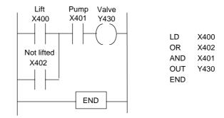
Figure 6.9 Valve operation program
