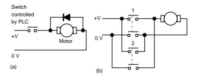
Figure 2.32 D.c. motor: (a) on-off control, (b) directional control
