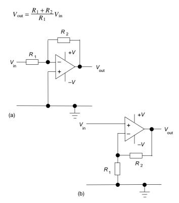
Figure 4.14 Operational amplifier circuits
