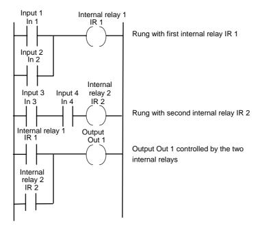
Figure 7.4 Use of two internal relays
