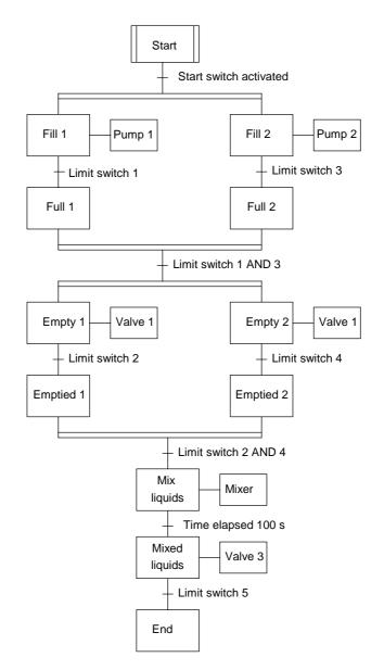
Figure 14.22 The mixing operation program
