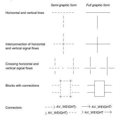
Figure 5.24 Function block diagrams representation
