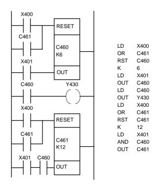
Figure 10.6 Ladder program for Figure 10.5 task
