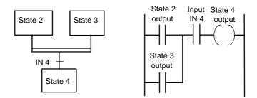
Figure 6.18 Simultaneous convergence: when IN 4 occurs State 4 follows from either State 2 or 3.
