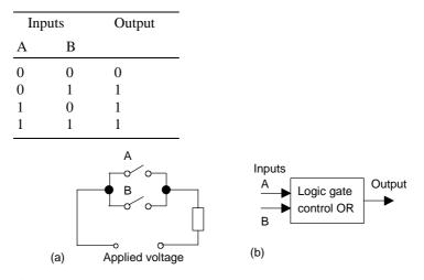
Figure 5.9 (a) OR electrical circuit, (b) OR logic gate
