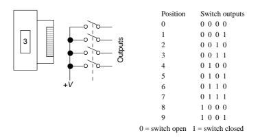
Figure 12.1 *Thumbwheel switch*
