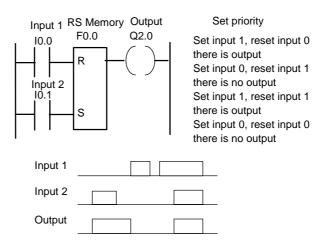
Figure 7.17 SET and RESET, with reset priority
