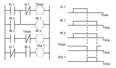
Figure 9.14 Pulse timer on, when output ceases
