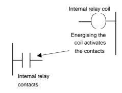
Figure 7.1 Internal relay
