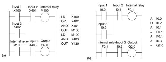
Figure 7.3 Figure 7.2 in: (a) Mitsubishi notation, (b) Siemens notation
