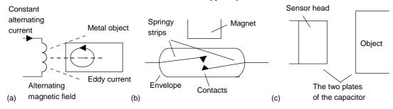
Figure 2.5 Proximity switches: (a) eddy current, (b) reed switch, (c) capacitive
