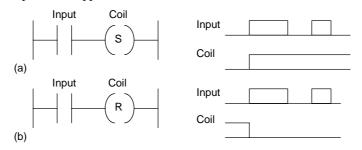
Figure 7.12 (a) SET and (b) RESET coils
