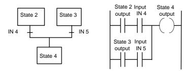
Figure 6.17 Convergence: state 4 follows when either IN 4 or IN5 occur.
