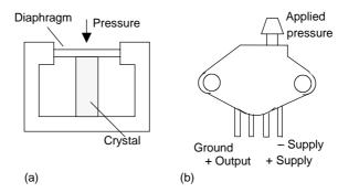
Figure 2.19 (a) Piezoelectric pressure sensor, (b) MPX100AP
