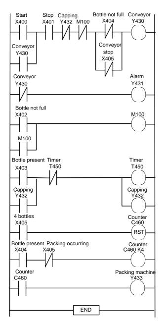
Y430 is the output to the conveyor. X400 is the start button, X401 the stop button - externally set closed. The conveyor is stopped by Y232, M100, X404 or X405 being activated.
