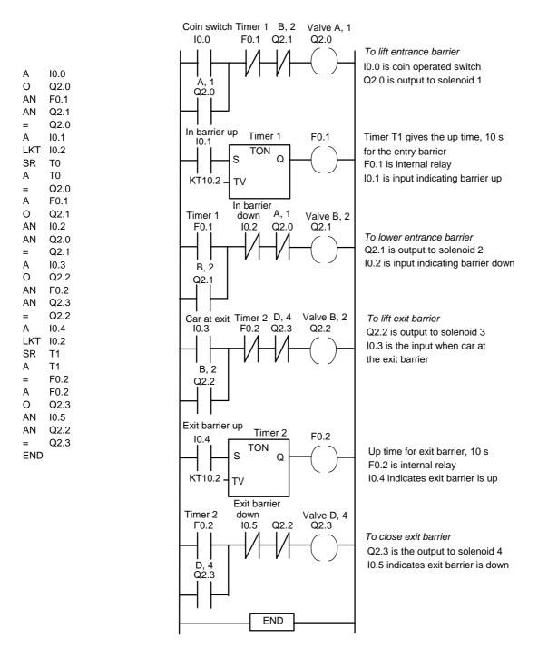
Figure 14.14 (b) Car barrier program, Siemens format
