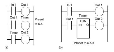
Figure 9.5 Sequenced outputs
