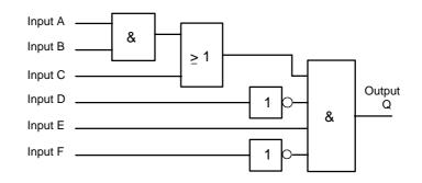
Figure 5.35 Logic diagram
