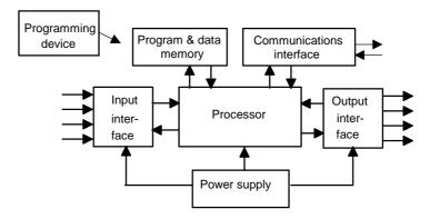
Figure 1.4 The PLC system
