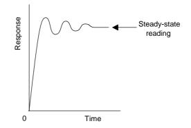
Figure 2.2 Response of a sensor or measurement system to a sudden input. You can easily see such a response when the current in an electrical circuit is suddenly switched on and an ammeter reading observed.
