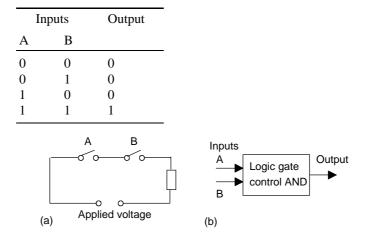
Figure 5.7 (a) AND circuit, (b) AND logic gate
