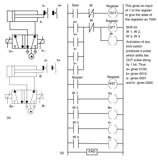
Figure 11.6 Sequencing cylinders
