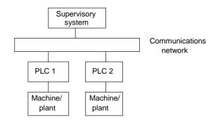
Figure 1.6 Basic communications model
