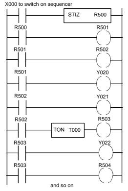
Figure 10.14 Sequencer with a Toshiba PLC
