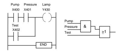
Figure 5.37 Signal lamp task
