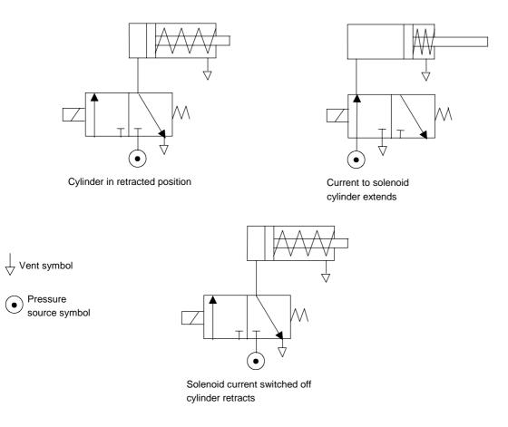
Figure 2.29 Control of a single-acting cylinder
