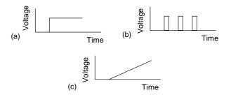
Figure 1.5 Signals: (a) discrete, (b) digital, (c) analogue
