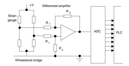
Figure 4.16 Signal conditioning with a strain gauge sensor
