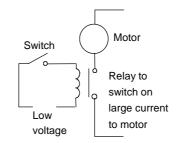
Figure 1.2 A control circuit
