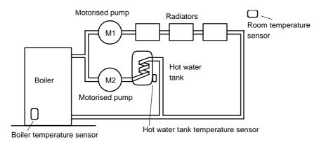
Figure 14.5 Central heating system
