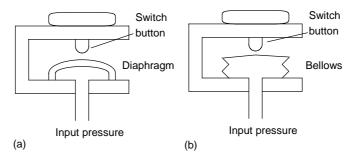
Figure 2.20 Examples of pressure switches
