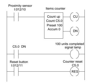
Figure 14.16 Conveyor belt counting of products
