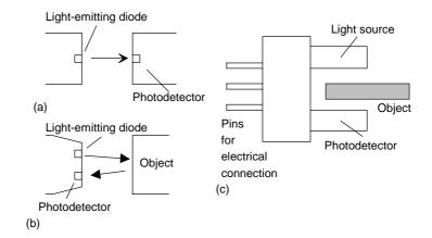
Figure 2.6 Photoelectric sensors
