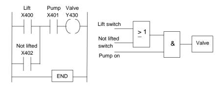
Figure 5.38 Valve operation program
