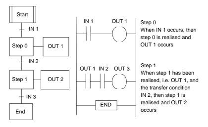
Figure 6.13 SFC and equivalent ladder diagram
