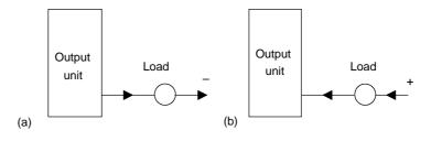
Figure 4.6 Output unit: (a) sourcing, (b) sinking
