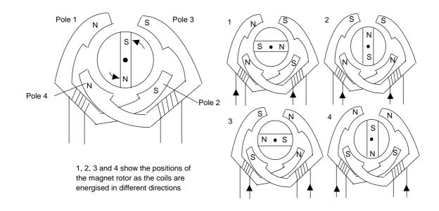
Figure 2.35 The basic principles of the permanent magnet stepper motor (2-phase) with 90° steps
