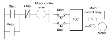
Figure 13.6 An unsafe stop system
