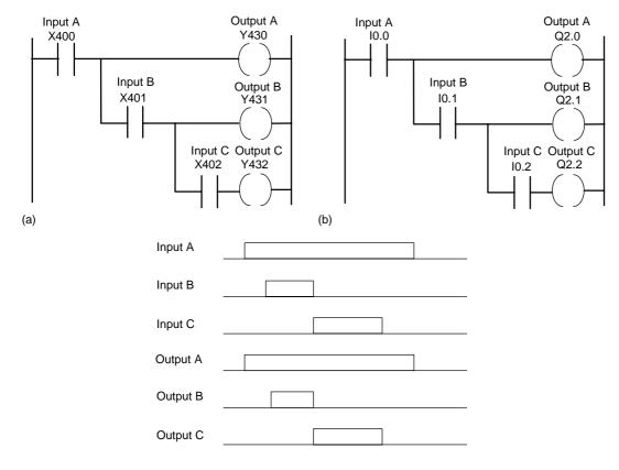
Figure 5.22 Sequenced outputs
