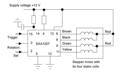
Figure 2.38 Driver circuit connections with the integrated circuit SAA1027
