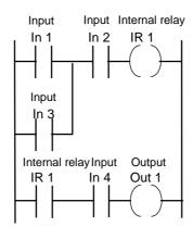
Figure 7.2 Internal relay
