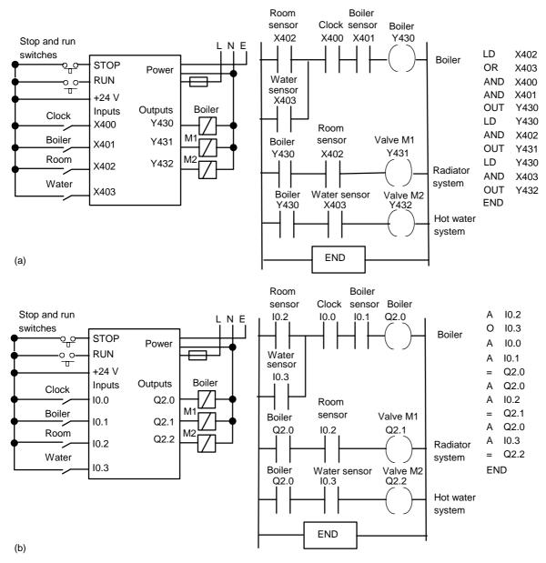
Figure 14.6 Central heating system: (a) Mitsubishi, (b) Siemens
