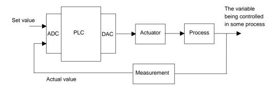
Figure 12.11 PLC for closed-loop control
