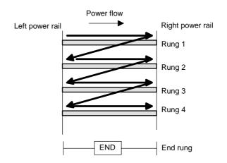
Figure 5.3 Scanning the ladder program
