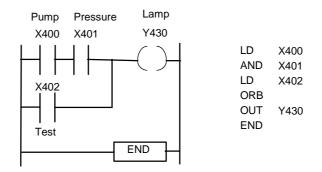
Figure 6.8 Signal lamp task
