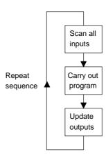
Figure 4.30 PLC operation
