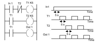
Figure 9.8 *On-off cycle timer*
