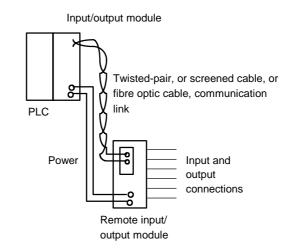
Figure 4.17 Use of remote input/output module
