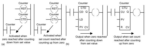
Figure 10.1 Forms of representation of counters. In (a) RST is reset. In (b), the IEC 1131-3 representation, CD is count down input, LD is for loading the input, PV is for the preset value, CV the current count value, CU is count up input, and R is for the reset input.
