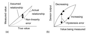
Figure 2.1 Some sources of error: (a) non-linearity, (b) hysteresis
