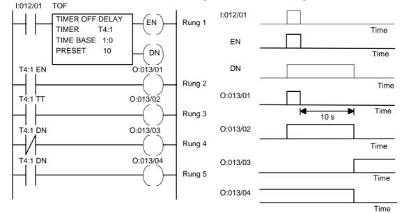
Figure 9.12 Application of an off-delay timer
