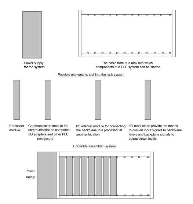
Figure 1.15 A possible arrangement of a rack system, e.g. the Rockwell Automation, Allen-Bradley PLC-5
