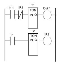
Figure 9.9 *On–off cycle timer*
