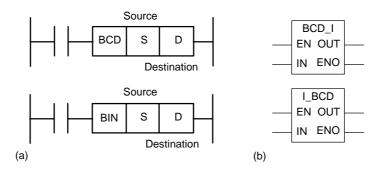
Figure 12.7 Conversion: (a) BCD-to-binary and binary-to-BCD, (b) BCD-to-integer and integer-to-BCD
