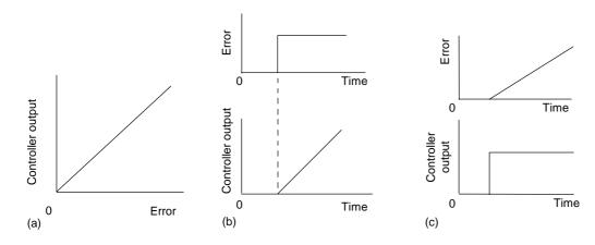
Figure 12.12 Control: (a) proportional, (b) integral, (c) derivative
