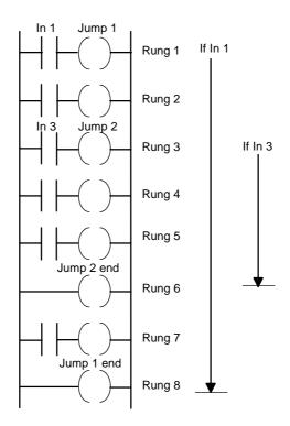
Figure 8.4 Jumps within jumps
