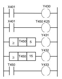
Figure 12.6 Sequential switching on
