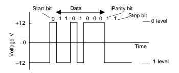
Figure 4.21 RS232 signal levels
