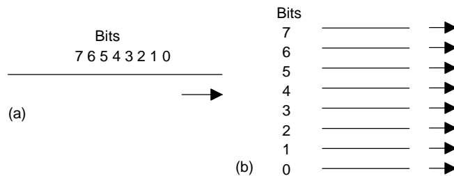
Figure 4.19 (a) Serial communication , (b) parallel communication
