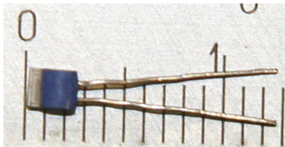
Figure 3.11 Simple sensor—PT100 (thin-film RTD)
