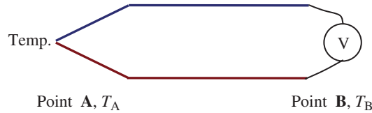
Figure 3.9 Principle of the thermocouple
