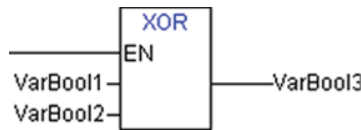
Figure 9.18 A function with EN input
