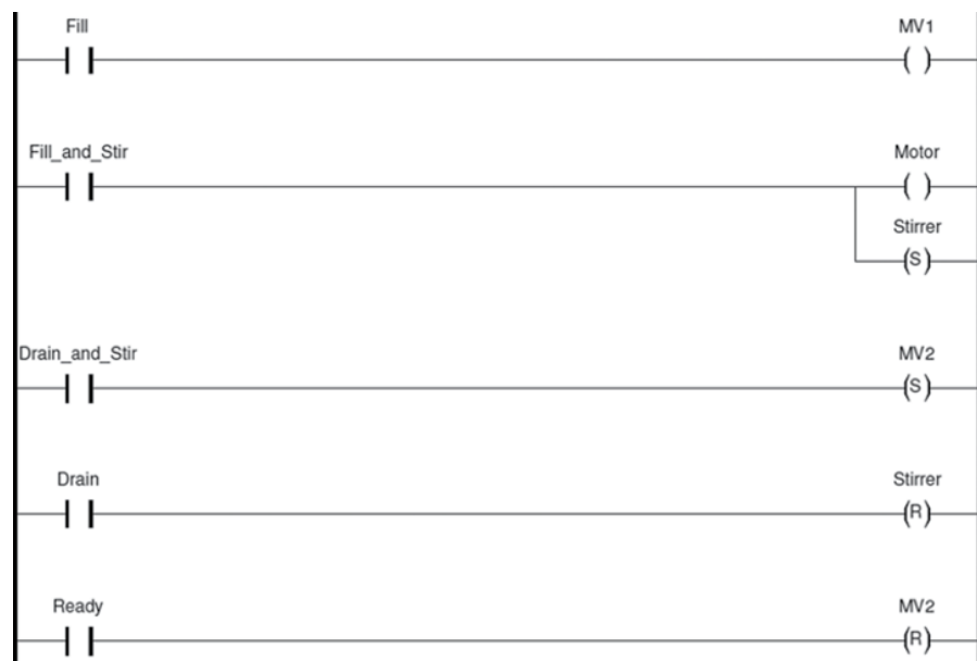
Figure 9.25 Program code based on the state flags
