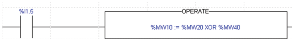
Figure 9.20 Integration of functions by use of a text-based block
