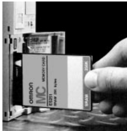
Figure 4-24. A removable memory card for a miniprogrammer.
