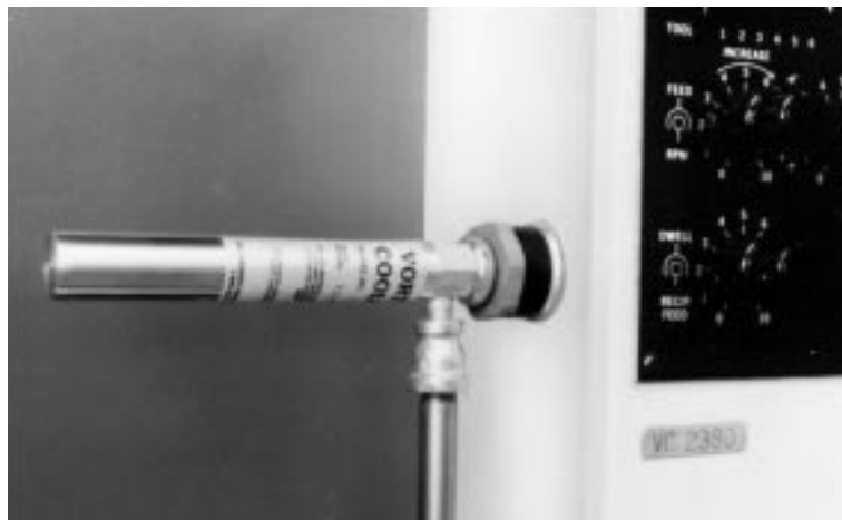
Figure 20-12. Vortex cooler used in cooling systems.
