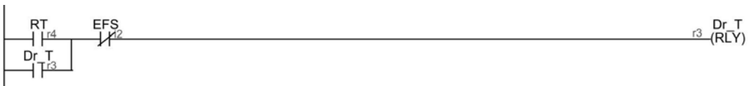
Figure 9-34 Transition logic for the drain tank state of the chemical treatment system
