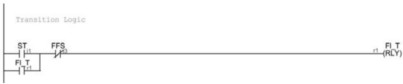
Figure 9-31 Transition logic for the fill tank state of the chemical treatment system
