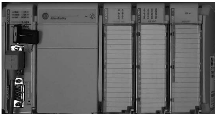
Figure 8-1 Picture of a PLC
