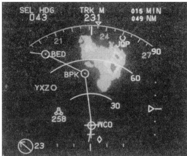
Figure 1.4 Computer-controlled displays in the glass cockpit. This figure illustrates the primary navigation display (or horizontal situation indicator) that the pilot uses to determine the direction in which the aircraft is traveling (in this case 231°—approximately south-west). In addition to the heading, the display indicates the position and density of cloud and the location of radio beacons. The three arcs indicate range from the aircraft (30, 60, 90 nautical miles).
