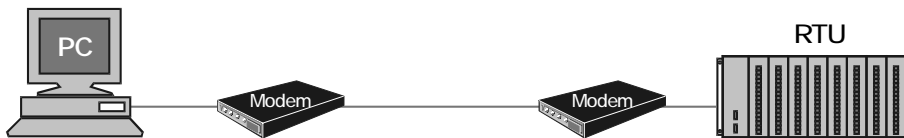
Figure 1.7 PC to RTU using a modem
