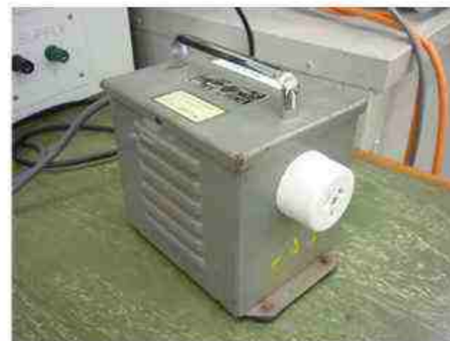
Page 265 Isolation transformer
