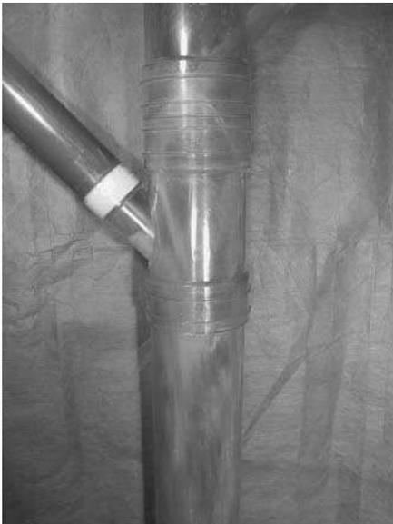
**Figure 4.13** Example of flow from a waste branch into a vertical stack. Internal view illustrates the reduction in air path cross section at and below the discharging branch (Courtesy of Heriot-Watt University)
