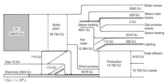
Figure 30.1 A typical Sankey diagram for a dyehouse
