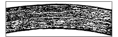
Figure 58.12 Failure due to rough pulley sidewalls
