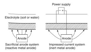
Figure 53.9 Cathodic protection
