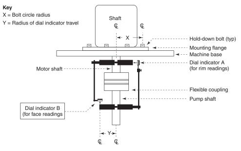
Figure 54.26 Determining bolt circle radius and radius of dial indicator travel
