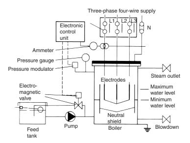
Figure 23.1 Diagrammatic layout of electrode boiler
