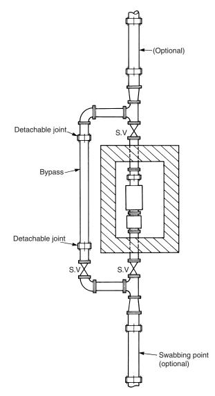
Figure 4.12 Standard bulk meter layout for a brick-built chamber (230 mm brickwork on a concrete base). *Notes:* (1) the flowmeter should be either on straight or bypass to suit specific site (i.e. to keep meter off road). (2) Chamber cover should be approximately 685 mm  $\times$  510 mm
