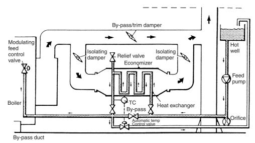
Figure 25.6 Typical installation layout
