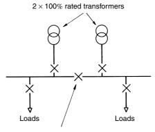
(a) Bus section switch, normally closed
