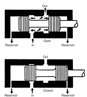
Figure 40.25 Two-way sliding spool valve
