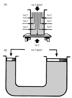
Figure 40.3 Effects of atmospheric pressure
