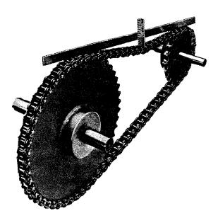
Figure 58.31 Proper technique to measure sag (Ref. 2)
