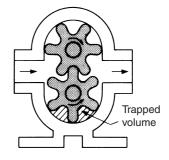
Figure 32.19 External gear pump
