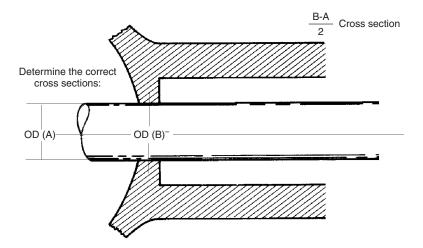
Figure 56.8 Selecting correct packing size
