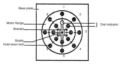
**Note**: Dial indicator B will be set up for taking face readings off of the lower bracket (as indicated by ). Readings will then be taken at positions indicated by .
