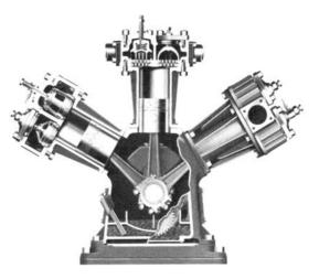
Figure 36.13 Three-piston compressor generates higher vibration levels
