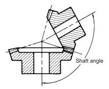
Figure 39.11 Shaft angle, which can be at any degree
