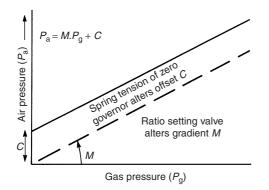
Figure 19.9 Relationship between air and gas pressures for crossloaded governor system
