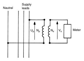
Figure 17.6 Voltage transformer
