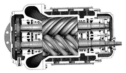
Figure 44.19 Single-stage screw compressor
