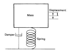
Figure 42.7 Mass/spring diagram
