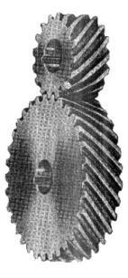
Figure 57.6 Typical set of helical gears
