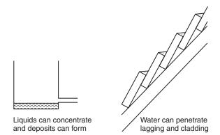
Figure 53.7 Details of design creating corrosion problems
