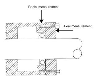
Figure 44.16 Measurement points should provide shortest direct mechanical link to shaft
