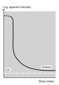
**Figure 52.10** Comparison of the apparent viscosities of a gear oil and a gear grease. The grease flows readily in the tooth-contact region, where shear stress is high, but resists leakage at seals and joints usually incorporated, and they are carefully selected to be compatible with both the poly-alkaline and the greasethickener system.
