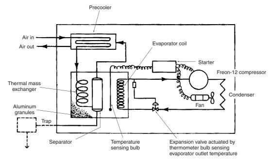
Figure 41.9 Diagram of equipment furnished in small self-contained direct-refrigeration dryer
