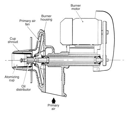
Figure 24.7 Section through rotary cup atomizer
