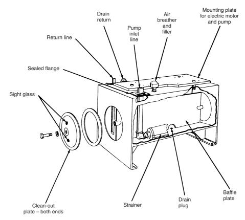
Figure 40.19 Non-pressurized reservoir
