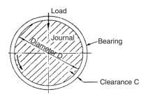
Figure 60.2 Plain cylindrical bearing
