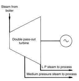
Figure 15.18 The double pass-out turbo-alternator
