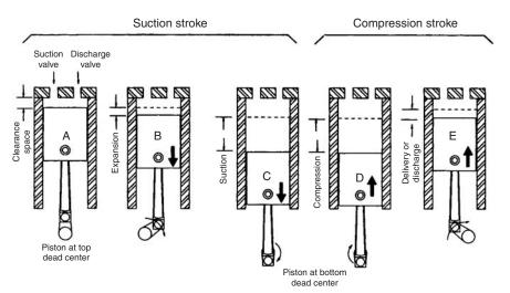
Figure 44.9 Two-cycle, or single-action, air compressor cylinders
