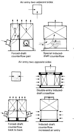
Figure 34.10 Configurations of cooling tower airflows
