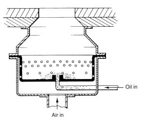
Figure 24.1 Vaporizing pot burner
