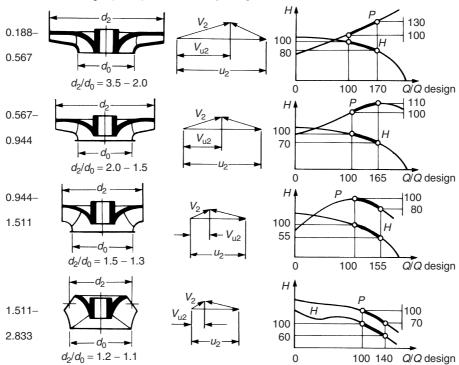
Figure 32.16 Flow path shapes, velocity diagrams and characteristics
