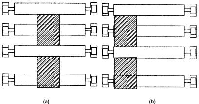
Figure 44.13 Rolls should be uniformly loaded
