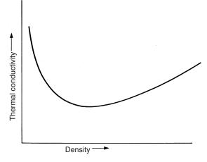
Figure 11.2 Typical relationship between thermal conductivity and density  $% \mathcal{F}_{\mathrm{rel}}(\mathcal{F})$
