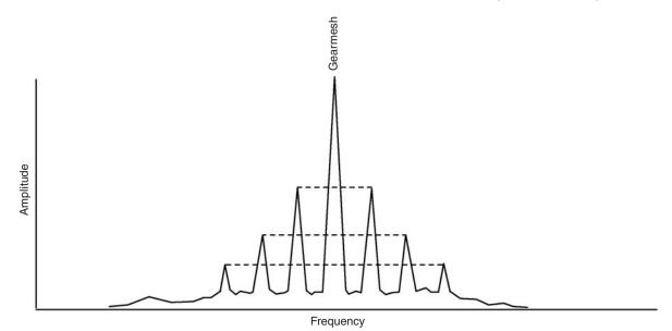
Figure 44.50 Normal gear set profile is symmetrical
