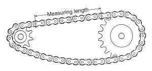
Figure 58.30 Illustration of recommended procedure for measuring chain length
