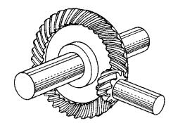
Figure 57.16 Spiral bevel gear
