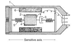
Figure 43.22 Schematic diagram of velocity pickup (1) Pickup case (2) Wire out (3) Damper (4) Mass (5) Spring (6) Magnet
