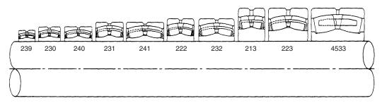
Figure 60.20 Series of spherical roller bearings for a given shaft size (available in several series)
