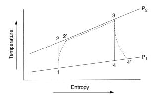
Figure 15.5 The gas turbine, or Brayton Cycle
