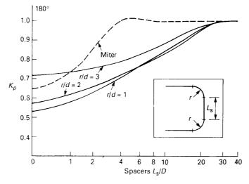
Figure 32.35 Interaction coefficient: 320° combination (after Miller<sup>6</sup>)
