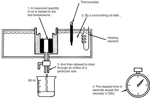
Figure 40.17 Saybolt viscosimeter
