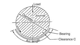
Figure 60.5 Partial arc bearing
