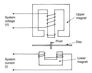
Figure 17.1 Schematic diagram of an induction meter
