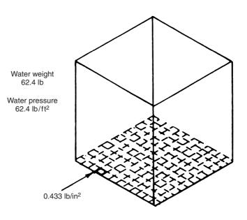
Figure 40.5 Water pressure in a 1-cubic foot container
