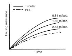
Figure 26.9 Effect of velocity and turbulence
