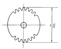
Figure 57.37 Using Method 2 to approximate the diametric pitch
