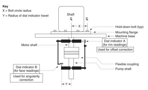
Figure 54.23 Bottom dial indicator in position to obtain "face readings" (Ref. 1)
