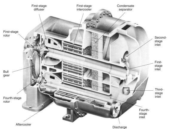
Figure 36.4 Bullgear centrifugal compressor
