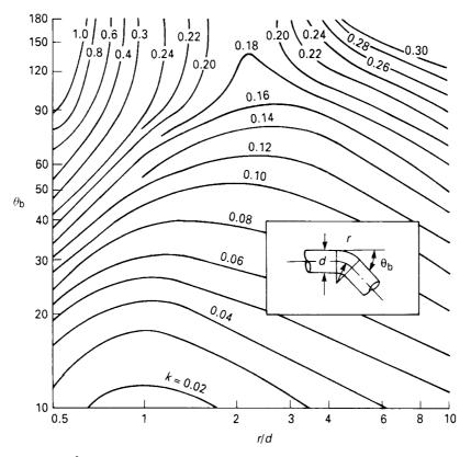
Figure 32.31 Bend loss coefficients<sup>6</sup>
