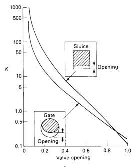
Figure 32.32 Gate valve losses<sup>6</sup>
