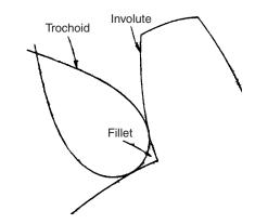
Figure 57.22 Involute tooth curve generated by straight-sided gear cutter
