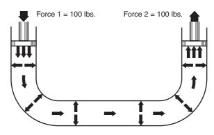
Figure 40.2 Transmission of forces
