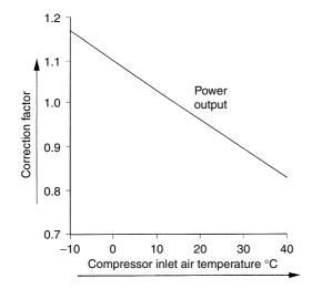
$\label{eq:Figure 15.6} \mbox{ Figure 15.6 Correction to gas turbine power output for changes in ambient temperature}$
