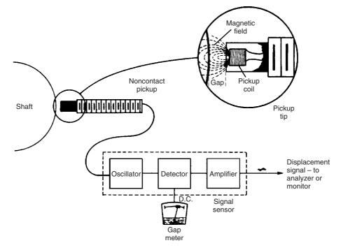
Figure 43.21 Displacement probe and signal conditioning system
