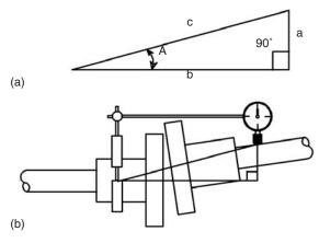
Figure 54.5 Common right triangle and simplified alignment-measuring apparatus
