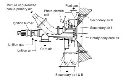
Figure 24.17 Pulverized fuel burner
