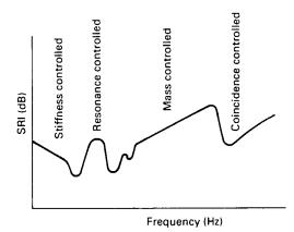
Figure 42.8 Typical insulation characteristics of a partition
