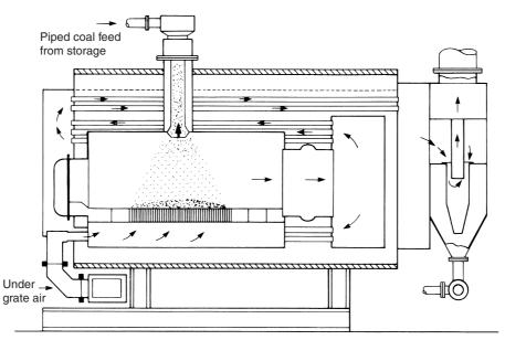
Figure 23.4 A fixed-grate coal-fired boiler
