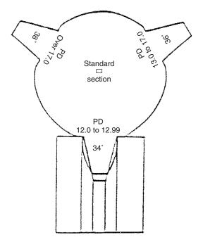
Figure 58.3 Illustration of a pulley groove gage
