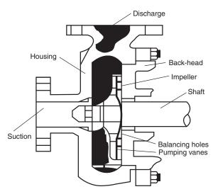
Figure 56.1 Cross-section of a typical end-suction centrifugal pump (Ref. 3)
