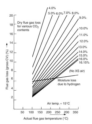
Figure 30.5 Flue gas losses - heavy fuel oil
