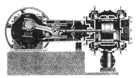
Figure 44.18 Typical cross-section of a reciprocating compressor
