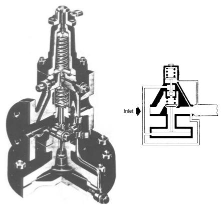
Figure 22.8 Pilot-operated reducing valve.
