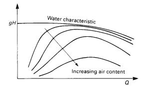
Figure 32.27 The effect of air content on pump behavior
