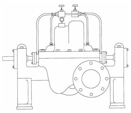
Figure 44.22 Typical horizontal split-case pump
