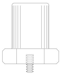
Stud mounted accelerometer
