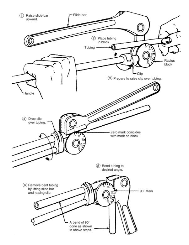
Figure 40.30 Bending tubing with hand-operated tube bender
