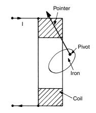
Figure 17.12 Moving-iron principle
