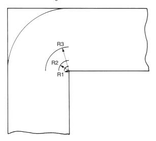
Figure 29.6 Splitters in miter bends
