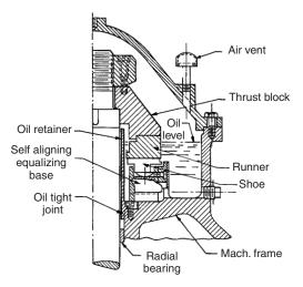
Figure 60.1 Half section of mounting for vertical thrust bearing
