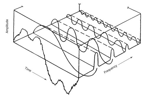
Figure 43.20 Relationship between time domain and frequency domain
