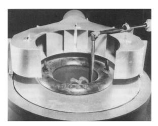
Figure 46.2 Captor-type claw hood for a furnace
