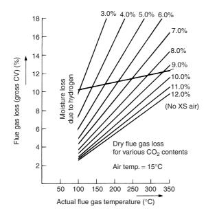
Figure 30.3 Flue gas losses - natural gas
