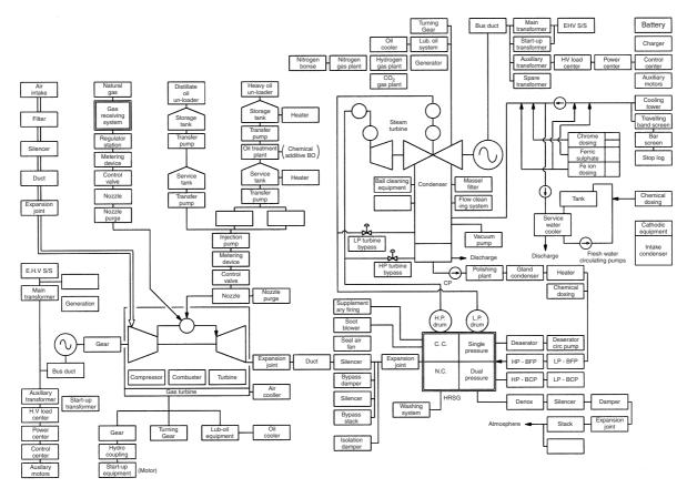
Figure 15.35 A typical combined-cycle power train
