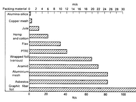
Figure 32.62 Soft packing - speed range
