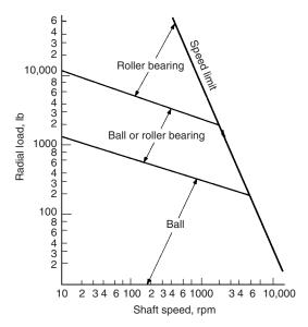
Figure 60.7 Guide to selecting ball or roller bearings
