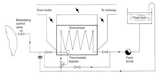
Figure 23.8 Schematic illustration of an installed economizer
