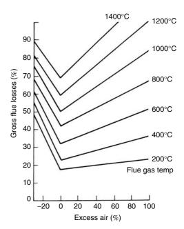
Figure 19.1 Gross flue losses versus excess air
