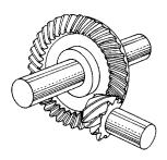
Figure 57.20 Hypoid bevel gear
