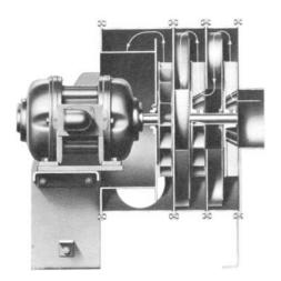
Figure 36.1 Cantilever centrifugal compressor is susceptible to instability
