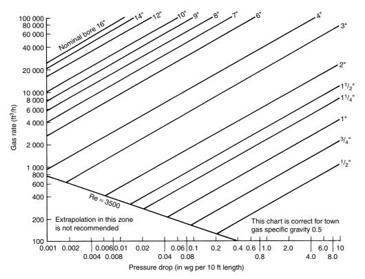
Figure 19.11 Chart for flow of town gas in pipes
