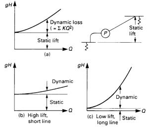
Figure 32.38 System loss characteristics
