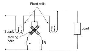
Figure 17.5 Schematic diagram of power factor meter
