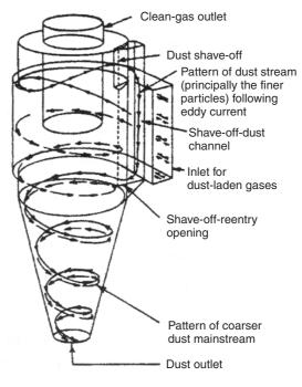
Figure 47.2 Flow pattern through a typical cyclone separator
