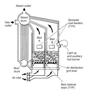
Figure 24.18 Fluid-bed combustion system with sectioned bed
