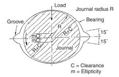
Figure 60.4 Elliptical bearing
