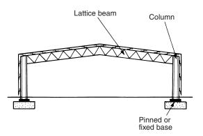
Figure 6.2 A typical lattice girder frame
