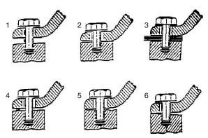
Figure 54.12 Diagrams of possible soft-foot causes (Ref. 3) 1. Loose foot, 2. Cocked foot, 3. Bad shims, 4. Debris under foot, 5. Irregular base surface, 6. Cocked foot
