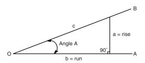
Figure 54.6 Concept of rise and run
