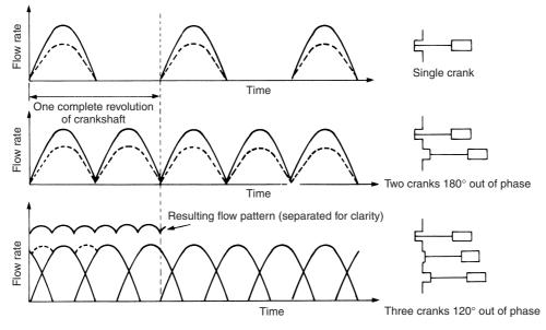
Figure 32.21 Reciprocating pump: variation of flow rate with numbers of cylinders
