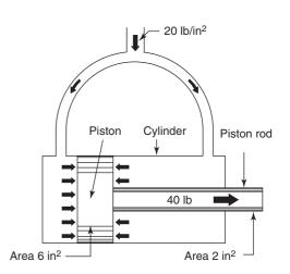
Figure 40.13 Differential areas on a piston
