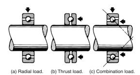
Figure 60.8 Three principal types of ball bearing loads
