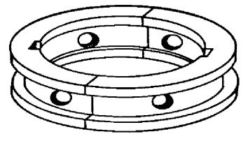
Figure 56.6 Lantern ring or seal cage
