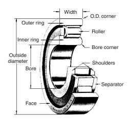
Figure 60.14 Cylindrical roller bearing
