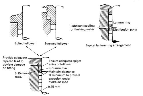
Figure 32.60 Stuffing box details
