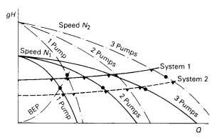
Figure 32.46 Variable-speed pumps in parallel
