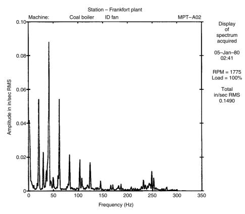
Figure 43.19 Typical frequency-domain signature
