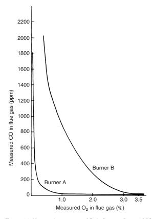
Figure 19.2 Measured percentage of  $O_2$  in flue gas. Range of CO versus  $O_2$  for a variety of burners
