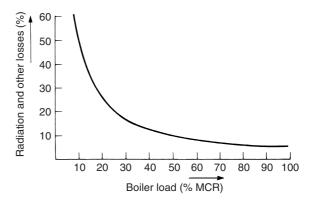
Figure 30.7 The variation in percentage radiation and other losses with the percentage boiler load factor
