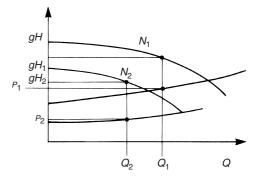
Figure 32.14 Prediction of speed change using equation (32.5)
