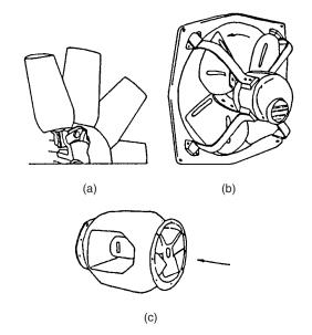
Figure 46.4 Axial-flow fans. (a) Axial flow; (b) propeller; (c) bifurcated
