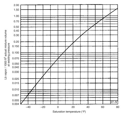
Figure 41.6 Moisture in air at any pressure for 100 ft<sup>3</sup> of actual volume at existing pressures
