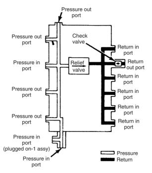
Figure 40.42 Fluid manifold flow diagram
