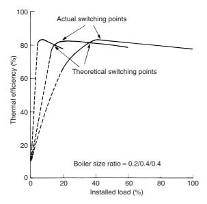
Figure 27.1 Evaluation of optimum boiler control
