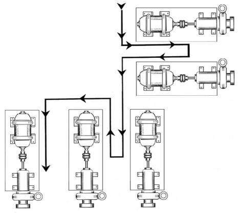
Figure 44.15 Typical measurement route
