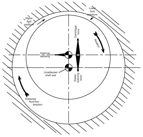
Figure 44.47 A normal Babbitt bearing has balanced forces
