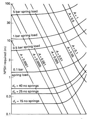
Figure 32.52 NPSH\_{required} for a reciprocating metering  $pump^7$
