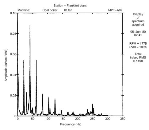
Figure 43.5 Typical frequency-domain vibration signature
