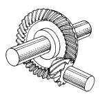
Figure 39.15 Hypoid bevel gear
