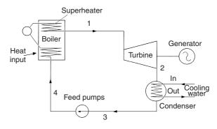
Figure 15.8 The condensing steam cycle
