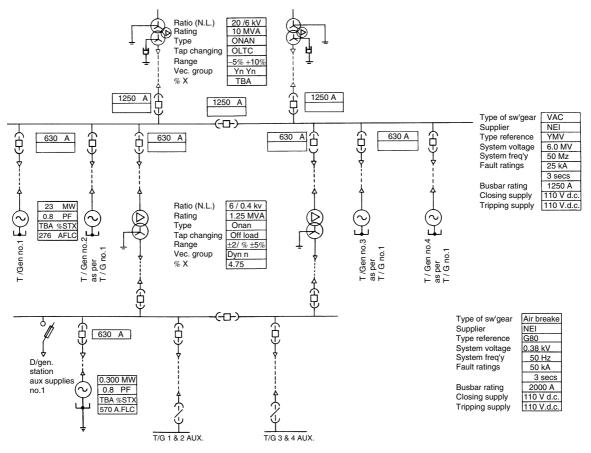
Figure 15.20 Typical electrical single-line diagrams for an 8MW power plant
