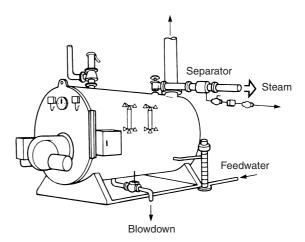
Figure 22.5 Boiler with separator at steam take off
