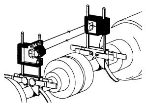
Figure 54.18 Typical optical or laser alignment system
