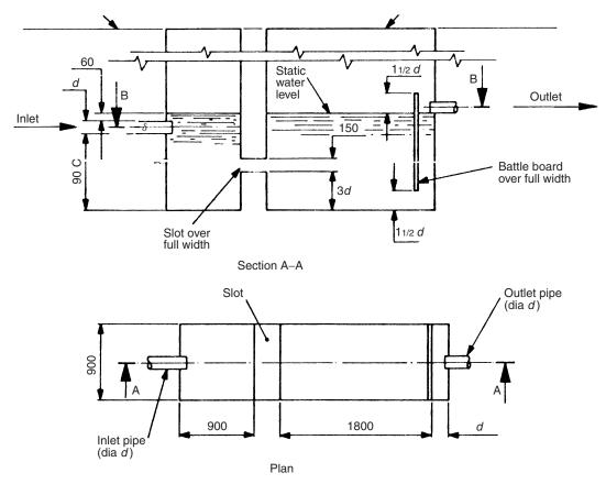
Figure 4.2 An alternative two-chamber gasoline interceptor. (Ventilation not shown: dimensions are in millimeters)
