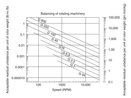
Figure 55.1 Balancing standards: residual imbalance per unit rotor weight (Ref. 5)
