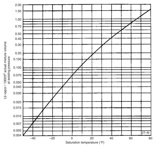
Figure 41.8 Moisture in air at any pressure
