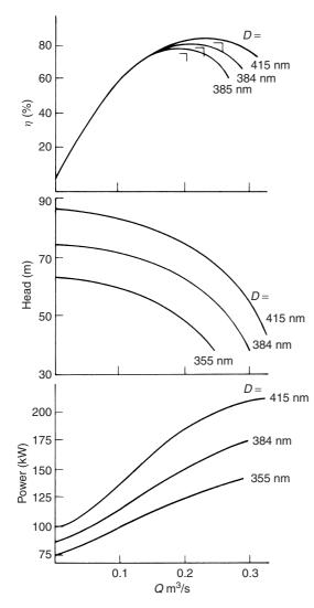
**Figure 32.17** Scaling laws applied to diameter change (after Karassik *et al*<sup>2</sup>.)
