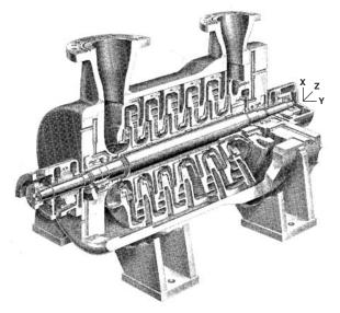
Figure 44.6 Typical in-line centrifugal compressor
