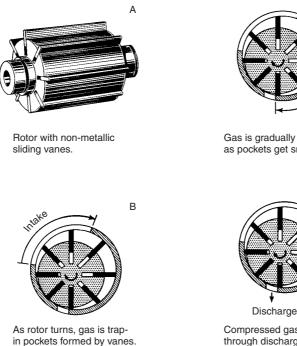
Figure 36.5 Rotary sliding-vane compressor
