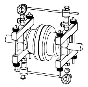
Figure 54.16 Typical reverse dial indicator fixture and mounting
