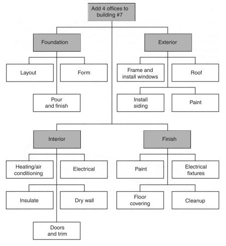
Figure 51.3 Sample work breakdown structure
