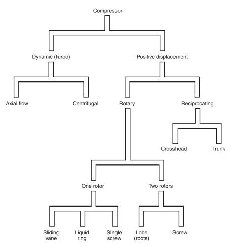
Figure 52.13 Compressor types
