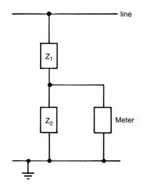
Figure 17.7 Voltage divider
