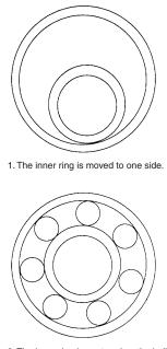
3. The inner ring is centered as the balls are equally positioned in place.
