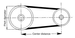
Figure 44.5 Pitch diameter and center-to-center distance between belt sheaves
