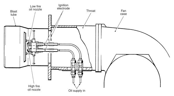
Figure 24.3 Combustion head pressure-jet burner
