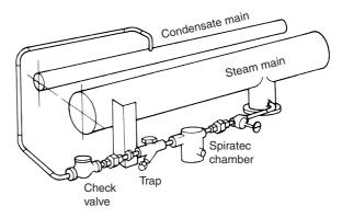
Figure 22.17 Flexible trapping arrangements
