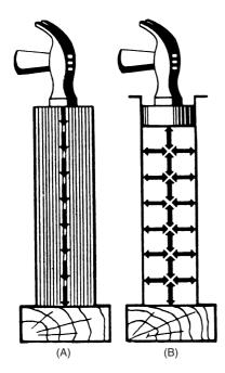
Figure 40.9 Transmission of force: (A) solid; (B) fluid
