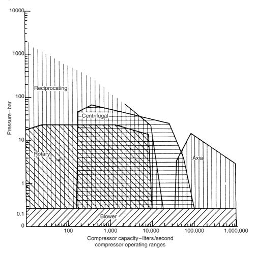
Figure 35.3 Compressor types - approximate capacity and pressure limitations
