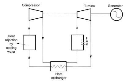
Figure 15.34 A closed-cycle gas turbine arrangement
