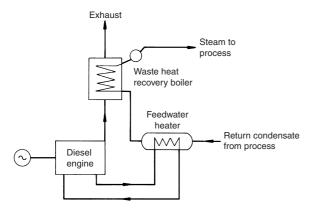
Figure 15.19 Diesel with waste heat recovery
