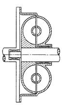
Figure 59.14 Typical hydraulic coupling
