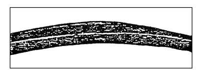
Figure 58.11 Failure due to substandard pulley diameter
