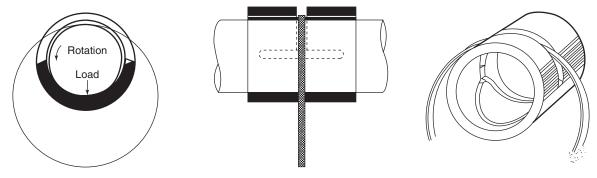
Figure 52.3 Ring oiled bearings
