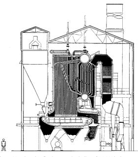
**Figure 23.5** A stoker-fired watertube boiler of 36,300 kg/h steam capacity at 28 bar and 385°C (from British Coal Publication, *Boiler House Design for Solid Fuel*, 1980, and kind permission from College of Fuel Technology)
