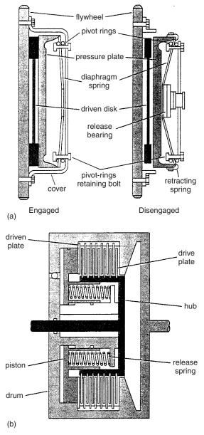
Figure 59.22 Friction clutch
