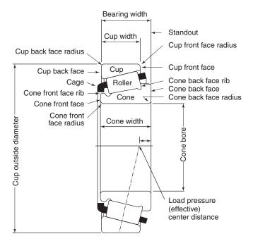
Figure 60.22 Information needed to identify a taper-roller bearing
