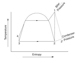
Figure 15.9 The Rankine Cycle with superheat
