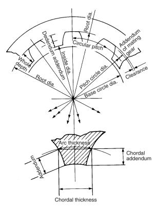
Figure 57.5 Parts of an internal spur gear
