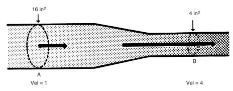
Figure 40.7 Volume and velocity of flow
