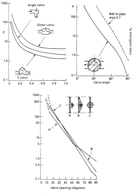
Figure 32.33 Some typical valve loss characteristics<sup>6</sup>
