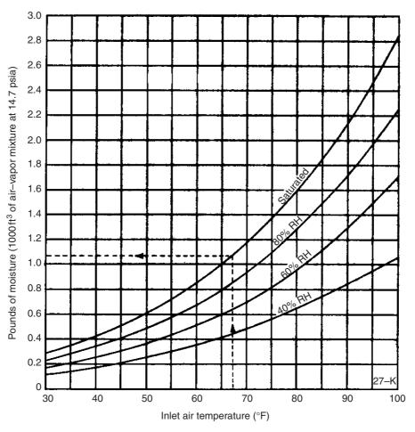
Figure 41.3 Effects of ambient temperature and relative humidity
