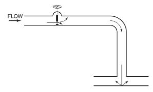
Figure 53.6 Areas affected by erosion corrosion
