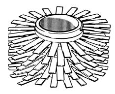
(b) Wound on - with turbulence inducing segments
