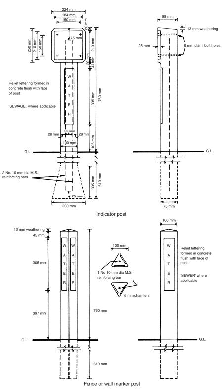
Figure 4.15 Pre-cast concrete indicator and marker posts
