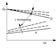
Figure 32.24 Effect of viscosity on positive displacement performance
