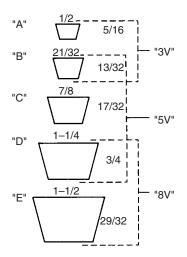
Figure 58.1 Nominal cross-section dimensions
