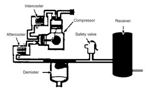
Figure 36.15 Safety valve function
