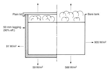
Figure 23.10 Heat losses from a feedwater tank operating at 93°C with ambient 21°C
