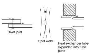
Figure 53.8 Details of jointing processes creating additional corrosion risks (crevices and stress concentrations)
