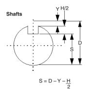
Figure 59.17 Shaft and hub dimensions
