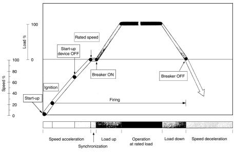
Figure 15.33 Gas turbine start-up and shutdown schedule
