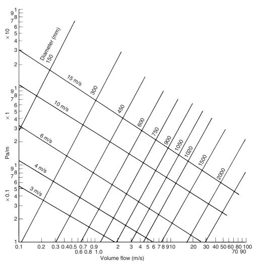
Figure 29.5 Pressure gradient in circular steel ducts
