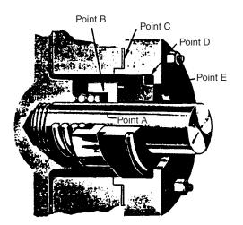
Figure 56.4 Pump stuffing box seal
