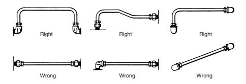
Figure 40.26 Correct and incorrect methods of installation
