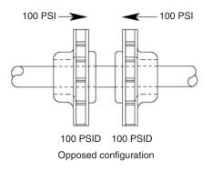
Figure 44.23 In-line and opposed impellers on multi-stage pumps
