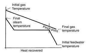
Figure 15.11 Heat-recovery diagram showing the pinch point
