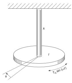
Figure 43.15 Torsional one degree-of-freedom system
