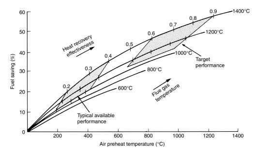
Figure 19.4 Fuel saving versus air preheat temperature
