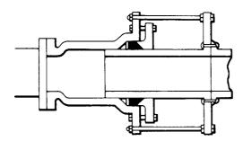
Figure 22.21 Sliding joint
