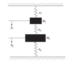
$\label{eq:Figure 43.16} \mbox{ Figure 43.16 Undamped two-degree-of-freedom system with a spring couple}$
