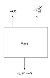
Figure 43.14 Damped forced vibration system
