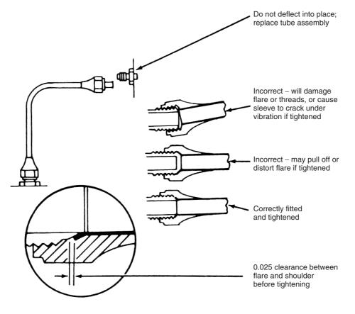
Figure 40.38 Correct and incorrect method of installing flared fittings
