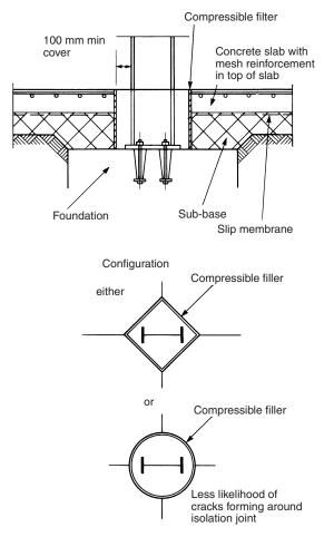
Figure 6.8 Isolation joint at foundation
