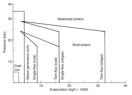
Figure 23.6 Guide to boiler capacities
