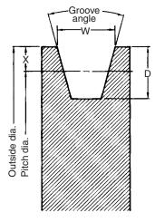
Figure 58.2 Typical pulley dimensions
