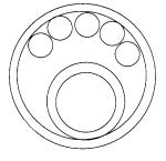
2. Balls are installed in the gap.
