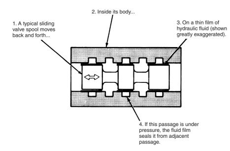
Figure 40.14 Fluid lubricates working parts
