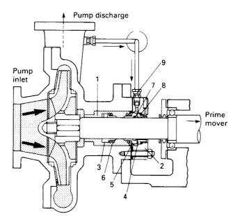
Figure 32.63 A typical mechanical seal installation. 1 Seal chamber; 2 seal plate; 3 spring sleeve; 4 seat; 5 seal ring; 6 spring; 7 dynamic secondary seal; 8 static secondary seal; 9 flush connection
