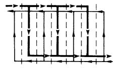
Figure 26.1 Single-pass operation
