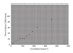
Figure 62.8 Normal hazard plot of generator fan failure data
