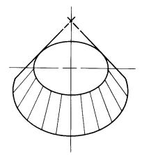
Figure 39.9 Basic cone shape of bevel gears
