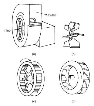
Figure 46.5 Centrifugal types of fan. (a) Centrifugal; (b) paddle or radial bladed; (c) forward curve; (d) backward curve
