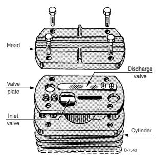
Figure 36.9 Finger valve configuration
