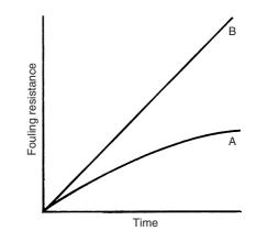
Figure 26.8 Build-up of fouling resistance
