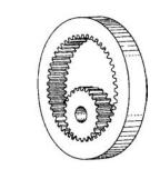
Figure 39.2 Example of an internal spur gear
