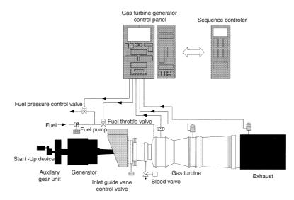
Figure 15.36 A gas turbine control system
