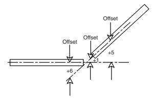
Figure 54.9 Offset measurement for angularly misaligned shafts
