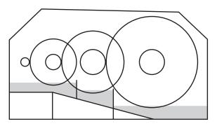
Figure 52.8 In a splash-fed gear the depth of immersion must be reasonably constant for all the gears, therefore the casing should incorporate stepped troughs for the oil
