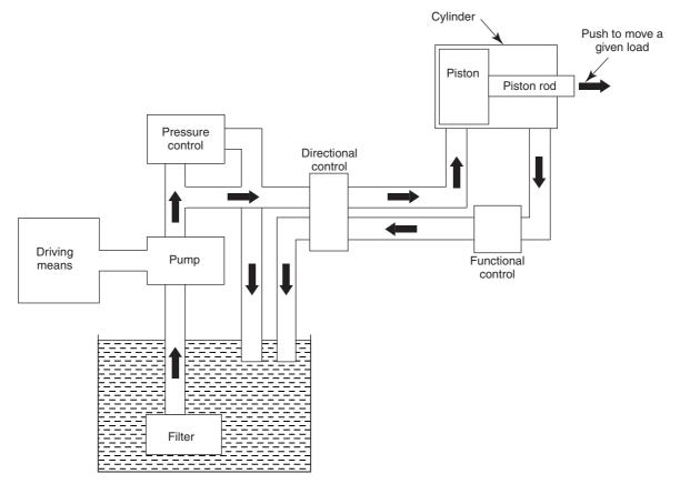
Figure 40.1 Basic hydraulic system
