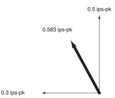
Figure 43.25 Resultant shaft velocity vector based on radial vibration measurements
