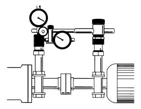
Figure 54.17 Typical configuration of a rim-and-face fixture (Ref. 2)
