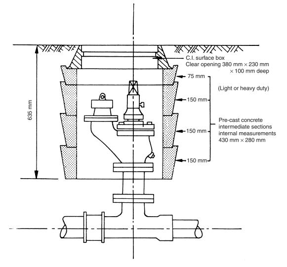
Figure 4.13 Standard pipe installations for a fire hydrant. *Notes:* (1) Hydrant Tee must be appropriate to type of main installed. (2) Depth of hydrant outlet must not exceed 300 mm below finished ground level. (3) Unless otherwise directed, pre-cast concrete units shall be bedded on well-compacted granular material Type A brought up from the base of the trench
