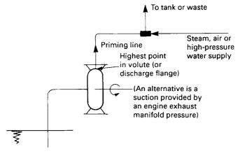
Figure 32.56 An ejector priming system
