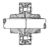
Figure 59.1 Typical flanged rigid coupling
