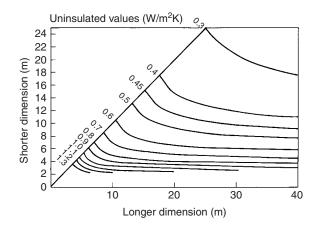
Figure 11.1 U-values of uninsulated solid concrete ground floors with four exposed edges. (Source: Eurisol UK, U-value Guide)
