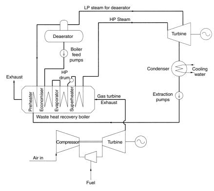
Figure 15.12 The single-pressure cycle diagram for a combined-cycle installation
