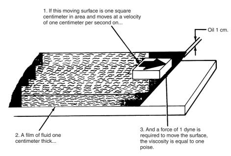
Figure 40.16 Measuring absolute viscosity
