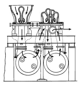
Figure 36.2 Airflow through a centerline centrifugal compressor
