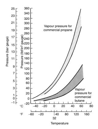
Figure 20.1 Vapor pressure/temperature curves for commercial propane and commercial butane
