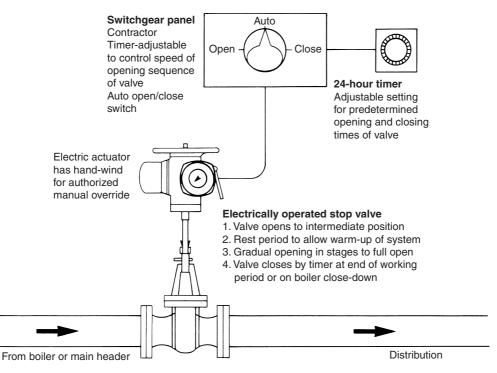
Figure 23.12 Diagram of electrically operated automatic steam stop valve (with permission of Hopkinsons Valves Ltd, Huddersfield, UK)
