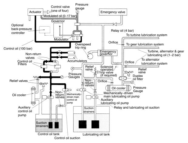
Figure 15.40 A control system for a speed-governed steam turbine
