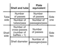
Figure 26.2 Comparison of pass arrangement: plate versus tubular
