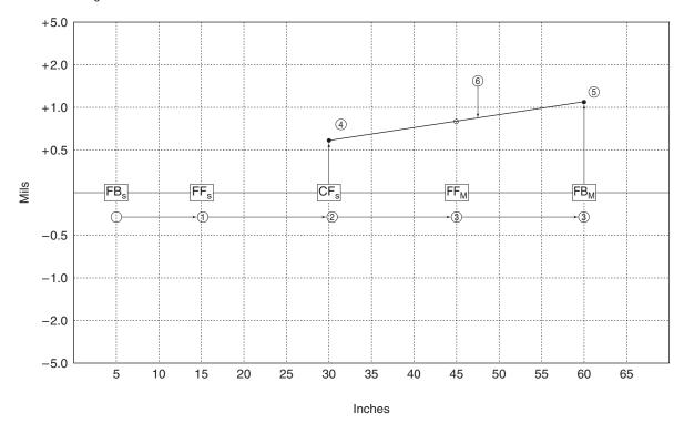
Figure 54.29 Graphical plotting of known foot correction
