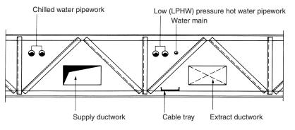
Figure 6.7 Typical services coordination through a lattice girder
