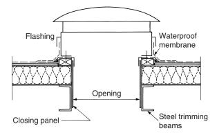
Figure 6.6 Typical roof penetration
