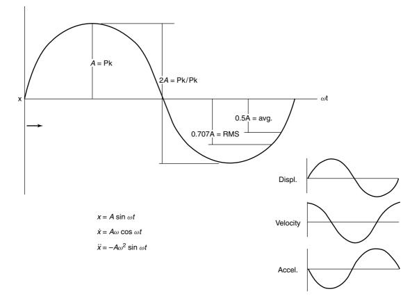
Figure 43.11 Relationship of vibration amplitude
