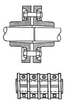
Figure 59.2 Typical split rigid coupling
