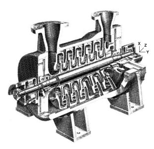
Figure 44.17 Multi-stage in-line compressors
