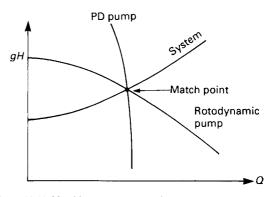
Figure 32.39 Matching constant-speed pumps to a system
