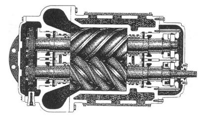
Figure 44.11 Screw compressor - steady-state applications only (Ref. 1)
