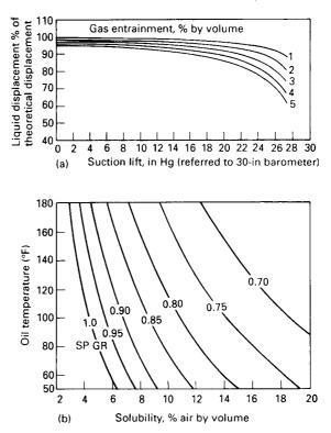
**Figure 32.29** (a) Effect of entrained gas on liquid displacement; (b) solubility of air in oil. *Example*: At 5 in Hg with 3% gas entrainment by volume, pump capacity is reduced to 84 per cent of theoretical displacement
