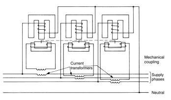
Figure 17.2 Three-phase meters
