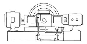
Figure 36.14 Opposed-piston compressor balances piston forces
