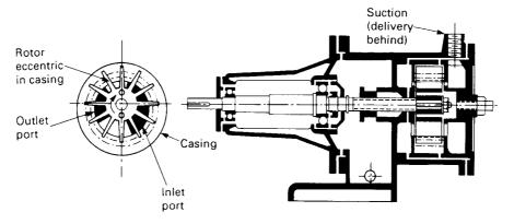
Figure 32.57 Schematic of a liquid ring pump
