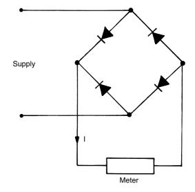
Figure 17.11 Full-wave rectification
