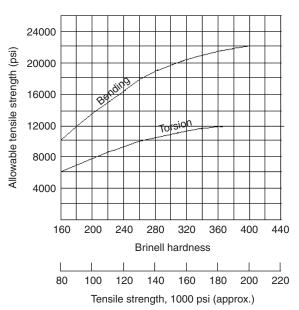
Figure 59.20 Allowable stress as a function of Brinell hardness
