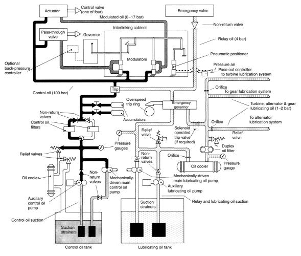
Figure 15.41 A control system for a pass-out steam turbine
