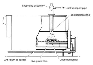
Figure 24.14 Fixed-grate coal burner with top feed
