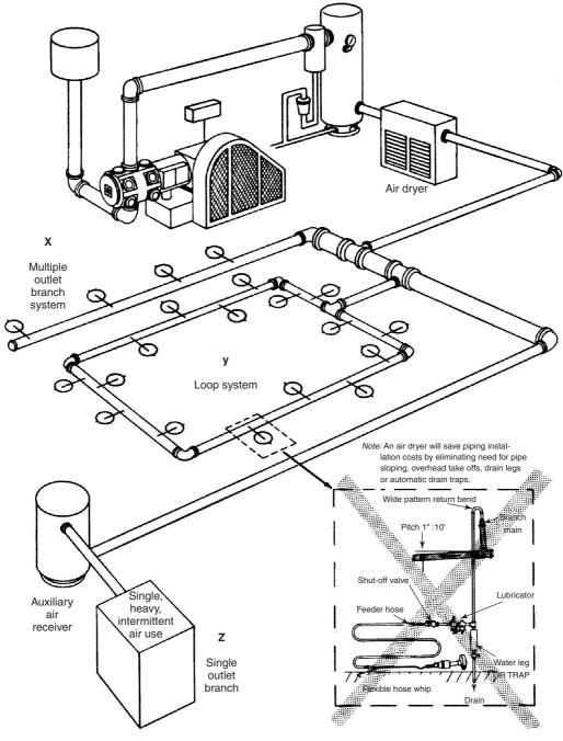
Figure 41.1 Typical compressed air supply
