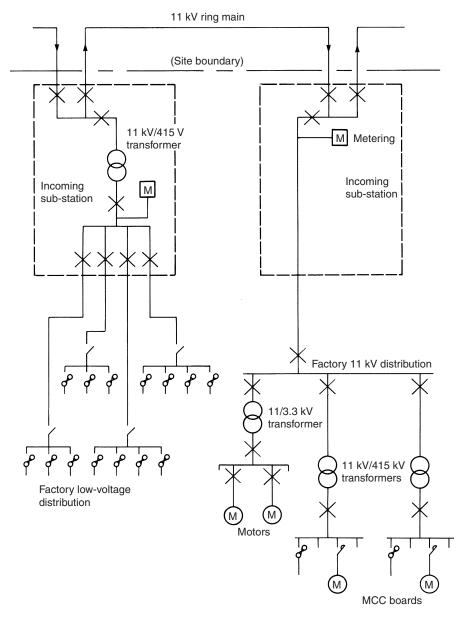
Figure 7.12 Typical power distribution system
