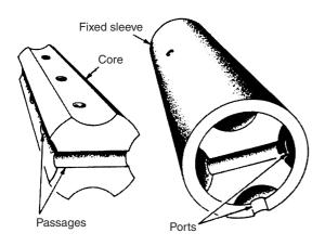
Figure 40.24 Parts of a rotary spool valve
