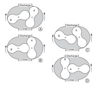
Figure 36.7 Helical lobe, or screw, rotary air compressor
