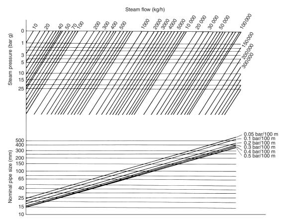
Figure 22.4 Pressure drop in steam lines
