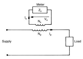
Figure 17.8 Current transformer
