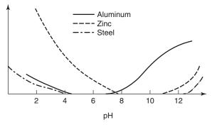
Figure 53.2 Variation in corrosion rate with pH
