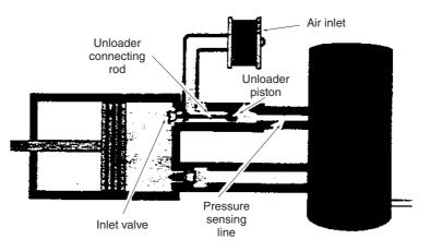
Figure 41.11 Typical hydraulic unloader and its location on the compressor
