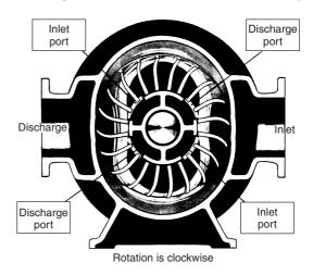
Figure 36.8 Liquid-seal ring rotary air compressor
