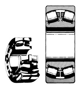
Figure 60.19 Spherical roller bearing assembly
