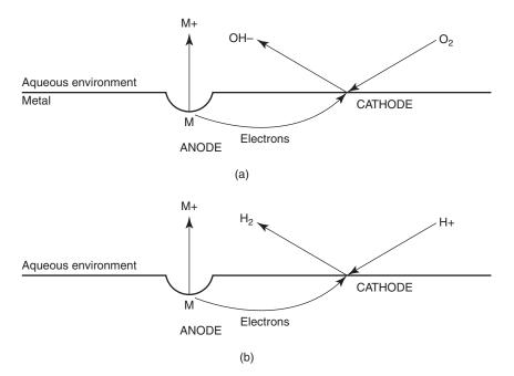
Figure 53.1 (a) Anodic, (b) Cathodic corrosion
