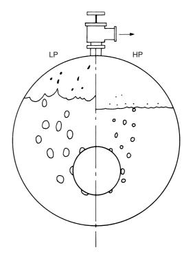
Figure 22.1 Boiler operation at low or high pressure
