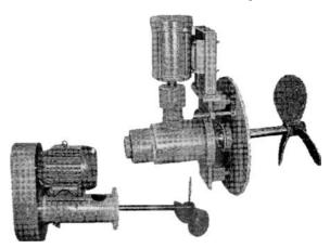
Figure 38.2 Side-entering propeller-type mixer
