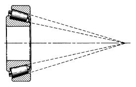
Figure 60.21 Taper-roller bearing
