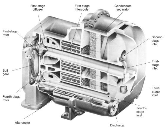
Figure 44.7 Cut-away of bullgear centrifugal compressor
