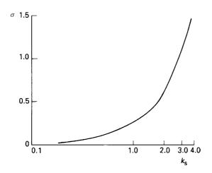
Figure 32.53 Variation of Thoma's cavitation parameter with specific speed for pumps<sup>3</sup>
