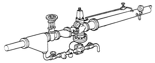
Figure 22.9 Pressure-control station
