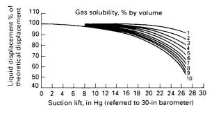
Figure 32.28 Effect of dissolved gas on liquid displacement
