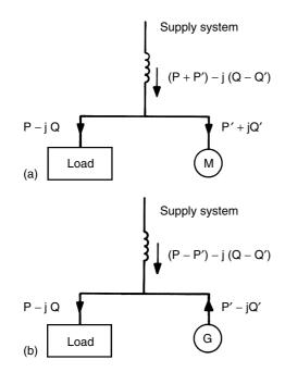
Figure 16.8 Synchronous machine operation. (a) Synchronous machine acting as a motor (over-excited); (b) synchronous machine acting as a generator (over-excited)
