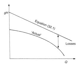
Figure 32.3 A pump's ideal and actual characteristics
