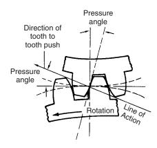
$\ensuremath{\textit{Figure 57.26}}$  Relationship of the pressure angle to the line of action
