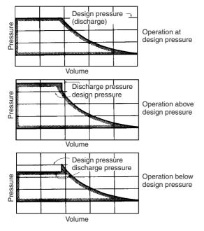
Figure 36.6 Theoretical operation curves for rotary compressors with built-in porting
