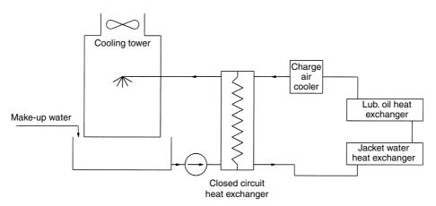
Figure 15.30 A typical closed-circuit secondary cooling system
