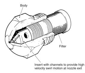
Figure 24.2 Pressure-jet nozzle
