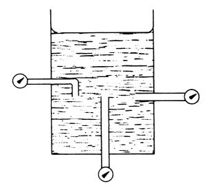
Figure 40.4 Pressure of a liquid is independent of direction
