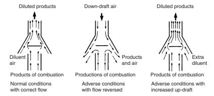
Figure 19.5 The function of the draft diverter
