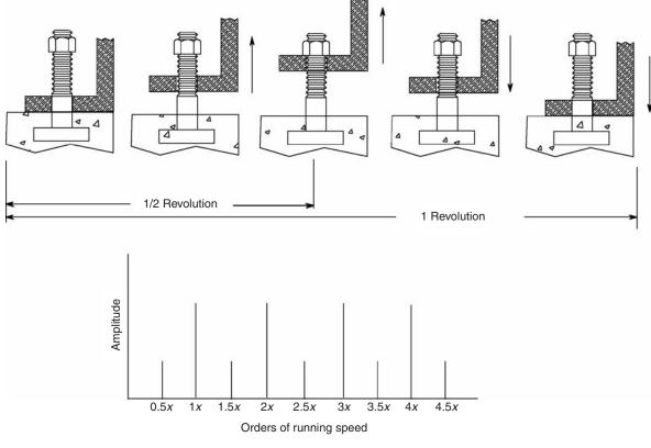
Figure 44.36 Multi-plane imbalance generates multiple harmonics
