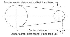
Figure 58.6 Distance required between pulleys
