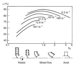
Figure 32.15 Variation of overall efficiency with non-dimensional specific  $\ensuremath{\mathsf{spec}}\xspace{\mathsf{d}}^3$
