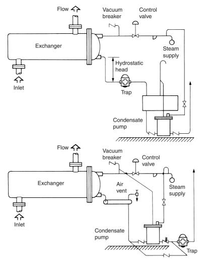
Figure 22.11 Lifting condensate drained from exchangers
