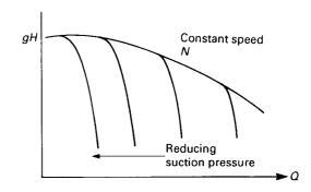
Figure 32.50 Effect of suction pressure on pump performance
