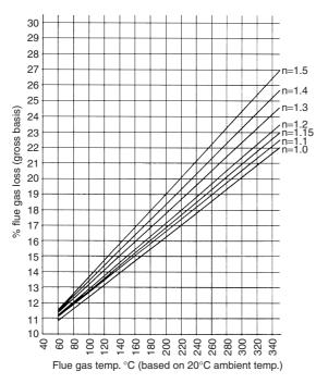
Figure 25.2 Total heat in gas-fired boiler exhaust
