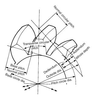
Figure 39.6 Helical gear and its parts
