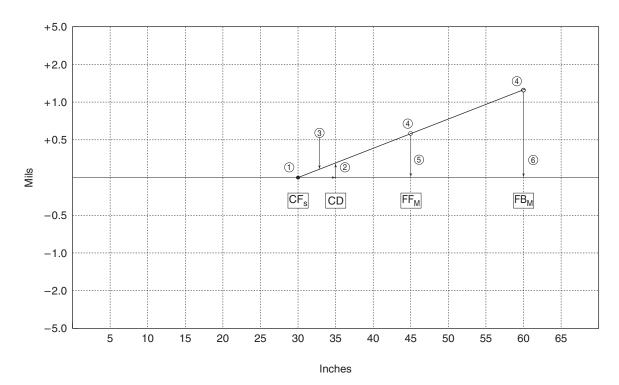
Figure 54.30 Graphical plotting of known coupling results
