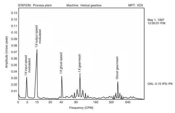
Figure 44.41 Difference modulation for a speed-increaser gearbox
