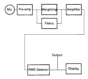
Figure 42.6 Schematic diagram of a sound level meter
