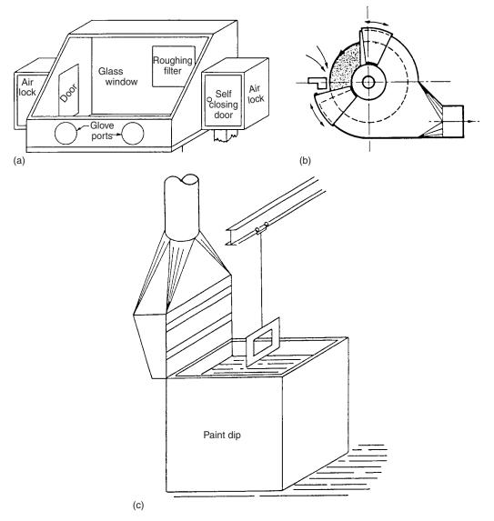
Figure 46.3 Types of hoods. (a) Enclosure; (b) receptor; (c) captor
