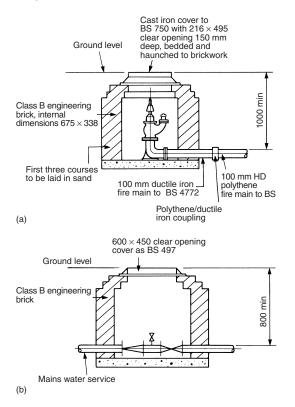
Figure 4.16 (a) Fire hydrant pit; (b) stop-valve pit. *Note:* To each fire hydrant an indicator plate with post must be provided and installed
