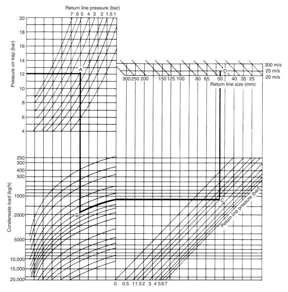
**Figure 22.14** Condensate line sizing chart where pressure at traps is above 4 bar (SI units). 1. From pressure upstream of trap move horizontally to pressure in return line (A). 2. Drop vertically to condensate load in kg/h (B). 3. Follow curve to RH scale and across to same return line pressure (C). 4. Move upward to return line flash velocity – say, 25 m/s maximum (D). 5. Read return line size.
