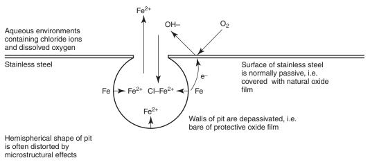
Figure 53.3 Pitting corrosion of stainless steel
