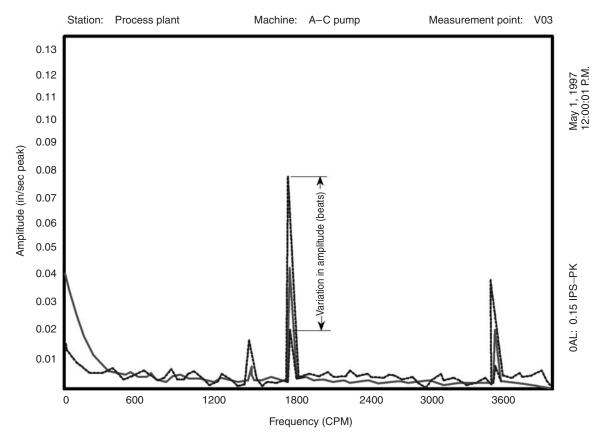
Figure 44.1 Vibration is dynamic and amplitudes constantly change
