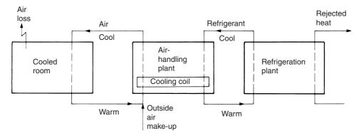
Figure 29.1 Heat flow paths in a direct expansion system
