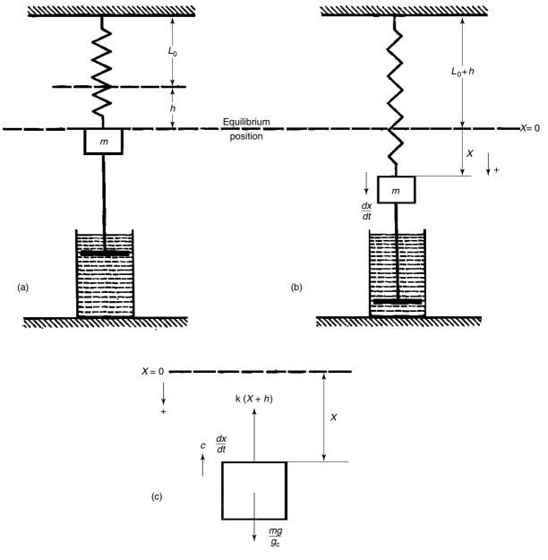
Figure 43.13 Damped spring-mass system
