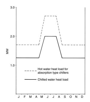
Figure 15.26 Chilled water heat load. The annual chilled water heat load is  $13\times10^6\,kWh$ ; the annual hot water heat load for absorption-type chillers is  $17.4\times10^6\,kWh$  (a COP of 75 per cent)
