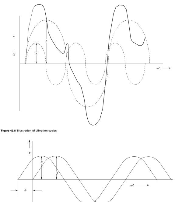
Figure 43.9 Two harmonic motions with a phase angle between them
