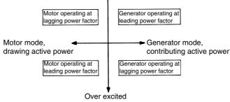
Figure 16.7 Synchronous machine operating modes
