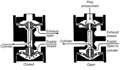
Figure 40.23 Operation of a simple poppet valve
