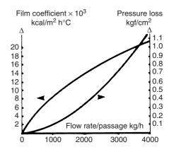
Figure 26.4 Performance details: plate exchanger
