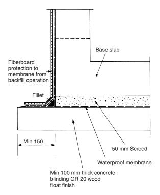
Figure 6.15 A typical external waterproof membrane detail
