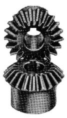
Figure 57.18 Miter gears with straight teeth
