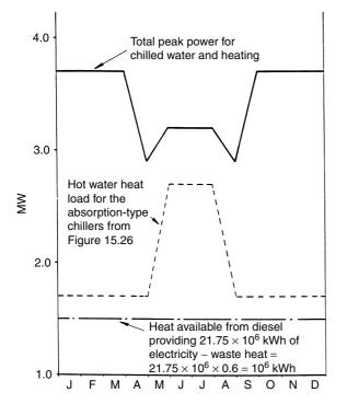
Figure 15.27 Total heat load. The heat available from the diesel waste gases of  $13\times10^6\,kWh$  will provide only a proportion of the heat required for the absorption-type chiller
