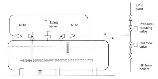
Figure 23.11 Diagrammatic layout of a steam accumulator
