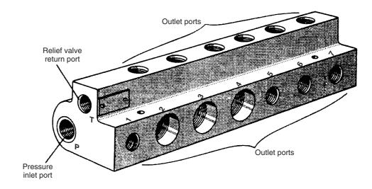
Figure 40.41 Fluid manifold
