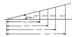
Figure 54.7 Rise/run measurements for constant angle
