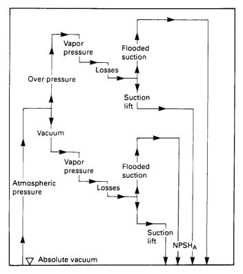
Figure 32.51 Visualization of  $NPSH_A$  (with acknowledgements to Girdlestone Ltd)
