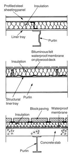
Figure 6.5 Typical roof constructions
