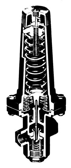
Figure 22.7 Direct-acting reducing valve
