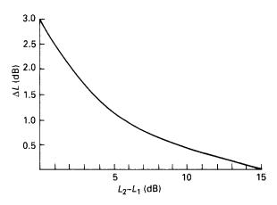
Figure 42.2 Noise-level addition graph
