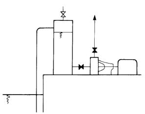
Figure 32.55 Priming tank arrangement
