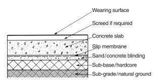
Figure 6.16 A typical section through a bearing slab
