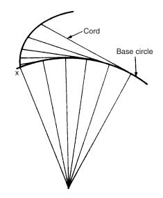
Figure 57.23 Theoretical generation of an involute tooth curve
