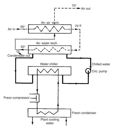
Figure 41.10 Diagram of a typical regenerative chiller-dryer
