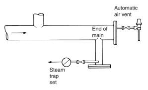
The capacity of a  $\frac{1}{2}$  in TD trap at 0.15 bar differential (2 lb/in<sup>2</sup>) is about 115 kg/h (255 pph) and this trap would have ample capacity.
