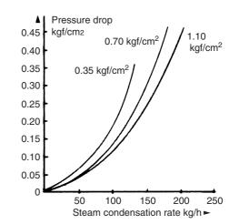
Figure 26.6 Steam-side pressure drop
