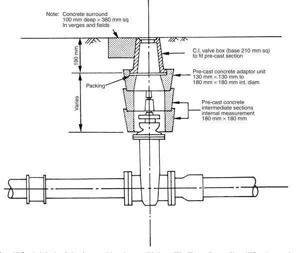
Figure 4.9 Standard pipe installations for water sluice valve up to 10 inches or 250 millimeter diameter. *Notes:* (1) If a valve extension spindle is required, a galvanized centering support must be provided. (2) Flanged valves with appropriate adapters must be used. (3) Unless otherwise directed, pre-cast concrete units shall be bedded on well-compacted granular material Type A brought up from the base of the trench
