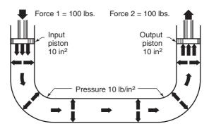
Figure 40.10 Force transmitted through fluid
