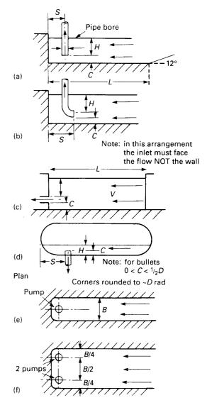
**Figure 32.48** Suction bay and tank proportions (based on reference 7). Possible suction arrangements: (a)–(c) open suction layouts commonly used; (d) tank intake system (recommended limits: 3 > (S/D) > 1; 2/3 > (C/D) > 1/2;  $(H/D) > [(V^2/3) + 1.5]$ ; [(L - S)/D] > 5; (e) single suction cell in plan (5 > (B/D) > 2; (f) double section cell in plan (4 < (B/D) < 10)
