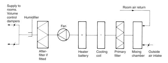
Figure 29.3 Airflow path in an air-conditioning system
