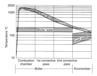
Figure 25.1 Temperatures in three-pass boilers and economizers
