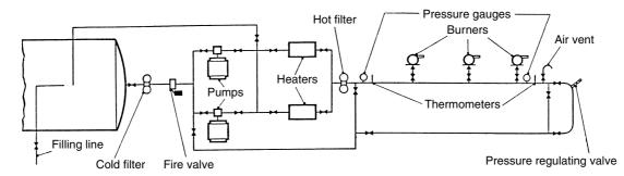
Figure 18.3 Typical hot oil ring main layout
