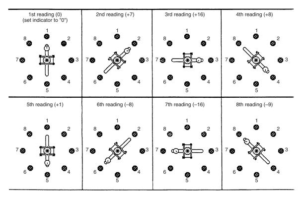
Figure 54.25 Determining the largest negative reading and the widest point
