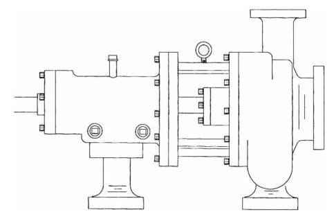
Figure 44.21 Typical end-suction, single-stage centrifugal pump
