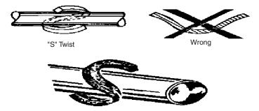
Figure 56.9 Proper and improper installation of packing
