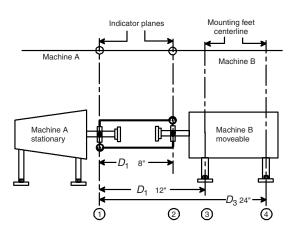
Figure 54.20 Reverse-dial indicator alignment setup
