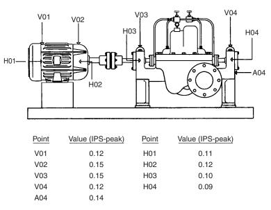
Figure 44.25 Typical broadband measurements
