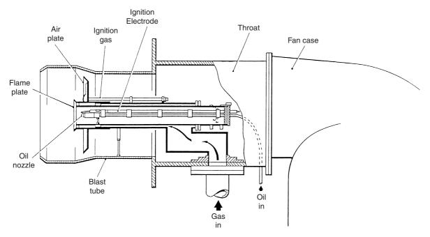
Figure 24.10 Dual-fuel burner based on pressure-jet configuration
