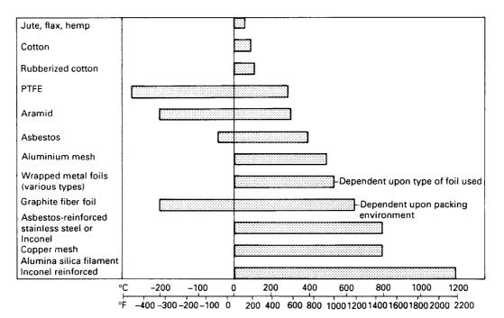
Figure 32.61 Soft packings – temperature range
