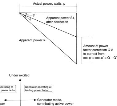
Figure 16.6 Power factor correction
