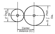
Figure 57.30 Pitch diameter and center distance
