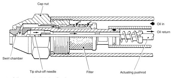
Figure 24.4 Spill return nozzle with tip shut-off needle
