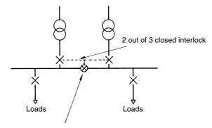
(b) Bus section switch, normally open
