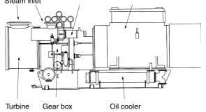
Figure 15.37 A single-stage steam turbine driving an alternator
