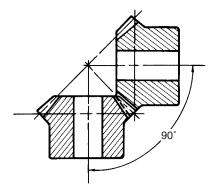
Figure 57.17 Miter gear shaft angle
