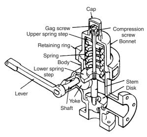
Figure 40.20 Cutaway of relief valve
