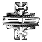
Figure 59.3 Typical compression rigid coupling
