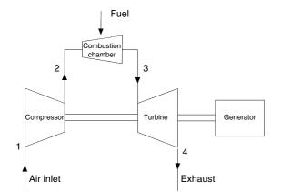
Figure 15.4 Basic gas turbine in open-cycle mode
