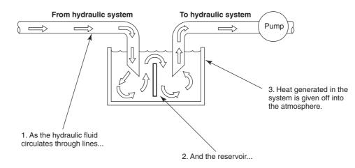
Figure 40.15 Circulating oil cools system
