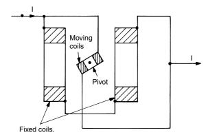
Figure 17.13 Schematic diagram of electrodynamics instrument
