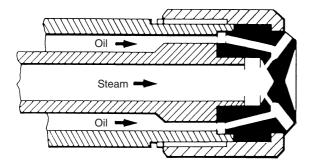
Figure 24.5 Steam-atomizing nozzle
