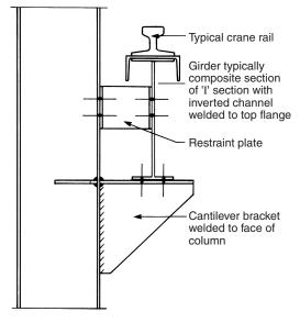
Figure 6.9 Crane gantry girder
