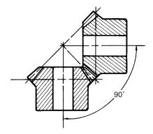
Figure 39.14 Miter gear shaft angle
