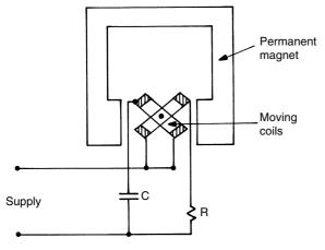
Figure 17.15 Frequency ratio meter
