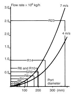
Figure 26.3 Throughput versus port diameter
