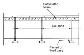
Figure 6.4 A typical multi-bay beam and post construction
