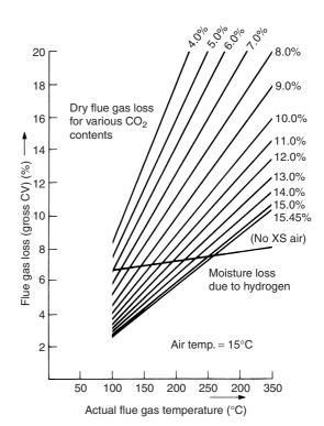
Figure 30.4 Flue gas losses – gas oil
