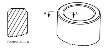
Figure 40.29 Properly burred tubing
