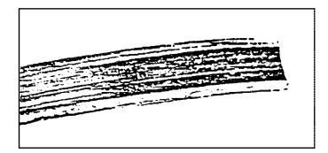
Figure 58.14 Failure due to belt rubbing guard
