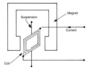
Figure 17.9 Moving-coil instrument
