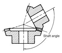
Figure 57.14 Shaft angle, which can be at any degree
