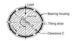
Figure 60.6 Tilting-pad bearing
