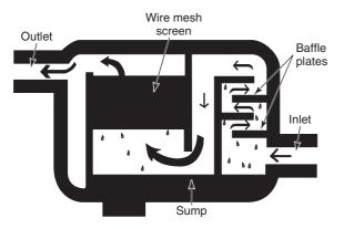
Figure 41.2 Basic oil separator system
