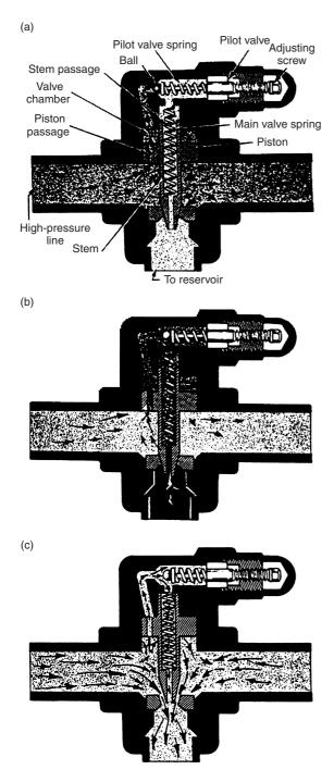
Figure 40.21 Hydraulic pressure regulator
