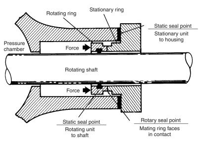
Figure 56.3 Simple mechanical seal
