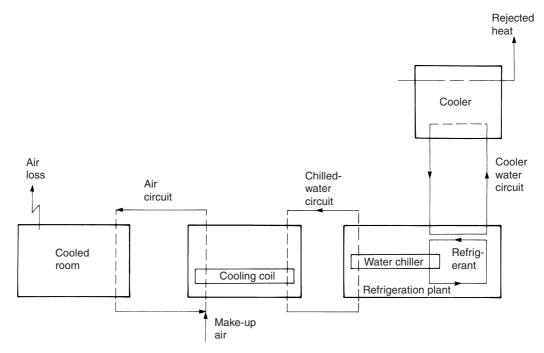
Figure 29.2 Heat flow paths in a chilled-water system
