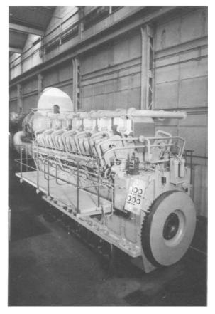
Figure 15.28 A Vee-12 diesel engine
