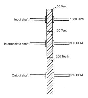
Figure 44.4 Double-reduction gearbox
