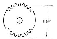
Figure 57.36 Using Method 1 to approximate the diametric pitch
