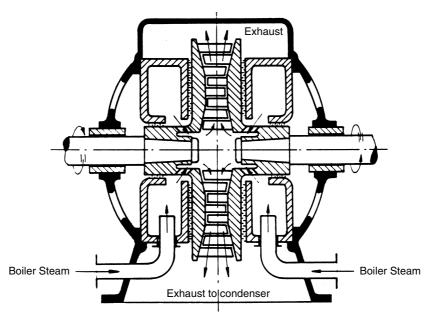
Figure 15.38 The radial-flow double-motion reaction turbine (Ljungström)
