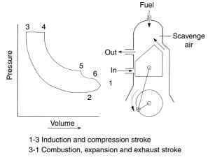
Figure 15.2 Two-stroke cycle for an internal combustion engine
