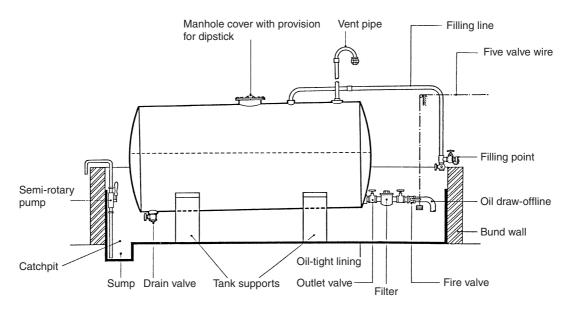
Figure 18.1 Typical storage tank for a distillate fuel oil
