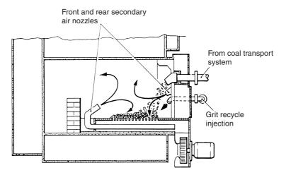
Figure 24.13 Fixed-grate coal burner with front feed
