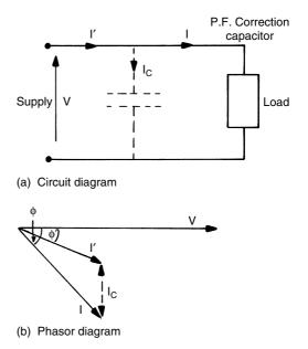
Figure 17.4 Power factor correction
