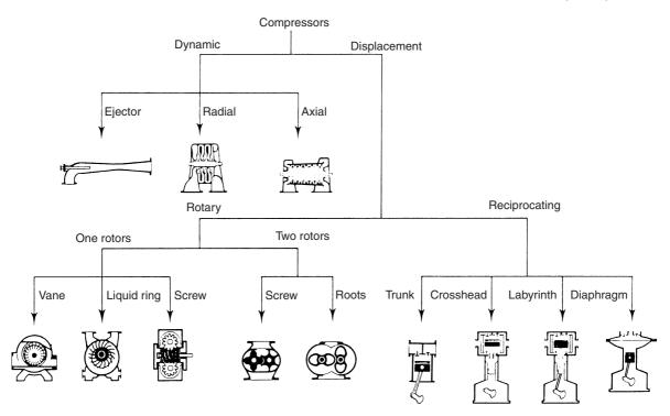
Figure 35.2 Basic compressor types
