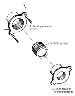
Figure 56.2 Typical packed stuffing box
