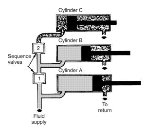
Figure 40.22 Installation of sequence valve
