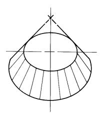
Figure 57.12 Basic cone shape of bevel gears
