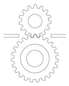
Figure 52.9 Oil is fed to some gears by jet or spray, so that the full benefits of lubrication and cooling are obtained precisely where they are needed. An extra jet at the 'exit' side of a meshing zone ensures that the teeth are cooled where the temperature is highest
