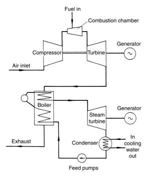
Figure 15.10 The gas turbine in combined cycle
