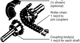
Figure 59.4 Typical chain coupling
