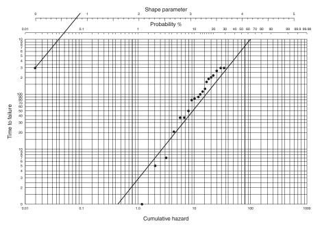
Figure 62.11 Weibull hazard plot of simulated Weibull data
