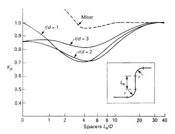
Figure 32.36 Interaction coefficient: S-bend combination (after Miller<sup>6</sup>)
