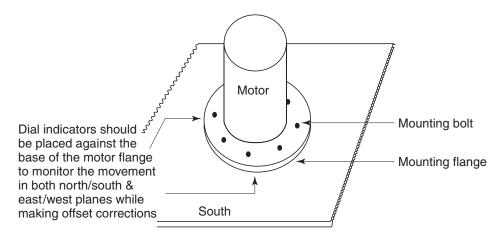
Figure 54.27 Placement of dial indicators to monitor offset corrections
