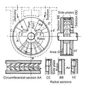
Figure 32.59 Peripheral pump layout and operating principle (after Addison<sup>1</sup>)
