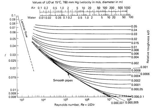
Figure 32.30 Friction factor f plotted against Re (after Miller<sup>6</sup>)
