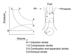
Figure 15.1 Four-stroke cycle for an internal combustion engine
