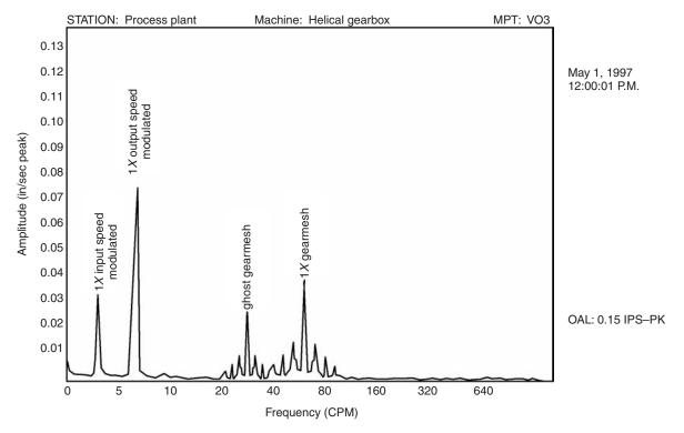
Figure 44.40 Sum modulation for a speed-increaser gearbox
