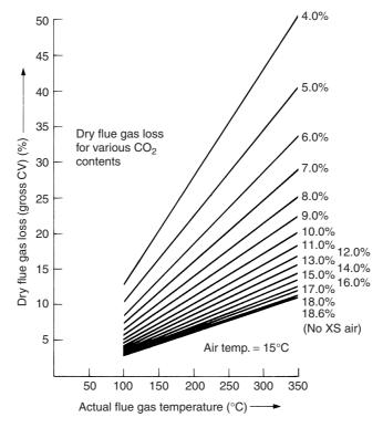
Figure 30.6 Flue gas losses - coal (Glasshoughton washed singles)
