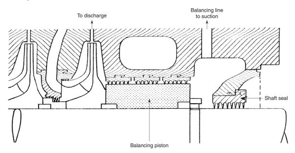
Figure 36.3 Balancing piston resists axial thrust from the in-line impeller design of a centerline centrifugal compressor
