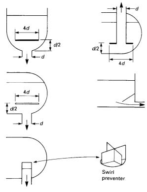
Figure 32.49 Vortex-prevention devices for tanks
