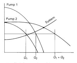
Figure 32.47 Dissimilar pumps in parallel
