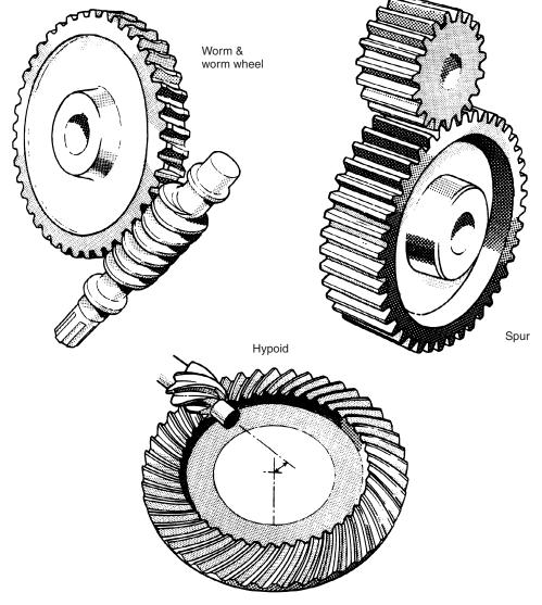
Figure 52.6 Gear types
