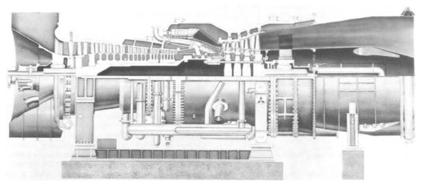
Figure 15.32 The Mitsubishi MW 701 gas turbine rated at 131 MW (ISO)
