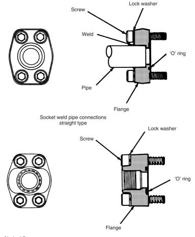
Figure 40.35 Four types of bolted flange connectors
