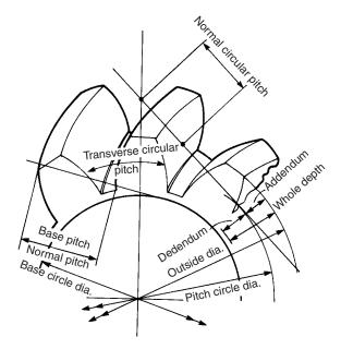
Figure 57.8 Helical gear and its parts
