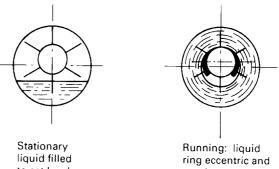
to set level. Rotor eccentric causing pumping action on air
