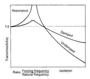
Figure 42.9 Performance of anti-vibration mounting
