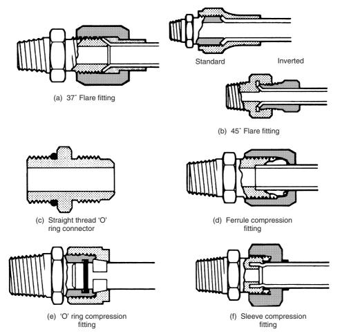
Figure 40.36 Flared tube fitting
