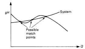
Figure 32.40 Combination of a flat system curve and an inflected pump curve
