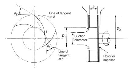
Figure 32.2 A simple centrifugal pump
