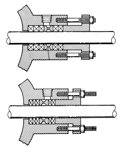
Figure 56.12 Proper lantern ring installation
