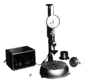
Figure 52.2 Grease penetrometer
