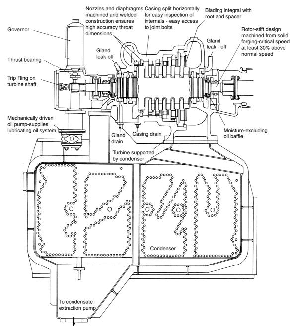
Figure 15.39 Longitudinal section of a small condensing turbine
