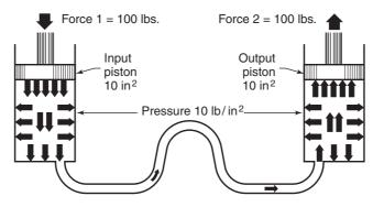
Figure 40.11 Transmitting force through small pipe
