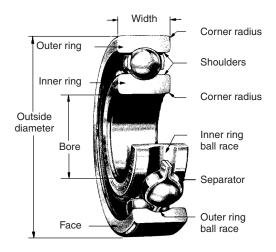
Figure 60.10 Conrad anti-friction ball bearing parts
