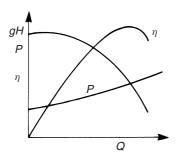
Figure 32.12 A pump's characteristic at fixed speed
