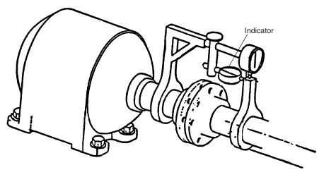
Figure 56.7 Dial indicator check for run-out
