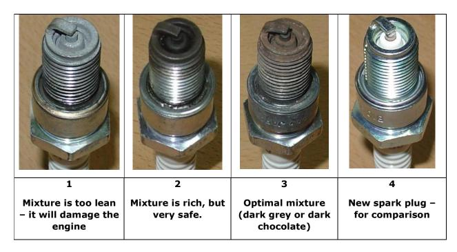
During the run-in time, a black or dark spark plug is a good sign because it means that the mixture is rich. During the run-in time, we advise you to err on the side of caution and use a rich mixture at the expense of slightly weaker engine performance.
