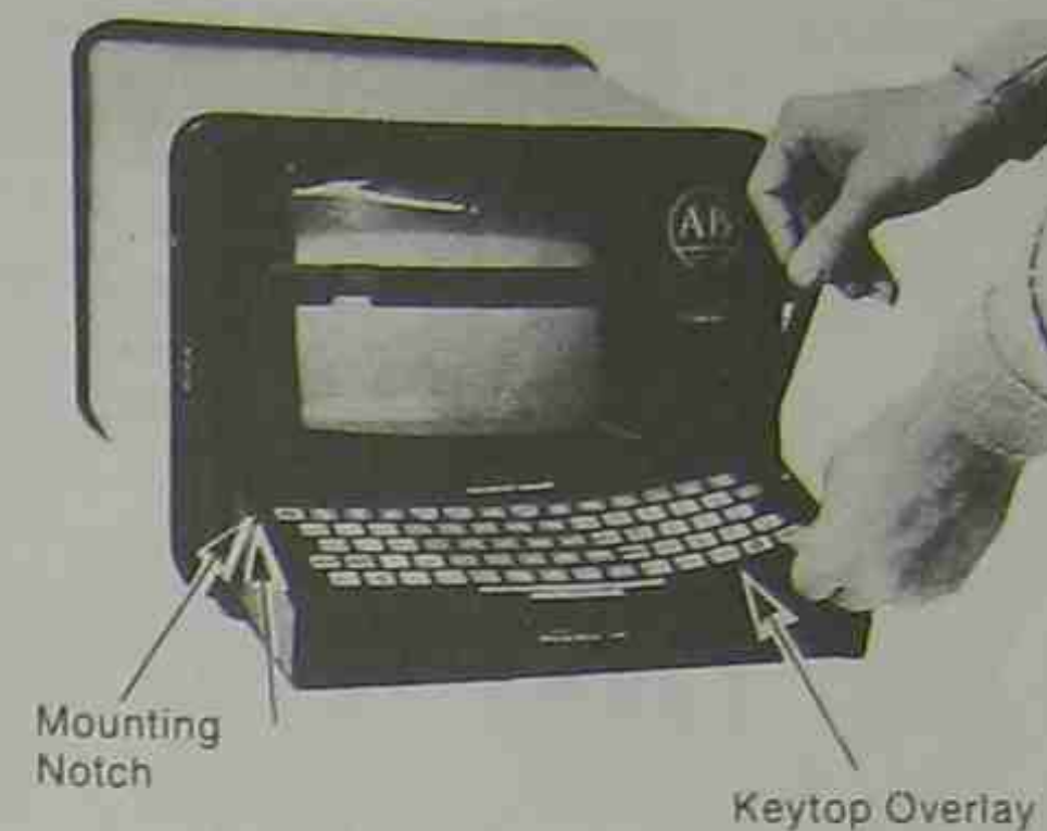
Figure 9-1c Installing an Overlay on the Keyboard (Courtesy of Allen-Bradley)
