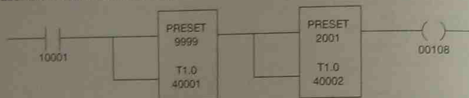
Figure 12-27b Cascading Timers in Series
