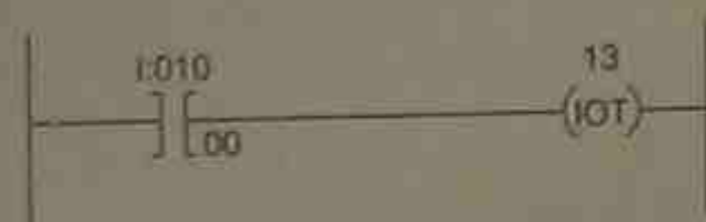
Figure 11-10 Programming the Immediate Output Instruction
