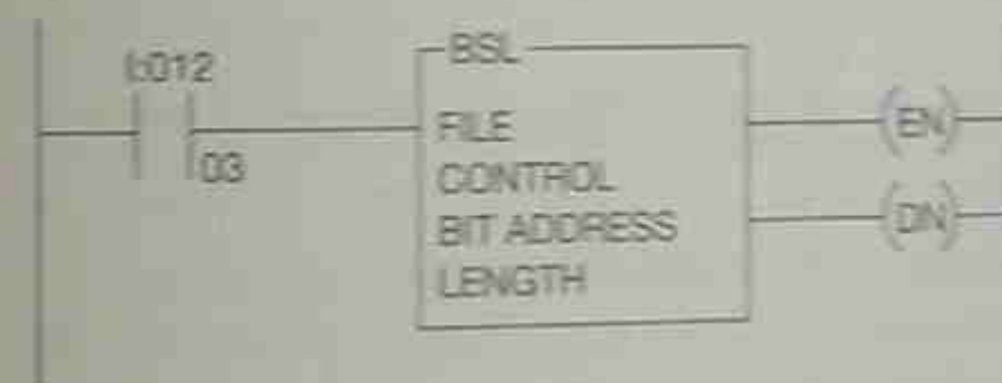
Figure 16-4 Bit Shift Left (BSL) Instruction
