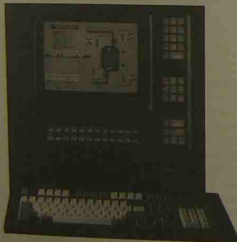
Figure 3-11 Allen-Bradley T-60 Industrial Terminal with 3 1/2" Floppy Disk and Hard Drive (Courtesy of Allen-Bradley)
