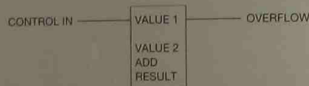
Figure 15-16 Format for Gould 984 Add Block Function
