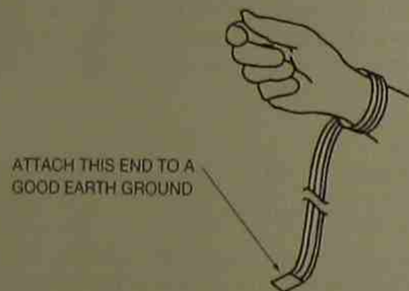
Figure 3-8 Wrist Strap Grounding Device (Courtesy of GE-Fanuc Automation)
