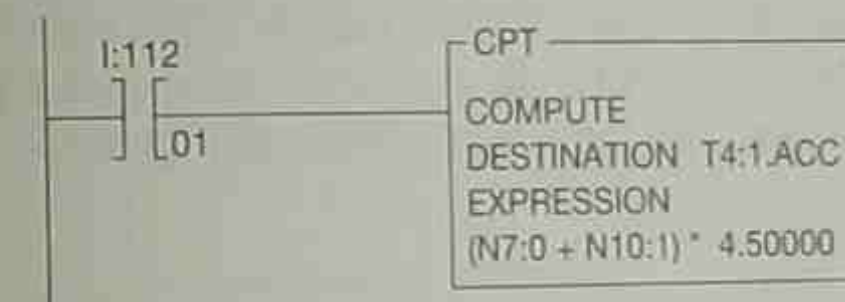
Figure 15-10 Programmed PLC-5 Compute (CPT) Instruction
