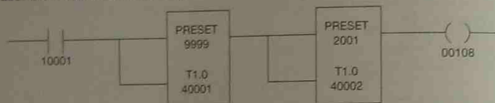
Figure 12-27b Cascading Timers in Series
