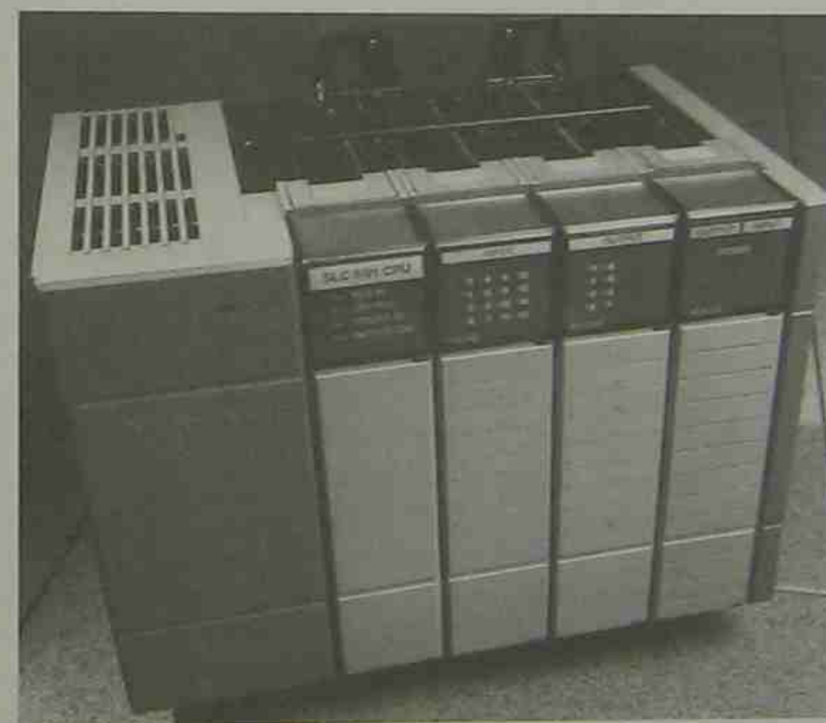
Figure 3-2 Allen-Bradley SLC 500 with a SLC 5/01 Processor (CPU) Installed (Courtesy of Allen-Bradley)
