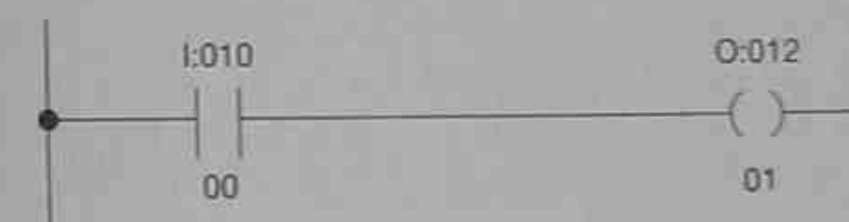
Figure 8-3 Equivalent Circuit Programmed with a PLC
