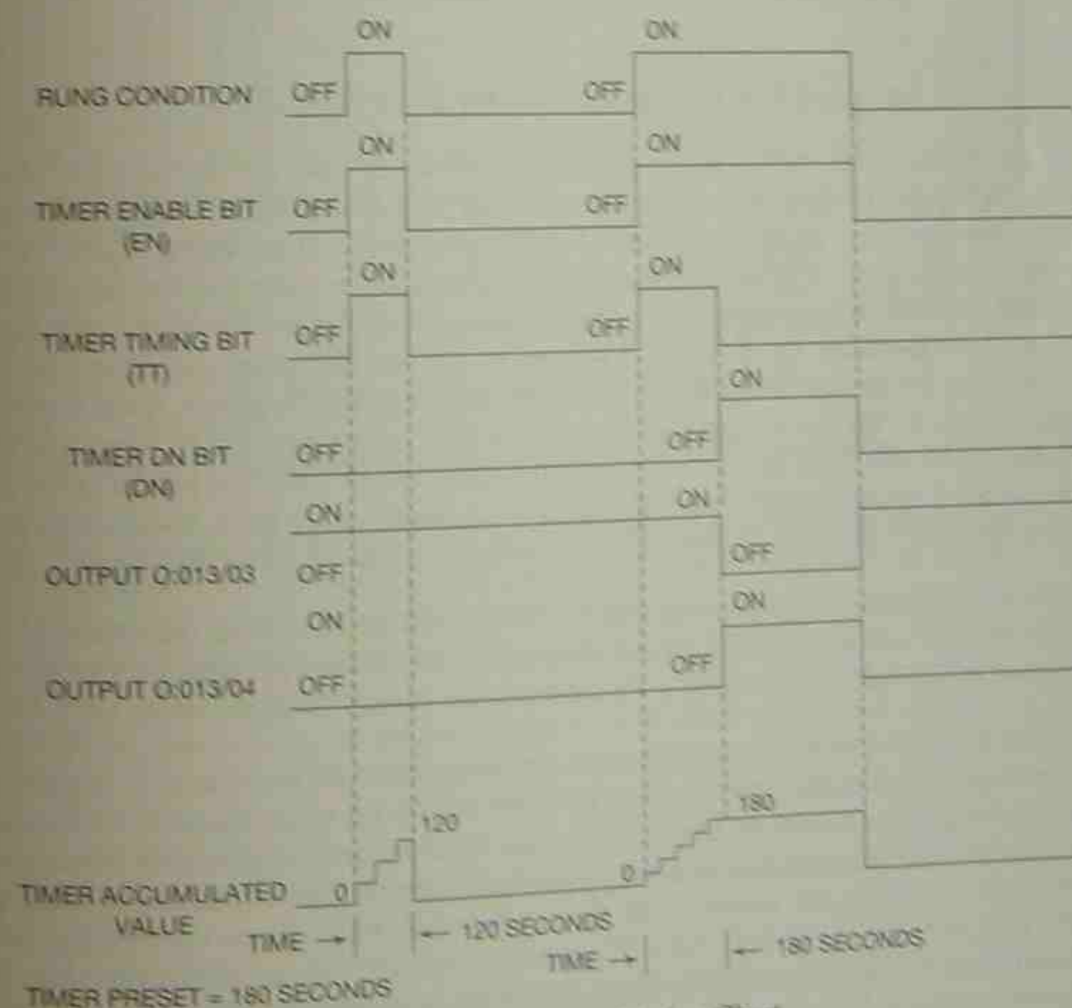
Figure 12-19 TON Timing Chart
