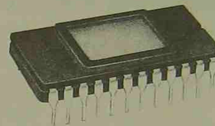
Figure 3-6 Typical UVPROM or EPROM Memory Chip (Courtesy of Allen-Bradley)
