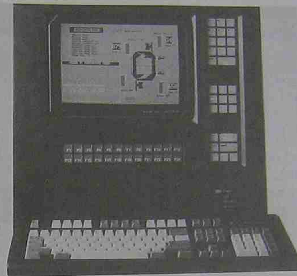
Figure 1-8 Programming Terminal (Courtesy of Allen-Bradley)
