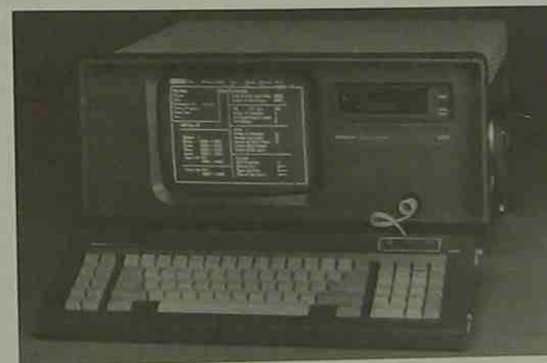
Figure 4-9 Modicon Inc. P230 Industrial Programming Panel (Courtesy of Modicon Inc.)
