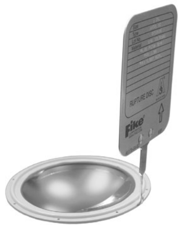
FIGURE 8.26 A reverse-acting rupture disk has a convex bulge facing into the fluid to be relieved. Fike Corporation.
