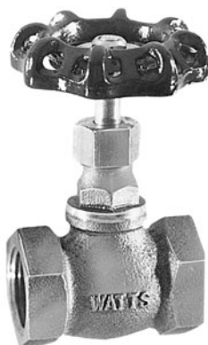
FIGURE 8.4 A threaded bronze globe valve with non-rising stem and threaded bonnet. Photo provided by Watts Regulator Company.
