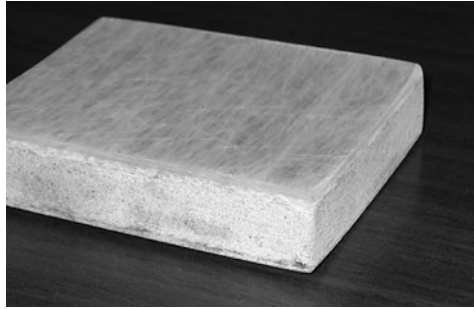
FIGURE 6.16 CCFRPM sample. Note the layering, with a smooth resin on the inside, a heavily reinforced chopped glass and mortar layer, a core of polymer mortar, followed by another heavily reinforced layer of chopped glass and resin, and finally, an exterior layer of sand and resin.
