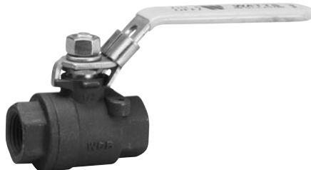
FIGURE 8.10 A two-piece threaded carbon steel ball valve with lockable handle. Photo provided by Watts Regulator Company.
