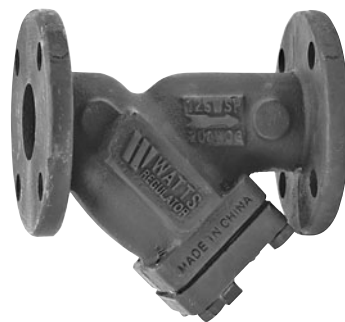
FIGURE 8.38 A Y-type strainer. The flange at the bottom is removed to remove the strainer screen. Photo provided by Watts Regulator Company.
