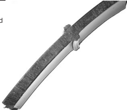
FIGURE 6.9 HDPE fusion welded joint. Note the weld bead on both the inside and outside surfaces.
