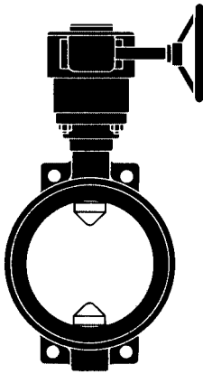
FIGURE 5.181 Butterfly valve.
