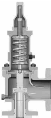
FIGURE 5.191 Conventional safety relief valve.
