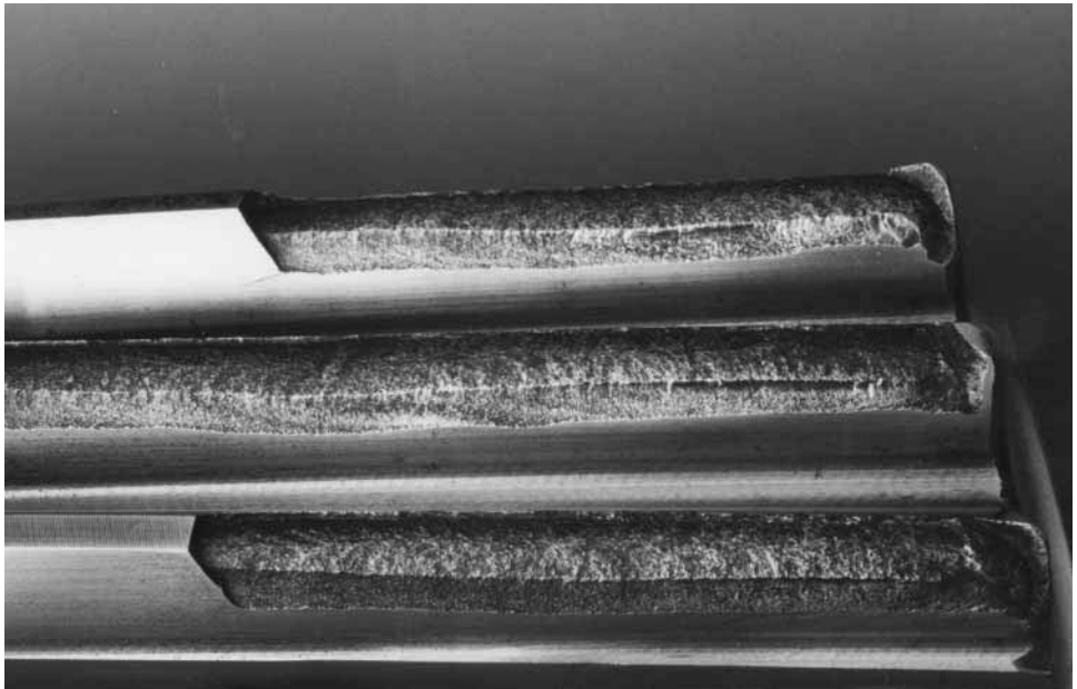
FIGURE 5.36 Case-core separation breakage. (AGMA; extracted from Ref. 13.)
