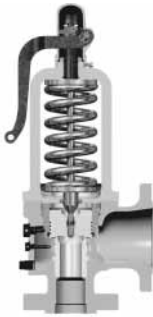
FIGURE 5.187 Pressure-relief device.
