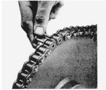
FIGURE 5.100 Inserting connecting link.
