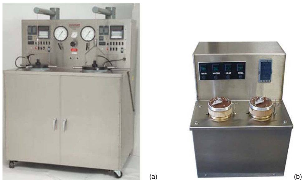
Fig. 4.3—Examples of (a) pressurized and (b) atmospheric consistometers. Courtesy of Halliburton.
