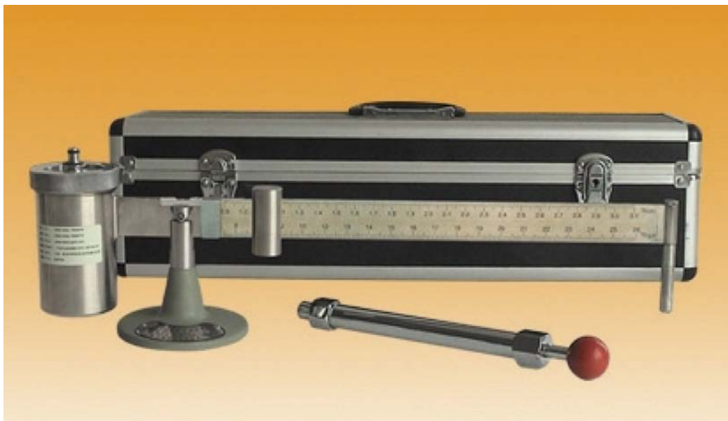
Fig. 3.14—Pressurized mud balance. Courtesy of Halliburton.
