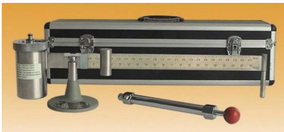
Fig. 4.2—Mud balance. Courtesy of Halliburton.
