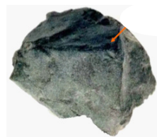
Angular cavings, shear failure due to excessive horizontal stress
