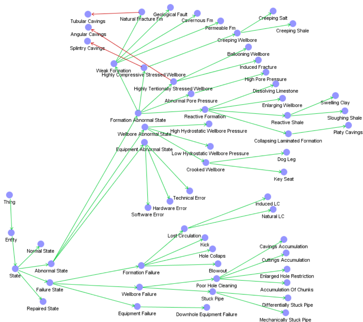
Figure 8-6: Error state with respect to location of where they emerge. If these errors are detected at the surface we call them indicative symptoms of failures.
