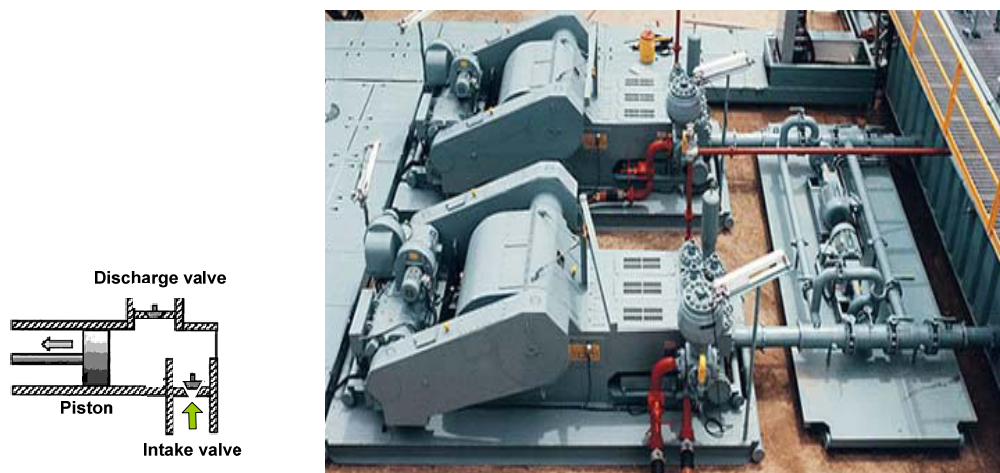
Figure 2-3: Two blue painted triplex (triplex means three pistons working in parallel), single acting piston pumps (single acting means acting only during on one of the two stroke directions). A single acting piston is shown to the left.
