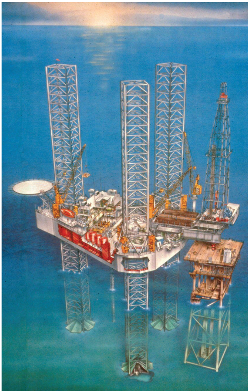
Fig. 14.8—Le Tourneau’s 116C cantilevered jackup with drill floor cantilevered over a fixed platform. Today’s workhorse design of jackups. Courtesy Le Tourneau, Inc.
