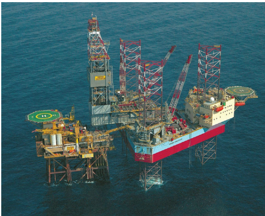
Fig. 14.18—Maersk's giant jackup (largest in the world) designed for deepwater use (550 ft in the GOM) and harsh North Sea environment. Courtesy Marine Structure Consultants.
