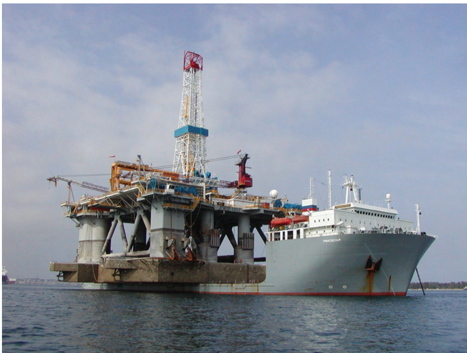
Fig. 14.22—Heavy lift ship performing a dry-tow transport of a semi ( Atwood Eagle ) from Angola to Australia in 2004. Courtesy Atwood Oceanics.
