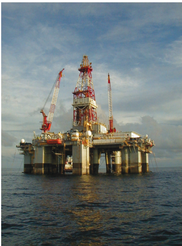
Fig. 14.14— Ocean Baroness , one of the Ocean Victory class (Fig. 14.12) second-generation semis upgraded to a fifth-generation unit. Note blister additions to column, deck expansion, and much larger derrick. This semi also did surface BOP work in Malaysia in 2003, along with setting the world's record self contained spread-mooring water depth (6,152 ft). Courtesy Diamond Offshore Drilling Inc.
