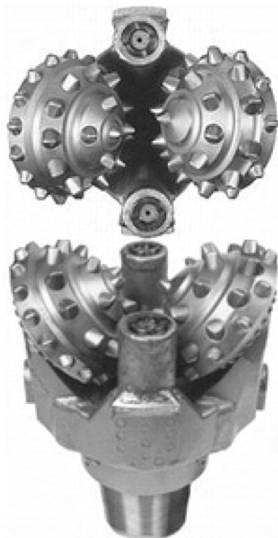
Fig. 5.17—Two-cone bit.
