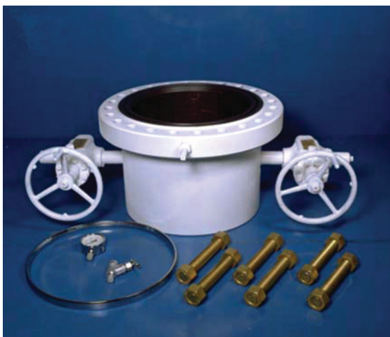
Fig. 8.2—Photo of a starting casing head and installation components. This casing head is typical of a thread-on or weld-on configuration used in land drilling operations.
