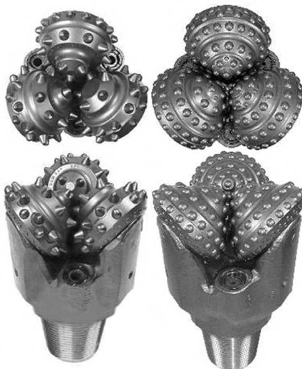
Fig. 5.5—Comparison of softer IADC 427Y (left) and harder 837Y (right) cutting structures.
