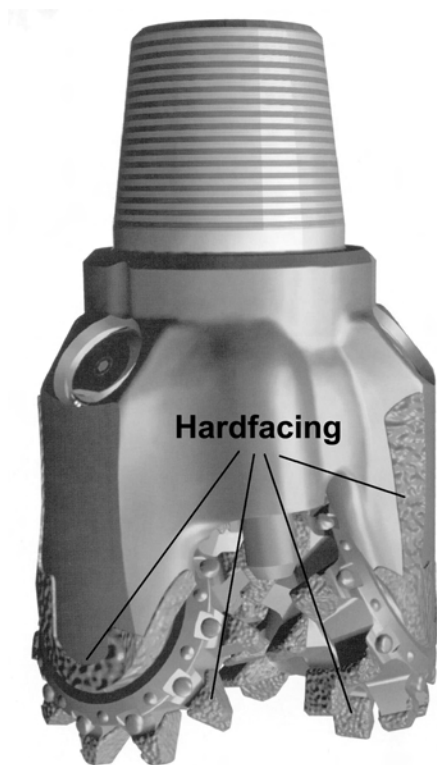
Fig. 5.8—Typical hard-facing applications on a milled-tooth bit.
