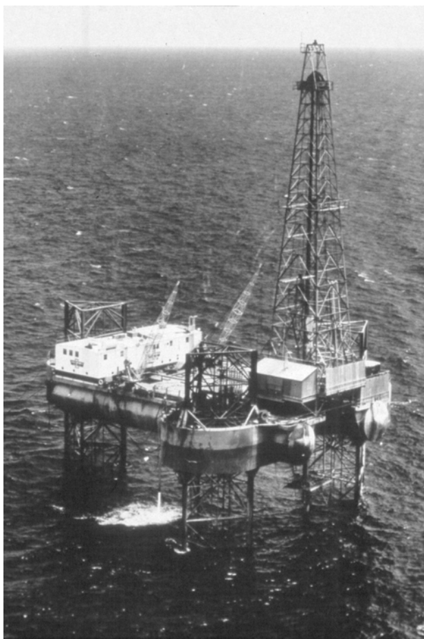
Fig. 14.7—Le Tourneau's Scorpion built for Zapata (now Diamond Offshore Drilling Inc.) in 1956 for 80-ft water depth as an independent-leg jackup. Lost in 1969.
