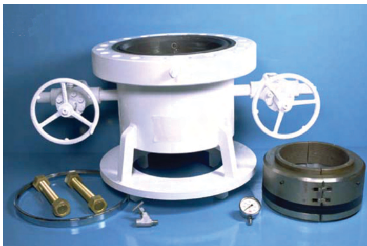
Fig. 8.3—Photo of a starting casing head and slip-and-seal assembly with installation components. This casing head has a gusseted base plate typically seen in jackup drilling operations.
