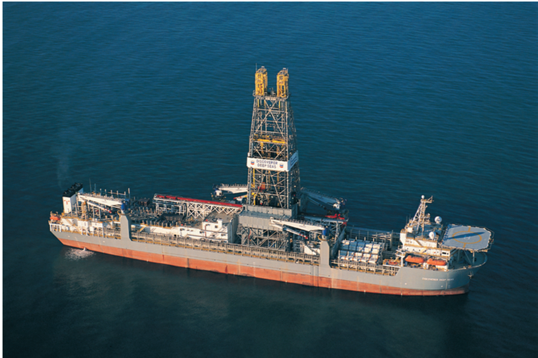
Fig. 14.21—Ultradeepwater drillship Transocean Discover class Discover Deep Seas that currently holds the world water depth record for drilling (10,011 ft). There are three of these type of units, which are 835 ft long with a power rating of 52,000 hp and displacement of 92,800 tons. Note the dual crown block for dual activity. Courtesy Transocean.
