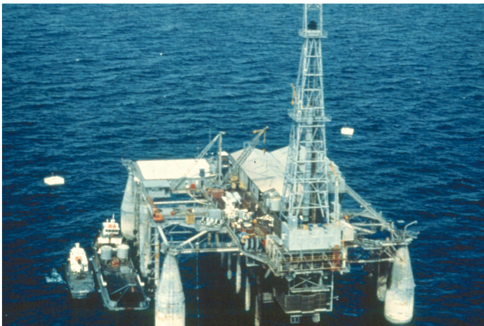
Fig. 14.10—World's first semi MODU, Bluewater No.1 , converted in 1961/1962 by Shell Oil from a submersible hull. Lost in 1964.
