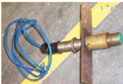
Fig. 15.2—Example of proximity and whisker switch.
