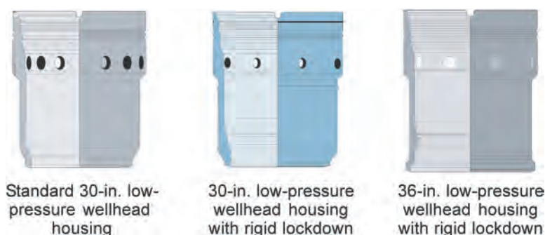
Fig. 8.23—Illustration of typical low-pressure wellhead housings. Each low-pressure housing can also incorporate various features based on the particular application and drilling environment.
