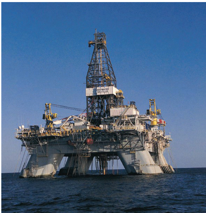
Fig. 14.13— Deepwater Nautilus , one of the newly built fifth-generation ultradeepwater semis that has DP assist for its spread-mooring system. Note spread columns for increased VDL and stability. Courtesy Transocean Inc.
