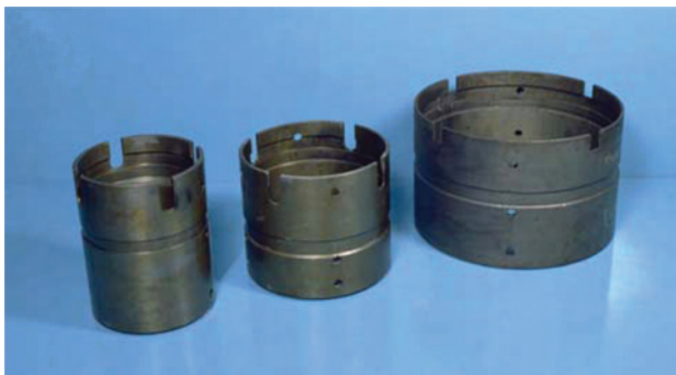
Fig. 8.9—Photos of the wear bushings for a typical land drilling wellhead system.
