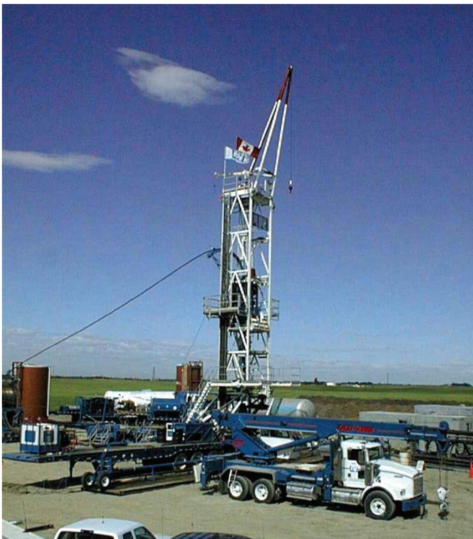
Fig. 16.24—Purpose built CTD rig working in Canada. These rigs are often built considering local area needs and regulations. This rig includes equipment for deploying BHAs into a pressurized wellbore (courtesy of BJ CT Services).
