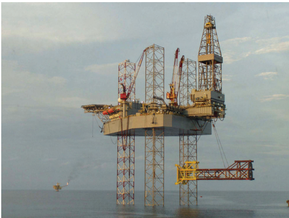
Fig. 14.20—Atwood Beacon enhanced premium jackup typical of the large and very capable vintage units of the 2000s. Note that the rig is setting a small fixed platform by jacking up to a 161-ft air gap, at which time the platform will be righted to vertical, and then the rig will jack down and set the platform on the sea bottom. Courtesy Atwood Oceanics.
