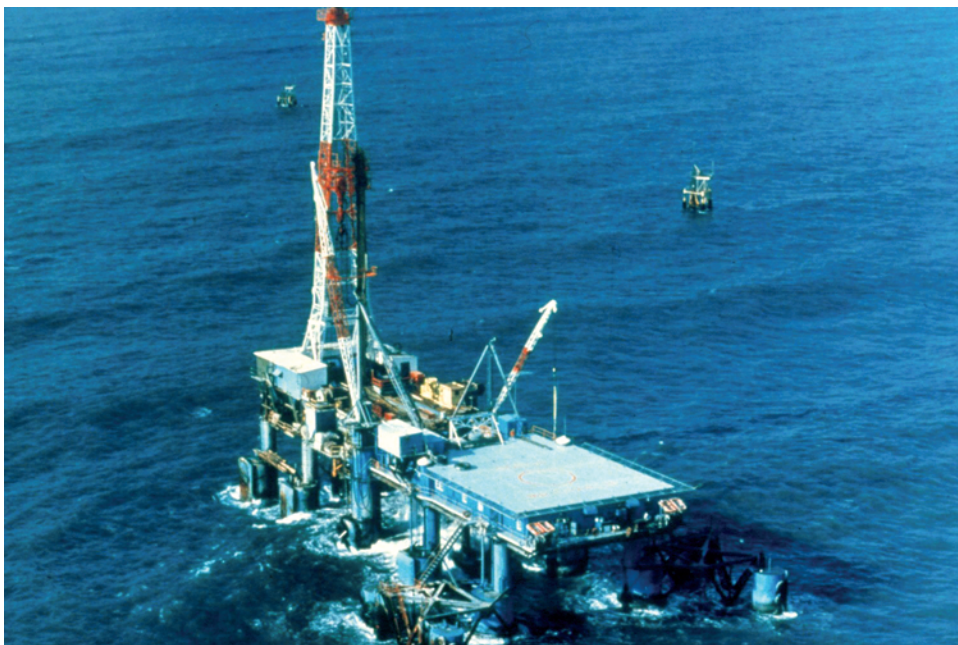
Fig. 14.2—Mr. Charlie, the first purpose-built (June 1954) open-water MODU rated for 40-ft water depth. Retired in late 1986 and now a museum and training rig in Morgan City, Louisiana.
