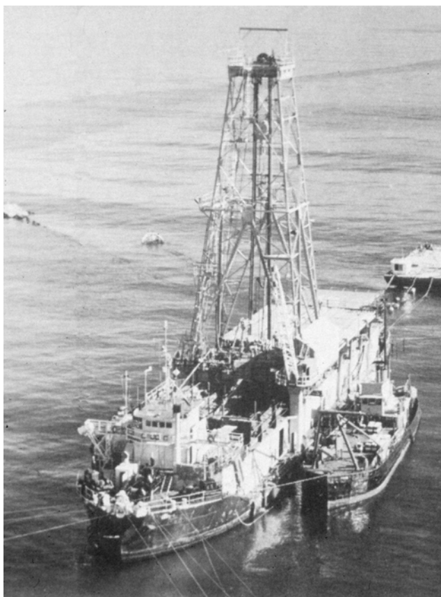
Fig. 14.3— Western Explorer , the first (1955) floating oil- and gas-drilling MODU that used subsea well control. Retired in 1972.
