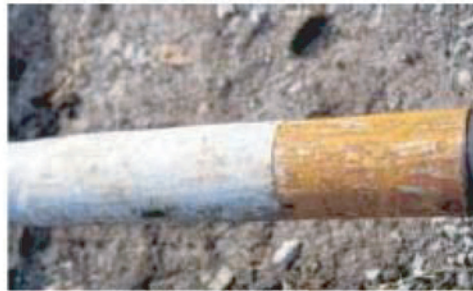
Condition of joint end after use—a little rust on the steel end, but the composite has only a few scratches.
