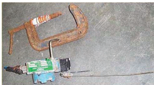
Fig. 15.2—Example of proximity and whisker switch.
