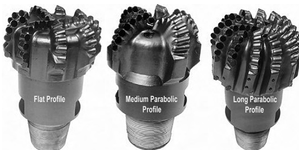
Fig. 5.27—PDC bit profile types.
