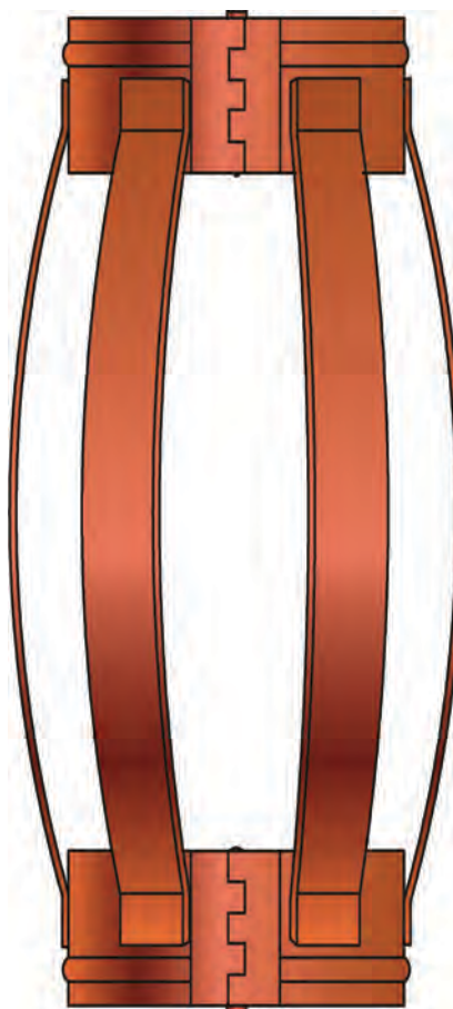
Fig. 9.13—Welded bow-spring centralizer (courtesy of Halliburton).
