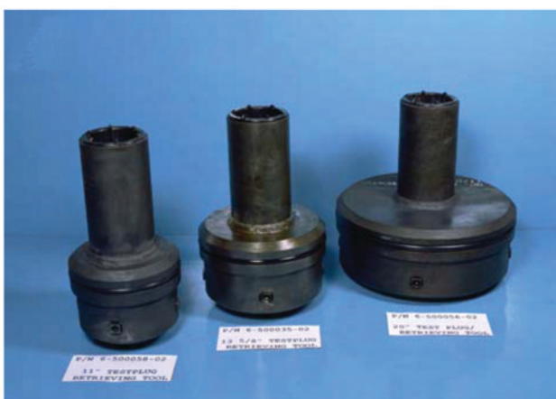
Fig. 8.10—Photo of the wear bushing running tools. These tools are also used to test the BOP stack.
