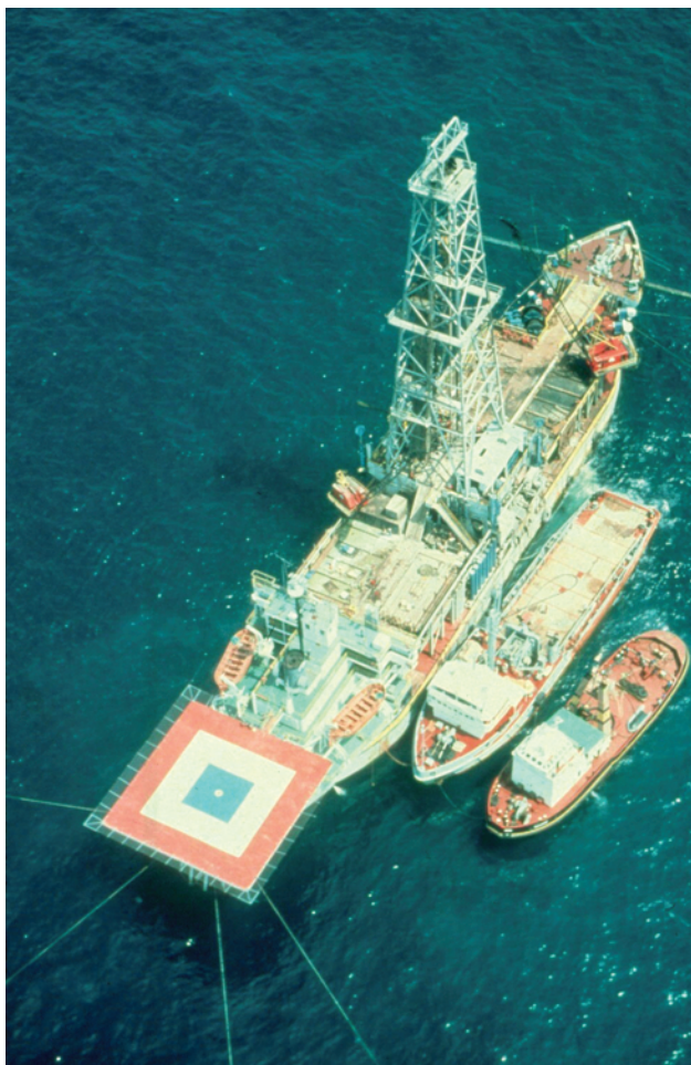
Fig. 14.16—Typical spread-moored drillship of the 1970s. Note workboat next to rig with small ocean-going tug next to it.
