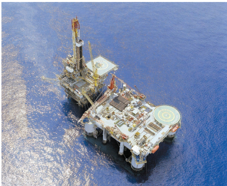
Fig. 14.9—World’s first purpose-built (conversion) semi TAD unit Seahawk . Converted in 1992 from a semi MODU. Courtesy Atwood Oceanics.
