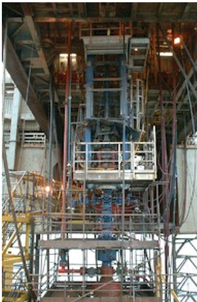
Fig. 12.24—Rig-assist snubbing system.
