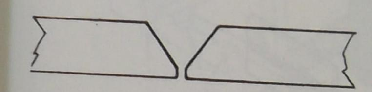
This weld is a single V butt joint commonly used on materials between 5 to 12mm thick. Whether or not the section has to be bevelled for full fusion depends on the thickness of the material. This type is the strongest of all the welded joint designs.
