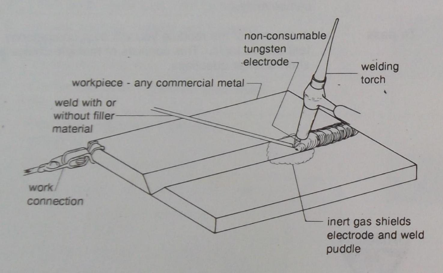
Gas tungsten arc is an electric arc process. The heat is produced by drawing an arc between a non-consumable tungsten electrode and the work (parent material). The weld zone, molten weld pool and electrode are shielded form atmospheric contamination. This inert gas shield is concentrated around the area of the arc by a ceramic gas nozzle. Filler material may or may not be used.
