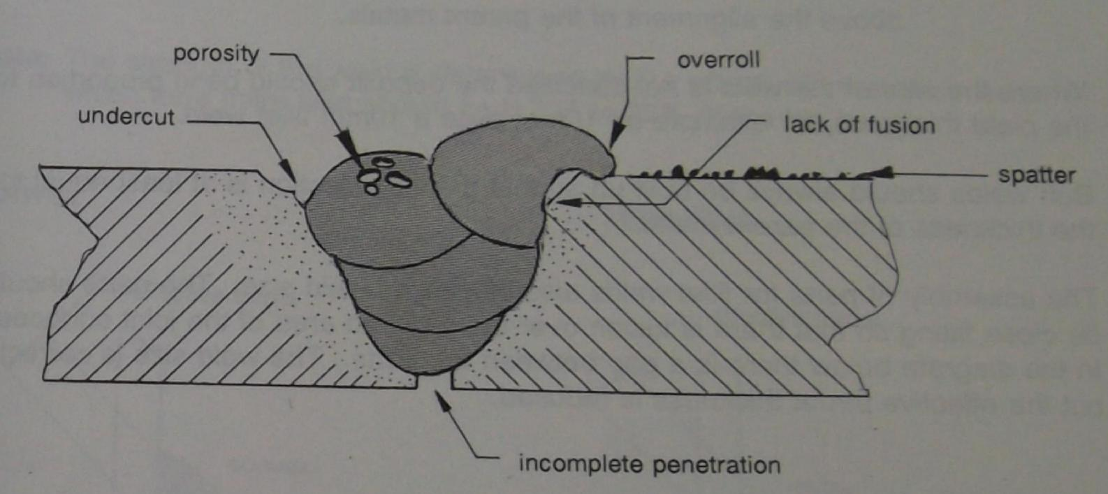
Overroll: a fault at the toe of a weld. Caused by molten weld overflowing onto a surface of unmelted parent metal which leaves an unfused area.
