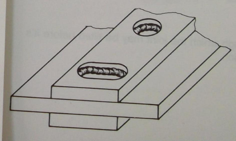
This special type of joint is used to fasten large flat plate sections together without buckling.
