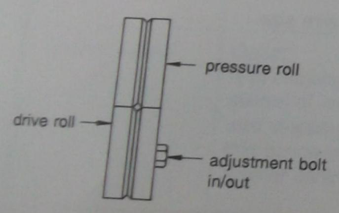
correct adjustment both rolls aligned with pressure roll at correct tension
