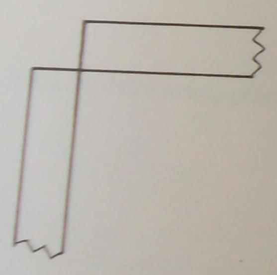
This type of weld joint is often used for hopper construction. The plate edges come together easily during fabrication and make a strong, watertight weld.
