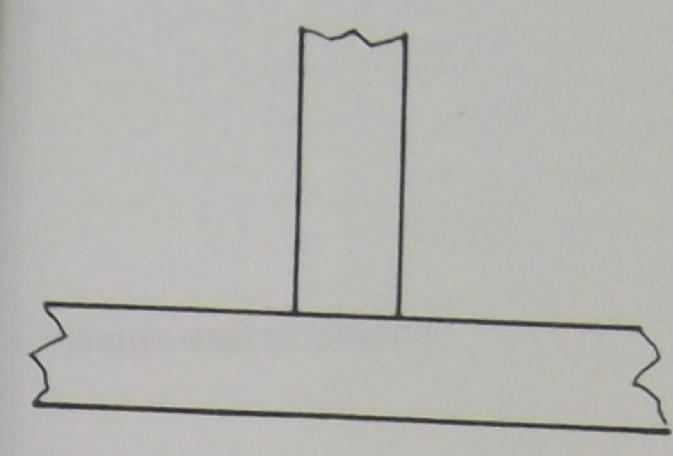
This is one of the most common welded joints used in the construction industry. It's easily fabricated and you can quickly deposit a weld that looks good.
