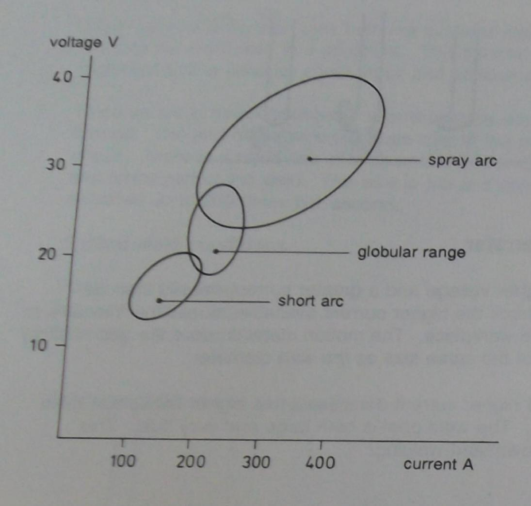
By carefully selecting wire speed and voltage, it's possible to set parameters to operate effectively within the three modes of transfer shown above. However, if welding parameters are set outside the three circles, your welding conditions will become erratic and uncontrollable.
