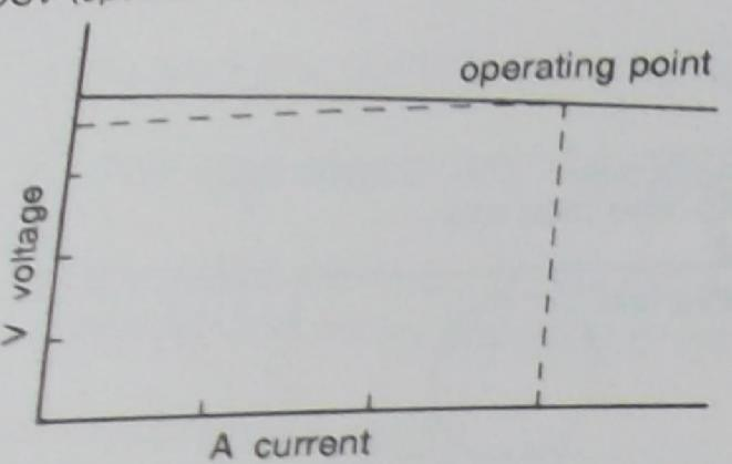
The constant potential power supply has an almost flat volt/ampere characteristic
