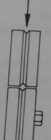
loose wire adjust pressure roll down
