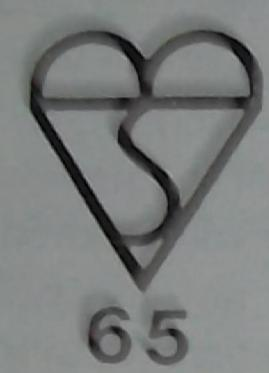
Figure 2: Example of BSI Kite Mark, as used on saltglazed stoneware drain pipes made to BS 65
