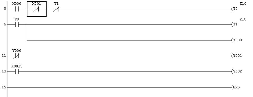
3. Select the horizontal line, i.e. key 6, to overwrite the X1 contact with a horizontal line (Figure 4.8).
