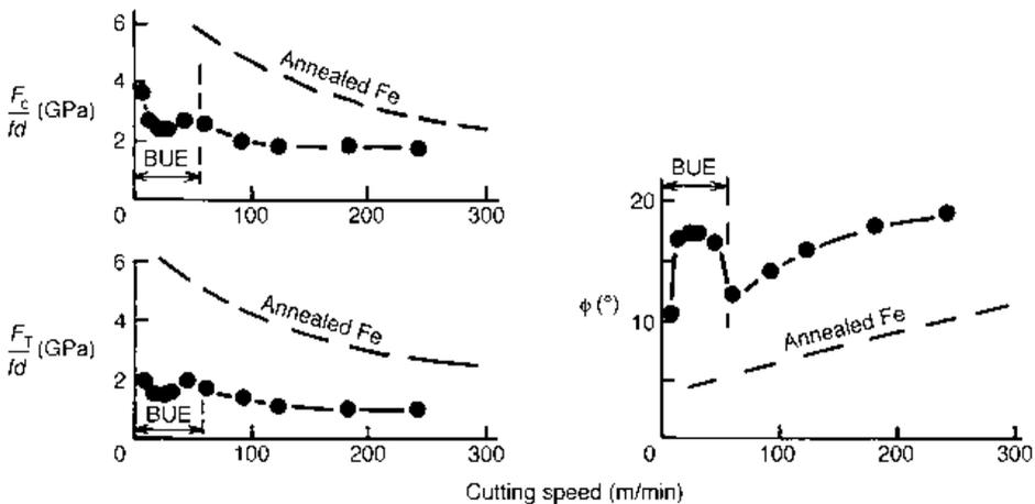
Fig. 3.14 Characteristics of built-up edge (BUE) formation (0.15C steel,  $f = 0.15$  mm,  $\alpha = 6^\circ$ )
