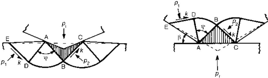
Fig. A3.3 Plastic indenting by, and flattening of, wedge-shaped asperities
