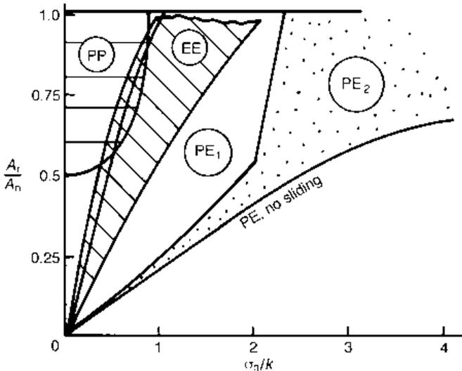
**Fig. 2.25** Ranges of possible degrees of contact: PP = plastic asperity on plastic chip; PE = plastic asperity on elastic chip; EE = elastic asperity on elastic chip
