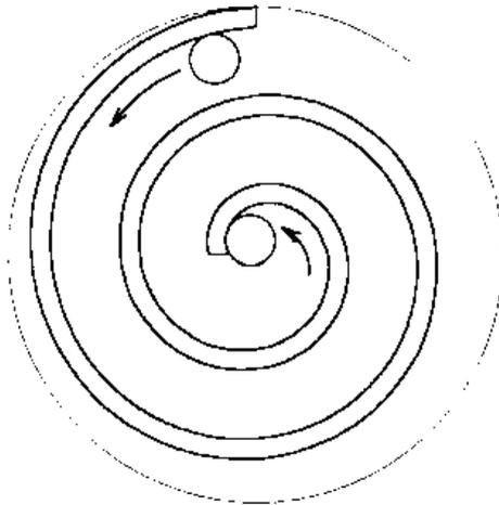
Fig. 9.5 Milling of scroll surfaces
