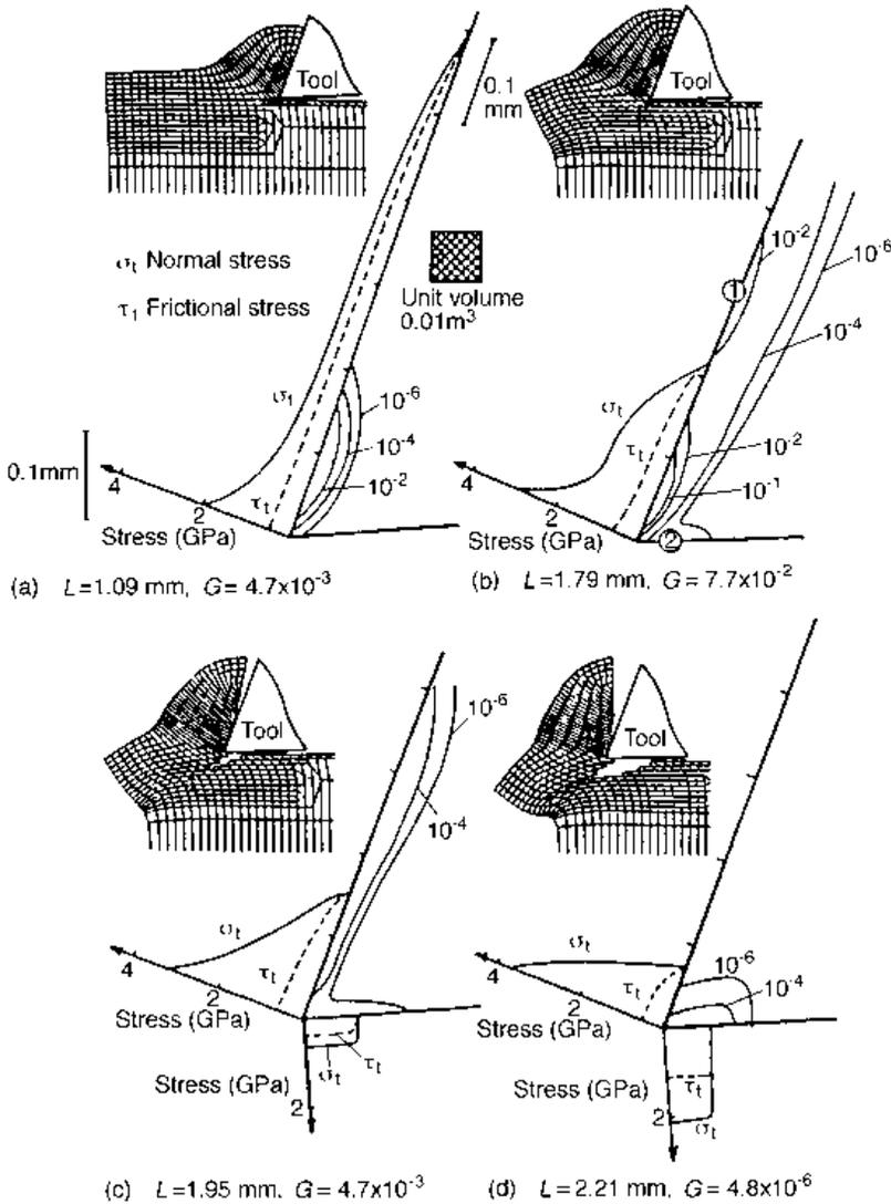
**Fig. 8.9** Changes of chip shape and tool edge fracture probability at exit, when machining a  $\beta$ -brass with an alumina ceramic tool at a cutting speed of 13 mm/min,  $f=0.25$  mm,  $d=3$  mm,  $\alpha=20^\circ$ , clearance angle  $\gamma=5^\circ$ , exit angle  $=90^\circ$ , friction coefficient  $\mu=1.0$  and no coolant
