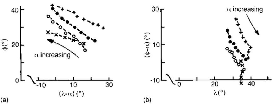
**Fig. 2.14**  $\phi$ - $\lambda$ - $\alpha$  relationships for normal production speed turning by high speed steel tools, with rake angles from 5° to 40°, of cold rolled (●) and annealed (○) free cutting steel, an aluminium alloy (+) and an  $\alpha$ -brass (×): (a)  $\phi$  versus  $(\lambda - \alpha)$  and (b)  $(\phi - \alpha)$  versus  $\lambda$  (data from Eggleston *et al.*, 1959)
