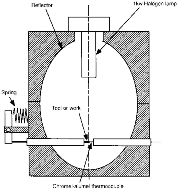
**Fig. 5.16** A tool–work thermocouple calibration set-up
