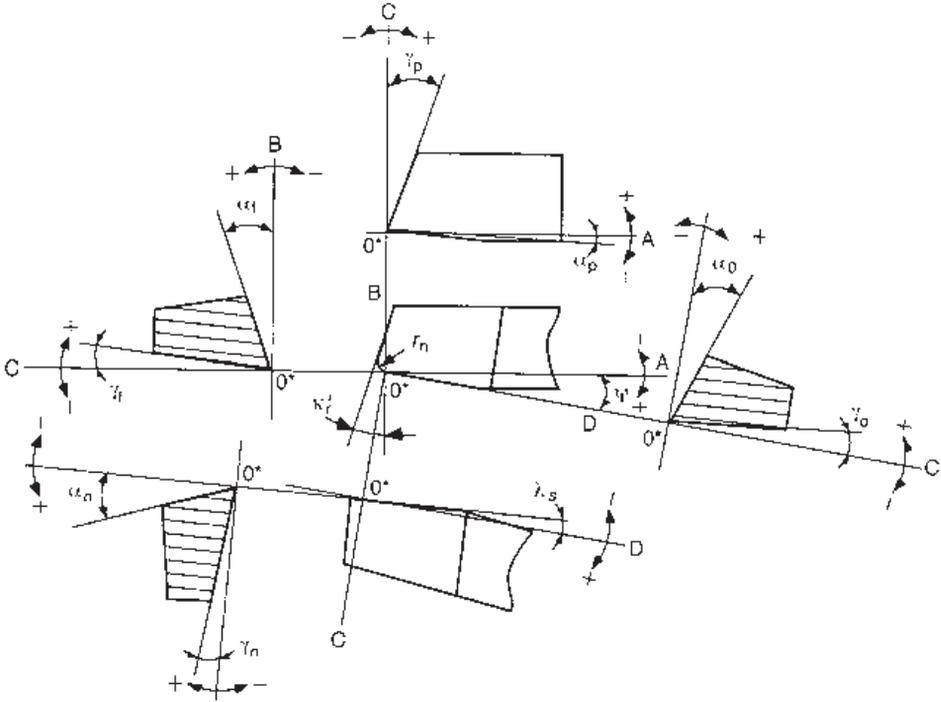
Fig. 6.16 Single point cutting tool geometry
