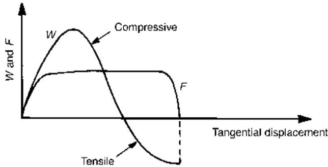
Fig. A3.10 Qualitative junction load history for zero normal displacement
