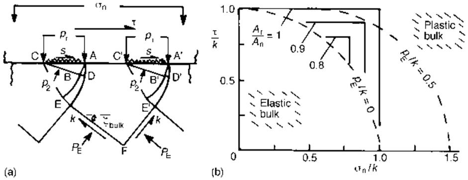
**Fig. A3.9** (a) Combined asperity and bulk plastic stressing and (b) derived degrees of contact  $A_r/A_n$ , depending on the apparent contact stresses and the bulk field hydrostatic stress level  $p_E/k$ , for  $s/k = 1$
