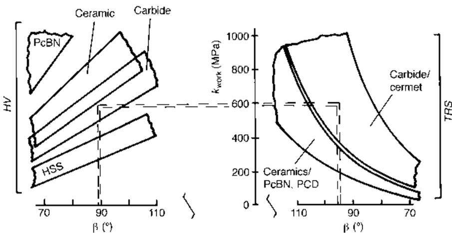
**Fig. 3.26** A way to estimate minimum tool wedge angles  $\beta$  to avoid failure of a given tool material (specified by  $HV$  and TRS), acted on by stresses characterized by  $k_{\text{work}}$ , developed from Figure 3.19
