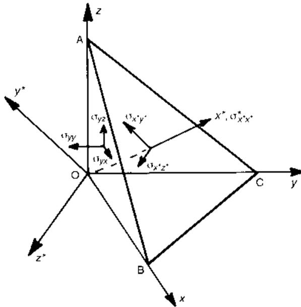
Fig. A1.9  $(x,y,z)$  and  $(x^*,y^*,z^*)$  co-ordinate systems
