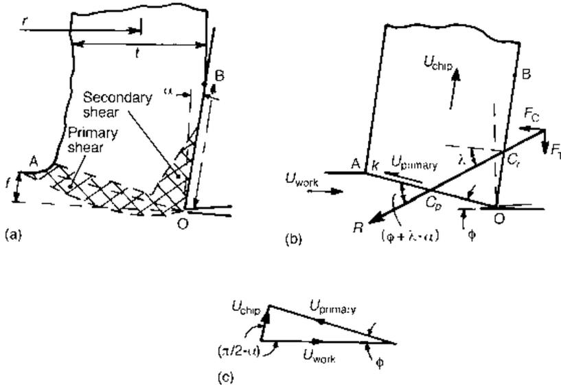
Fig. 2.5 Chip flow (a) sketched from Figure 2.4(a); (b) simplified and (c) its velocity diagram
