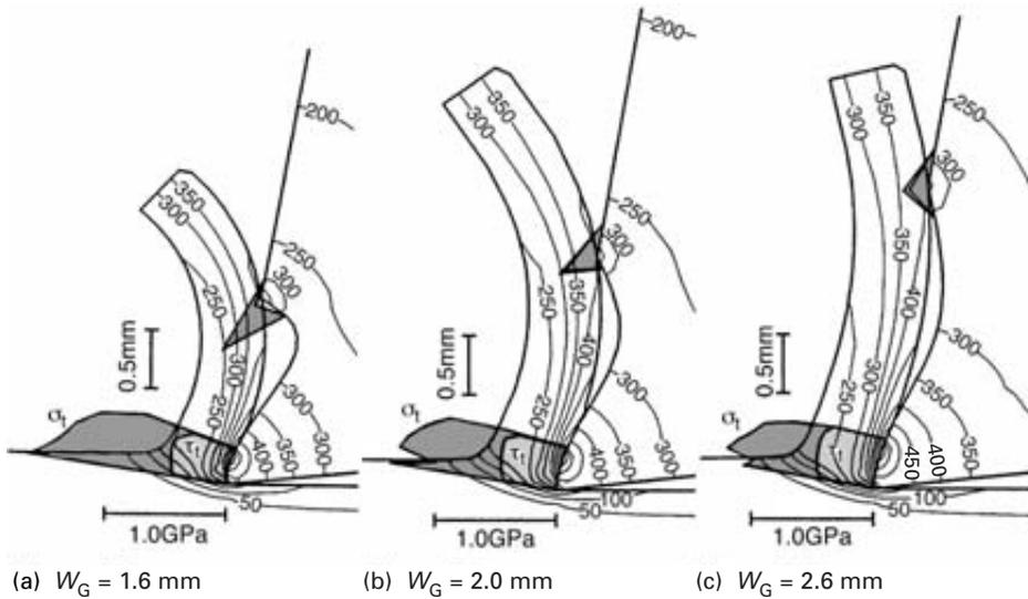
**Fig. 8.21** Predicted chip shape and distributions of temperature ( $^{\circ}\text{C}$ ) and stresses with changing  $w_G$  ( $h_B=0$ ) when machining 0.18% C steel with carbide P20 at  $V=100$  m/min, undeformed chip thickness  $t_1=0.25$  mm and without coolant
