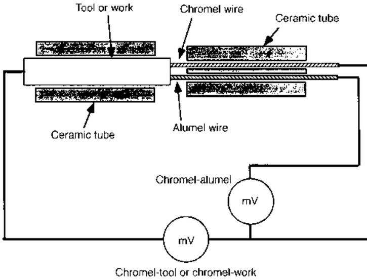
Fig. 5.17 A detail of the hot junction and the associated measurement circuit
