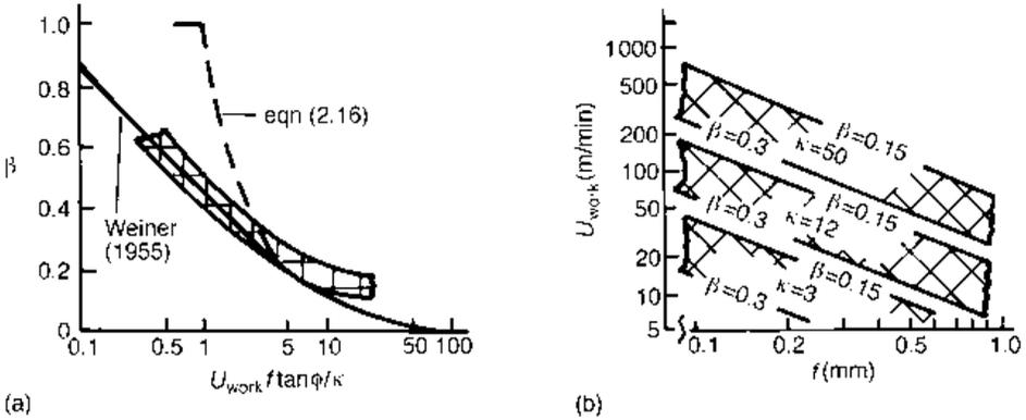
**Fig. 2.18** (a) Theoretical (—, ---) and observed (hatched region) dependence of  $\beta$  on  $[U_{work} f \tan \phi / \kappa]$ ; (b) iso- $\beta$  lines ( $\beta = 0.15$  and  $0.3$ ) mapped onto a  $(U_{work}, f)$  plane for  $\kappa = 3, 12$  and  $50 \text{ mm}^2/\text{s}$  and  $\phi = 25^\circ$
