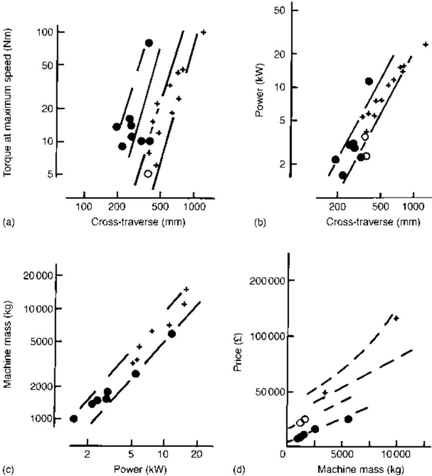
**Fig. 1.16** (a) Torque and (b) power as a function of cross-traverse capacity and (c) mass/power and (d) price/mass relations, from manufacturers' catalogues, for mechanical (•) and basic CNC (o) milling machines and centres (+)
