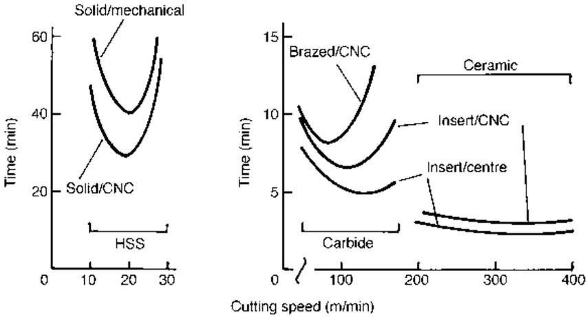
**Fig. 1.26** The influence on manufacturing time of cutting speed, tool material (high speed steel/carbide/ceramic) and manufacturing technology (solid/brazed/insert tooling in a mechanical/simple CNC/turning centre machine tool) for turning the part in Figure 1.25
