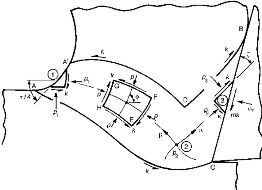
Fig. 6.1 A wrong guess of a chip plastic flow zone shape, to illustrate some rules of slip-line field theory
