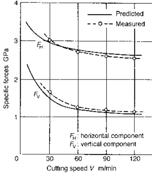
**Fig. 7.17** Comparison of predicted specific forces with experiment for the same feed and rake angle as Figure 7.14, but with varying cutting speed
