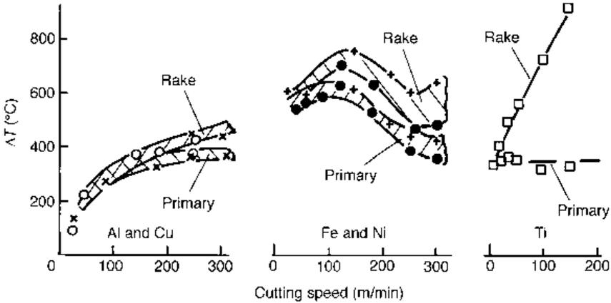
Fig. 3.5 Temperatures estimated from the observations of Figure 3.3
