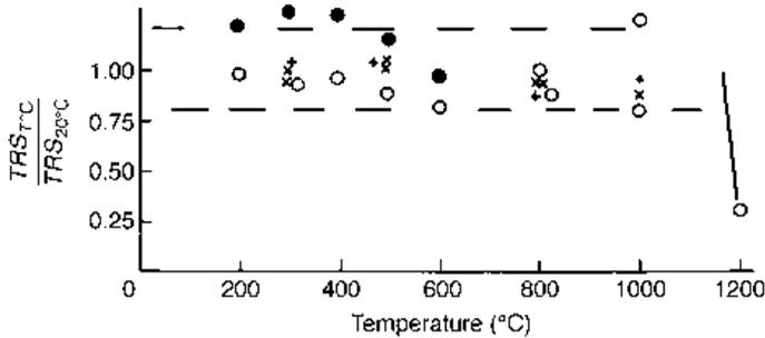
**Fig. 3.23** Representative values of TRS relative to TRS at 20°C for HSS(•), carbide/cermet (x), Al<sub>2</sub>O<sub>3</sub>(o) and Si<sub>3</sub>N<sub>4</sub>(+) based tool materials
