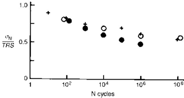
Fig. 3.25 Representative bending fatigue behaviour at room temperature of three tool materials: HSS(•),  $\text{Al}_2\text{O}_3$ (o) and  $\text{Si}_3\text{N}_4$ (+) based
