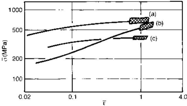
**Fig. 2.9** Equivalent stress-strain data for (a) a mild steel, (b) an aluminium alloy; and (c) an  $\alpha$ -brass obtained from compression testing (—) and values from metal cutting tests (hatched), after Kobayashi and Thomsen (1959)
