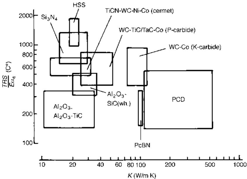
**Fig. 3.21** Tool materials' characterization by thermal conductivity and shock resistance
