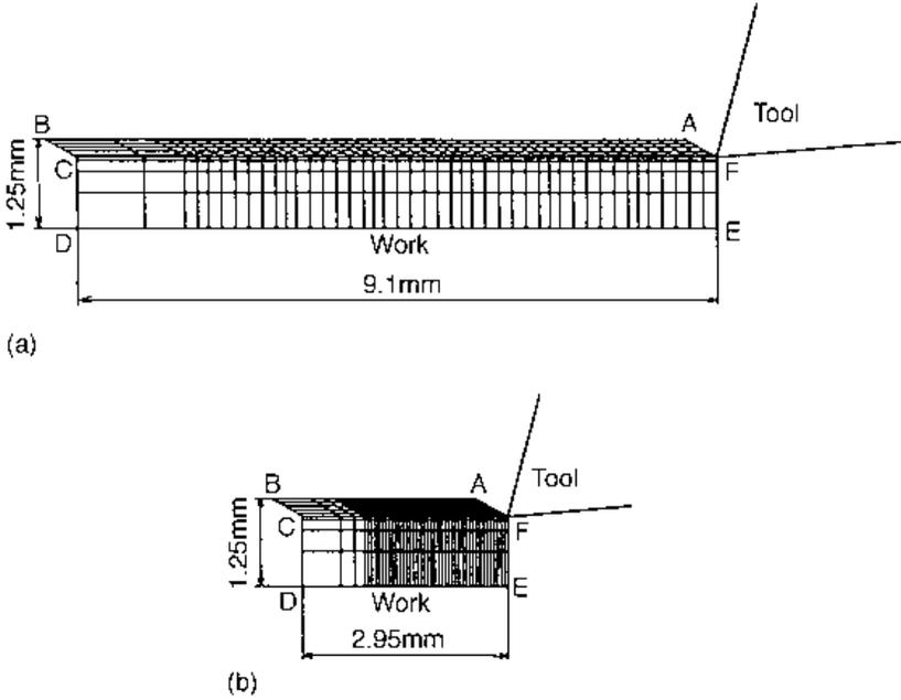
Fig. 7.18 (a) Coarse (b) fine finite element mesh
