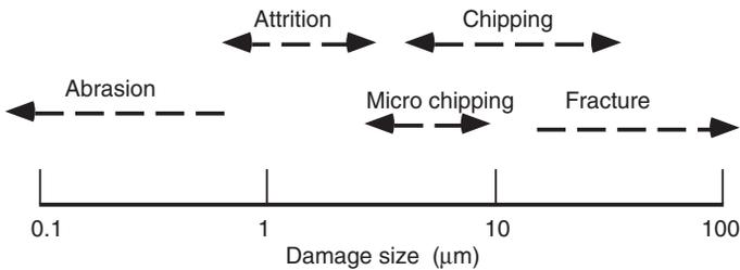
Fig. 4.4 Classification of mechanical damages
