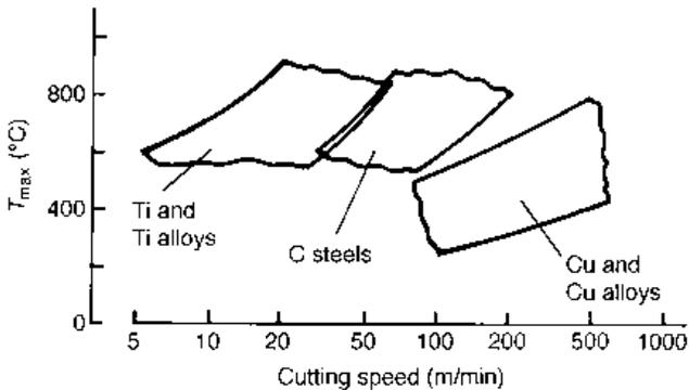
Fig. 1.23 Maximum tool face temperatures generated during turning some titanium, ferrous and copper alloys at a feed of 0.25 mm (after Trent, 1991)
