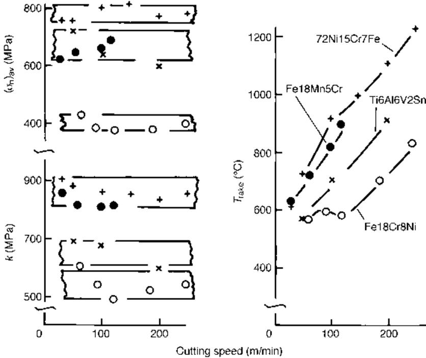
Fig. 3.11 Process stresses and temperatures derived from (and symbols as) Figure 3.10
