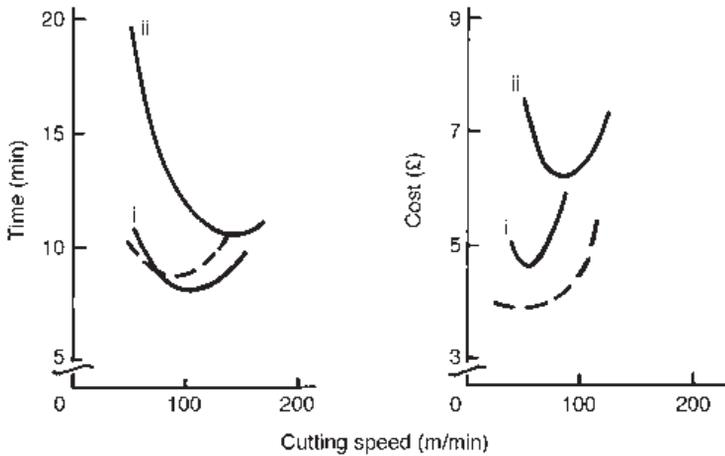
**Fig. 1.28** Times and costs to remove metal by milling, for the conditions i and ii of Table 1.7 compared with removing the same metal by turning (---)
