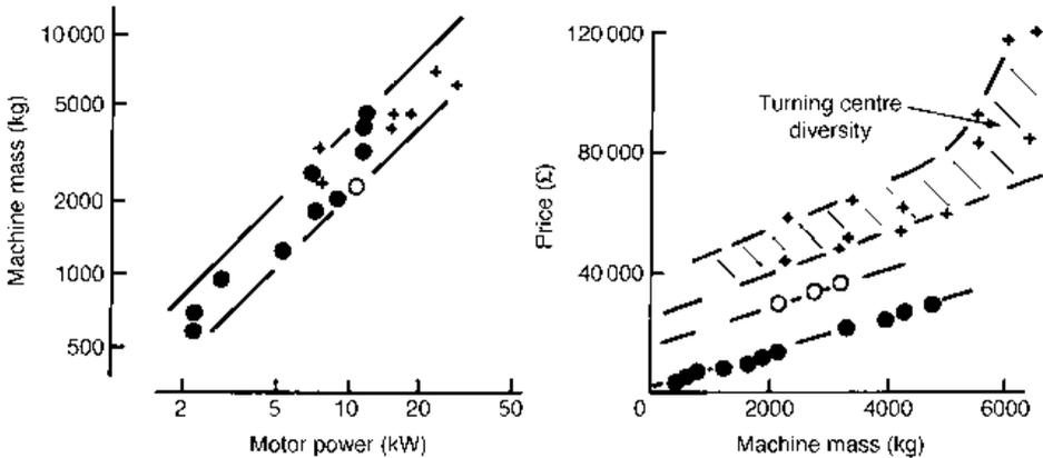
Fig. 1.10 Mass/power and price/mass relationships for turning machines
