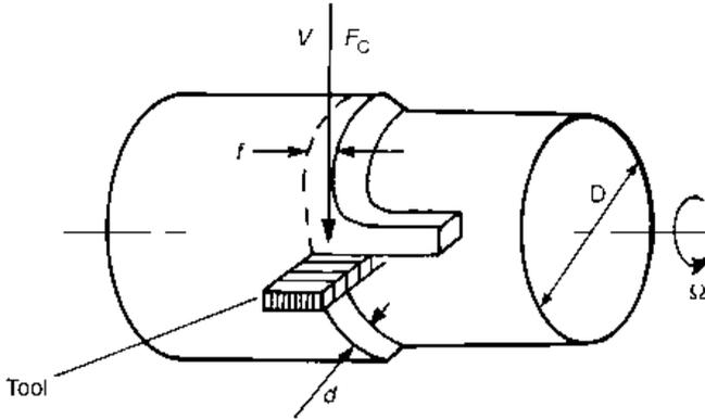
Fig. 1.7 The turning process – not to scale
