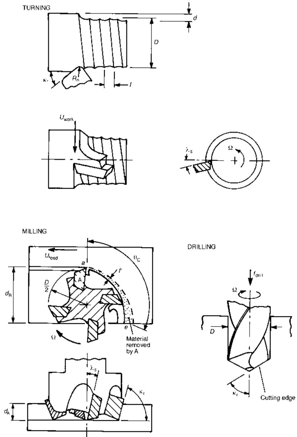
Fig. 2.3 Turning, milling and drilling processes
