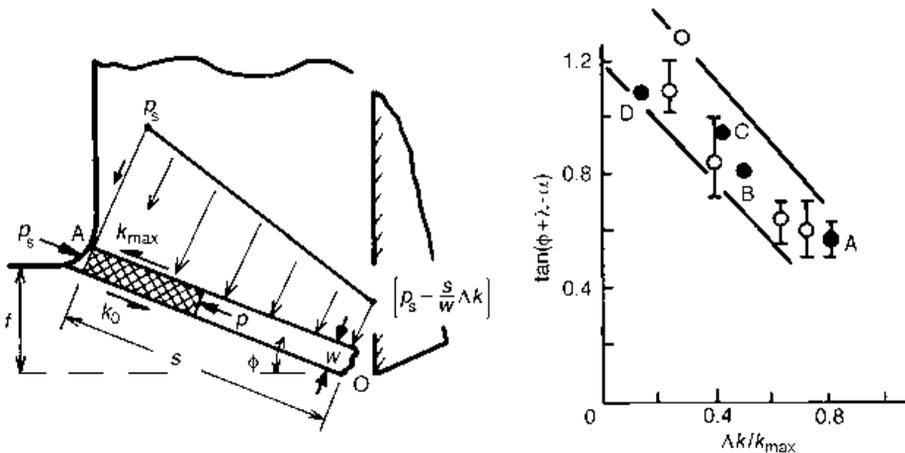
Fig. 2.11 (a) The primary shear region modelled as a parallel-sided zone of thickness  $w$ , showing pressure variations due to work hardening; and (b) observed reductions of  $\tan(\phi + \lambda - \alpha)$  with increasing work hardening
