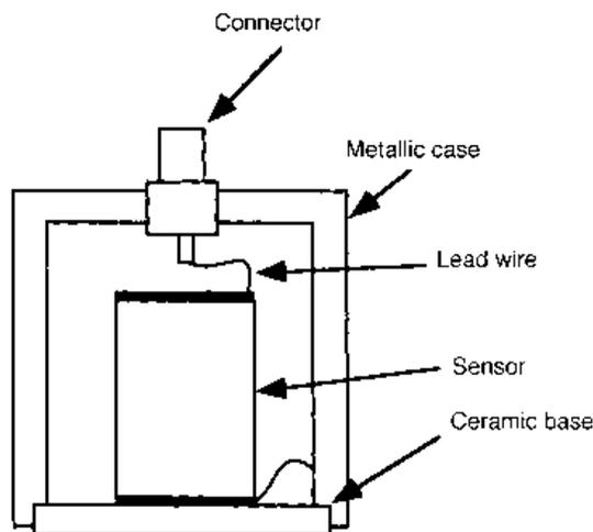
Fig. 5.22 Structure of an AE sensor
