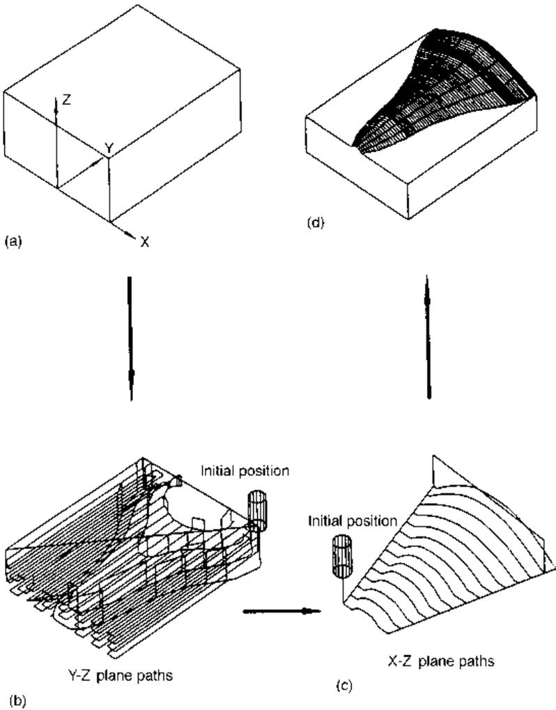
**Fig. 9.34** Tool path for machining an aerospace component (Tarng *et al.*, 1995): (a) original workpiece, (b) tool paths in the  $Y-Z$  planes; (c) tool paths in the  $X-Z$  planes; and (d) machined workpiece
