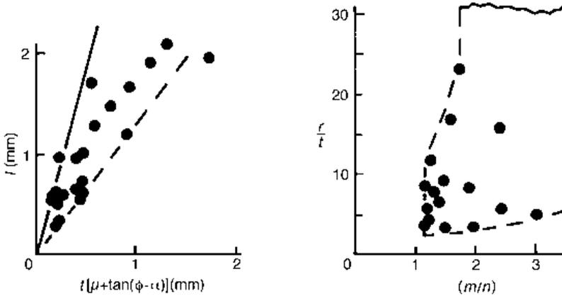
**Fig. 2.10** Chip/tool contact length and chip radius observations. (a) Measured dependence of chip/tool contact length on chip thickness; and (b) wide variations of dimensionless chip radius ( $r/t$ ) with  $(m/n)$
