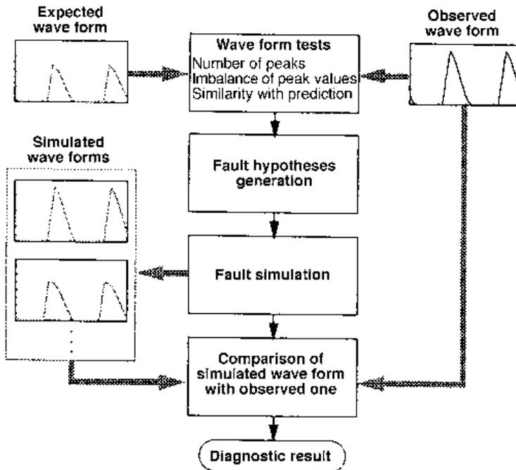
Fig. 9.38 Diagnosis procedure for faulty machining states (Takata, 1993)
