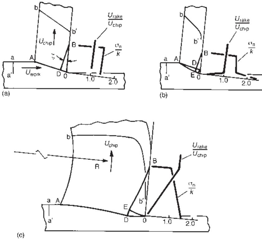
Fig. 6.2 Possibilities of chip formation,  $\alpha = 5^\circ$ ,  $m = 0.9$
