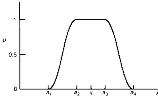
Fig. 9.21 Fuzzification of a numerical value  $\bar{x}$
