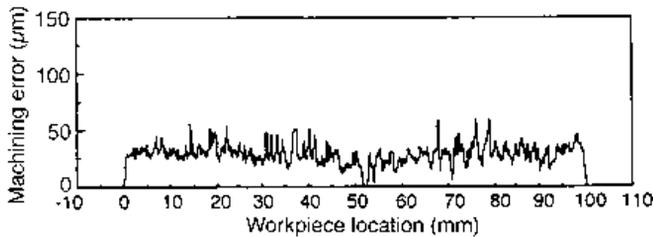
(d) Change in the machining error with the optimized feed rate command
