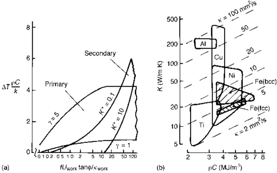
Fig. 3.2 Thermal aspects of machining: (a) a summary of heating theory and (b) thermal property ranges of Al, Cu, Fe, Ni and Ti alloys
