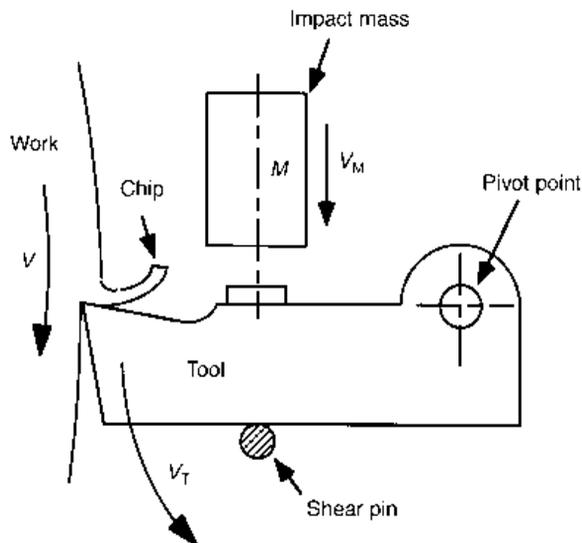
**Fig. 5.1** The principle of a quick-stop device for use in turning
