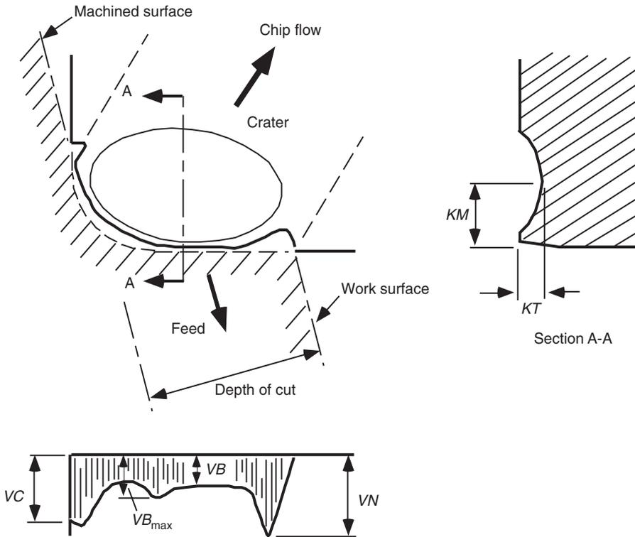
Fig. 4.1 Typical wear pattern of a carbide tool
