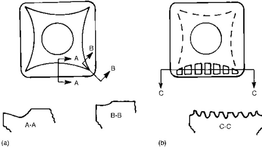
**Fig. 3.31** Three-dimensional opportunities for edge strengthening and chip control, not to scale: rake profile varying (a) smoothly along a cutting edge and (b) in a 'rib and pocket' manner
