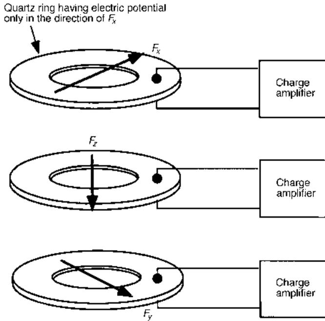
Fig. 5.10 The principle of piezoelectric dynamometry
