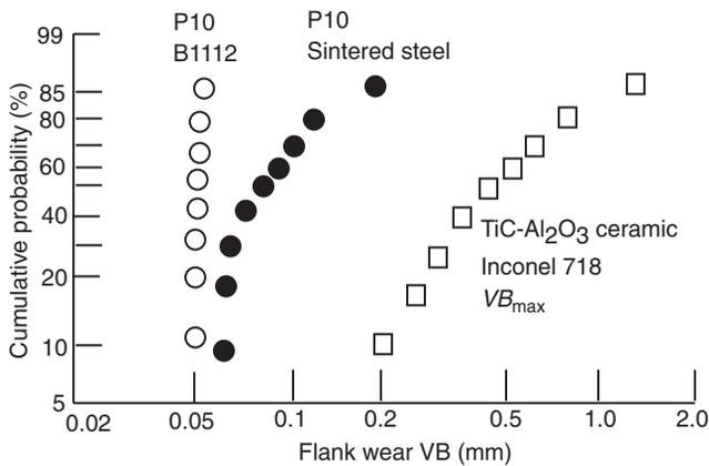
B112 - P10,  $V = 200\text{m/min}$ ,  $d = 0.5\text{mm}$ ,  $f = 0.1\text{mm/rev}$
