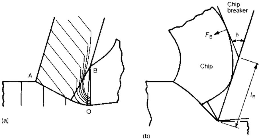
**Fig. 6.6** Slip-line field models of cutting with (a) zero rake restricted contact and (b) chip breaker geometry tools, after Usui *et al.* (1964) and Dewhurst (1979)
