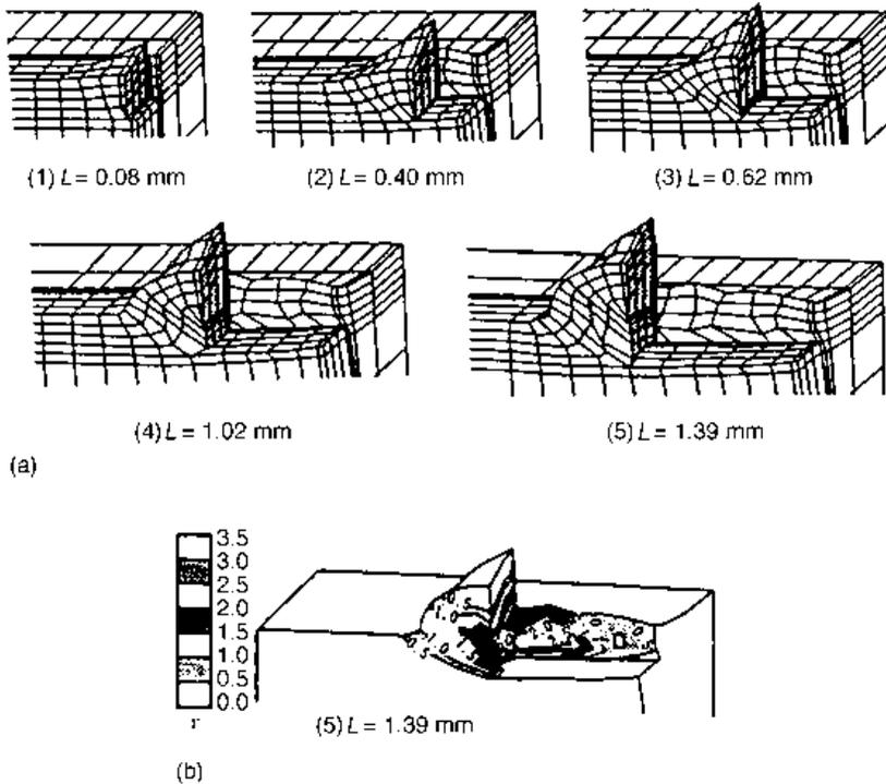
**Fig. 7.10** Three-dimensional non-steady chip formation (Sasahara *et al.*, 1994): (a) element deformations and (b) equivalent plastic strain distribution
