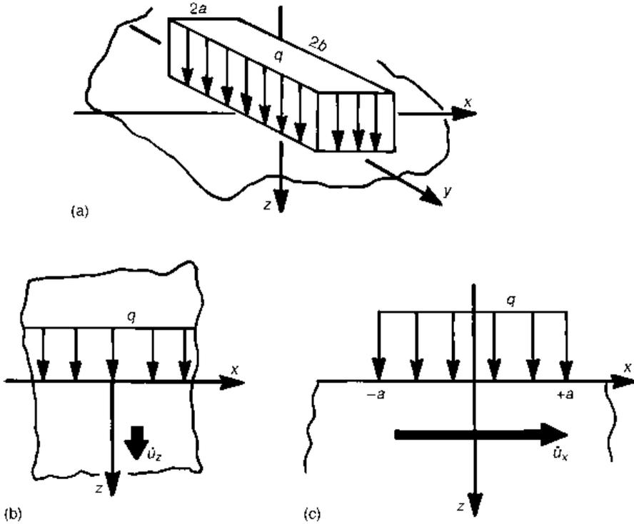
**Fig. A2.2** Some problems relevant to machining: (a) surface heating of a stationary semi-infinite solid; (b) an infinite solid moving perpendicular to a plane heat source; (c) a semi-infinite solid moving tangentially to the plane of a surface heat source
