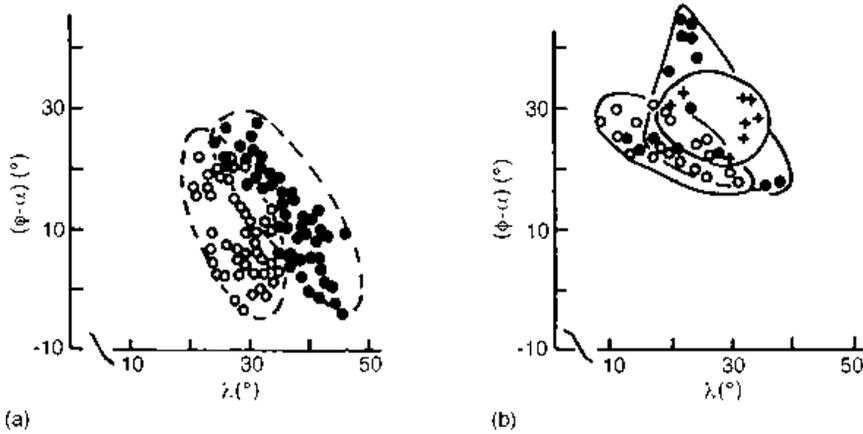
**Fig. 2.15**  $\phi$ - $\lambda$ - $\alpha$  relationships compared for (a) free-machining (o) and non-free machining ( $\bullet$ ) carbon and low alloy steels; and (b) austenitic stainless and high manganese steels (o), nickel-chromium heat resistant ( $\bullet$ ) and titanium alloys (+) turned by cemented carbide and ceramic tooling
