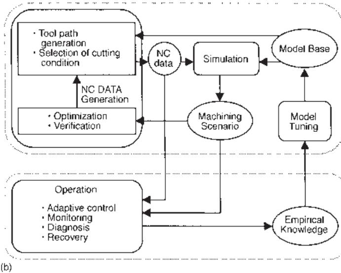
**Fig. 9.1** Model-based systems for design and control of machining processes: (a) CAD assisted milling process simulator and planner (Spence and Altintas, 1994) and (b) machining-scenario assisted intelligent machining system (Takata, 1993)
