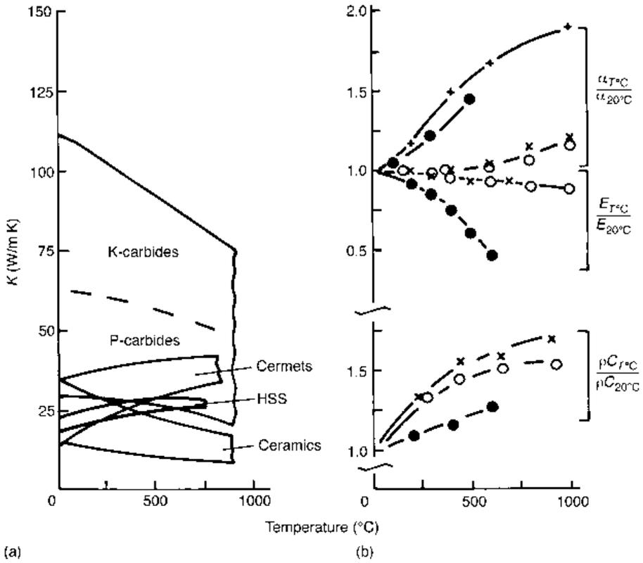
Fig. 3.24 The dependence on temperature of (a) thermal conductivity and (b) relative heat capacity, Young's modulus and thermal expansion coefficient, for HSS(•), carbide/cermet (x),  $\text{Al}_2\text{O}_3$ (o) and  $\text{Si}_3\text{N}_4$ (+) based tool materials
