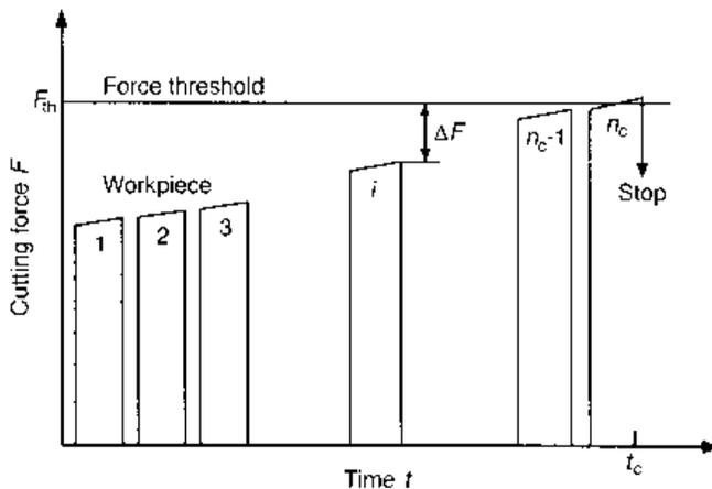
Fig. 9.24 Detection of tool life with a threshold
