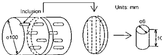
**Fig. 8.12** Specimen preparation for high speed compression testing
