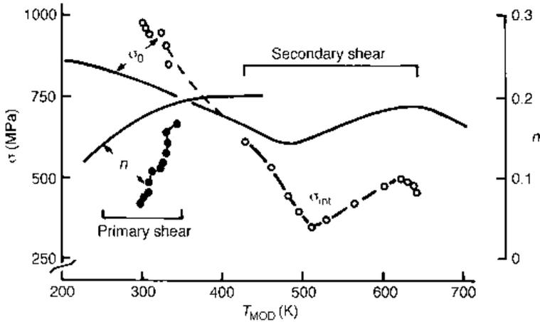
**Fig. 6.11** Variations of  $\sigma_0$  (o) and  $n$  (•) for a low carbon steel, derived from machining tests, compared with compression test data (—)
