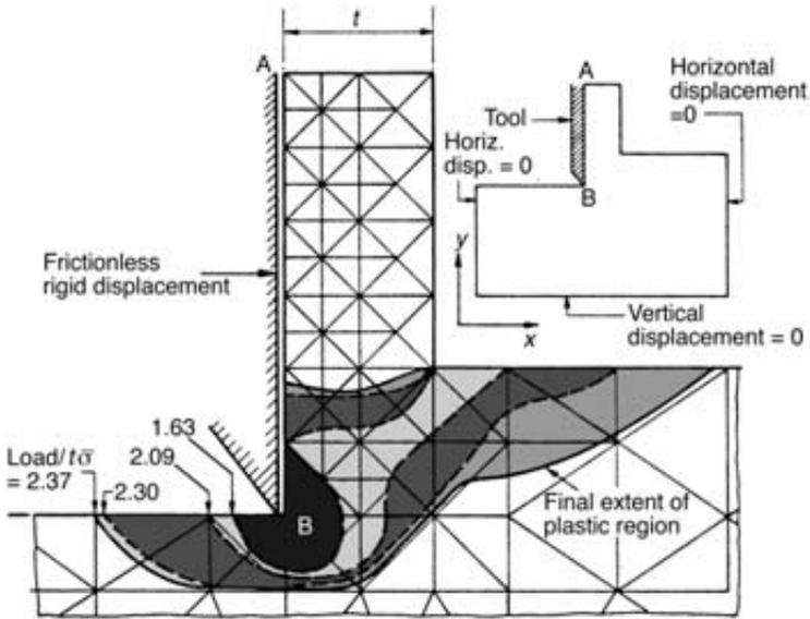
Fig. 7.3 Shear zone development, loading a pre-formed chip (Zienkiewicz, 1971)
