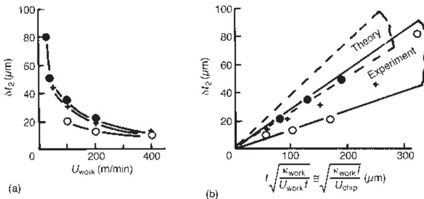
Fig. 6.12 Variation of flow-zone thickness with (a) cutting speed, at feeds (mm) of 0.5 (●), 0.25 (+) and 0.125 (○); and (b) replotted to compare with theory (see text)
