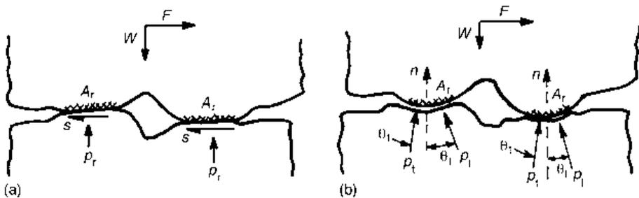
Fig. A3.1 Friction caused (a) by shear stresses  $s$  and (b) by direct stresses  $p$
