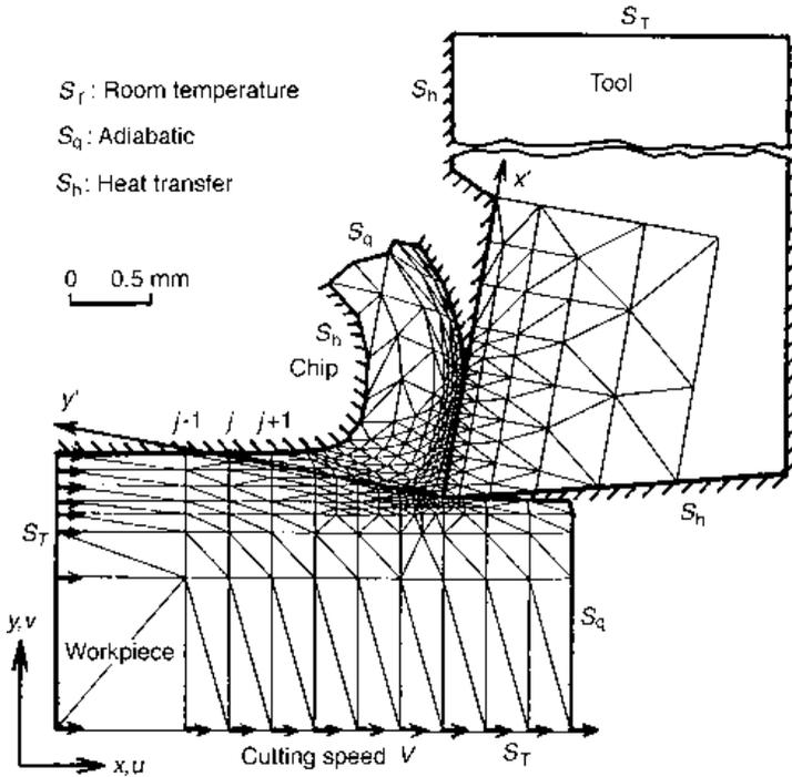
Fig. 7.13 Two-dimensional finite element assemblage with boundary conditions
