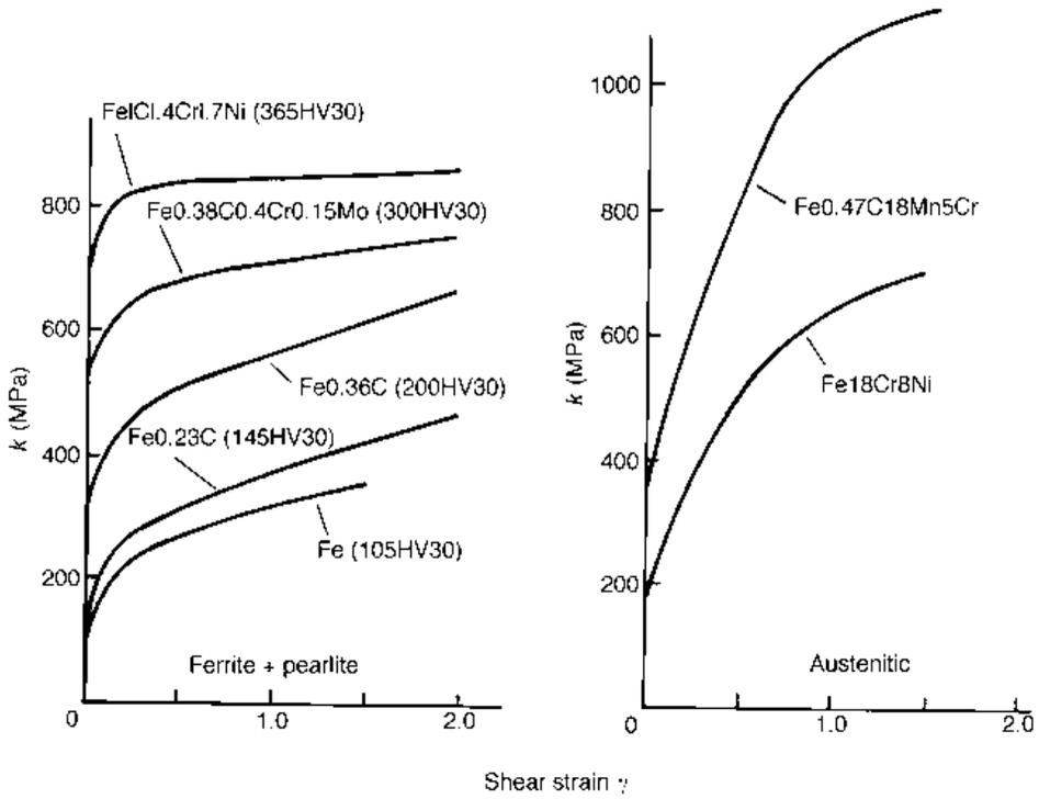
Fig. A4.2 Shear stress-strain behaviours of some ferritic/pearlitic and austenitic steels
