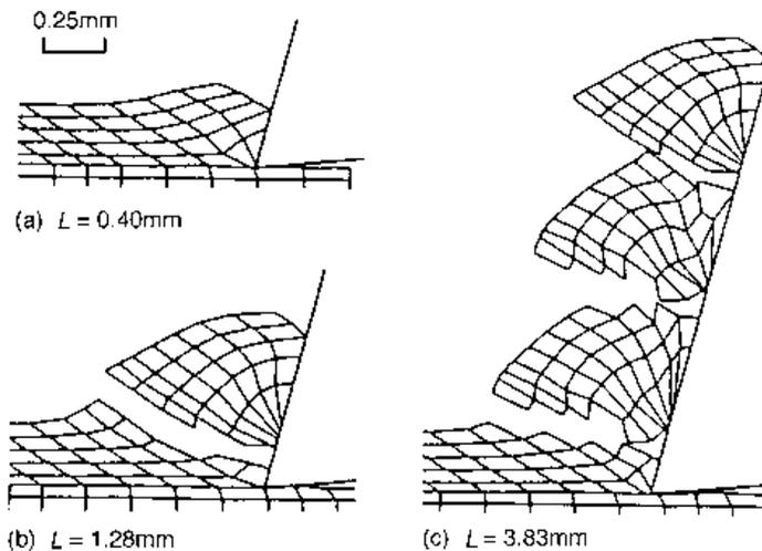
**Fig. 8.6** Predicted discontinuous chip in  $\beta$ -brass machining: cutting speed of 13 mm/min,  $f=0.25$  mm,  $d=1$  mm,  $\alpha=15^\circ$  and no coolant
