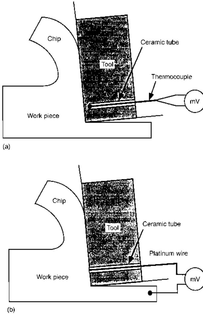
Fig.5.19 (a) Inserted thermocouple or (b) thermocouple wire
