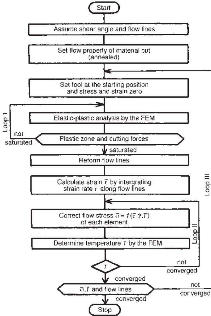
Fig. 7.12 Developed flow-chart of the iterative convergence method
