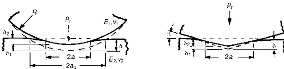
Fig. A3.2 Models of elastic asperity deformation
