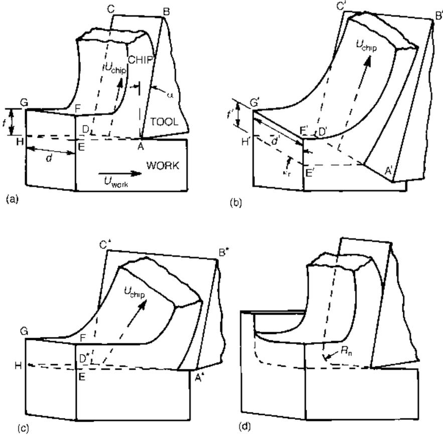
Fig. 2.2 (a and b) Orthogonal, (c) non-orthogonal and (d) semi-orthogonal chip formation.
