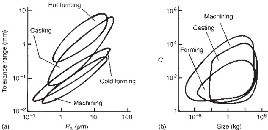
**Fig. 1.2** (a) Typical accuracy and finish and (b) complexity and size achievable by machining, forming and casting processes, after Ashby (1992)
