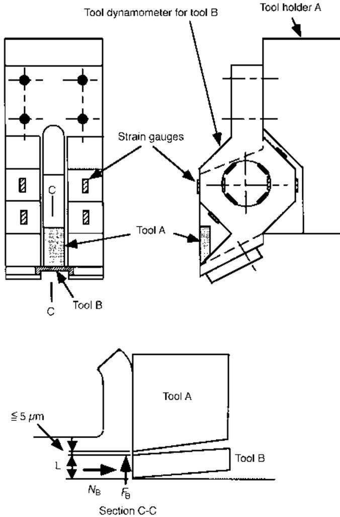
Fig. 5.12 A split-tool dynamometer arrangement
