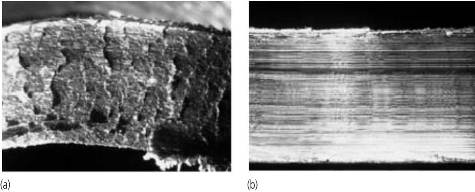
**Fig. 5.4** The back surface of chips formed from 0.15% C steel by P20 carbide tools: (a) with built-up edge,  $v = 40 \text{ m min}^{-1}$ ,  $d = 2.0 \text{ mm}$ ,  $f = 0.08 \text{ mm rev}^{-1}$ ; (b) without built-up edge,  $v = 100 \text{ m min}^{-1}$ ,  $d = 2.0 \text{ mm}$ ,  $f = 0.12 \text{ mm rev}^{-1}$ .
