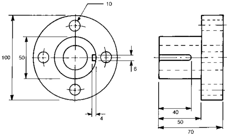
Fig. 1.25 An example machined component (dimensions in mm)
