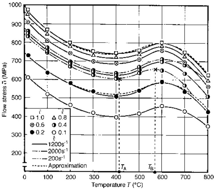
Fig. 8.5 Relation between flow stress and temperature of the 0.18% C steel
