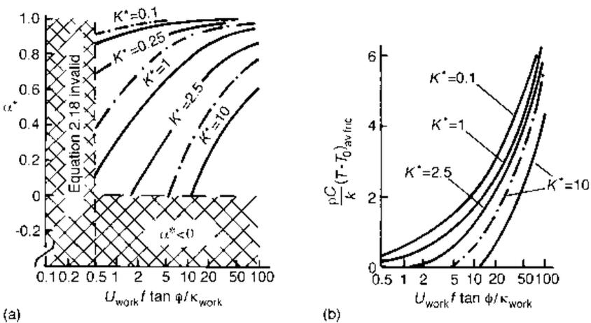
**Fig. 2.19** Dependence of (a)  $\alpha^*$  and (b) friction heating mean contact temperature rise on  $[U_{\text{work}} f \tan \phi / \kappa_{\text{work}}]$ ,  $K^* = K_{\text{tool}} / K_{\text{work}}$  from 0.1 to 10;  $s_f = 1$  (—) and 2 (---)
