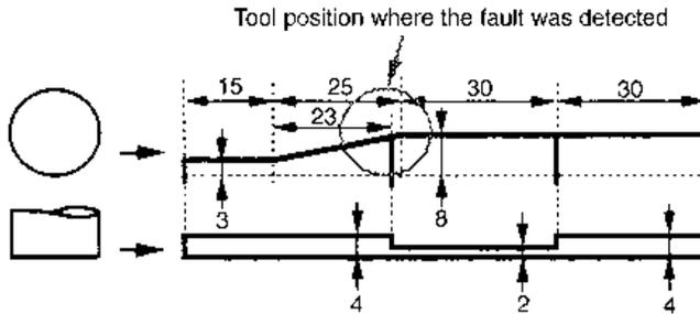
Fig. 9.39 Diagnosis of machining a different workpiece (Takata, 1993)
