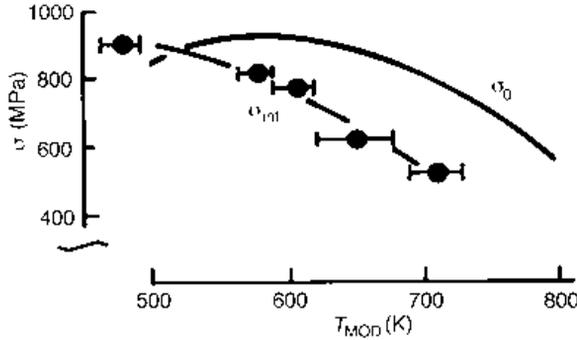
**Fig. 6.13** 0.45% C steel data from Figure 2.22(a), replotted ( $\bullet$ ) as  $\sigma_{\text{int}}$  versus  $T_{\text{MOD}}$  and compared with  $\sigma_0$  for a similar steel taken from Oxley (1989)
