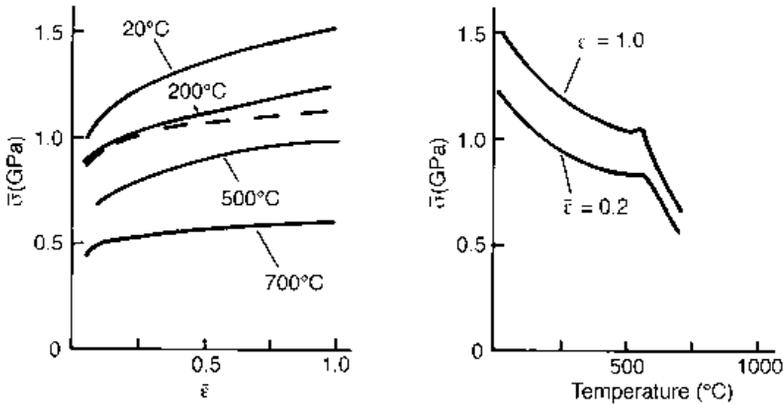
Fig. 7.21 Flow stress behaviour of a low alloy steel: dashed line at 20°C and a strain rate of 10<sup>-3</sup> s<sup>-1</sup>; solid lines at strain rate of 10<sup>3</sup> s<sup>-1</sup> and temperatures as marked
