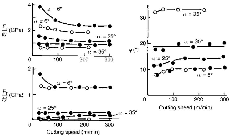
**Fig. 3.6** Specific force and shear plane angle variations for annealed (●) and pre-strained (○) commercially pure copper ( $f = 0.15$  to  $0.2$  mm,  $\alpha = 6^\circ$  to  $35^\circ$ )
