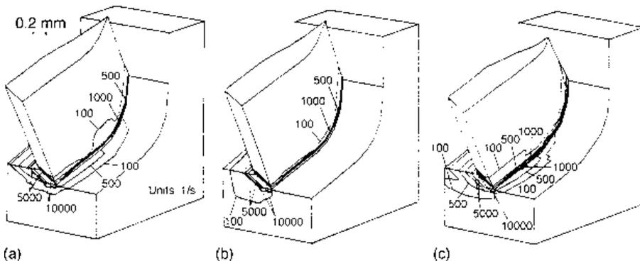
Fig. 8.29 Equivalent plastic strain rate distribution and chip configuration when machining 18%Mn-18%Cr steel at a cutting speed of 60 m/min,  $f = 0.2$  mm and  $d = 2$  mm with (a) conventional, (b) type I and (c) type II P20 carbide tools
