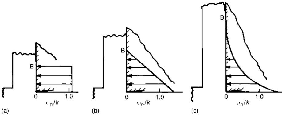
**Fig. 2.12** A range of possible rake face contact pressure distributions  $\sigma_n/k$ , for  $\alpha = 0^\circ$ ,  $\phi = 10^\circ$  and  $\lambda = 35^\circ$  and  $n =$  (a)  $1/2$ , (b)  $1/3$  and (c)  $1/6$
