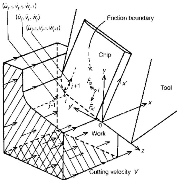
**Fig. 8.26** Three-dimensional machining model and boundary conditions
