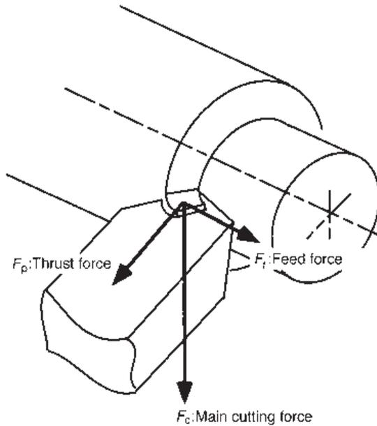
Fig. 5.5 Forces acting on cutting tool in turning
