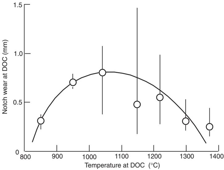
**Fig. 4.11** Al<sub>2</sub>O<sub>3</sub>/TiC DOC notch wear variation with temperature, turning Inconel 718 for 30 s at various speeds at a feed of 0.19 mm and a depth of cut of 0.5 mm, after Narutaki and Yamane (1993)
