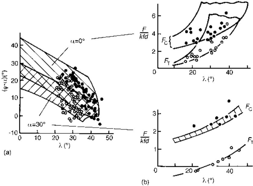
Fig. 6.3 Slip-line field allowed ranges of (a)  $(\phi - \alpha)$  and (b) specific forces and  $\lambda$ , for tools of rake angle  $0^\circ$  and  $30^\circ$ : experimental data for carbon steels (Childs, 1980)
