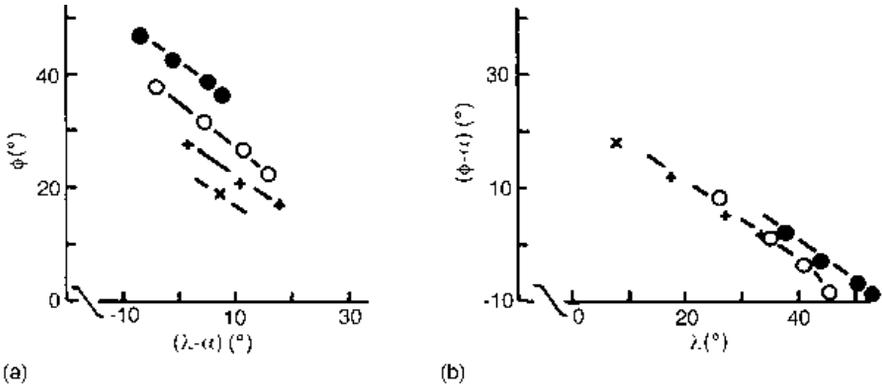
**Fig. 2.13**  $\phi$ - $\lambda$ - $\alpha$  relationships for low speed turning of a free cutting steel with tools of different rake angle (0°, 16°, 30°, 45°), varying friction by selection of cutting fluid: (a)  $\phi$  versus  $(\lambda - \alpha)$  and (b)  $(\phi - \alpha)$  versus  $\lambda$  (after Shaw, 1984)
