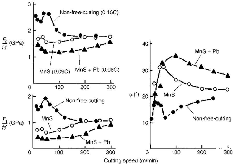
**Fig. 3.16** Representative specific force and shear plane angle variations for low carbon free-machining steels turned by a steel cutting grade of carbide tool ( $f = 0.1$  to  $0.15$  mm,  $\alpha = 6^\circ$ )
