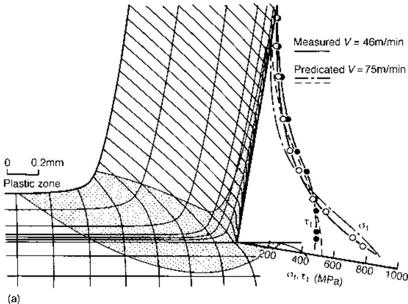
**Fig. 8.1** Simulated machining of a 0.18%C steel at a cutting speed of 75 m/min where no BUE appears: (a) distorted grid pattern and normal stress and friction stresses on the tool rake face, (b) distributions of maximum shear strain  $\gamma_m$  and strain rate  $\dot{\gamma}_m$  and (c) distributions of shear flow stress  $k$  and temperature  $T$  ( $^\circ\text{C}$ )
