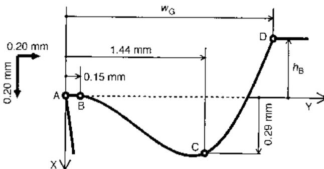
Fig. 8.20 Rake face geometry with chip former
