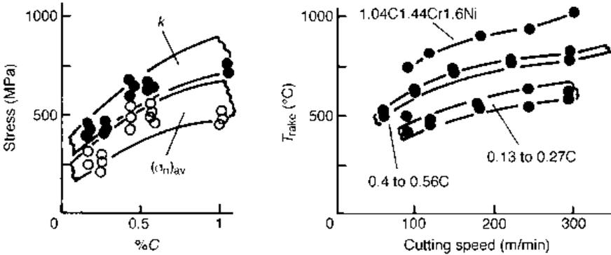
Fig. 3.13 Process stresses and temperatures derived from Figure 3.12
