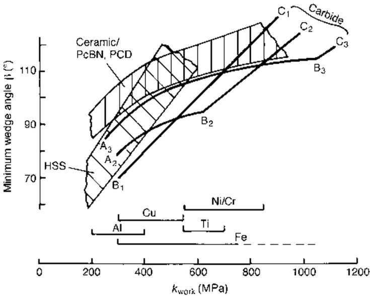
Fig. 3.27 Minimum values of  $\beta$  to prevent tool plastic or brittle failure, derived from Figure 3.26
