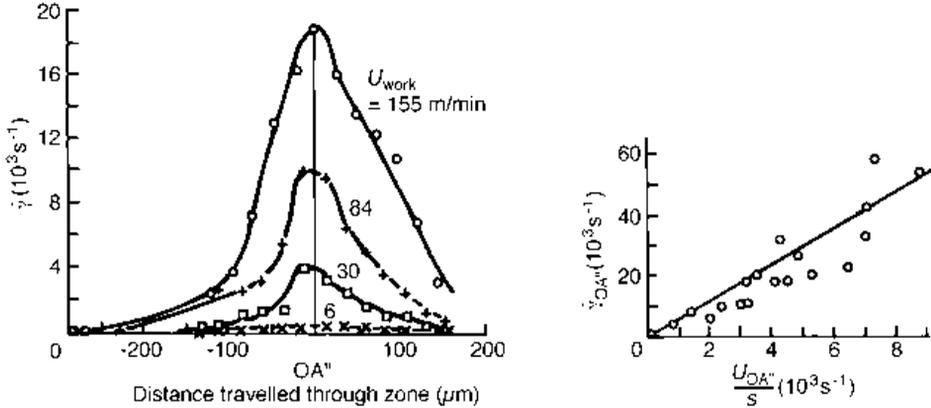
**Fig. 6.10** Shear strain rate variations along a central stream-line, and peak shear strain rate changes with cutting speed and feed, as described in the text
