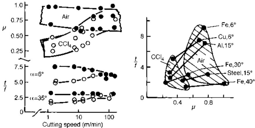
**Fig. 2.7** (a) Collected data on the machining of copper, dry ( $\bullet$ ) and lubricated ( $\circ$ ); and (b) lubricant effects for a range of conditions at cutting speeds around 1 m/min
