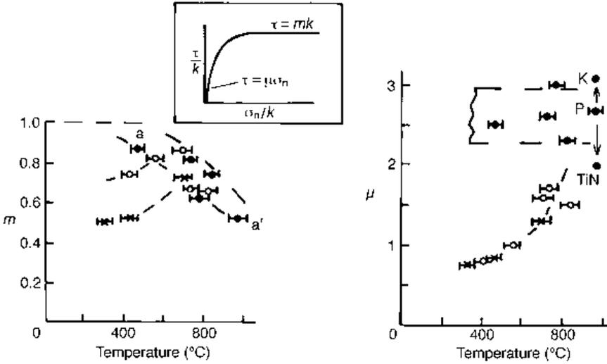
**Fig. 2.23**  $m$  and  $\mu$  variations with temperature for a plain carbon (•); a resulphurized (o); and a resulphurized and leaded (x) steel (authors' data)
