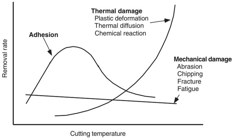
Fig. 4.3 Tool damage mechanisms and cutting temperature
