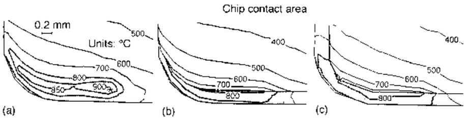
Fig. 8.30 Tool rake face isotherms in the conditions of Figure 8.29: (a) conventional, (b) type I; and (c) type II tools
