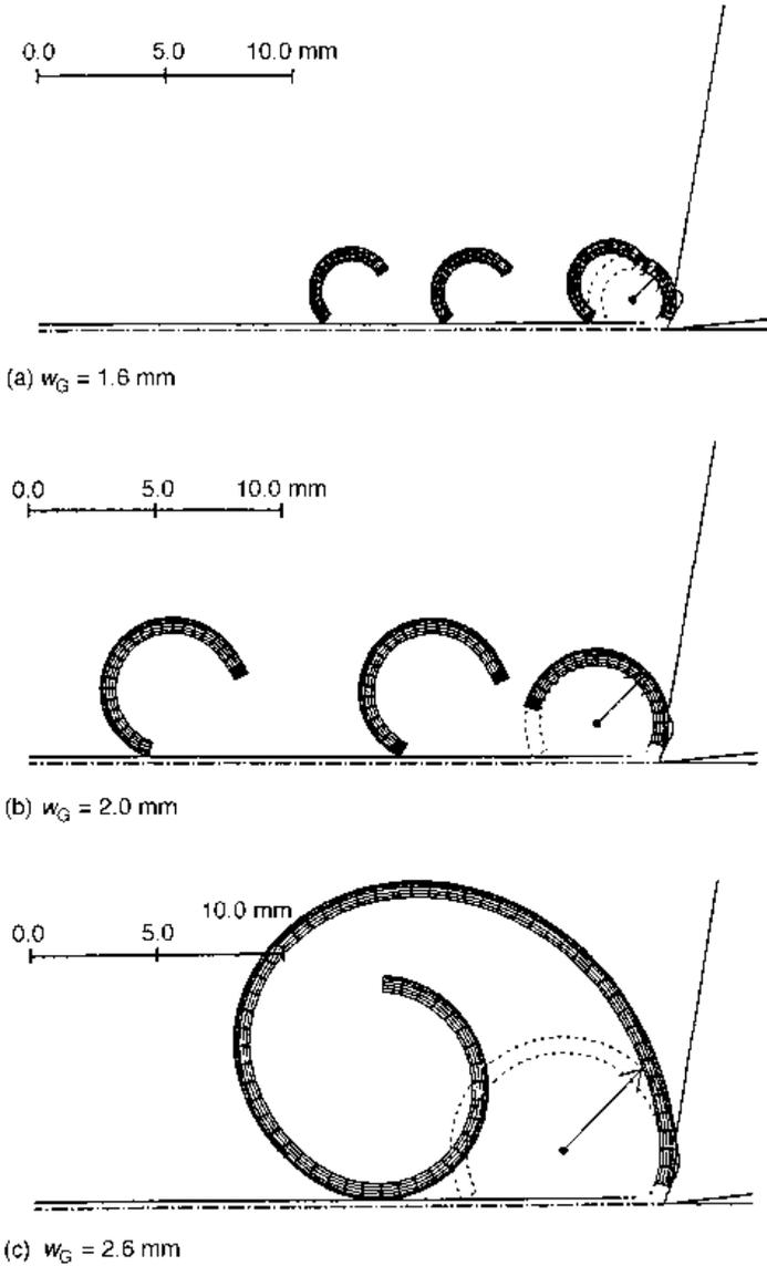
**Fig. 8.23** Predicted chip shape with changing  $w_G$  ( $h_b=0$ )
