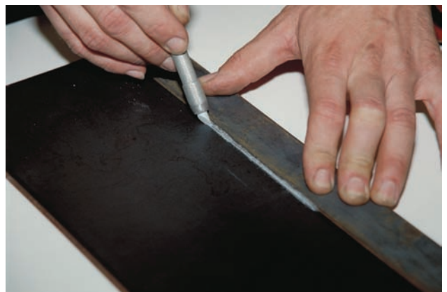
FIGURE 17-59 Be sure that the soapstone is held tightly to the part being traced. Courtesy of Larry Jeffus.
