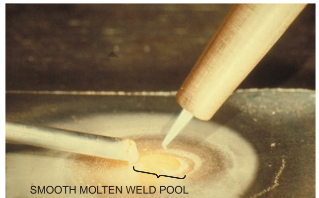
FIGURE 4-7 Neutral flame (balanced oxygen and acetylene). Courtesy of Larry Jeffus.
