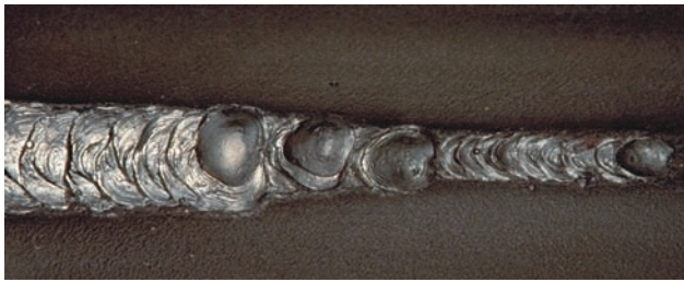
FIGURE 10-22 Uniformity in each pass shows a high degree of welder skill and increases the probability the weld will pass testing. Courtesy of Larry Jeffus.
