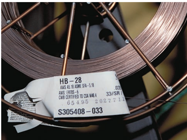
FIGURE 12-5 When installing the spool of wire, check the label to be sure that the wire is the correct type and size. Courtesy of Larry Jeffus.
