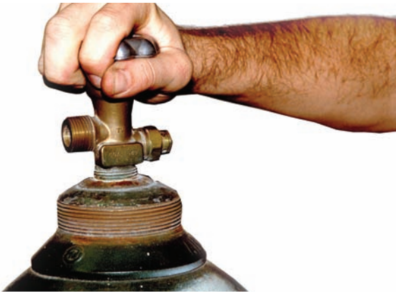
FIGURE 3-47 Crack the oxygen and fuel cylinder valves to blow out any dirt lodged in the valves. Courtesy of Larry Jeffus.
