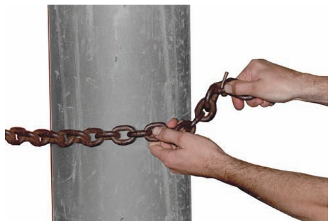
FIGURE 12-3 Make sure the gas cylinder is chained securely in place before removing the safety cap. Courtesy of Larry Jeffus.
