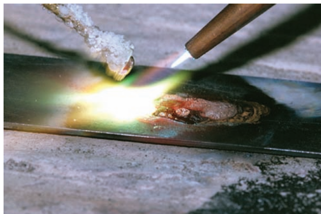
FIGURE 5-26 Observe the molten flux flowing ahead of the molten weld pool. Courtesy of Larry Jeffus.
