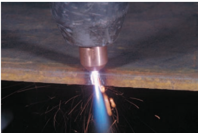
FIGURE 7-28 Start the plasma right next to the edge of the plate, and slowly bring it to the edge of the plate to start the cut.
