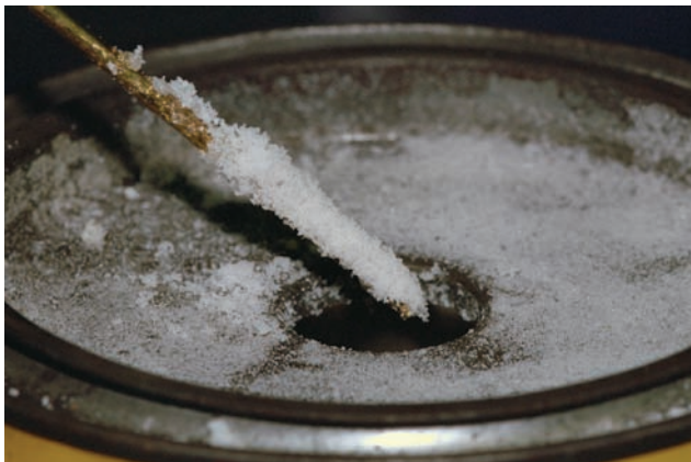
FIGURE 5-22(C) Flux stuck to rod ready for brazing. Courtesy of Larry Jeffus.
