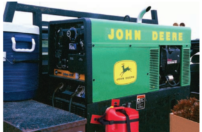
FIGURE 2-61 Magna-Ties™ are used to secure a gas can in the bed of this pickup truck. Courtesy of Larry Jeffus.
