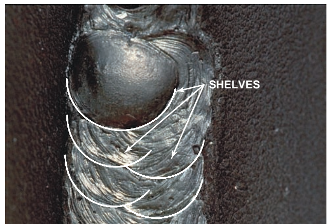
FIGURE 9-30 Using the shelf to support the molten pool for vertical welds. Courtesy of Larry Jeffus.
