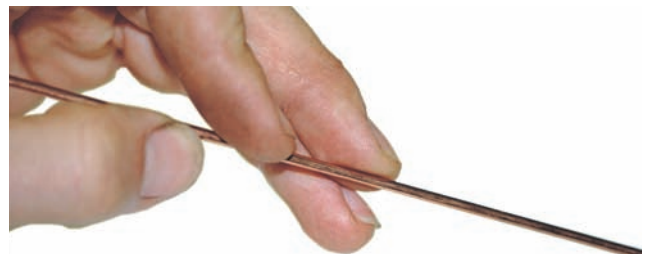
FIGURE 4-10 Feed the filler rod by using your index finger. Courtesy of Larry Jeffus.
