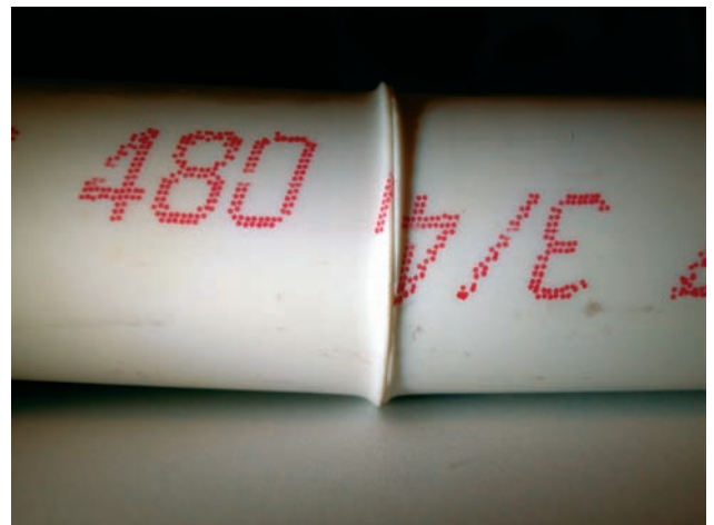
FIGURE 18-30 PVC butt weld. Courtesy of Larry Jeffus.
