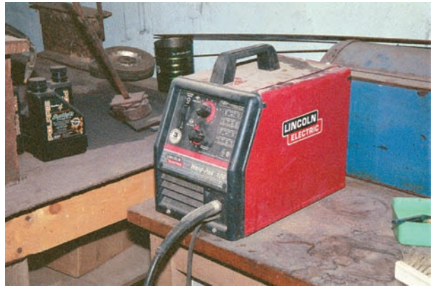
FIGURE 13-27 Although this is not the manufacturer's recommended way of storing an FCA welder, it's how they are often treated on farms and ranches. Courtesy of Larry Jeffus.
