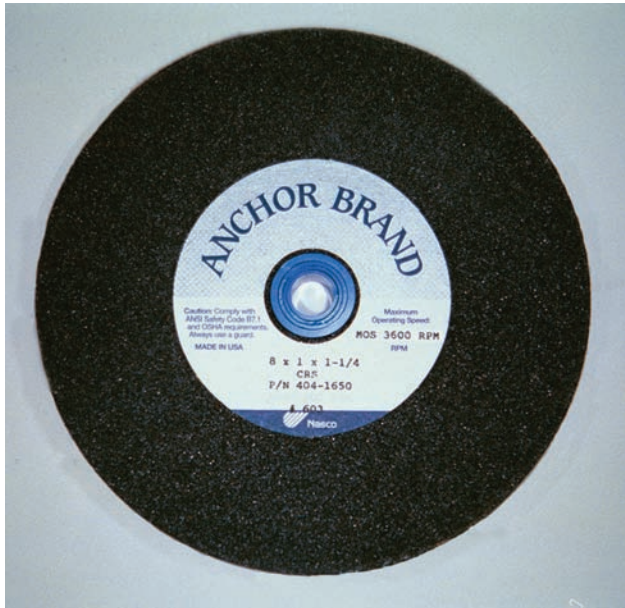
FIGURE 2-49 Always check to be sure that the grinding stone and the grinder are compatible before installing a stone. Courtesy of Larry Jeffus.
