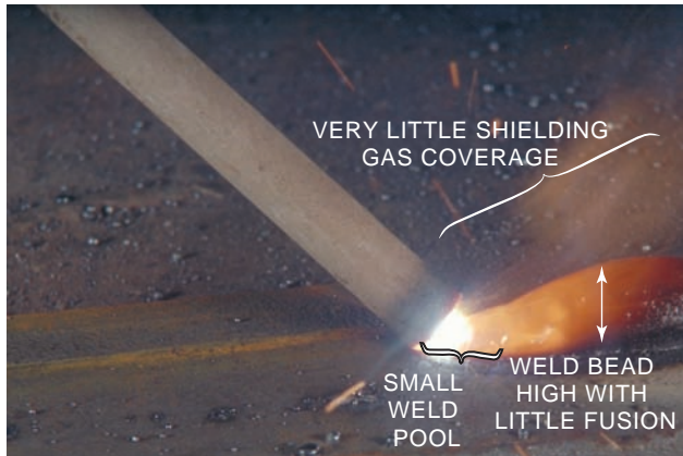
FIGURE 9-6 Welding with the amperage set too low.
