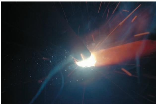
FIGURE 9-34 New welders frequently see only the arc and sparks from the electrode. Courtesy of Larry Jeffus.
