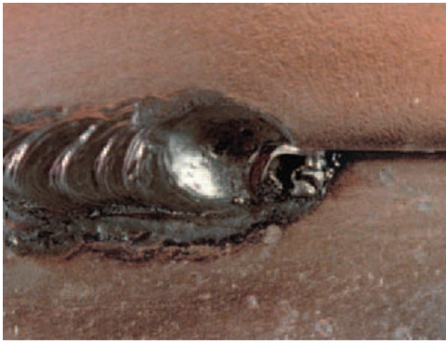
FIGURE 14-31 Watch the root of the weld bead to make sure there is complete fusion. Courtesy of Larry Jeffus.
