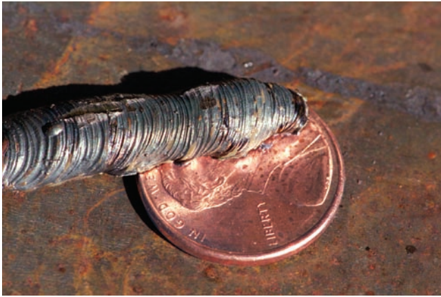
FIGURE 12-1 Weld separated from the plate; there is no fusion between the weld and plate. Courtesy of Larry Jeffus.
