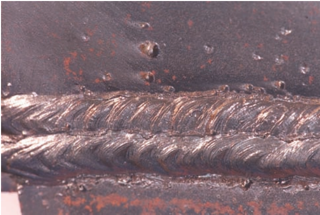
FIGURE 10-17 Filler pass using stringer beads. Courtesy of Larry Jeffus.
