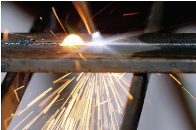
FIGURE 6-39 Poor cut. The slag is backing up because the cut is not going through the plate. Courtesy of Larry Jeffus.
