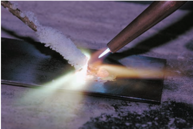
FIGURE 5-24 Checking the surface temperature with a spot of braze metal. Courtesy of Larry Jeffus.
