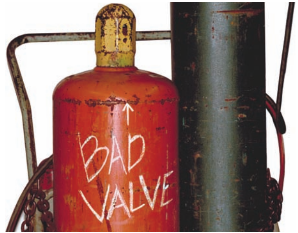
FIGURE 3-59 Identify any cylinder that has a problem by marking it. Courtesy of Larry Jeffus.
