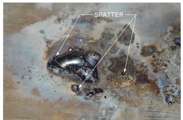
FIGURE 9-8 Hard weld spatter fused to base metal.
