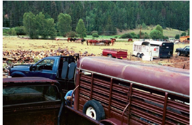
FIGURE 2-4 Truck was parked so horses could not look at arc. Courtesy of Larry Jeffus.
