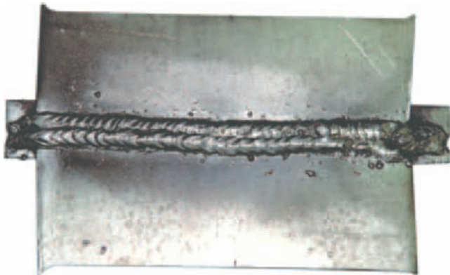
FIGURE 14-23 Starting and runoff tabs help control possible underfill or burn-back at the starting and stopping points of a groove weld. Courtesy of Larry Jeffus.
