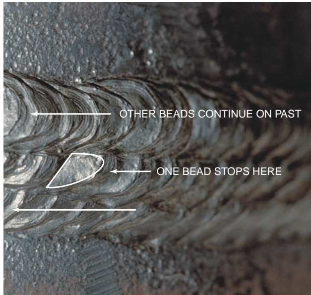
FIGURE 10-20 Avoid starting and stopping all weld passes in the same area. Courtesy of Larry Jeffus.
