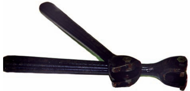
FIGURE 2-51 Use a grinding stone redressing tool as needed to keep the stone in balance. Courtesy of Larry Jeffus.
