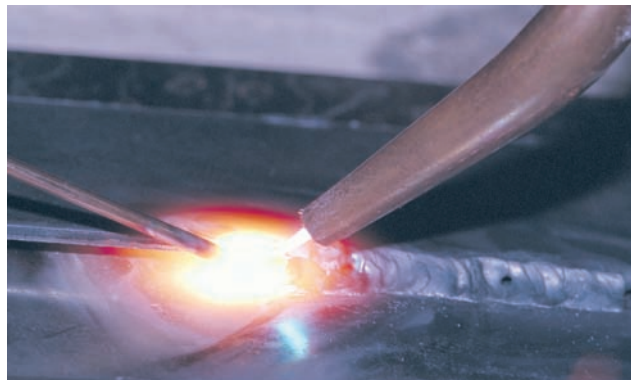
FIGURE 4-20 Filler metal being incorrectly added by allowing the rod to melt and drip into the molten weld pool. Courtesy of Larry Jeffus.
