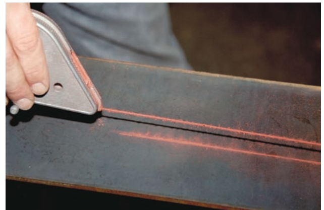
FIGURE 17-44(B) Check to see that the line is dark enough. Courtesy of Larry Jeffus.
