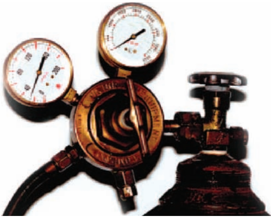
FIGURE 3-53 Back out both regulator adjusting screws before opening the cylinder valve. Courtesy of Larry Jeffus.
