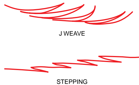
FIGURE 9-65 “J” weave and stepped pattern.
