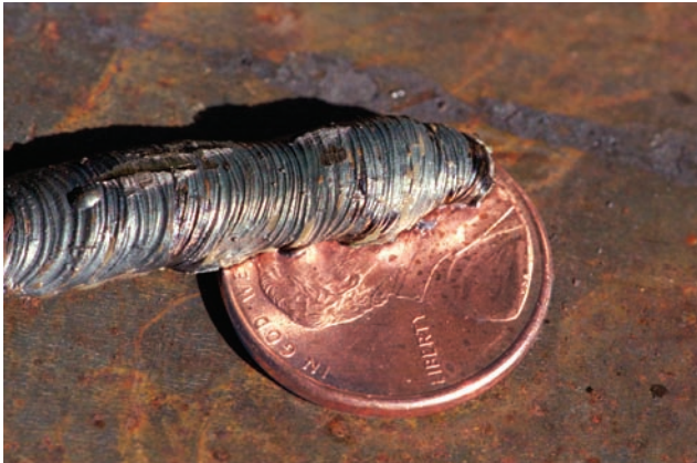
FIGURE 16-1 Improper welding technique for filler metal resulting in lack of fusion. Courtesy of Larry Jeffus.
