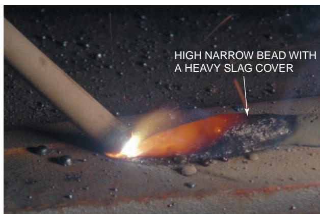
FIGURE 9-11 Welding with too short an arc length. Courtesy of Larry Jeffus.
