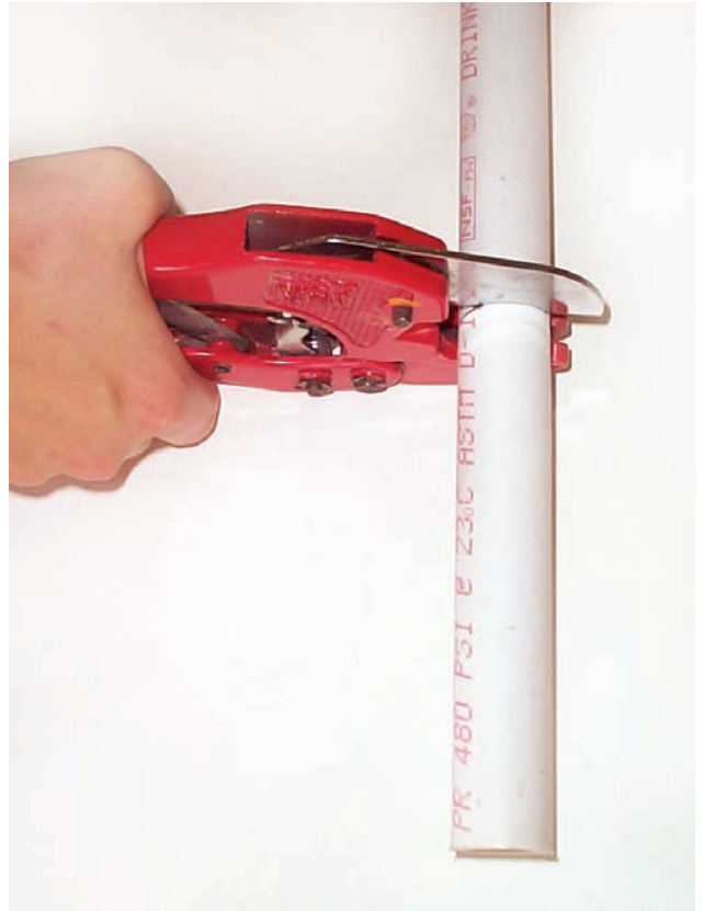
FIGURE 18-24 Cut the PVC with ratchet scissors plastic pipe cutter. Courtesy of Larry Jeffus.
