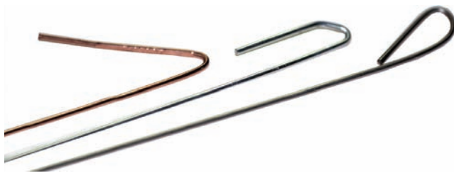
FIGURE 4-11 The end of the filler rod should be bent for safety and easy identification. Courtesy of Larry Jeffus.
