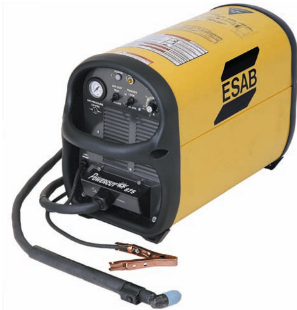
FIGURE 7-1 Plasma arc cutting machine. This unit can have additional power modules added to the base of its control module to give it more power. Courtesy of ESAB Welding & Cutting Products.
