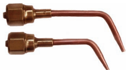
FIGURE 3-20 A variety of tip styles and sizes for one torch body. Courtesy of Larry Jeffus.
