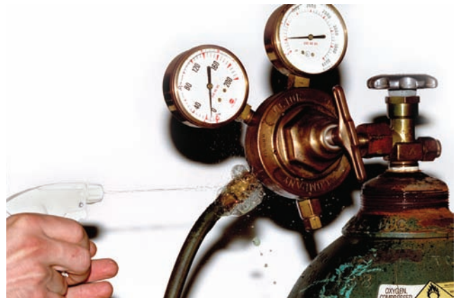
FIGURE 3-18 Check all connections for possible leaks and tighten if necessary. Courtesy of Larry Jeffus.
