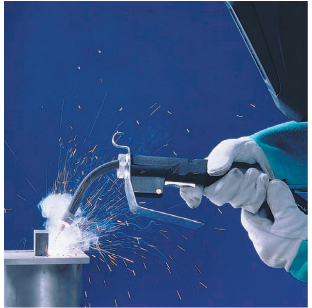
FIGURE 11-27 A typical GMA welding gun used for most welding processes with a heat shield attached to protect the welder's gloved hand from intense heat generated when welding with high amperages. Courtesy of Tweco, a Thermadyne Company.
