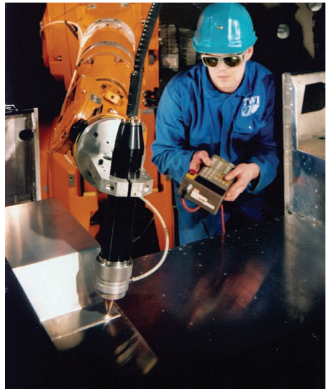
FIGURE 11-20 Robot welding. Courtesy of ESAB Welding & Cutting Products.
