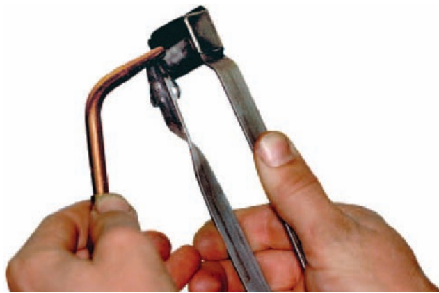
FIGURE 3-61 Sparklighter held too close over the end of the tip. Courtesy of Larry Jeffus.
