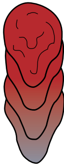
FIGURE 9-54 Watch the trailing edge of the weld pool to judge the correct travel speed.
