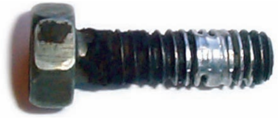
FIGURE 5-1(B) Solder has been applied to the threads to act as a lock tight. Courtesy of Larry Jeffus.
