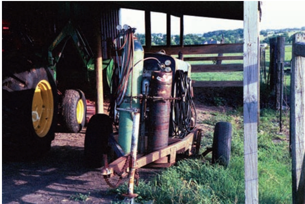
FIGURE 8-32 Keep leads stored so they will not be damaged. Courtesy of Larry Jeffus.
