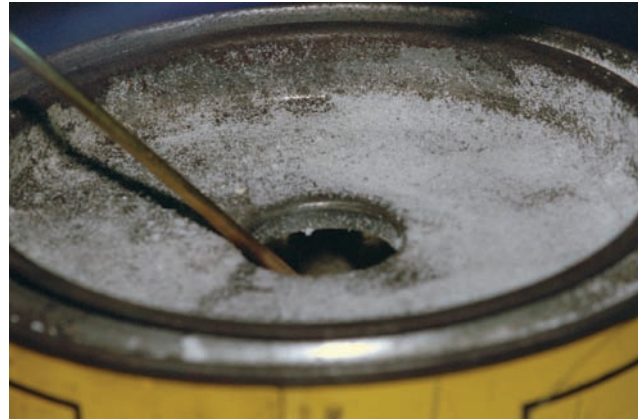
FIGURE 5-22(B) Dipping the heated rod into the flux. Courtesy of Larry Jeffus.
