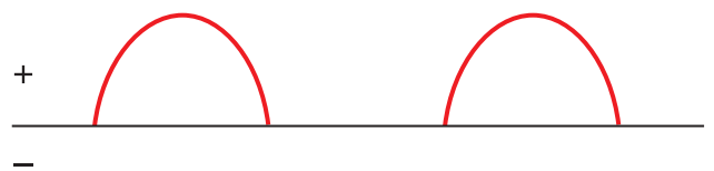
FIGURE 8-28 One rectifier in a welding power supply results in pulsating power.
