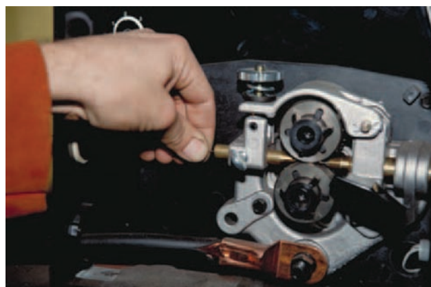
FIGURE 14-7 Push the wire through the guides by hand. Courtesy of Larry Jeffus.
