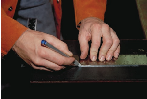
FIGURE 17-48 Using a square to draw a straight line. Courtesy of Larry Jeffus.
