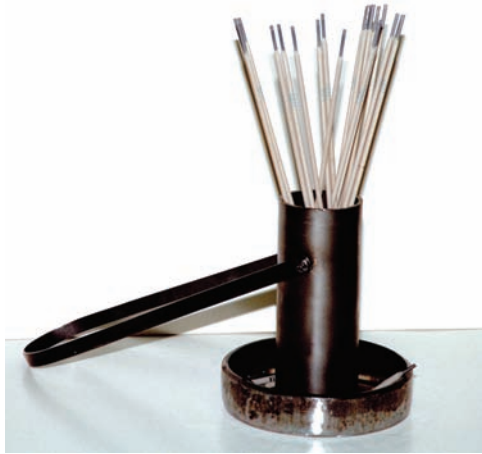
FIGURE 2-43 An easy-to-build electrode caddy can be used to hold both electrodes and stubs. Courtesy of Larry Jeffus.
