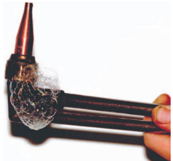
FIGURE 6-12 Checking a cutting tip for leaks. Courtesy of Larry Jeffus.
