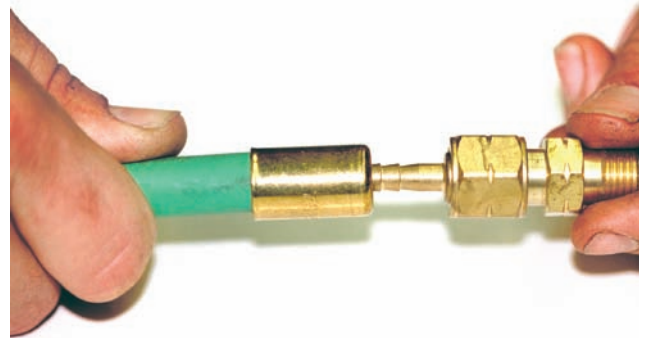
FIGURE 3-29 Screwing the hose nut onto a fitting will help when pushing the nipple into the hose. Courtesy of Larry Jeffus.
