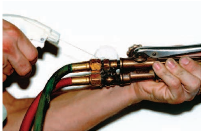
FIGURE 6-14 Leak-check all gas fittings. Courtesy of Larry Jeffus.
