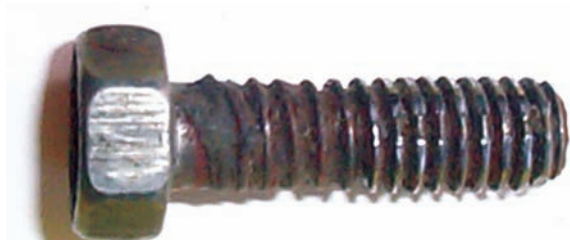
FIGURE 5-1(A) This bolt's threads are too worn to hold without vibrating loose. Courtesy of Larry Jeffus.
