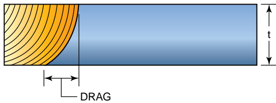
FIGURE 6-27 Drag is the distance by which the bottom of a cut lags behind the top.
