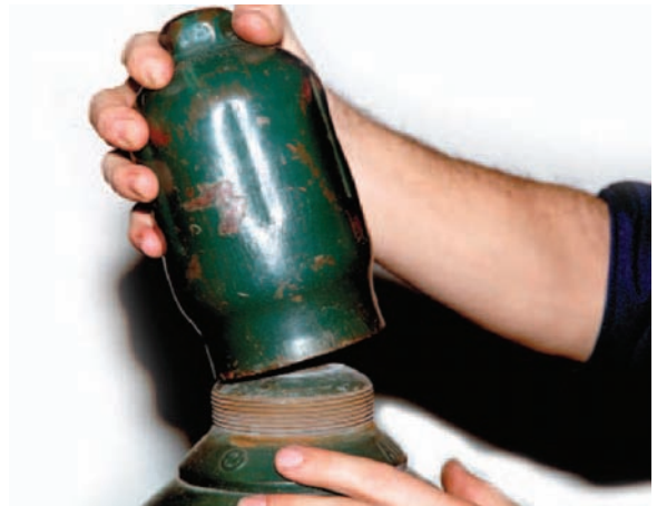
FIGURE 3-46 Unscrew the valve protector caps. Put the caps in a safe place, because they must be replaced on empty cylinders before they are returned. Courtesy of Larry Jeffus.
