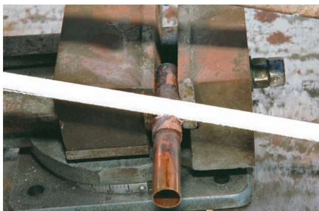
FIGURE 5-46 Saw the joint in two. Courtesy of Larry Jeffus.
