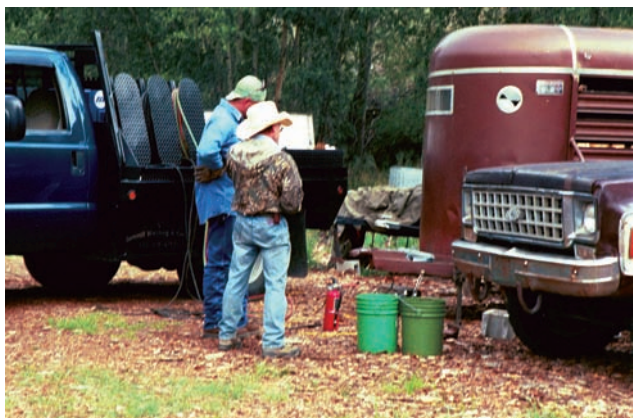
FIGURE 6-52 Have plenty of water and a fire extinguisher available before starting to cut or weld. Courtesy of Larry Jeffus.
