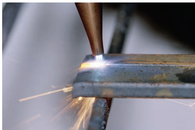
FIGURE 6-58 The torch is rotated to allow the preheating of the plate ahead of the cut. This speeds the cutting and also provides better visibility of the line being cut. Courtesy of Larry Jeffus.
