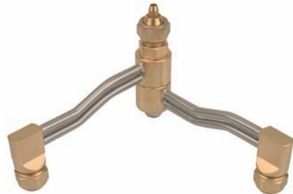
FIGURE 6-49 Slitting adaptor for cutting machine. It can be used for parallel cuts from 1 in. (38 mm) to 12 in. (500 mm) and is ideal for cutting test coupons. Courtesy of Victor Equipment, a Thermadyne Company.
