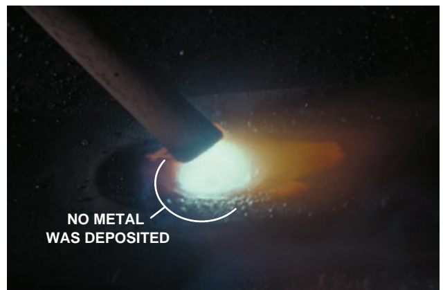
FIGURE 9-29 The electrode does not deposit metal or melt the base metal. Courtesy of Larry Jeffus.
