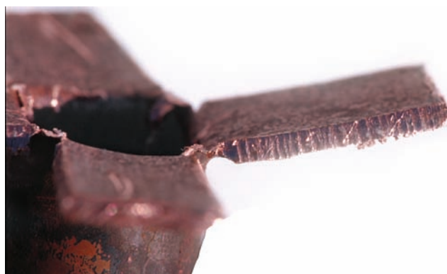
FIGURE 5-49 Complete joint fill. Courtesy of Larry Jeffus.
