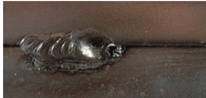
FIGURE 9-40 The tack weld should be small and uniform to minimize its effect on the final weld. Courtesy of Larry Jeffus.
