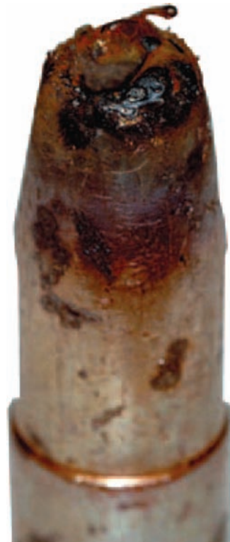
FIGURE 12-41 Gas nozzle damaged after shorting out against the work. Courtesy of Larry Jeffus.
