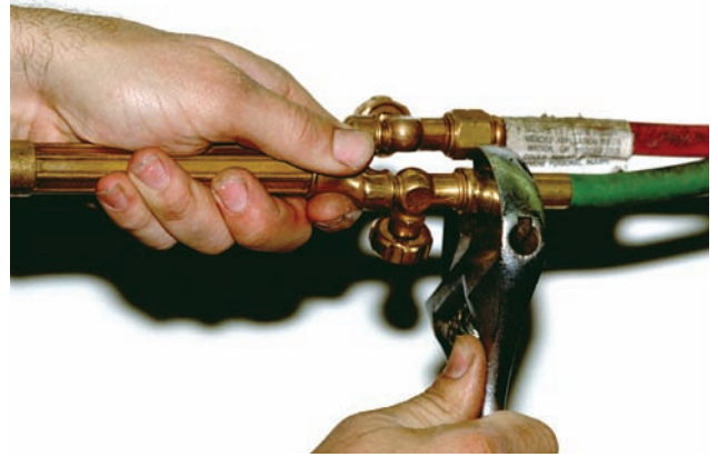
FIGURE 3-17 One hose fitting nut will protect the threads when the other nut is loosened or tightened. Courtesy of Larry Jeffus.
