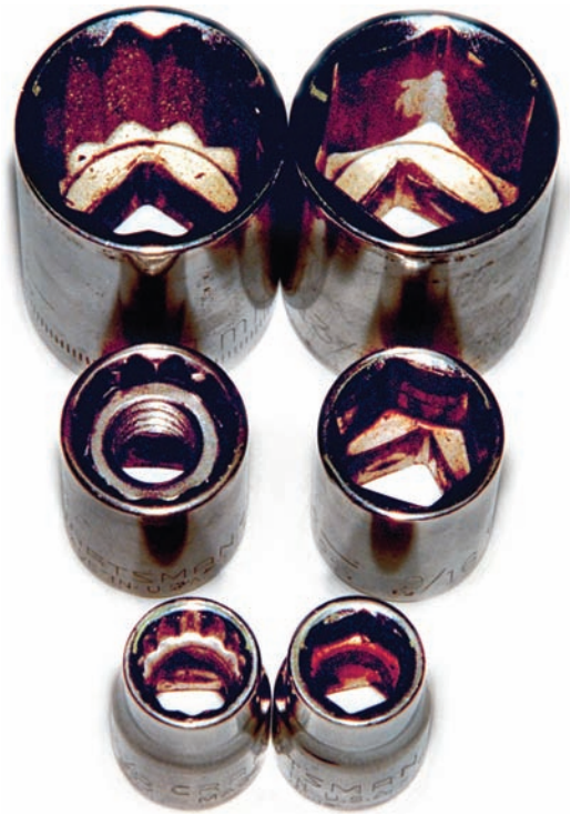
FIGURE 2-45 The fewer the points, the less likely the wrench is to slip. Courtesy of Larry Jeffus.
