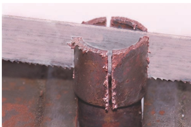
FIGURE 5-47 Quarter-saw the joint. Courtesy of Larry Jeffus.
