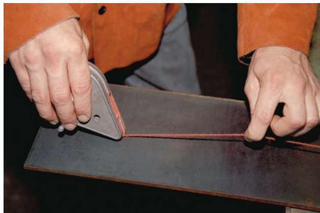
FIGURE 17-44(A) Pull the chalk line tight and then snap it. Courtesy of Larry Jeffus.
