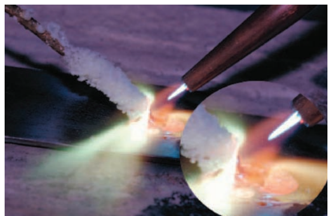
FIGURE 5-23 Deposit a spot of braze on the plate and continue heating the plate until the braze flows onto the surface. Courtesy of Larry Jeffus.
