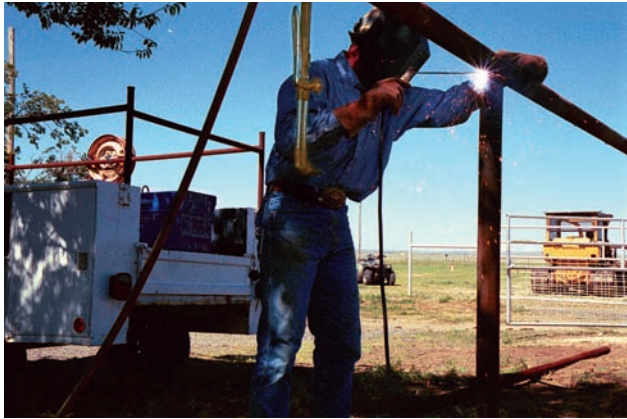
FIGURE 8-23 Engine generator welders make welding on a ranch easier. Courtesy of Larry Jeffus.
