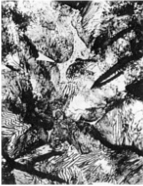
Fig. 7 Steadite in gray cast iron. Etched using 2% nital. 400×
