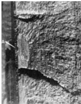
Fig. 14 Changes in fracture mechanism and appearance that were caused by changes in chemical and stress environment for a chromium-plated aluminum alloy 7079-T6 forging. Small corrosion pits formed beneath the layer of chromium plate, as at A, and generated stress-corrosion cracks B. Growth of these cracks altered the stress intensity at the crack tips, leading to propagation of fatigue cracks C. Final, fast fracture D occurred when the critical crack-tip stress-intensity value was reached. Light fractograph. 5.7\times
