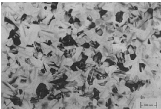
Fig. 17 Transmission electron microscopy grain orientation contrast in a sample of fine-grained polycrystalline silicon. Courtesy of Tom Headley, Sandia National Laboratories
