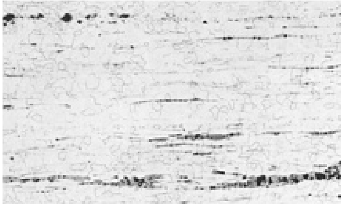
Fig. 17 Microstructure of wrought iron (longitudinal plane). Etched with 2% nital. 50×
