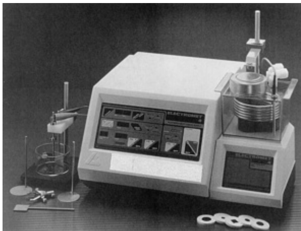
Fig. 14 A commercially available electrolytic polishing and etching system
