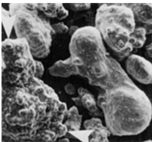
Fig. 5 Scanning electron micrograph of water-atomized iron particles exhibiting a fair degree of irregularity or roughness on the surface (note particle indicated by arrows). 190×
