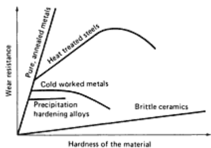
Fig. 8 Schematic representation of the correlation between wear resistance and hardness of different materials in various microstructural conditions
