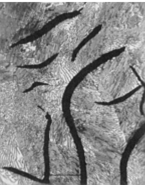
Fig. 2 Class 30 gray iron, as-cast. Structure consists of type A graphite in a pearlitic matrix.
