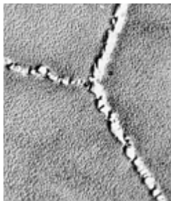
Fig. 6 Continuous or nearly continuous MC film produced in grain boundaries of Waspaloy after high-temperature forging soak with no subsequent reduction, followed by normal solution treating and aging. 2700×
