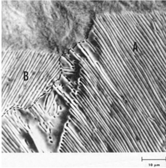
Fig. 7 Secondary electron image of polished and etched sample of Fe-0.8%C showing details of pearlite (A and B) growing into austenite (transformation interrupted by quenching). Source: Ref 3
