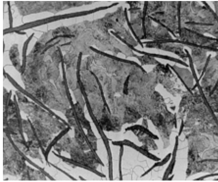
Fig. 3 Microstructure of a gray cast iron with a ferrite-pearlite matrix. Note the graphite flakes dispersed throughout the matrix. 4% picral etch. 320 \times . Courtesy of A.O. Benscoter, Lehigh University
