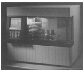
Fig. 10 A fully automatic polishing system
