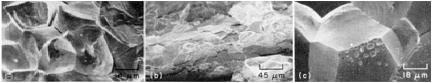
Fig. 20 Intergranular brittle fractures in tungsten, iridium, and a tungsten-3 wt% rhenium alloy. (a) Sintered tungsten rod drawn to 1.5 mm (0.060 in.) diam, recrystallized for 100 h at 10^{-6} torr and 2600 °C (4712 °F), and fractured in tension. (b) Iridium sheet annealed for 50 h in purified helium at 1700 °C (3092 °F) and broken by bending. (c) Tungsten-3 wt% rhenium alloy that was prepared in the same manner as the sintered tungsten rod in fractograph (a). Microvoids ("bubbles") at grain boundaries resulted from segregation of potassium (an impurity).
