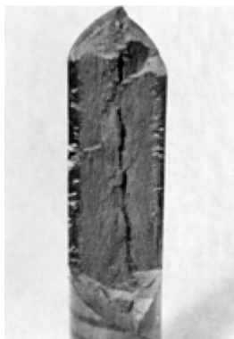
Fig. 9 A torsional-fatigue fracture in an induction-hardened 1037 steel shaft 25 mm (1 in.) in diameter that finally fractured in longitudinal shear. No clear point of origin is visible because the surfaces rubbed as the crack propagated. Light fractograph. \sim 0.95\times
