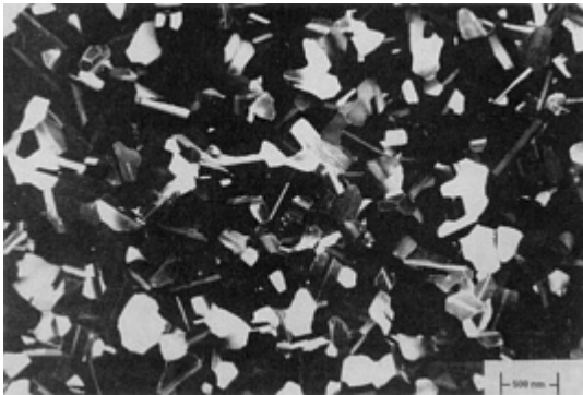
Fig. 19 Transmission electron microscopy dark field image of same area as in Fig. 17. Dark field image was obtained by imaging numerous diffraction spots, so most areas that strongly diffracted and appeared dark in Fig. 17 now appear bright. Areas that diffracted weakly and appeared bright in Fig. 17 now appear dark. Courtesy of Tom Headley, Sandia National Laboratories
