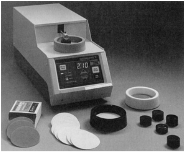
Fig. 11 An automatic single-specimen grinder/polisher
