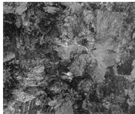
Fig. 2 Microstructure of a typical fully pearlitic rail steel showing the characteristic fine pearlite interlamellar spacing. 2% nital + 4% picral etch. 500×
