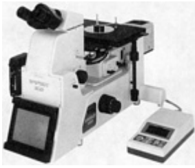
Fig. 16 Example of an inverted metallurgical reflecting microscope for photomicroscopy (referred to as a metallograph). Courtesy of C. Brandmaier, Nikon Inc.
