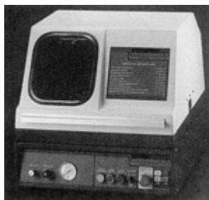
Fig. 1 A tabletop automated abrasive cutoff saw
