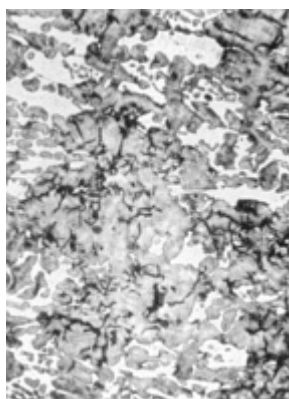
Fig. 6 Mottled cast iron etched using 4% picral. The white phase is eutectic carbide. 50×
