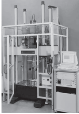
Figure 3.1 Instron VzHS160/100-20 High Velocity Testing System
