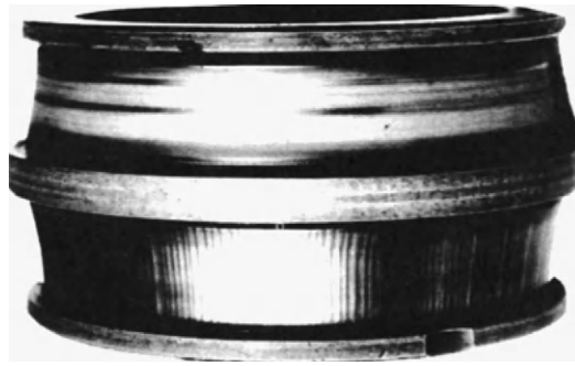
Figure 3-64: Fluting on inner raceway of spherical roller bearing.
