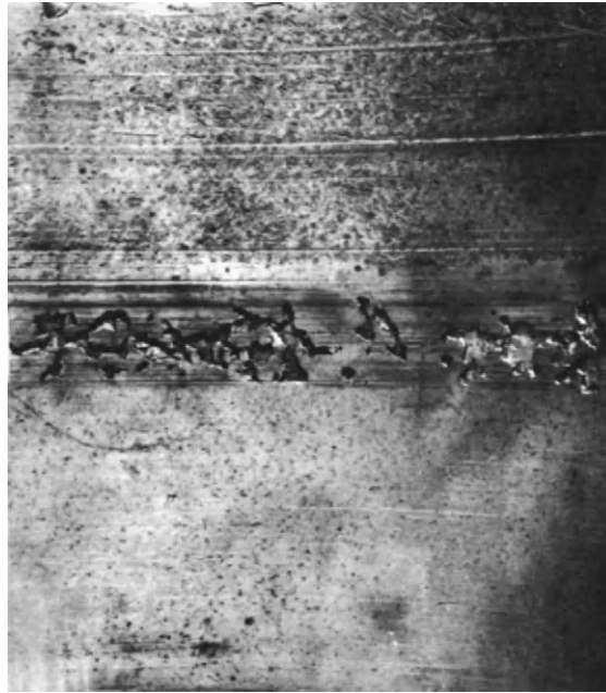
Figure 3-74: Fatigue cracking due to shaft ridging.
