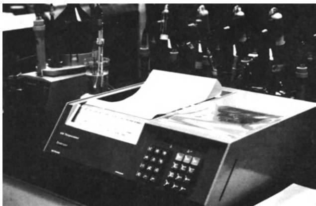
Figure 3-185: Titroprocessor determines total acid number.
