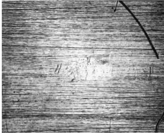
Figure 3-58: Example of false brinelling—100x.
