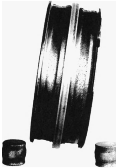
Figure 3-48: Advanced abrasive wear.
