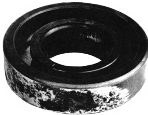
Figure 3-18: Wear due to fretting corrosion.
