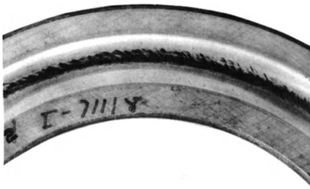
Figure 3-22: Smearing in ball thrust bearing.
