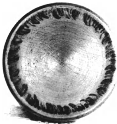
Figure 3-39: Smearing on spherical roller end.
