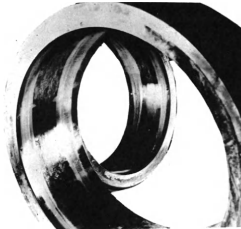
Figure 3-16: Mirror view of spherical roller-bearing outer ring pinched by housing.
