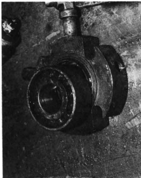
Figure 9-10: Double row (outboard) bearing and seal gland.
