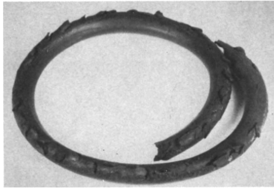
Figure 3-154: Chemical attack of O-rings.
