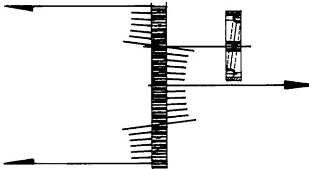
Figure 3-147: Developed plan of an angularly misaligned gear coupling half. 15
