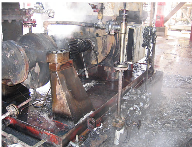
Figure 7-16: No. 2 fuel oil pump failure.
