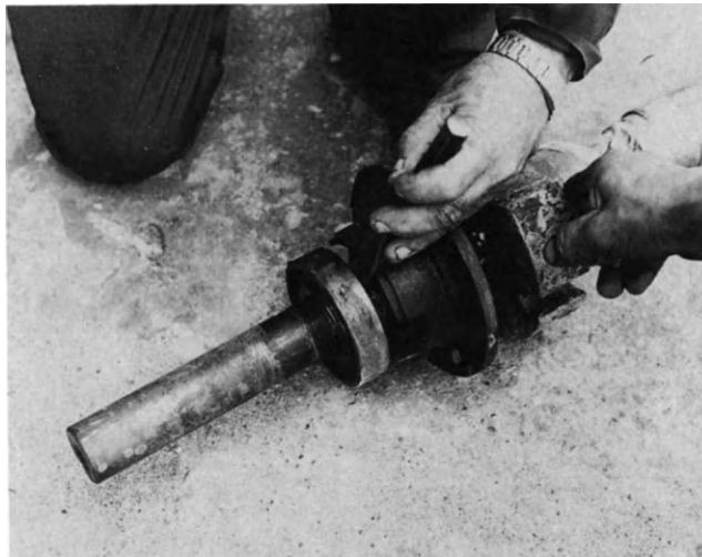
Figure 9-12: Careless disassembly of defective bearing.
