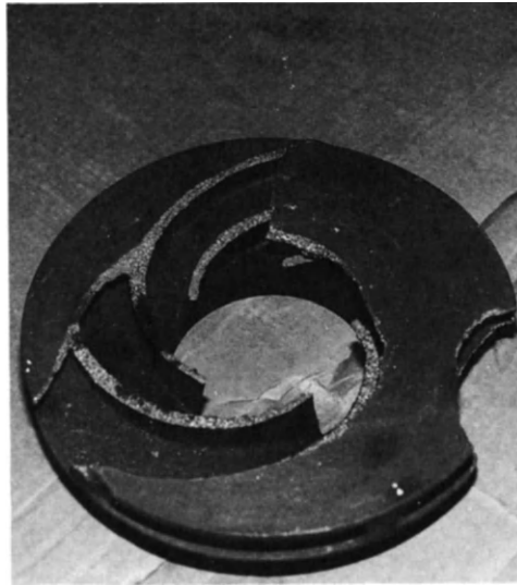
Figure 9-11: Impeller after careless disassembly.
