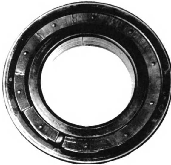
Figure 3-46: Broken cage caused by ineffective lubrication.
