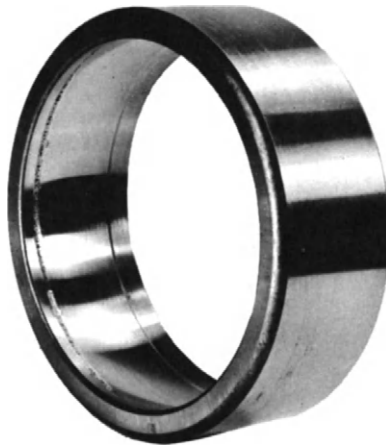
Figure 3-30: Spalling from parasitic thrust.
