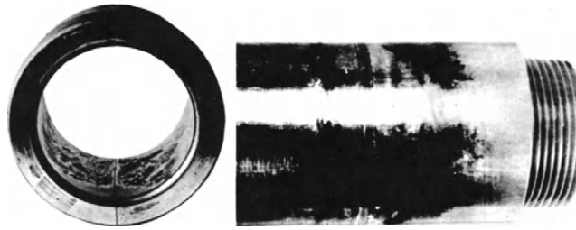
Figure 3-20: Fretting caused by yield in the shaft journal.
