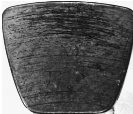
Figure 3-69: Dirt-intrusion damage at low-speed operation.
