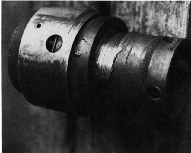
Figure 9-9: Mechanical seal surface indicating contact with stationary pump internals.
