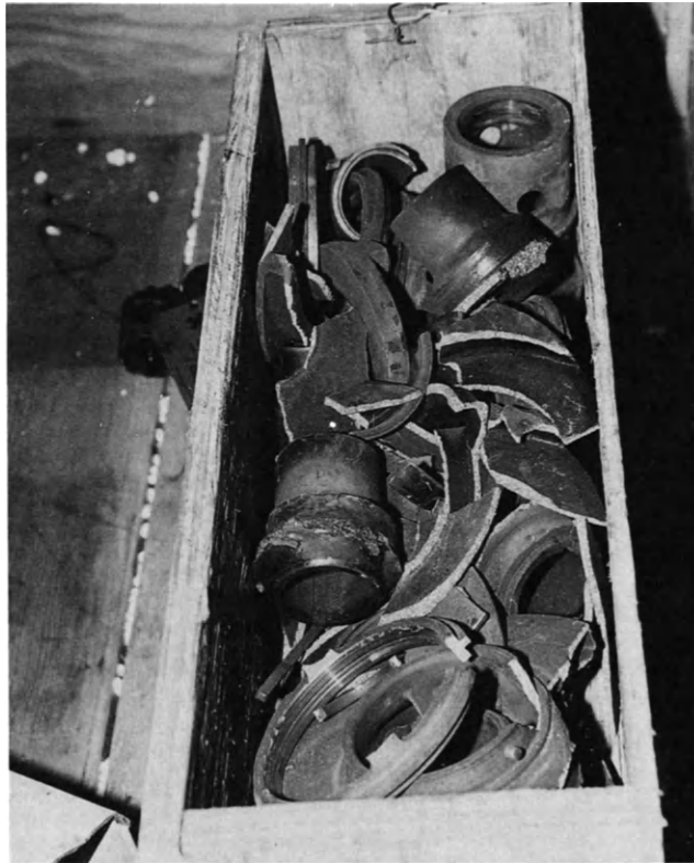
Figure 9-13: Impellers after careless removal from shaft.
