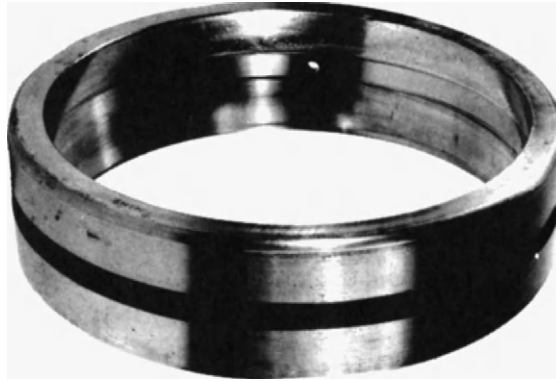
Figure 3-45: Grooves caused by wear due to inadequate lubrication.
