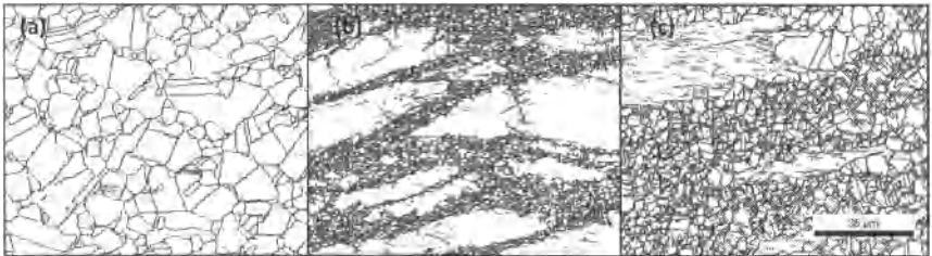
Figure 4. Microstructure after compression at \epsilon^*=0.65 : grain boundary map from EBSD for the following deformation conditions: 1100^{\circ}C at (a) 0.001s^{-1} , (b) 0.1s^{-1} and (c) 10s^{-1}
