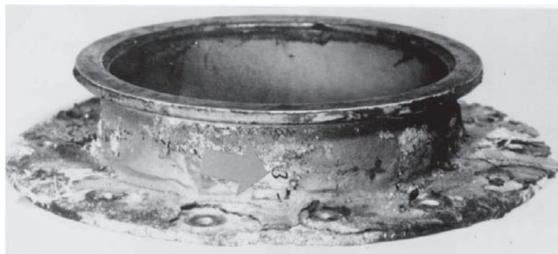
Fig. 27.1 Severely corroded magnesium part. Source: Ref 1
