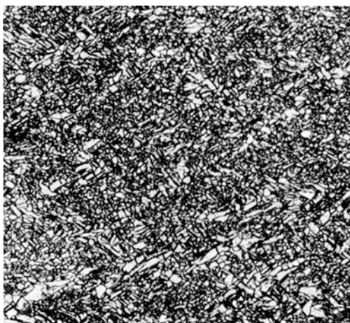
Fig. 27.11 Microstructure of warm-worked AZ31B-H24 sheet. Original magnification: 250×. Source: Ref 7
