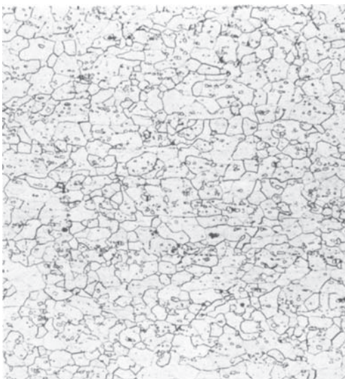
Fig. 23.3 Microstructure of annealed 446 stainless steel strip. Original magnification: 100 \times . Source: Ref 3
