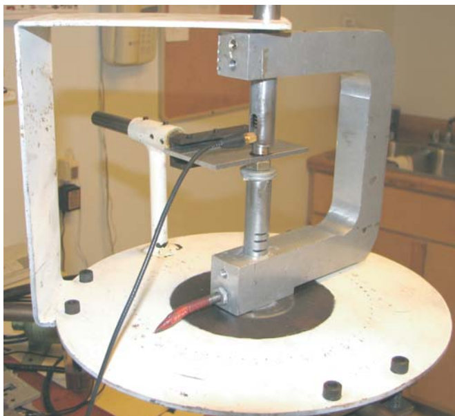
Figure 10.5 Shear wave probe set up for birefringence investigation. Courtesy of Don E. Bray, Inc.
