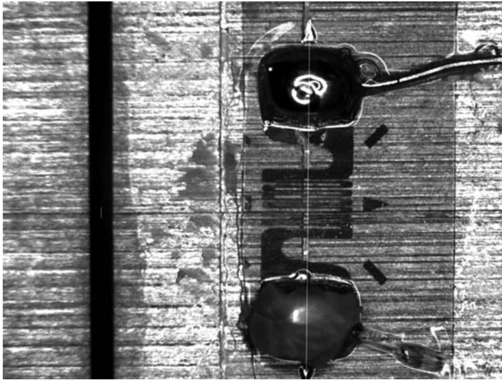
Figure 4.5 Post-experiment, microscopic image of a front face strain gage next to the EDM slit, after removal of waterproof coating. The gage grid length = 0.79 mm and slit width = 0.25 mm). Note the precision achieved by microscopic gage placement: the trimmed gage backing (darker area under the gage grid), masked gage-bonding adhesive (vertical line just left of the gage backing), and the masked waterproof coating (transition from shiny (coated) to dull (uncoated) surface just right of the slit). Copyright 2013, Hill Engineering, LLC
