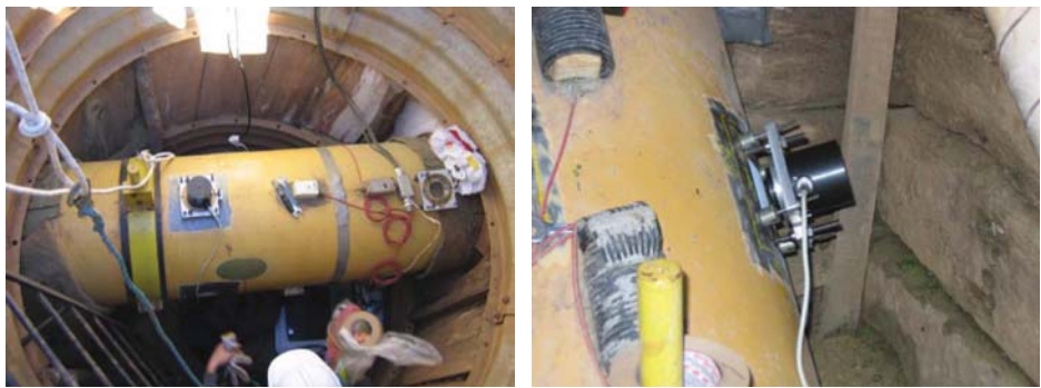
Figure 11.15 Hole drilling system being used to find stresses in a gas pipeline in service. Reproduced with permission from [43], Copyright 2009 SPIE
