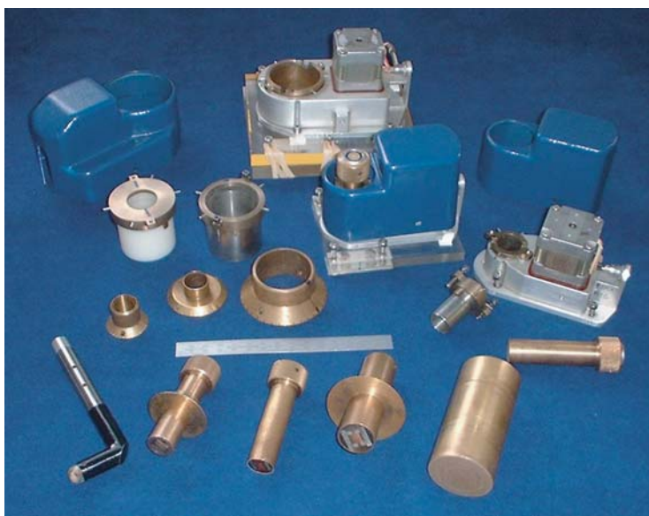
Figure 9.15 Examples of some MAPS probes (front) and motor units (back) and fittings. Reproduced with permission from [17]
