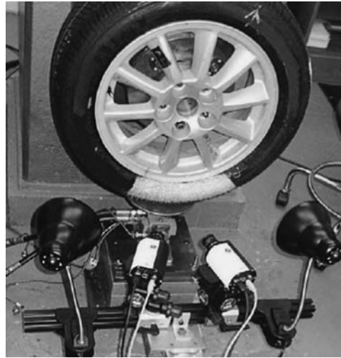
Figure 11.13 Digital image correlation set-up for measurement of tyre deformations showing two cameras and ordinary lamps. Reproduced with permission from [74], Copyright 2007 Wiley
