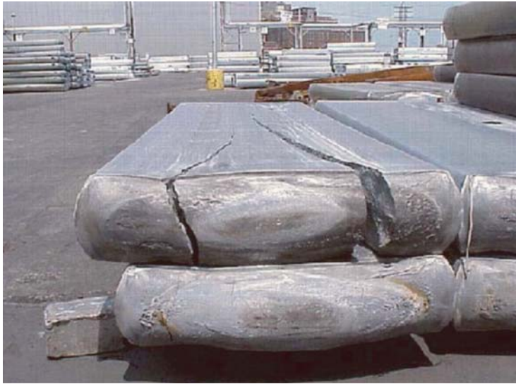
Figure 1.3 Cracking in a cast aluminum ingot due to excessive residual stresses. Courtesy of Alcoa Inc.
