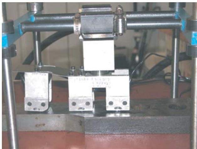
Figure 10.7 Dual receiver rotating probe arrangement under hydraulic pressure. Courtesy of Don E. Bray, Inc.
