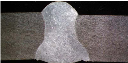
Fig. 21 Macrostructure of the LBW welded AA6061-T6.
