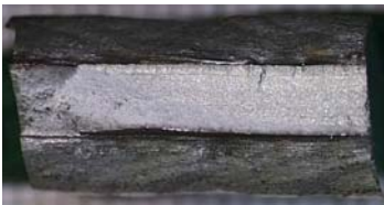
(b) AA6061-T6 MIG specimen with fracture surface
