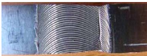
Fig. 2 Crack path of AA6082-T6 FS welded specimen.
