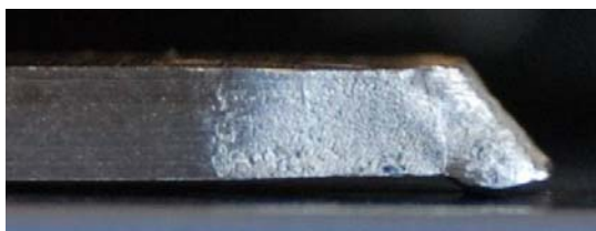
Fig. 3 LB weld crack orientation.
