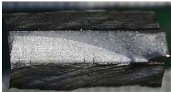
(a) AA6082-T6 MIG specimen with fracture surface
