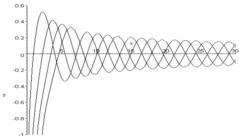
The Bessel functions  $Y_0, Y_1, Y_2, Y_3$ , identified in this order by the ordering, from left to right, of the first peak on each curve.
