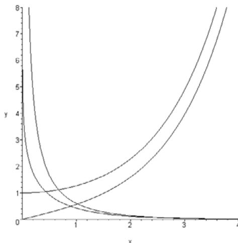
The modified Bessel functions  $K_0, K_1, I_0, I_1$ , identified in this order by the ordering,
