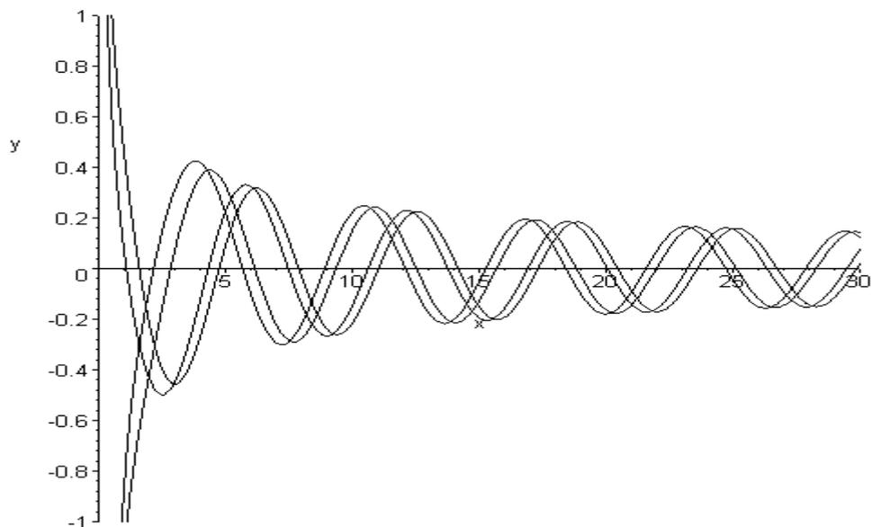
The Bessel functions  $J_{-7/4}, J_{-3/2}, J_{-3/4}, J_{-1/2}$ , identified in this order by the ordering, from left to right, of the first peak (ignoring the asymptote along the  $y$ -axis) on each curve.
