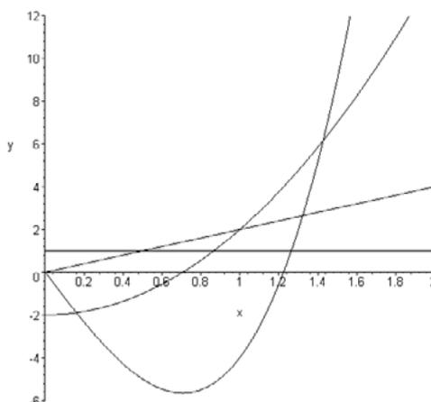
The Hermite polynomials,  $H_0, H_1, H_2, H_3$ , identified in this order by
