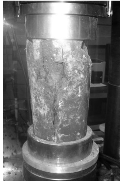
FIGURE A.41 Example of fracture with vertical cracks.
