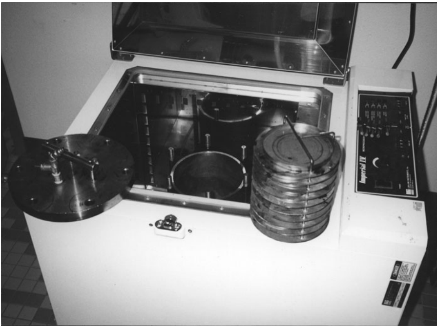
FIGURE 9.17 Pressure-aging vessel apparatus.
