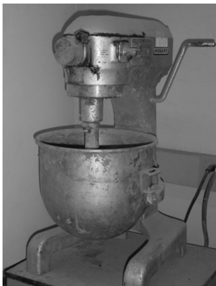
FIGURE A.57 Mixing HMA using a mechanical mixer.
