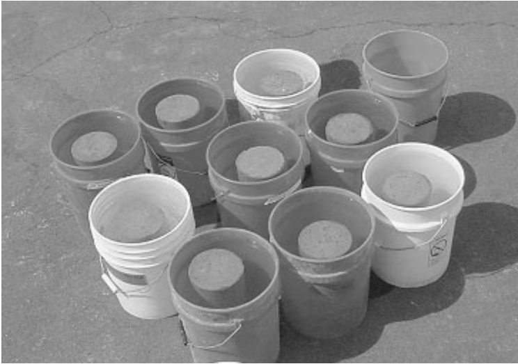
FIGURE A . 3 6 Curing concrete cylinders in lime-saturated water.
