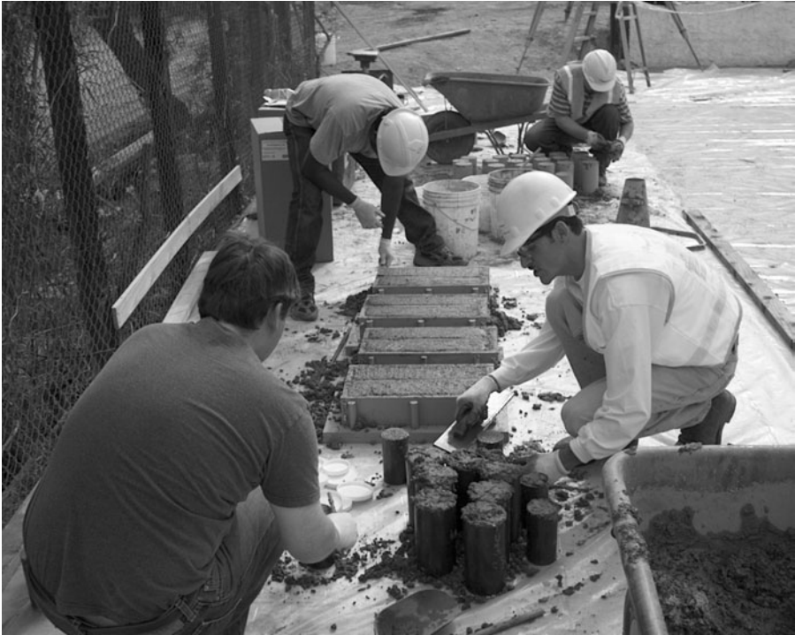
FIGURE A.33 Making concrete cylinders and beams.
