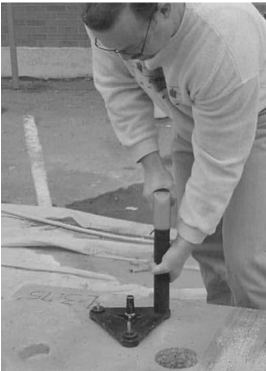
FIGURE A . 45 Firing and driving Windsor probe into concrete using triangular positioning device.
