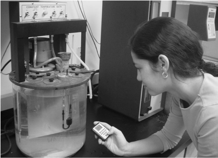
FIGURE A.53 Measuring flow time using a stop watch.
