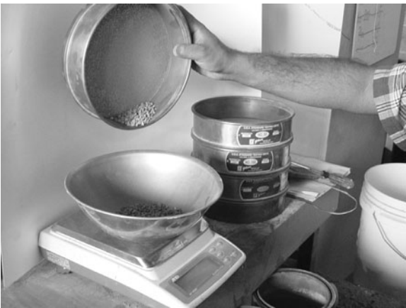
FIGURE A.20 Weighing aggregate retained in sieves.
