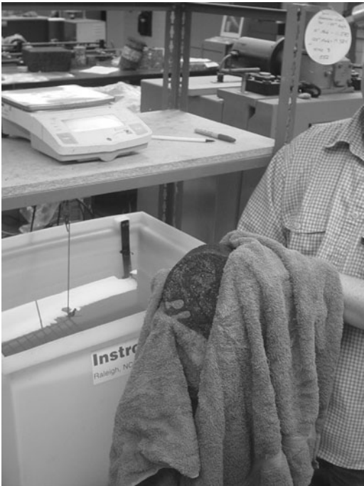
FIGURE A.63 Drying HMA specimen with a damp towel.
