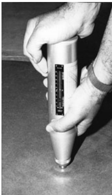
FIGURE 7.37 Rebound hammer for nondestructive evaluation of hardened concrete.
