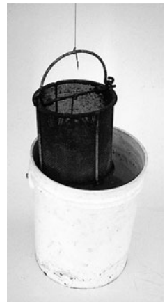
FIGURE A.23 Wire basket and water tank used to determine bulk specific gravity and absorption of coarse aggregate.
