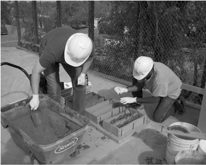
FIGURE A.34 Filling and rodding concrete in beams.
