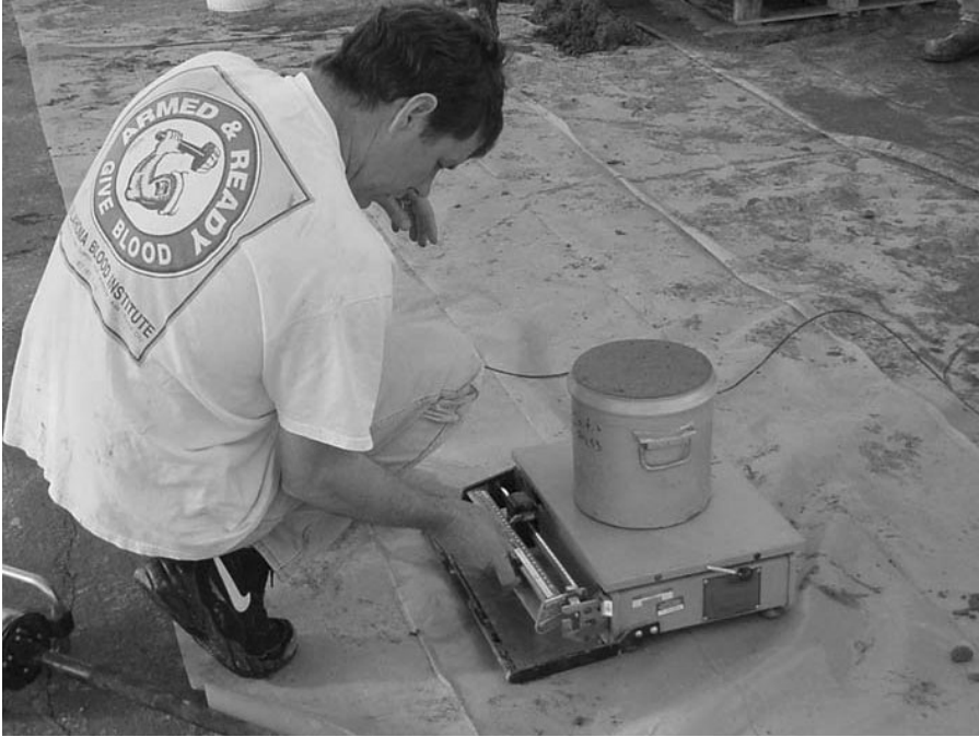
FIGURE A.30 Weighing concrete inside the container.
