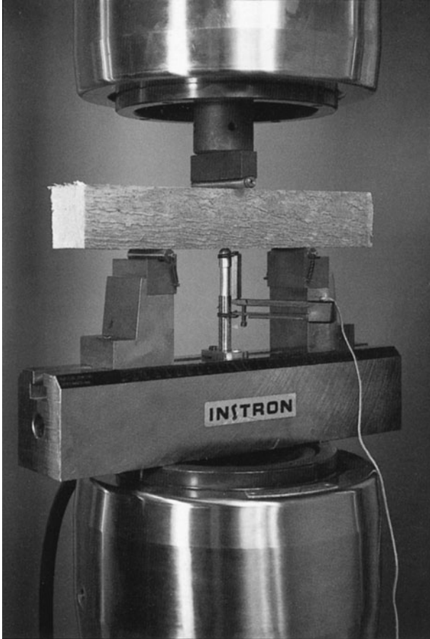
FIGURE A.68 Wood specimen during static bending test. (Courtesy of Instron®)
