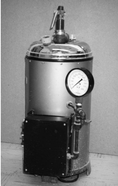
FIGURE 6.7 Cement autoclave expansion apparatus.
