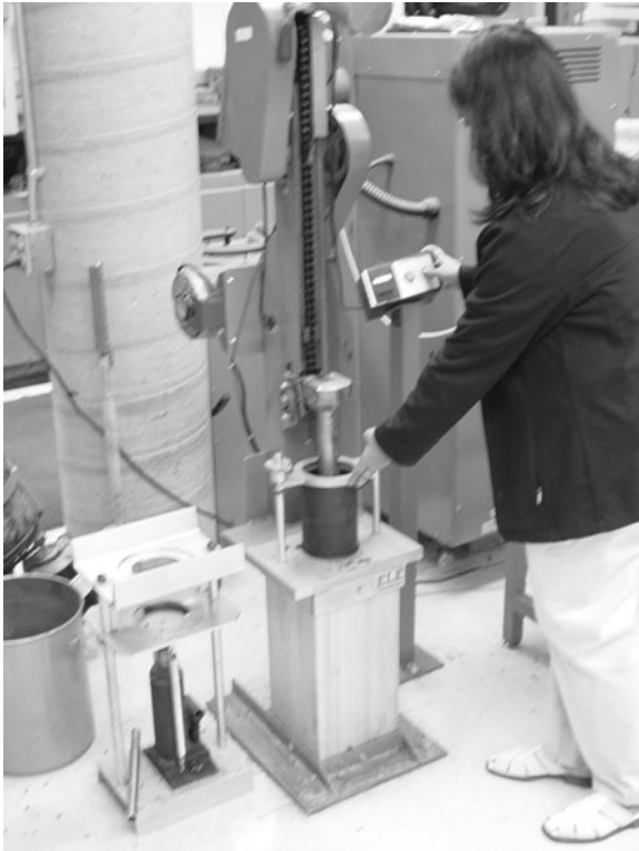
FIGURE A.59 Compacting an HMA specimen using a mechanical Marshall hammer.
