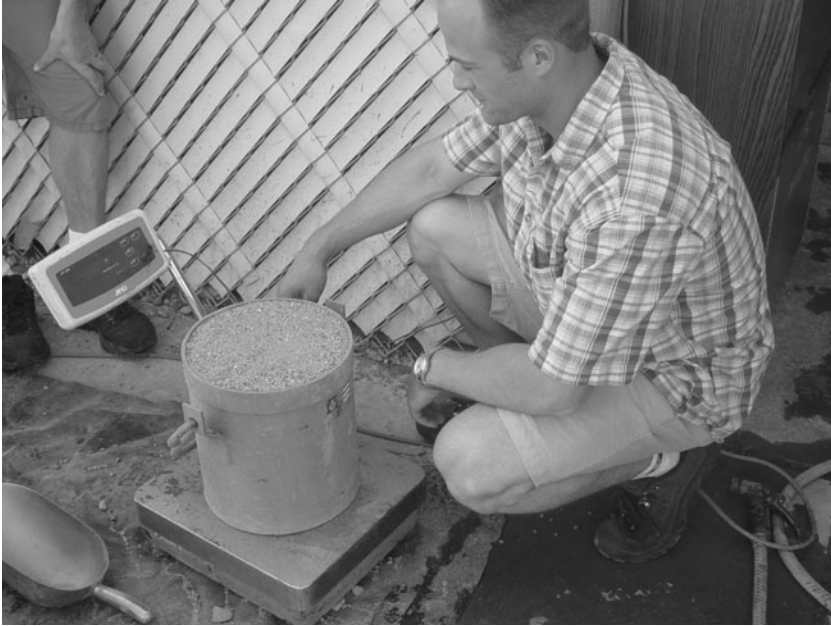
FIGURE A.26 Weighing the aggregate.
