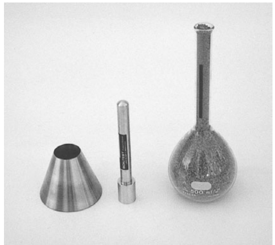
FIGURE A.24 Mold, tamper, and volumetric flask used to determine bulk specific gravity and absorption of fine aggregate.
