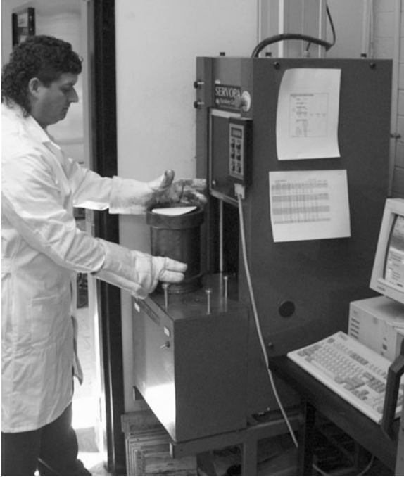
FIGURE A.55 Placing the mold in the gyratory compactor.
