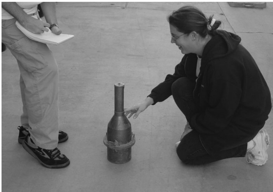
FIGURE A.32 Reading air meter.
