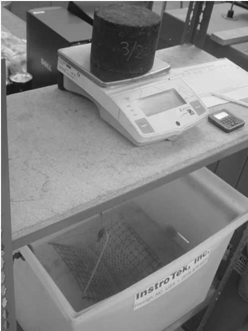
FIGURE A.61 Weighing HMA specimen in air.
