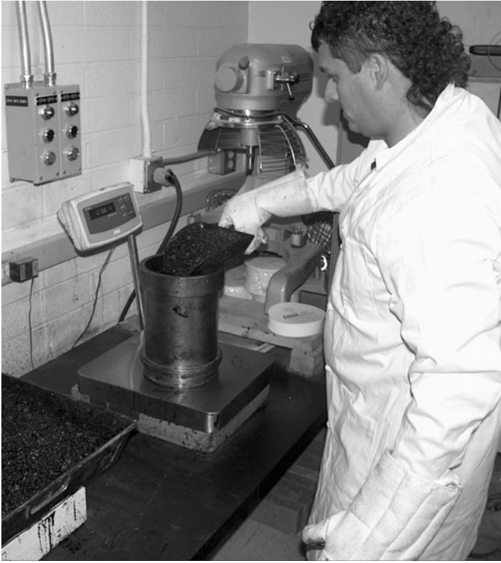
FIGURE A.54 Placing HMA in mold.
