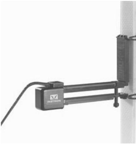
FIGURE A.71 Extensometer on plastic specimen. (Courtesy of Instron®)
