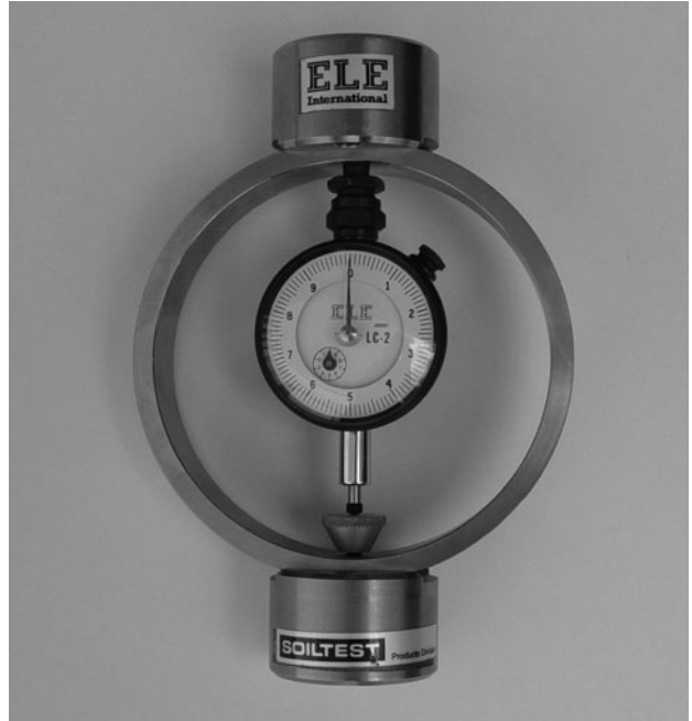
FIGURE 1.34 Proving ring. (Courtesy of Humboldt Mfg. Co.)
