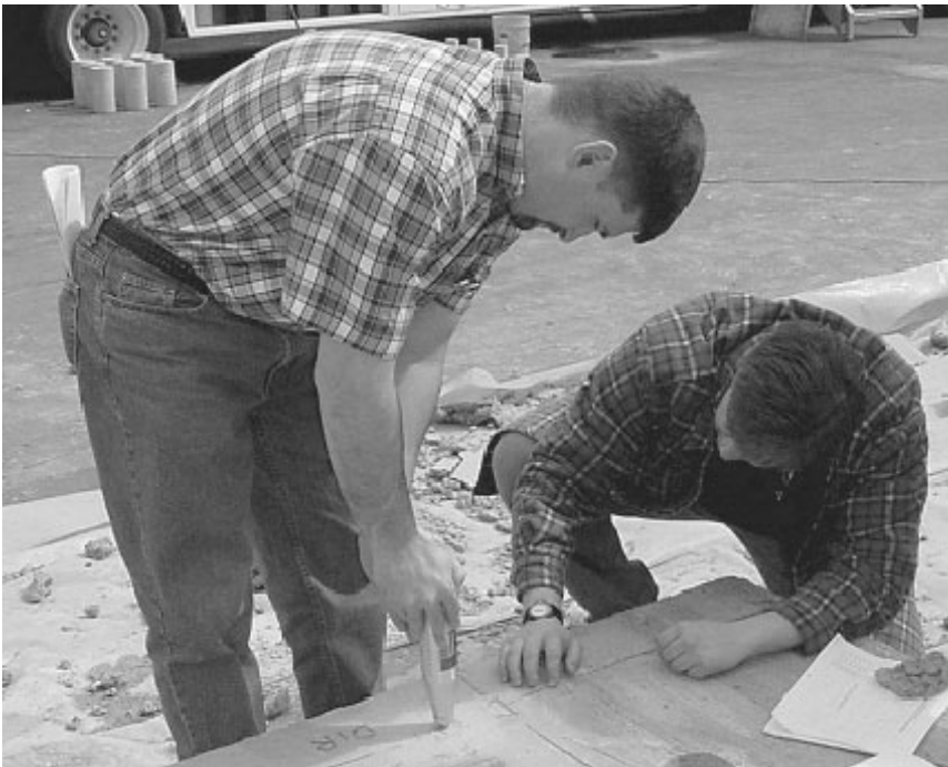
FIGURE A.43 Testing concrete slab with a rebound hammer.
