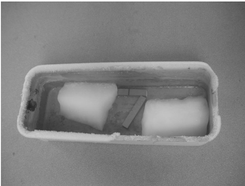
FIGURE A.13 Charpy specimens in dry ice and isopropyl alcohol.
