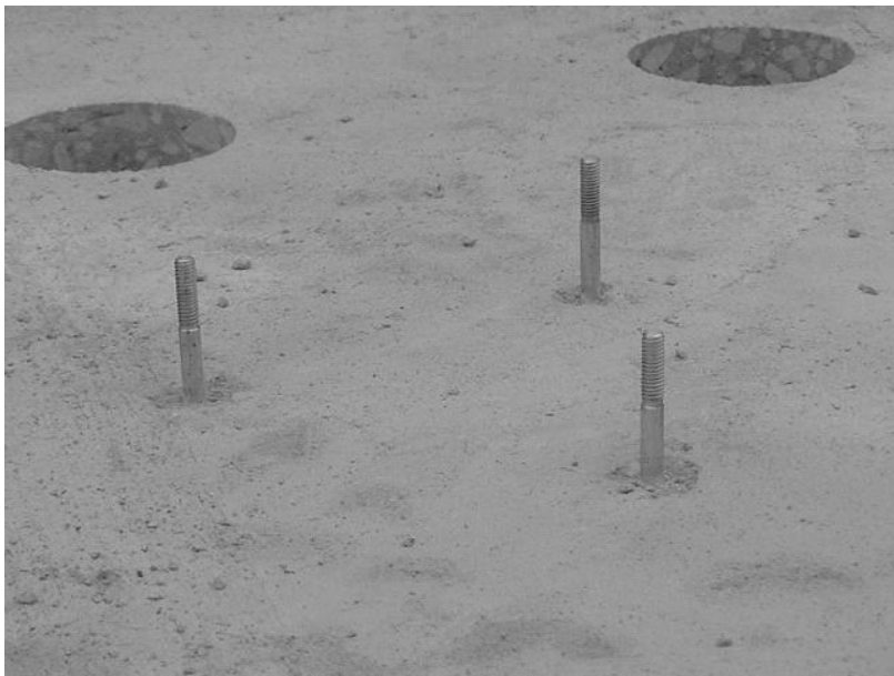
FIGURE A . 46 Three probes driven into concrete.
