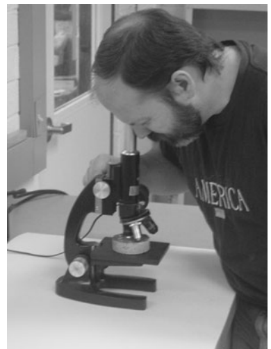
FIGURE A.16 Viewing concrete specimen with an optical microscope.
