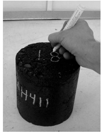
FIGURE A.56 Specimen prepared with gyratory shear compactor.
