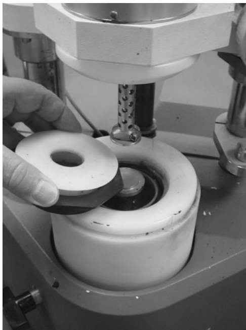
FIGURE A.51 Water bath for controlling specimen temperature during testing.
