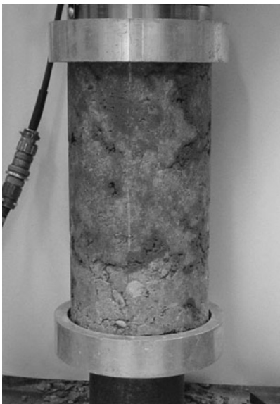
FIGURE A.39 Neoprene caps used for capping a concrete cylinder.
