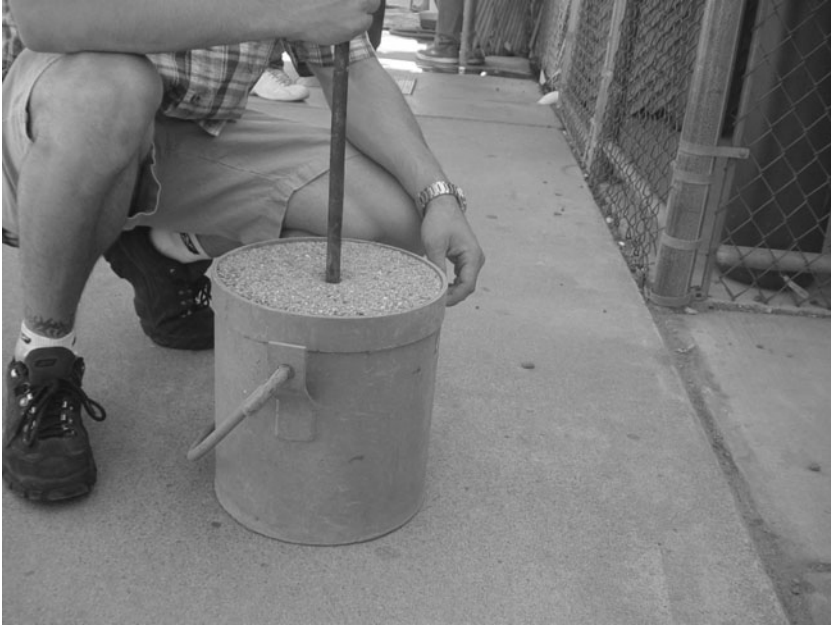
FIGURE A.25 Rodding aggregate in the container.
