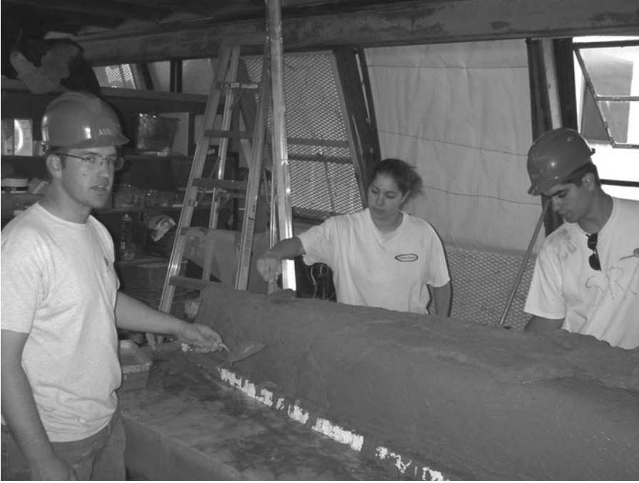
FIGURE 7.47 ASCE students at Arizona State University making a concrete canoe using lightweight concrete.
