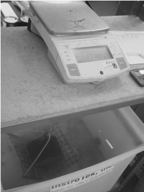
FIGURE A.62 Weighing HMA specimen in water.
