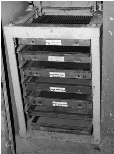
FIGURE 5.12 Sieve shaker for large samples of aggregates.
