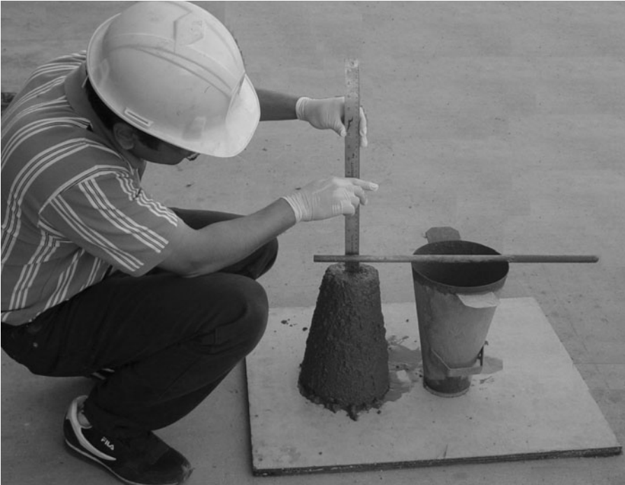
FIGURE A.29 Measuring the slump of freshly mixed concrete.
