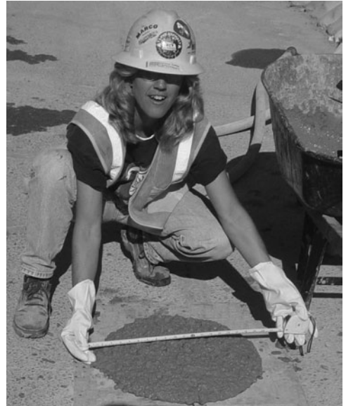
FIGURE 7.42 Measuring the spread during the slump flow test.
