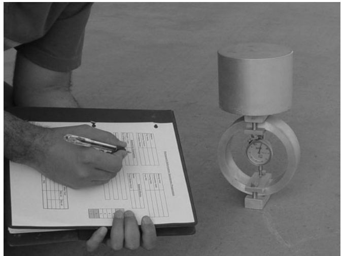
FIGURE A.3 Calibrating a proving ring using a known-weight object.
