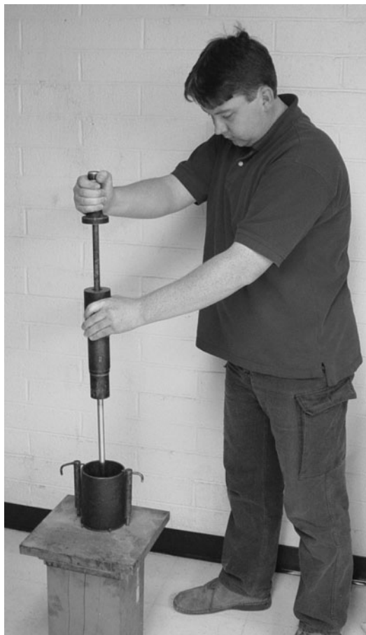
FIGURE A.58 Compacting an HMA specimen using a manual Marshall hammer.
