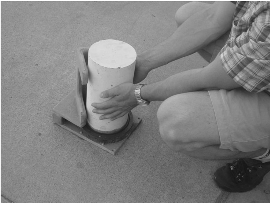
FIGURE A.37 Capping a concrete cylinder using an alignment device.
