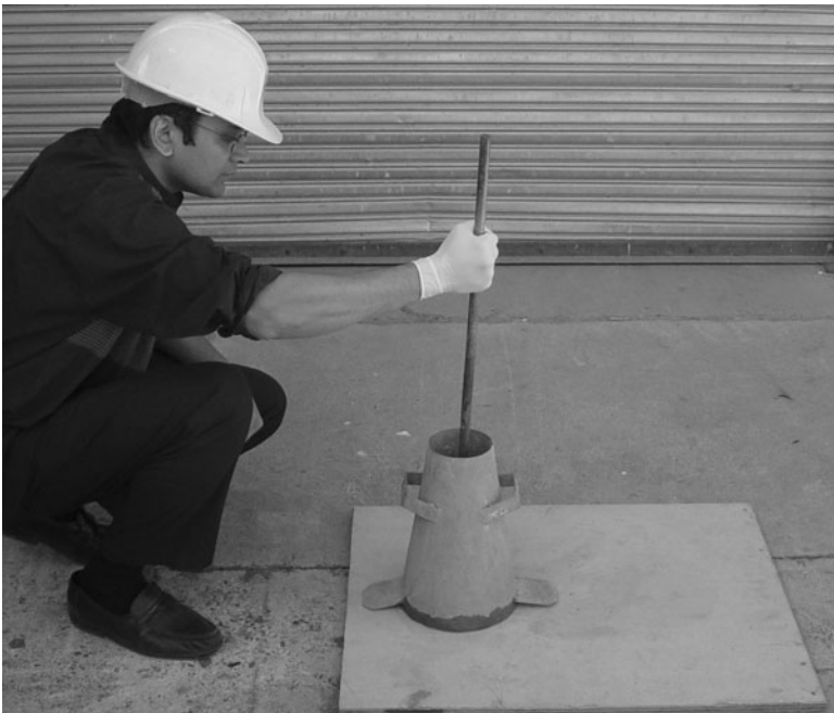
FIGURE A.28 Rodding fresh concrete in the slump cone with a tamping rod.
