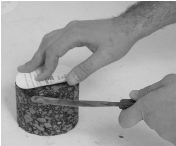
FIGURE A.60 Removing paper disk from a Marshall plug.
