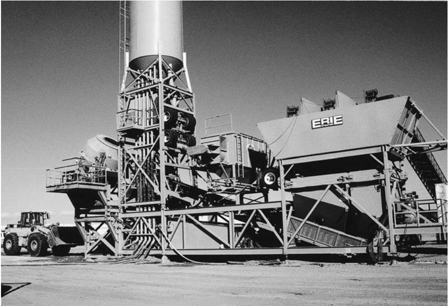
FIGURE 7.5 Mobile batcher mixer at the job site.
