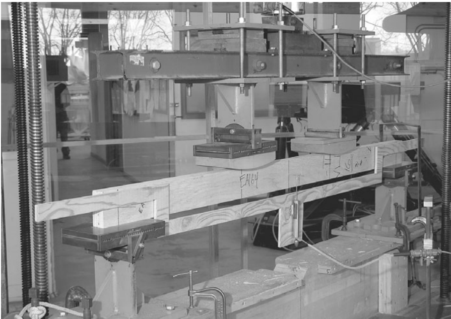
FIGURE 10.16 Two-point loading flexure test on a glulam structural member.
