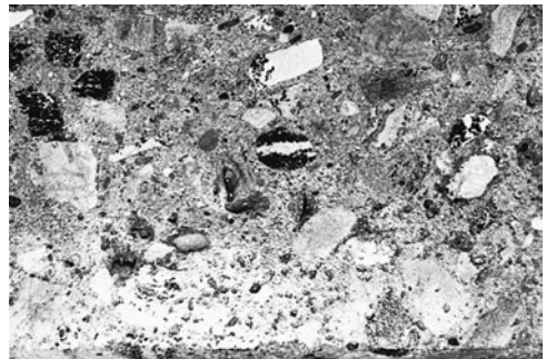
FIGURE 11.12 Cross section of portland cement concrete showing cement paste and aggregate particles.
