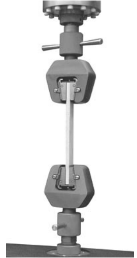
FIGURE A.72 Tension test on a plastic specimen.
