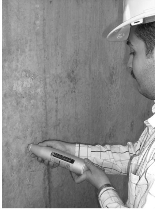
FIGURE A.44 Testing concrete wall with a rebound hammer.
