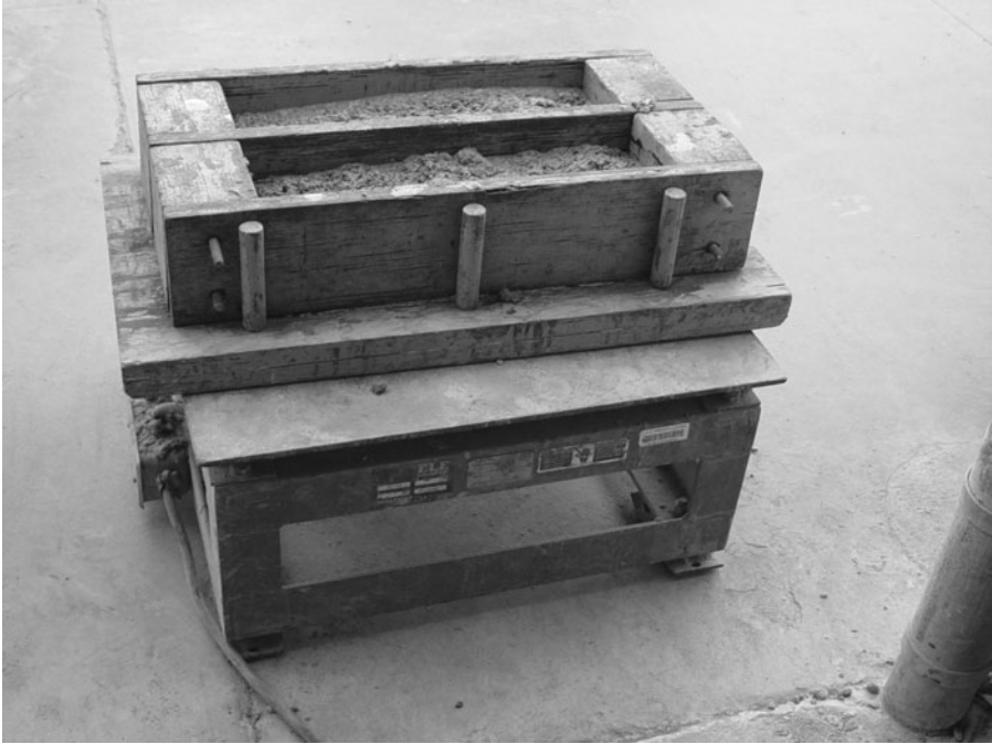
FIGURE A.35 Consolidating concrete in a beam mold using an external vibrator.
