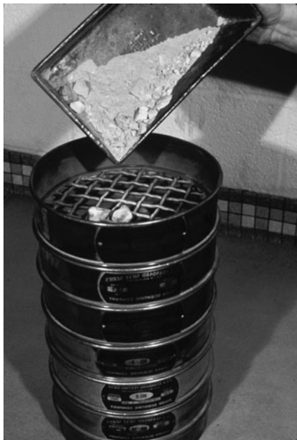
FIGURE A.19 Placing aggregate sample in the sieves before sieving.
