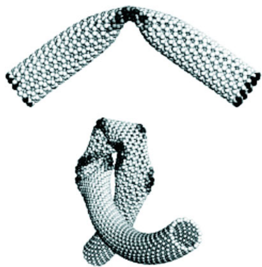
Figure 6.68. Illustration of the deformation modes of SWNTs, resulting in a high elasticity. This behavior is likely an artifact of in-plane flexibility of a graphene sheet, and facile rehybridization of carbon atoms from sp^2 to sp^3 geometries. Reproduced with permission from Ajayan, P. M. Chem. Rev. 1999 , 99, 1787. Copyright 1999 American Chemical Society.
