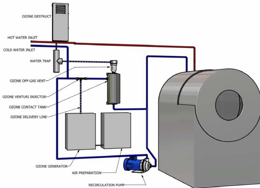
**Figure 6.** Schematic diagram of Pressurized Ozone Charge System.
