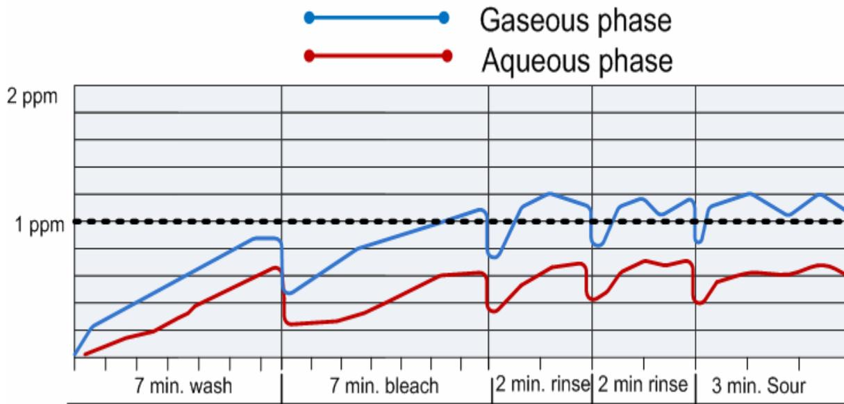
**Figure 9.** Ozone in aqueous and gaseous phases in an Ozone Diffusion washer. Ozone in gas phase controlled by means of an Aquawing ozone monitor/controller (graphic courtesy of Dave Spofford, AWOIS LLC, Auburn, NH, USA).
