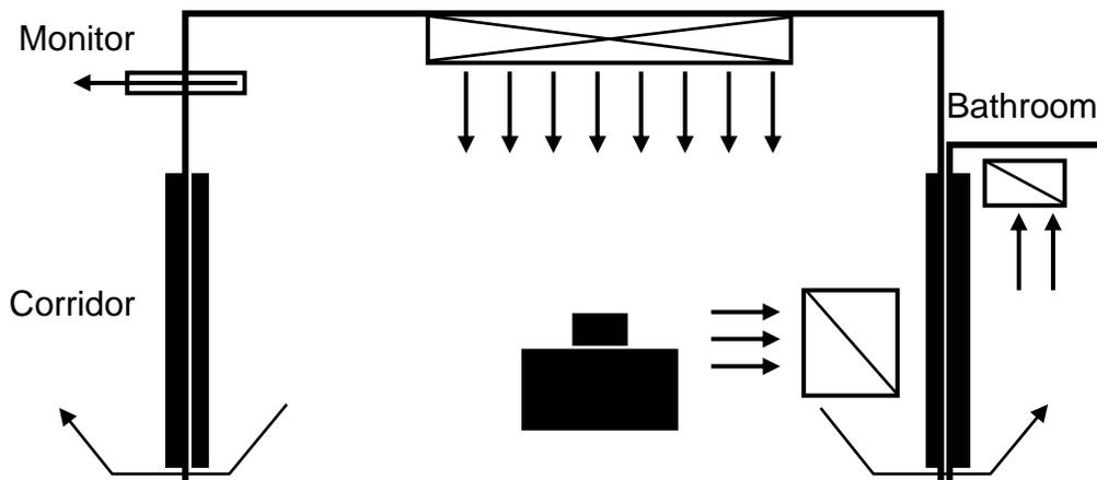
\* Stacked black boxes represent patient's bed. Long open box with cross-hatch represents supply air. Open boxes with single, diagonal slashes represent air exhaust registers. Arrows indicate directions of air flow.
