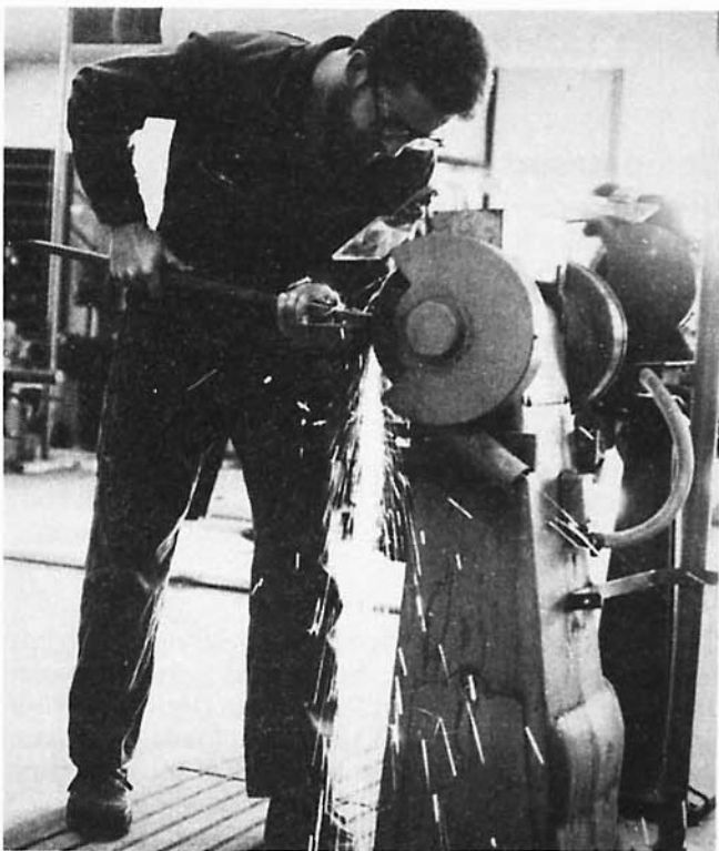
Figure 5 Safety when grinding (Note the eye protection and the safety shield around the wheel)
