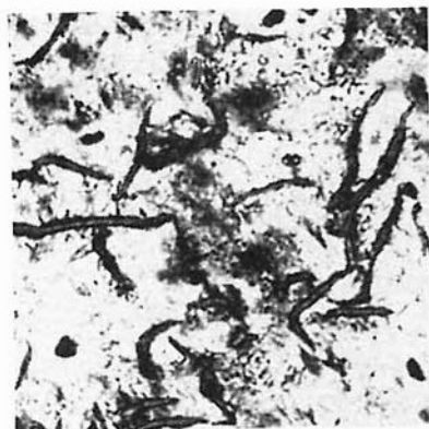
Figure 1 Microstructure of ferritic pearlite (grey cast iron)
