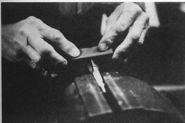
Figure 9 Using an oilstone to sharpen a tap
