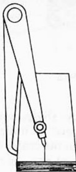
Figure 8 Scribing a line parallel to an outside edge
