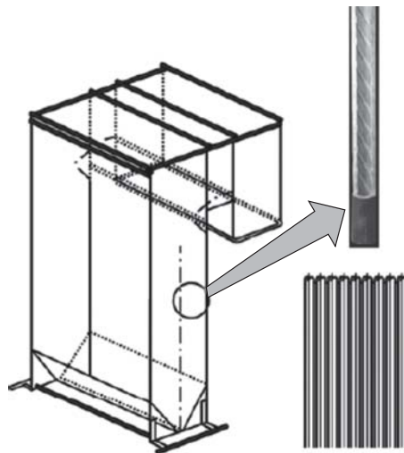
Figure 4-5. Structure of vertical water-wall furnace with rifled tubes. (From [5], © IEEE 2001.)
