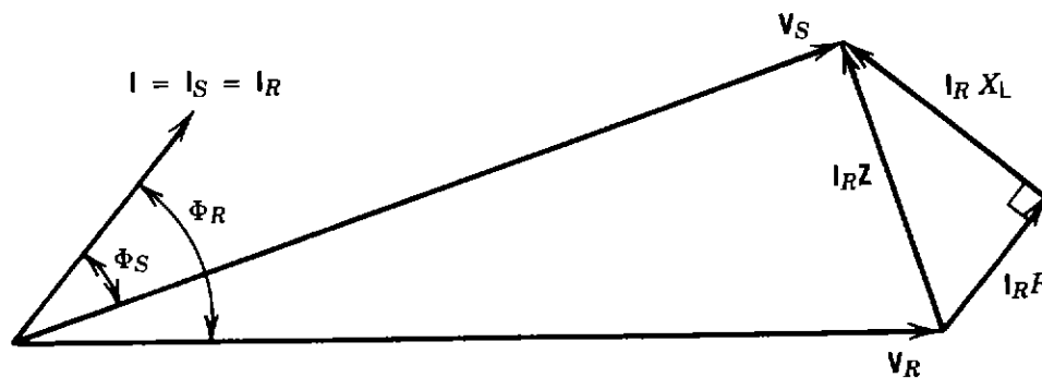
Figure 2.25. Phasor diagram of short transmission line connected to capacitive load.
