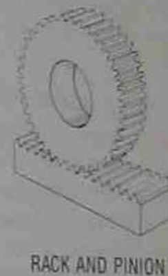
Fig. 7-49 Spur gears.
