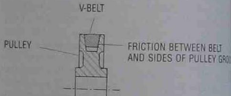
Fig. 7-2 V-belt in pulley.
