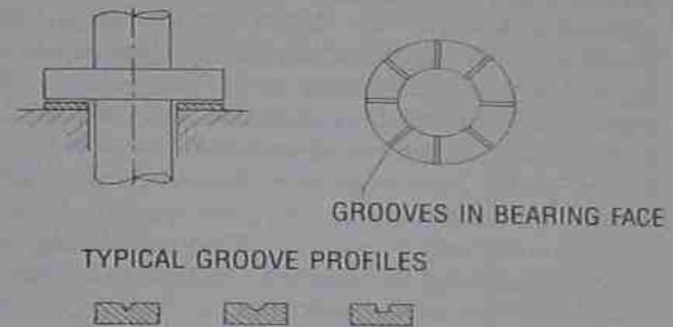
Fig. 6-7 Plain thrust bearing.
