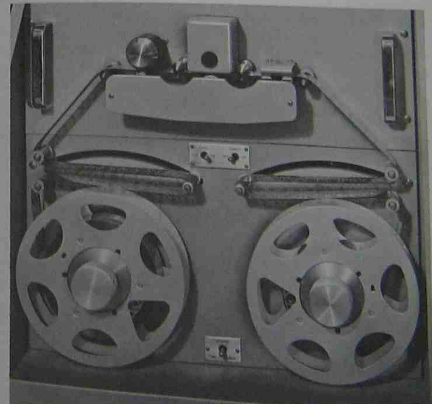
Fig. 3-2. The reels shown above, for a hardwire control system, handle the punched tape as it passes through the photoelectric tape reader. A special code punched at the end of the tape run actuates a signal that automatically stops the operation and rewinds the tape.
