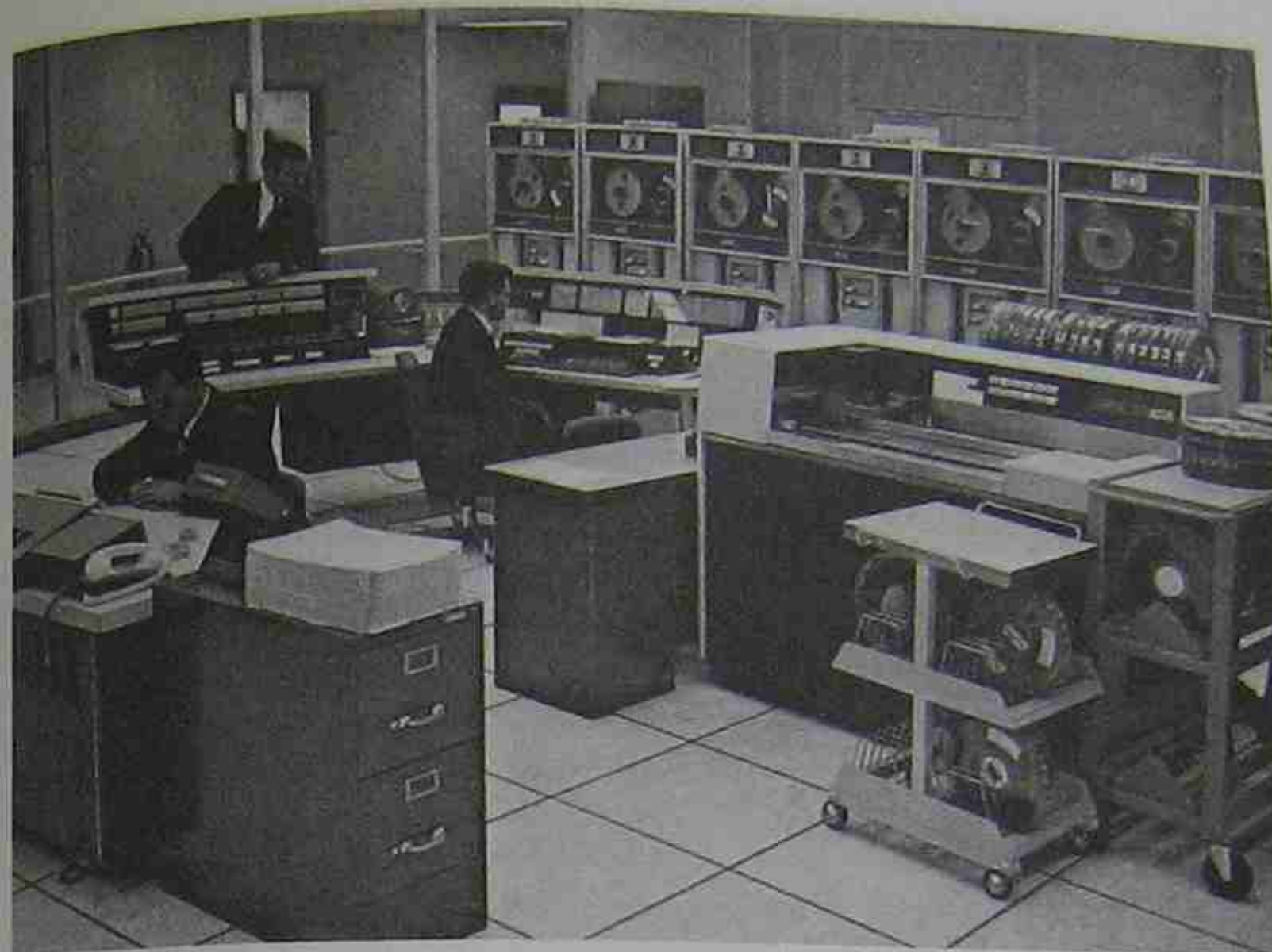
Fig. 5-2. This large scale computer, which is used quite frequently for numerical control calculations, is capable of performing several million calculations per second.
