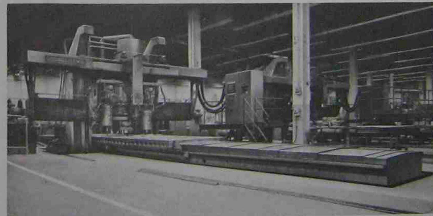
Fig. 1-3. The large numerically controlled skin milling machine shown here is capable of machining two parts simultaneously. This machine was part of the original 35-million dollar numerical control machine tool procurement program initiated in 1955 by the U.S. Air Force.
