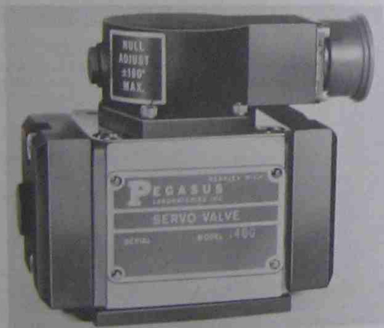
Fig. 2-20. This hydraulic servo valve regulates the amount of fluid to be passed to the hydraulic motor. This regulation depends on the distance to be moved and the velocity as called for on the punched tape. This unit measures about four inches across.
