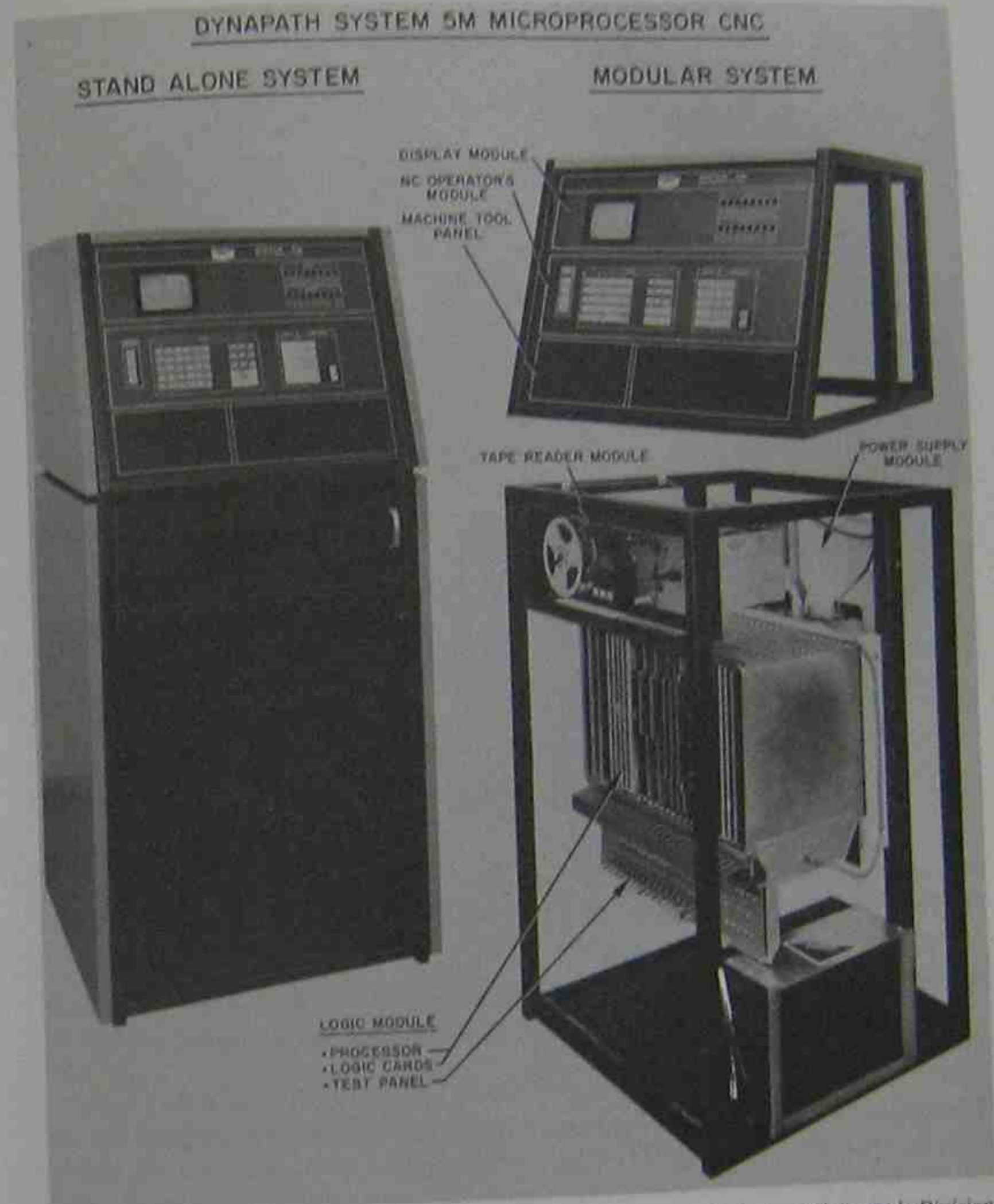
Fig. 2-5. The CNC system shown consists of several compact microcomputers together with the other requirements of a control system. This particular system may be procured as a stand-alone unit or in modules for installation as an integral part of a machine tool.
