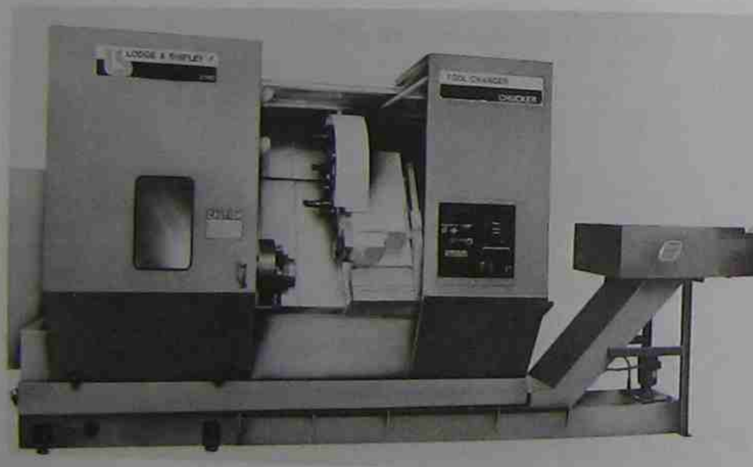
FIGURE 13-3 A modern CNC turning center employing automatic tool change (Photo courtesy of Lodge and Shipley Co.)
