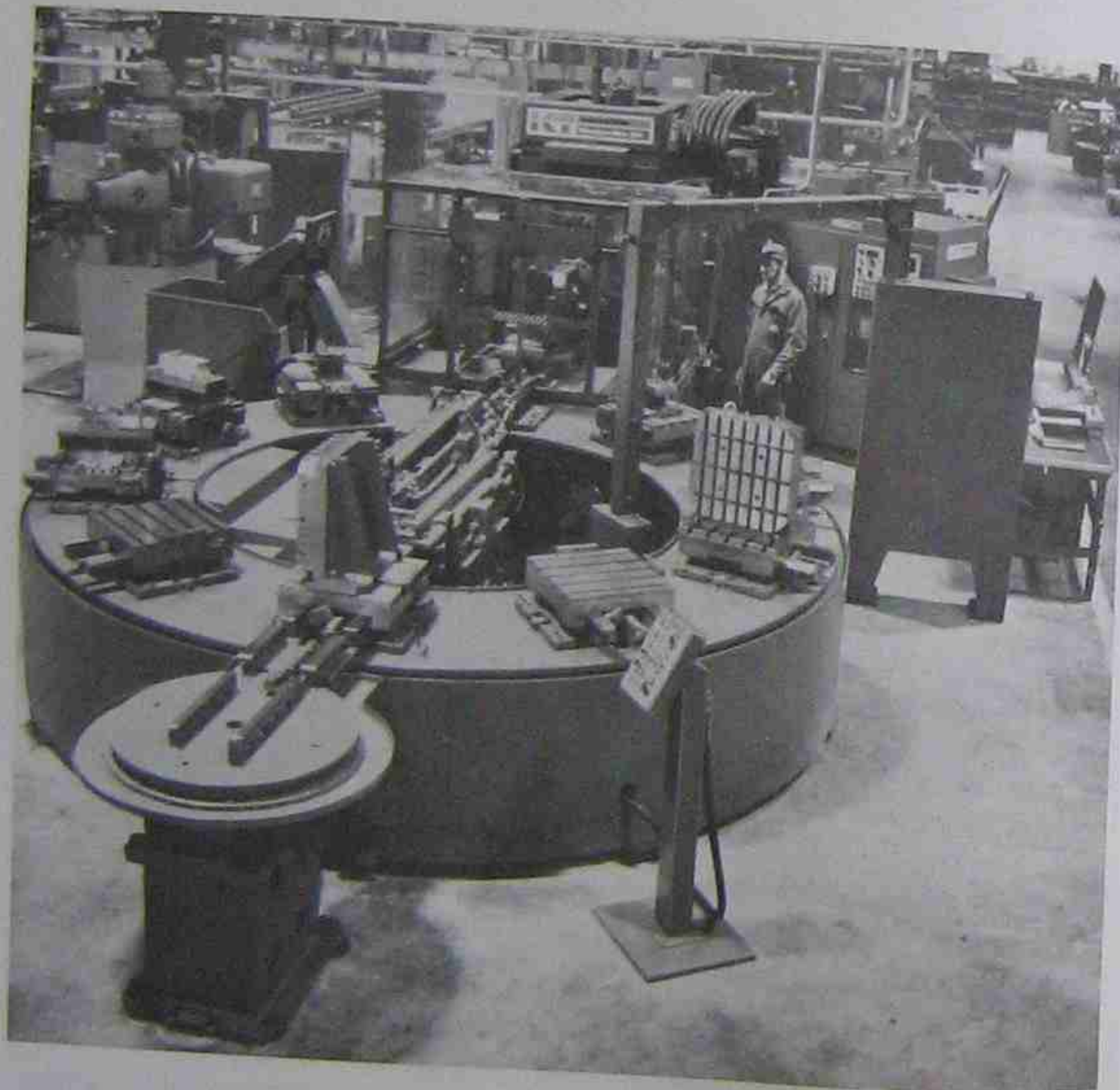
Fig. 9-11. Shown is a multiple pallet changer which automatically feeds a variety of parts to a numerical control machining center.
