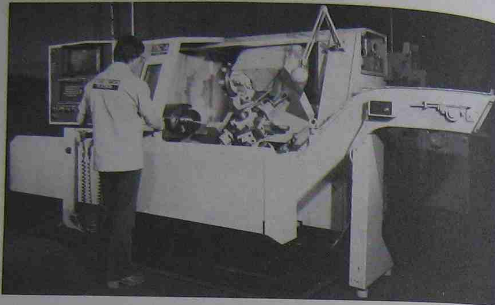
Fig. 2-2. The operator's panel and the control system are incorporated in the headstock of the lathe shown (just to the left of the operator).
