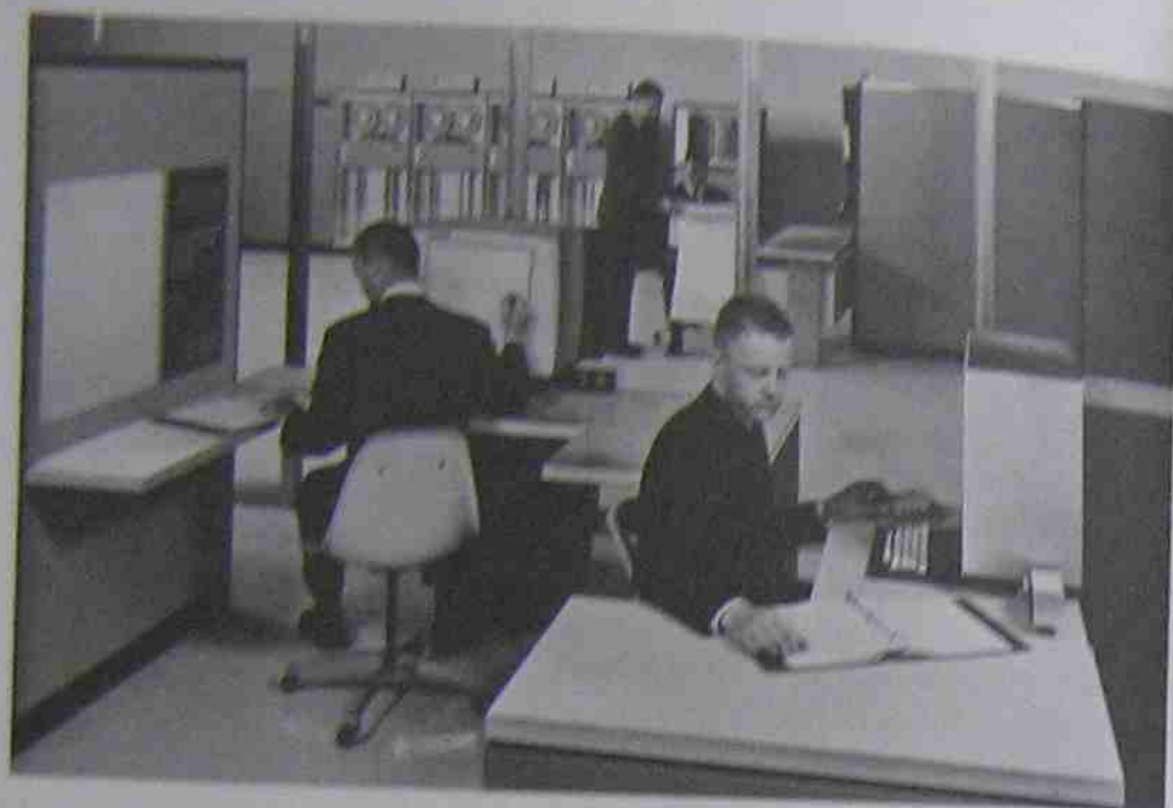
Fig. 9-1. Designs and graphical illustrations are "drawn" on the face of the cathode ray tube (CRT) shown in front of the operator on the left. As the operator draws the figure it is stored in the computer. This CRT-computer arrangement permits the operator to "call up" various predesigned and stored computations and figures. It also allows him to rotate the figures shown on the CRT in order to permit viewing at different angles.
