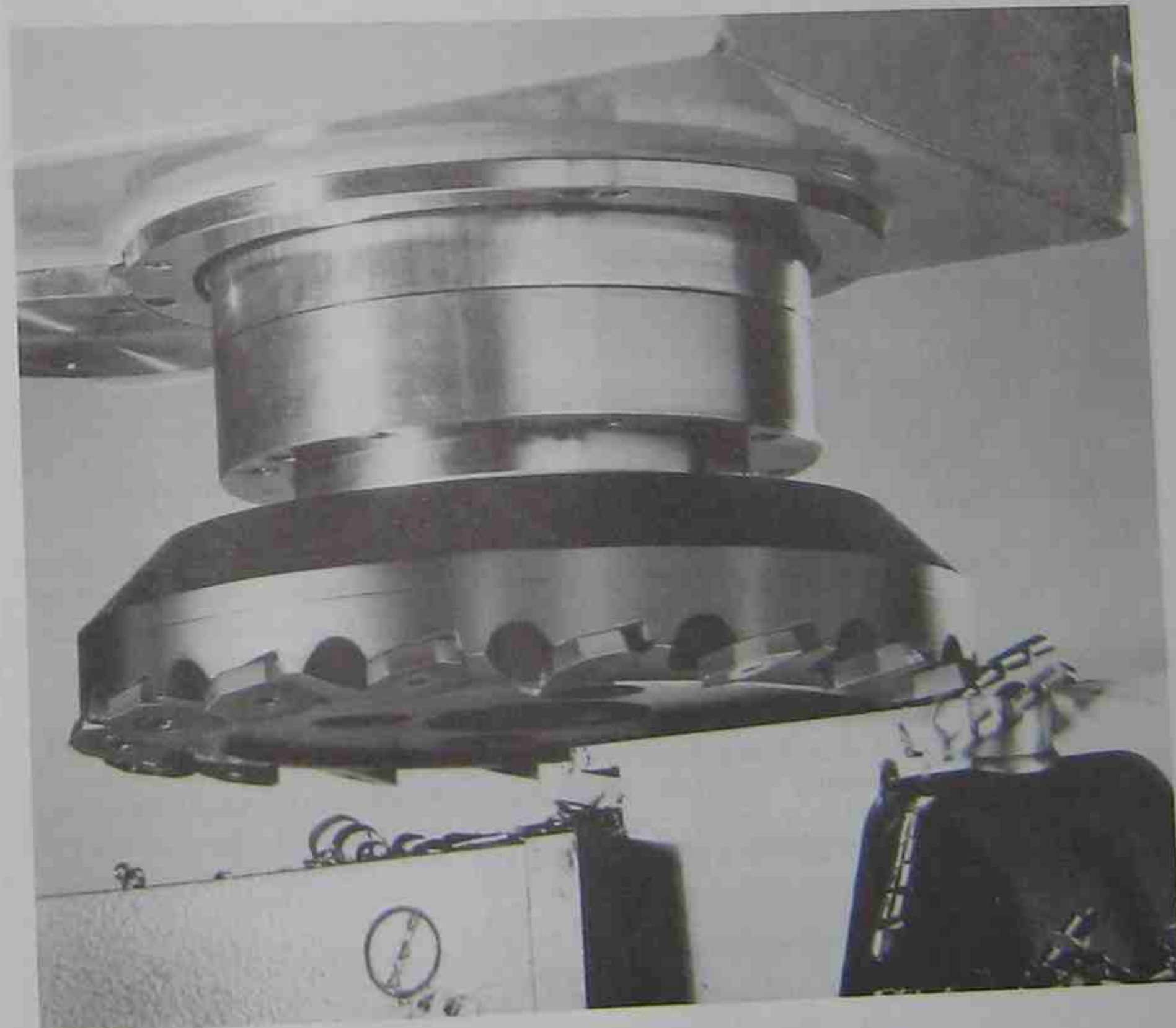
FIGURE 3-20 Large inserted face mill—note number of inserts on cutter (Photo courtesy of GTE Valenite)
