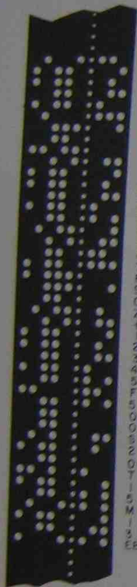
Fig. 3-7. The block of tape instructions shown above would cause the part to move to the absolute coordinate positions of X = 1.2345'' , Y = 6.7890'' , and Z = 1.2345'' at a feedrate of 5 ipm. At the same time the spindle is automatically adjusted to a speed
