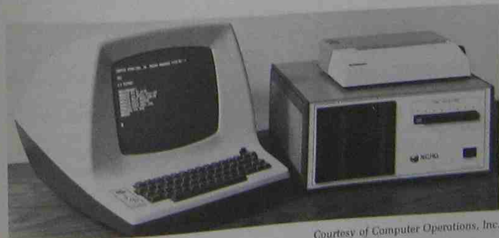
Fig. 9-16. Shown above is a relatively low cost Distributed Numerical Control arrangement, which also has part program editing capabilities and a hard-copy printer. The unit on the right accepts floppy discs, on which part programs are stored and from which the part programs can be directed to any one of eight NC machines.
