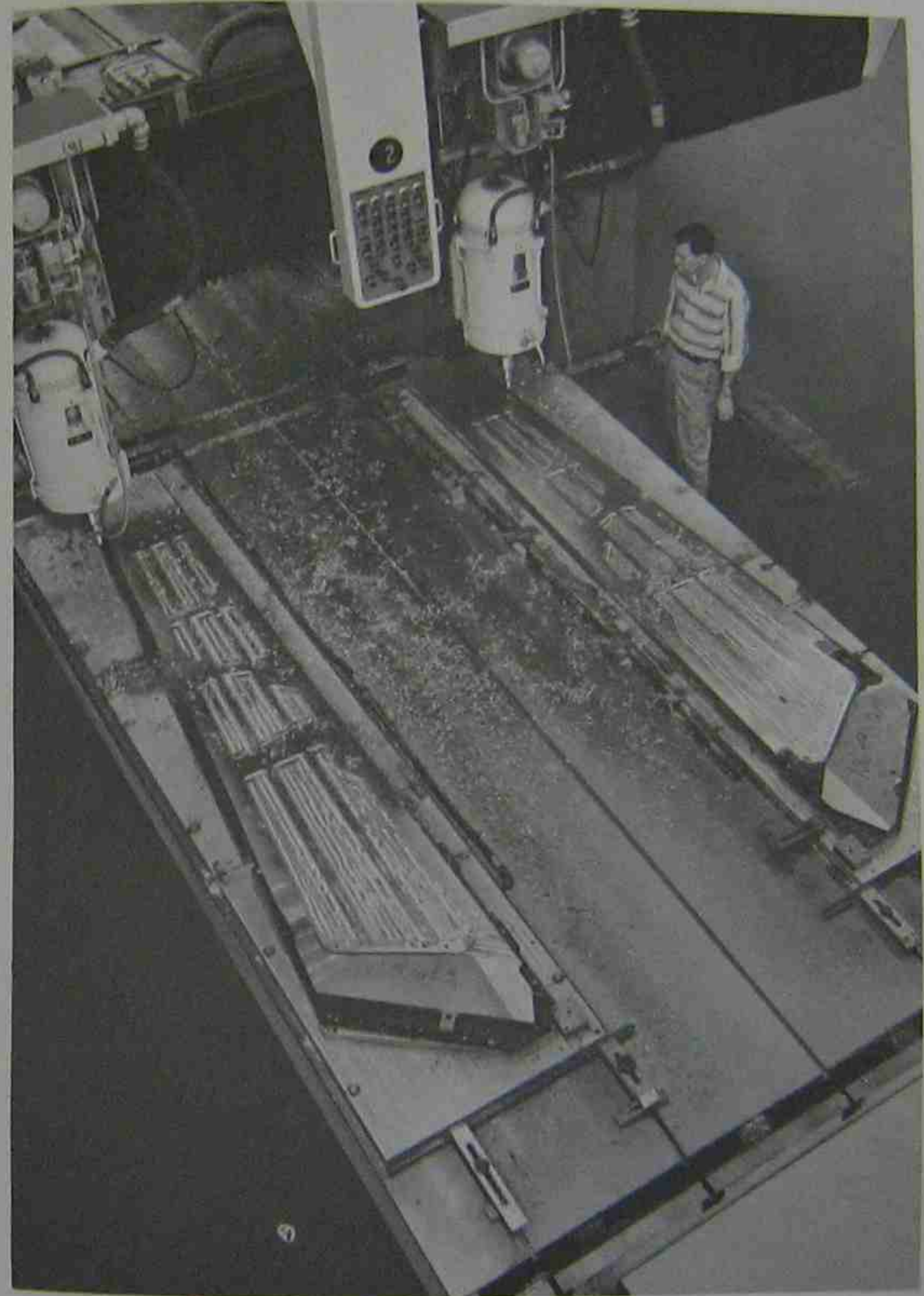
Fig. 1-21. The two large airframe structures shown are being machined simultaneously on a large, continuous-path skin milling machine. The parts are for use on the wing panels of an Air Force supersonic jet fighter.
