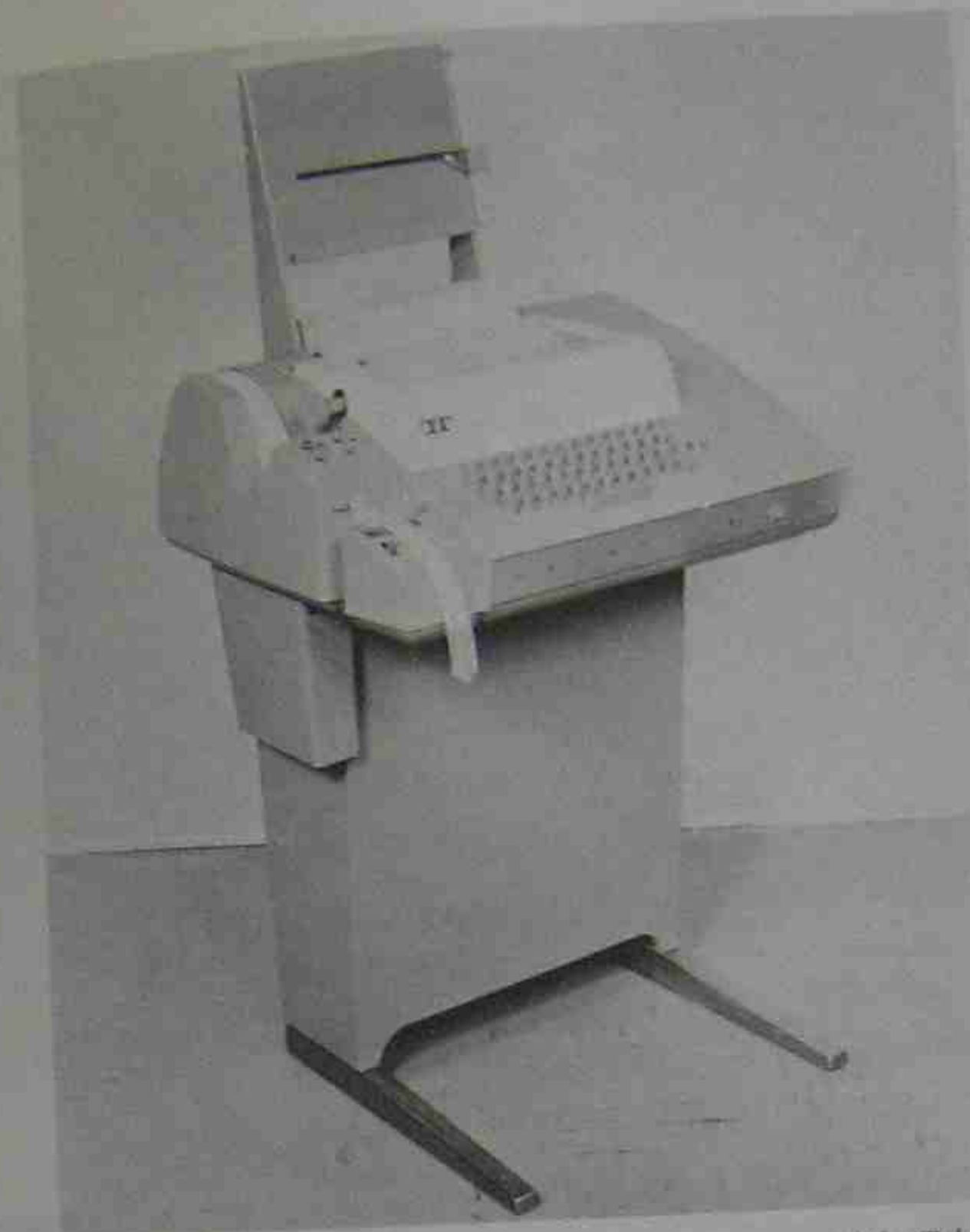
Fig. 6-26. The device shown here is a common type for preparing machine control tapes. The keyboard is similar to that of a standard typewriter. The punched tape produced is shown at the left of the unit.
