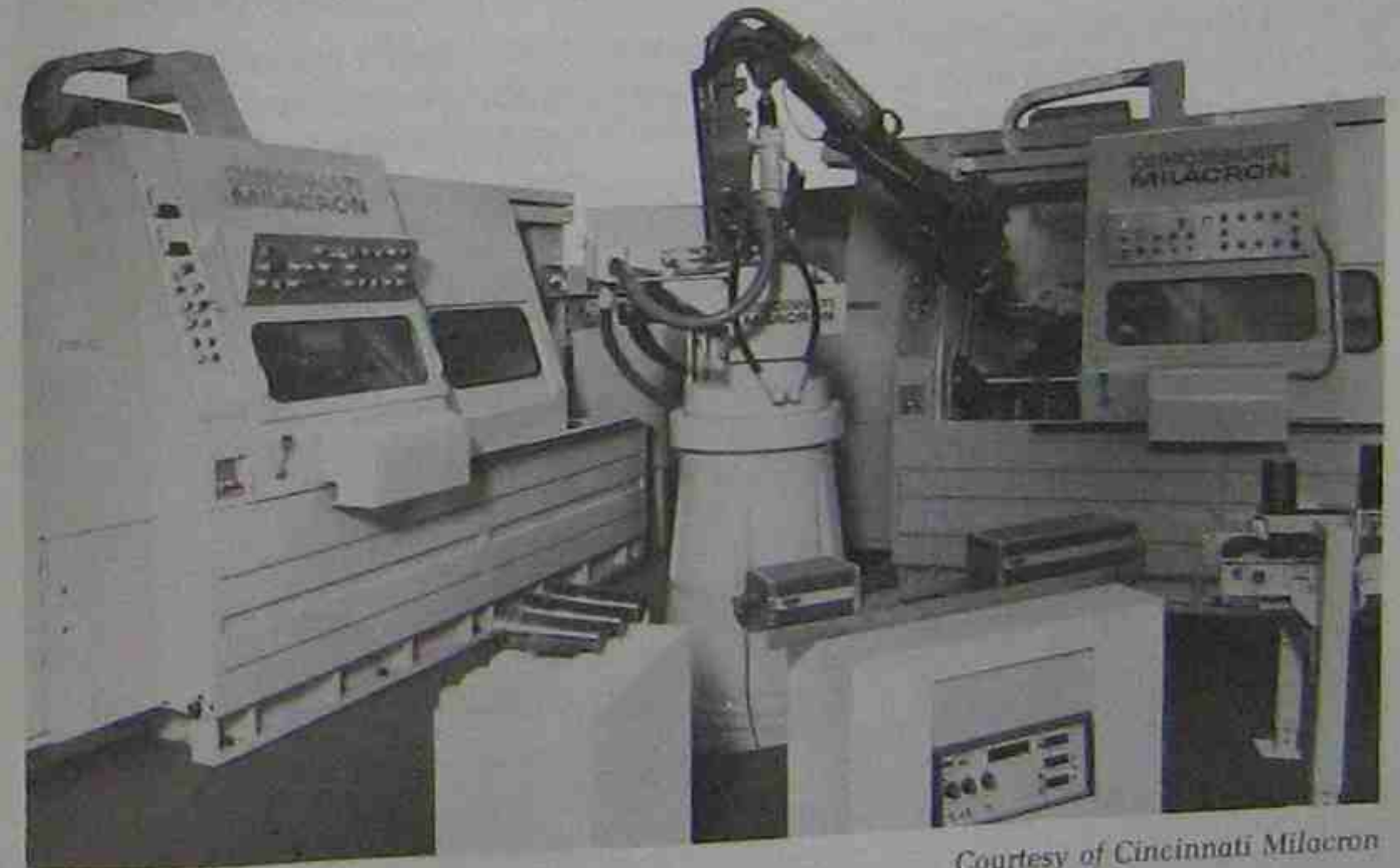
Fig. 9-13. The robot shown in the photograph is feeding two numerical control lathes. Raw material enters from the right on a belt conveyor. It is then picked up by the robot's "hand" and placed in the chuck of one of the lathes. After the part is machined it is removed by the robot and positioned in the electronic gage shown in the front of the photograph. If the part passes inspection, it is put on a pallet; if it fails, it is put on another, or scrap, pallet. If the parts are becoming out of tolerance, say due to tool wear, tool compensation is automatically entered into the control system.
