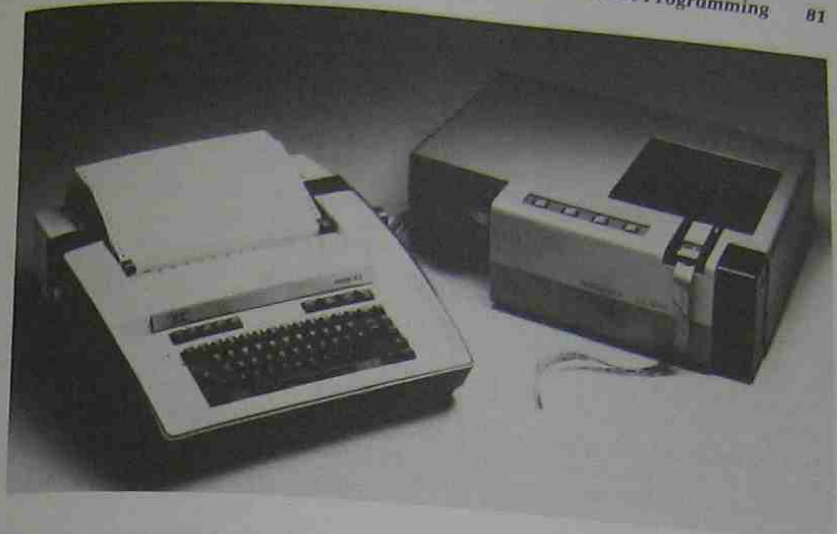
Fig. 4-2. The tape preparation system shown can edit programs in addition to preparing tapes. It can also be tied into a remote computer part programming service (see Chapter 5).
