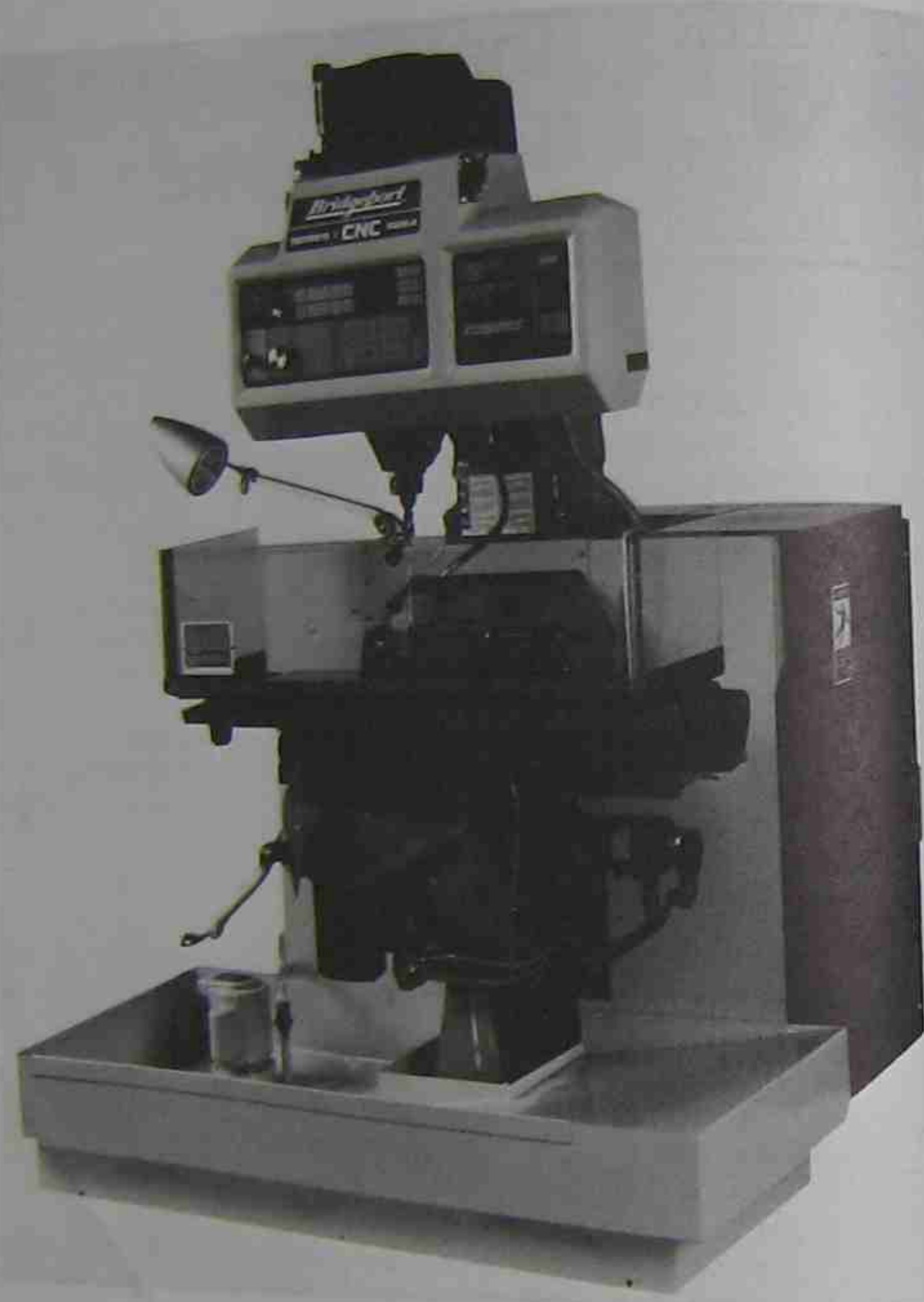
FIGURE 4-1 A vertical spindle CNC milling machine. Note the quick-change tooling system installed in the spindle. (Photo courtesy of Bridgeport Machines Division of Textron Inc.)
