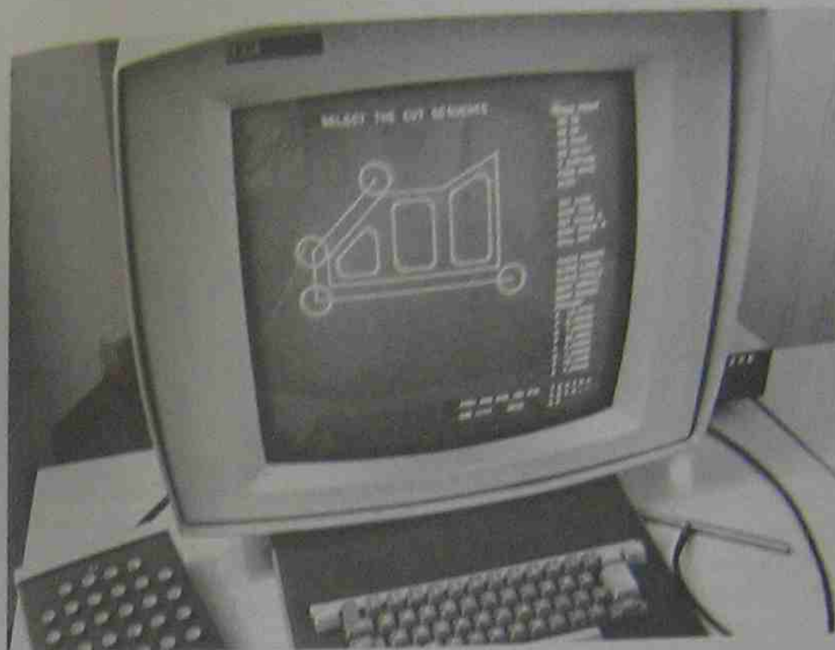
Fig. 9-2. Utilizing an electronic light pen, the programmer has the capability of moving the circular image (representing the cutting tool) around the part. A tape for the machine tool is also prepared by the computer almost simultaneously.
