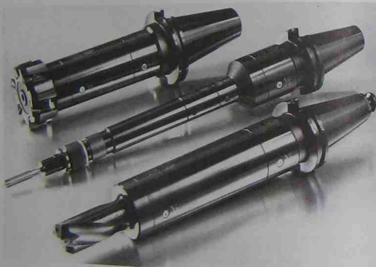
FIGURE 3-23 Special inserted tooling for use with NC. From top to bottom: an inserted milling cutter with interchangeable tooling extensions, a machine tap in a tap holder with interchangeable tooling extensions, and an inserted drill mounted in a holder with interchangeable extensions. (Photo courtesy of GTE Valenite)
