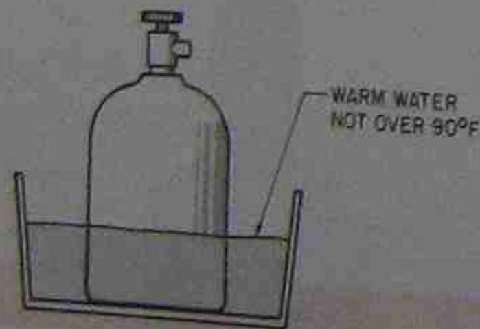
Figure 10-4. Refrigerant drum in warm water (not greater than 90° F).
