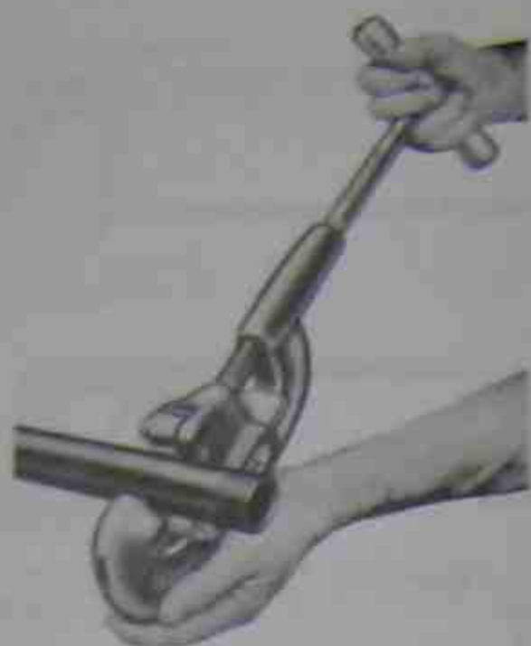
Figure 6-38. Cutting steel pipe with a pipe cutter. Courtesy Ridge Tool Company, Elyria, OH
