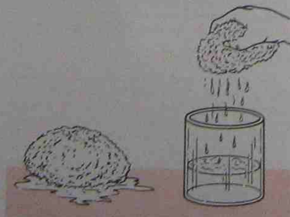
Figure 19-3. How a sponge absorbs water. The water can then be carried in the sponge to another place. When the sponge is squeezed, the water is rejected to another place. The squeezing of the sponge is considered the energy that it takes to pump the water.
