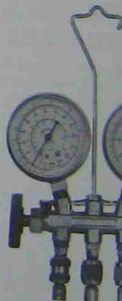
Figure 1-22. The gage on the left is called a compound gage because it reads below atmospheric pressure as well as above atmospheric pressure in psi.
