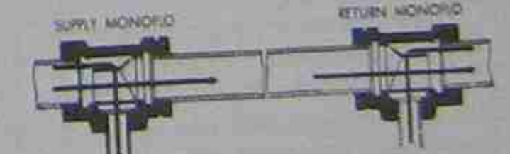
Figure 33-24. A tee for one-pipe systems. Partial water flow is diverted through the tee to the terminal unit. Courtesy ITT Fluid Handling Division
