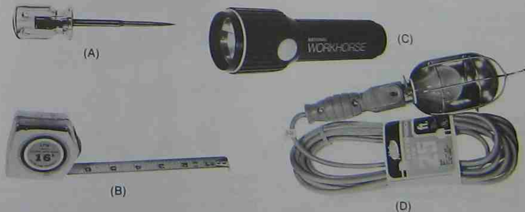
Figure 4-6. Other general-purpose tools. (A) Awl. (B) Rule. (C) Flashlight. (D) Extension cord/light. Courtesy (A) Vaco Products Company. Photos (B-D) by Bill Johnson
