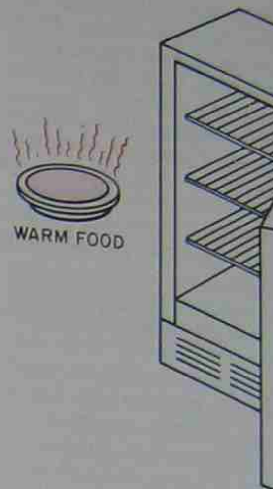
Figure 3-3. Warm food that is moved from the room adds heat to the refrigerator and is cooled. This added heat has to be removed, or the room temperature will rise.
