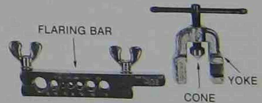
Figure 4-16. Flaring tool. This tool has a flaring bar, a yoke and a feed screw with flaring cone. Photo by Bill Johnson
