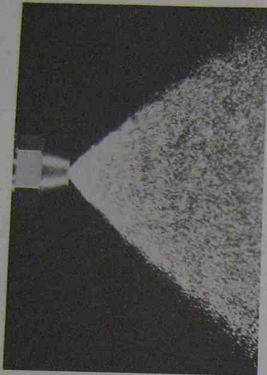
Figure 32-5. Atomized fuel oil droplets and air leaving burner nozzle. Courtesy Delavan Corporation
