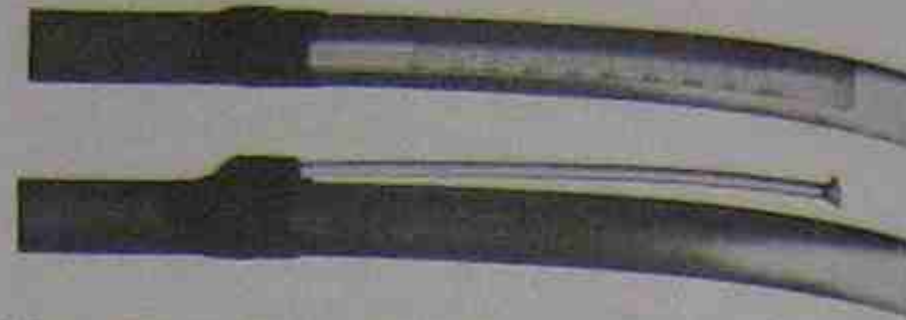
Figure 43-13. Glass thermometer strapped to a refrigerant line. Photos by Bill Johnson
