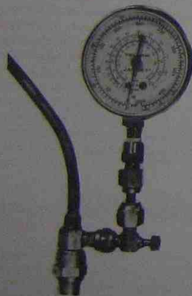
Figure 45-49. High-pressure gage for checking the head pressure on a heat pump with a critical charge. Photos by Bill Johnson
