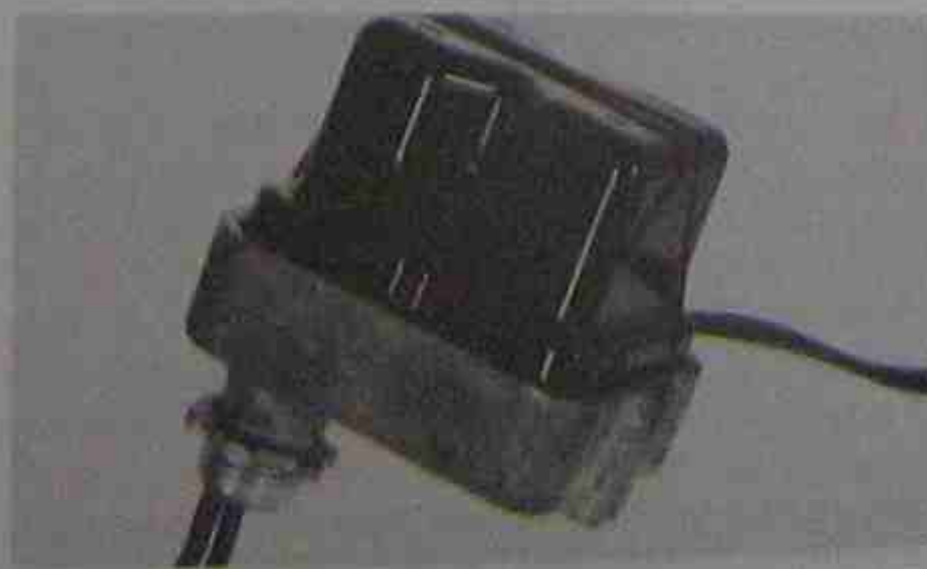
Figure 41-16. Fan relay. Photo by Bill Johnson
