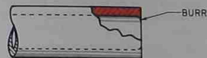
Figure 6-35A. Burr inside a pipe.
