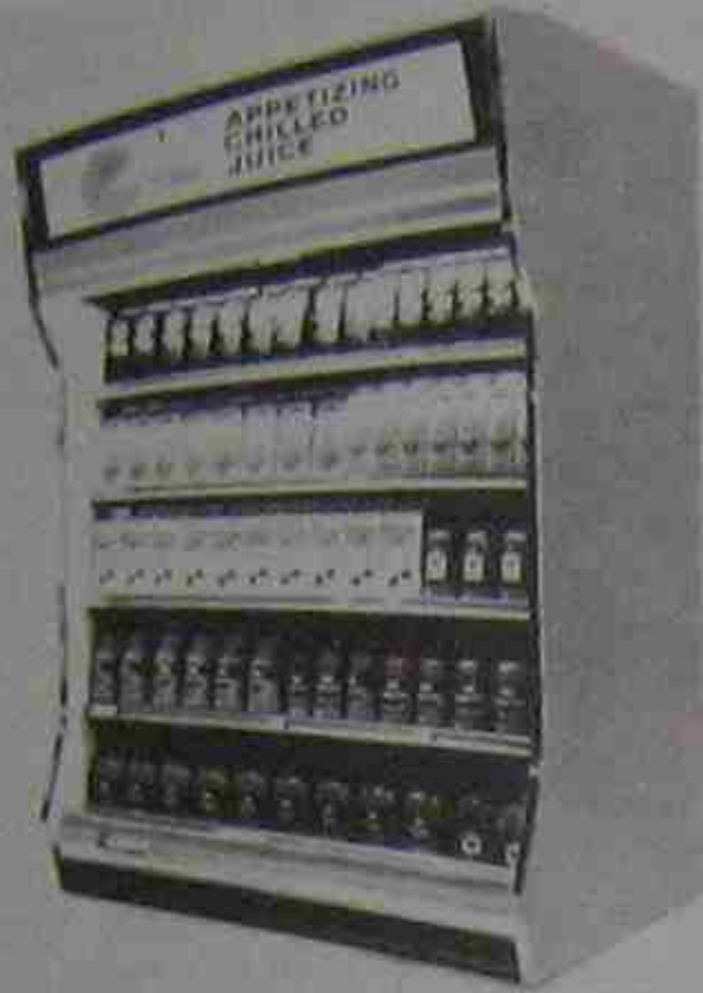
Figure 24-3. Self-contained refrigerated box has its condensing unit built in. Refrigeration tubing does not have to be run. This box rejects the heat it absorbs back into the store. It is movable because it only needs an electrical outlet and, sometimes, a drain, depending on the box. Courtesy Hill Refrigeration.
