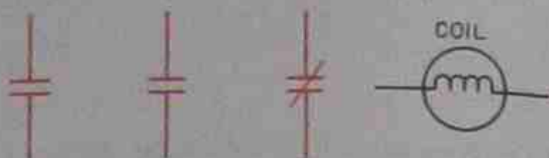
Figure 28-5. Relay with two sets of contacts that close and one set that opens when the coil is energized. It has two normally open contacts (NO) and one normally closed (NC).
