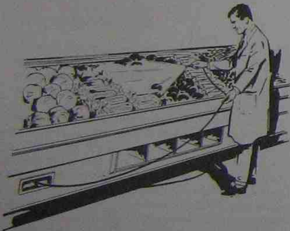
Figure 24-14. Open display case used to store fresh vegetables. The case has a drain, so the vegetables can be wet down with a hand-operated sprinkler. Courtesy Tyler Refrigeration Corporation
