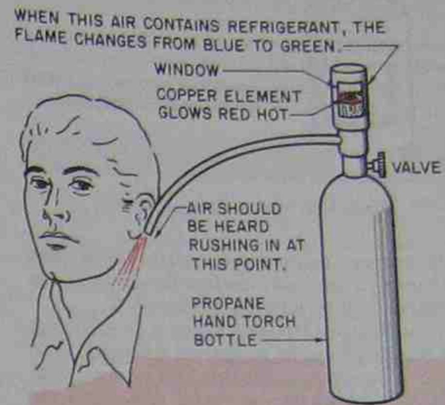
Figure 9-28. A rushing sound may be heard at the end of the sampling tube if the halide torch detector is pulling in air and working correctly.
