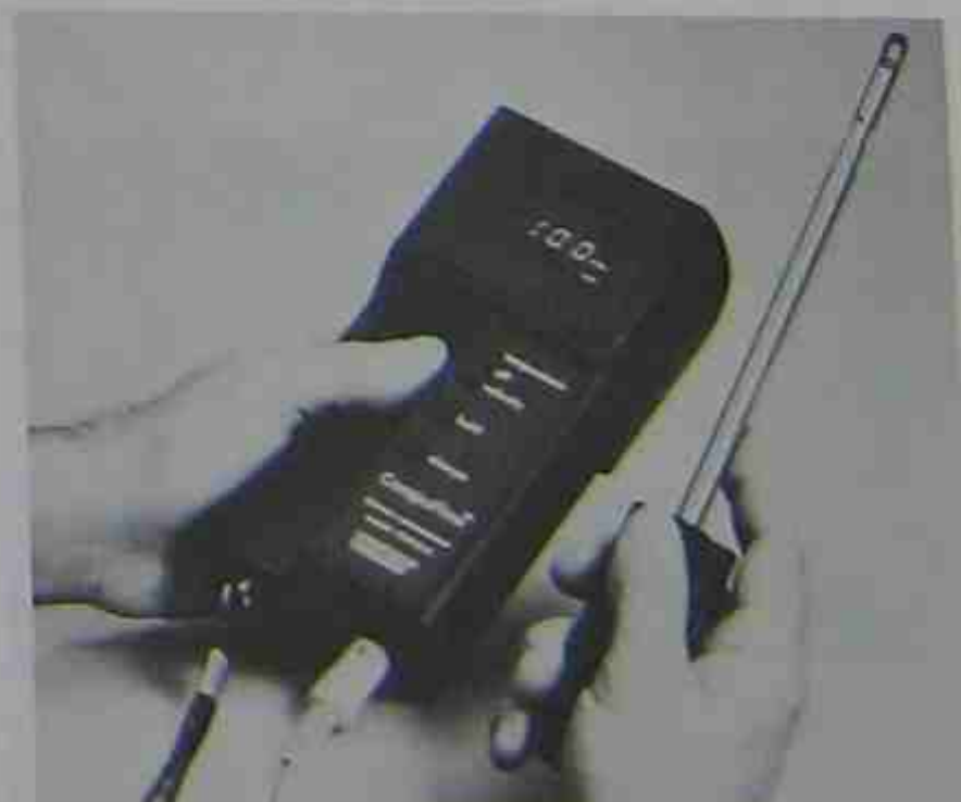
Figure 4-44. Air velocity measuring instrument with microprocessor. Courtesy Alnor Instrument Company
