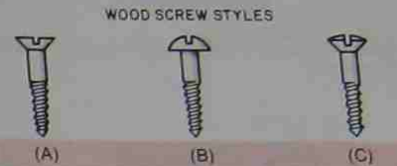
Figure 5-7. (A) Flat head wood screw. (B) Round head wood screw. (C) Oval head wood screw.
