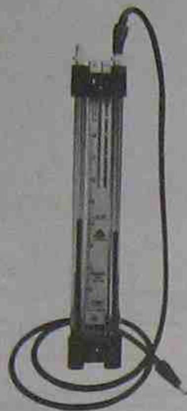
Figure 31-8. A manometer used for measuring pressure in inches of water column. Courtesy Robinair Division—Sealed Power Corporation
