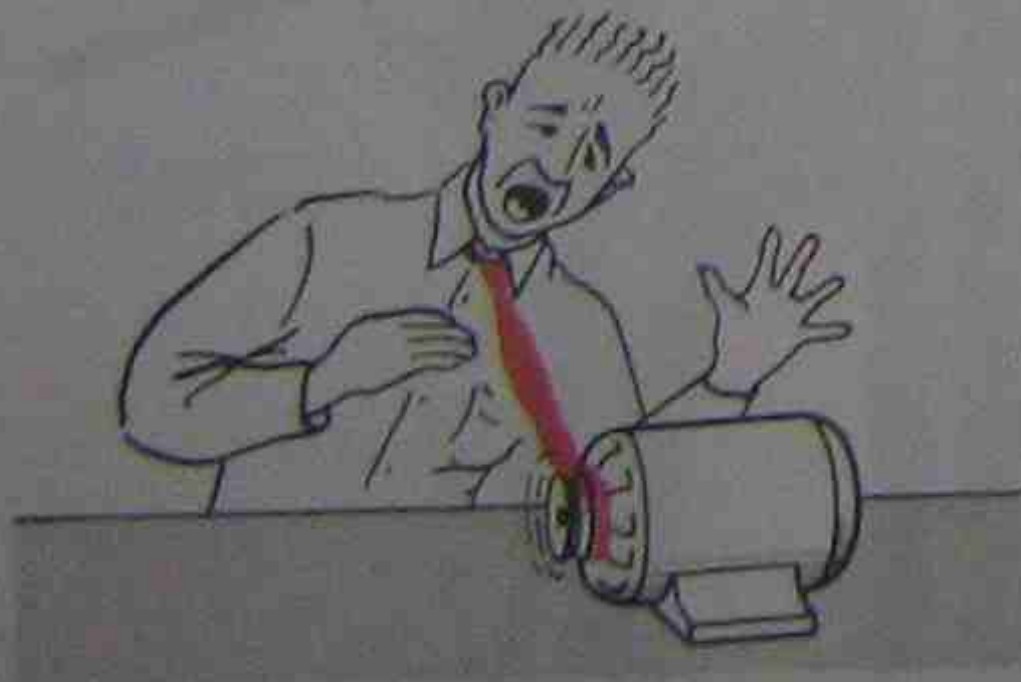
Figure 10-14. *Never wear a necktie or loose clothing when using or working around rotating equipment.*
