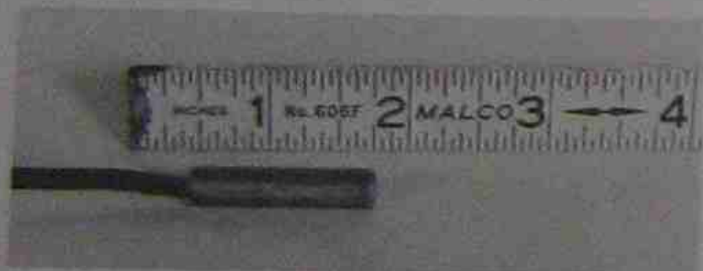
Figure 12-23. A thermometer probe using a thermistor to measure temperature. Photo by Bill Johnson
