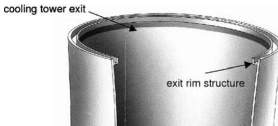
Figure 17: Stabilizing structure at the inner rim side.
