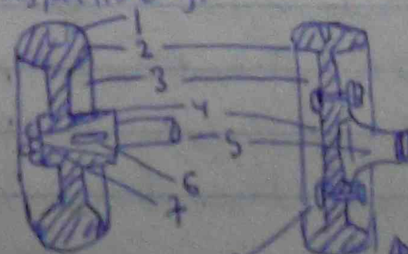
Fig / Section of flywheel coupled with crankshaft
