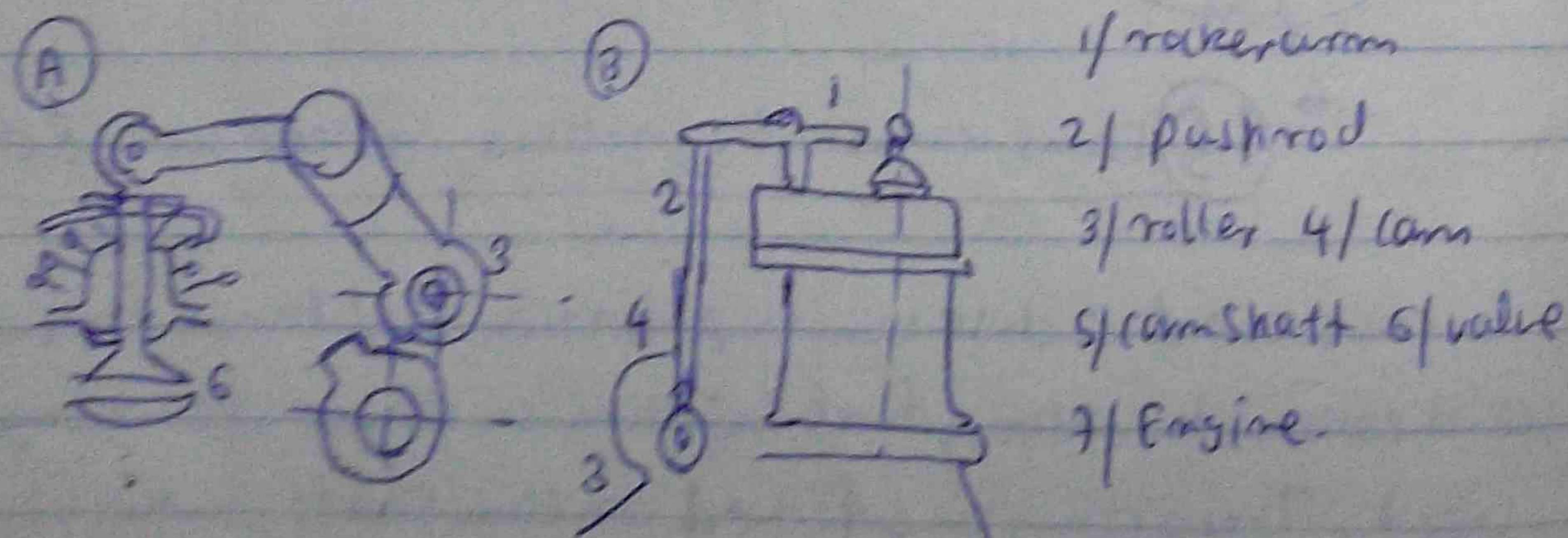
Fig 1 valve driving mechanism for low speed four cycle engines
