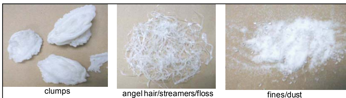
Figure 3.3 Types of degradation in delivery/conveying
