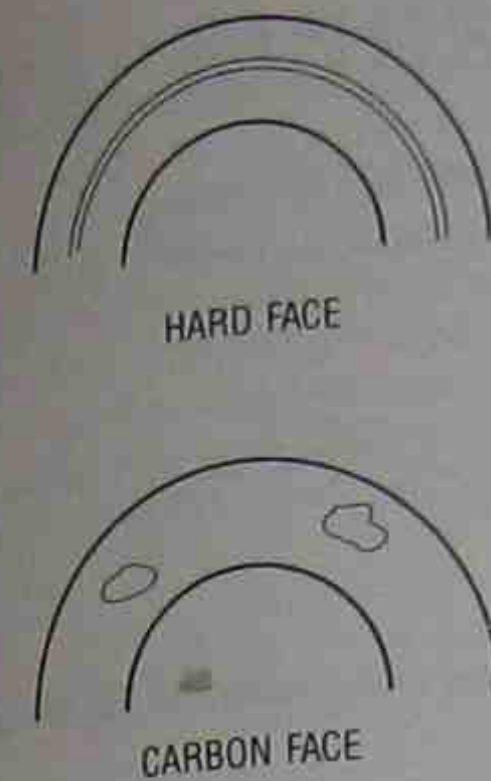
Fig. 9-45 Typical evidence of sludging and bonding.
