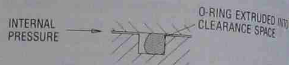
Fig. 9-16 Evidence of extrusion.
