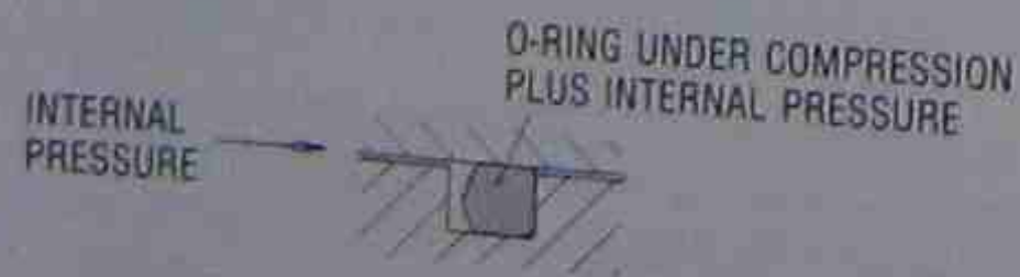
Fig. 9-13 The O-ring is forced against the side of the groove.
