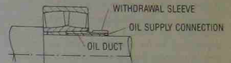
Fig. 6-58 Withdrawal sleeve machined with oil ducts.
