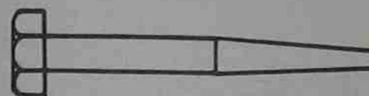
Fig. 25 — A drift pin made from a bolt
