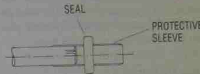
Fig. 9-63 Using a protective sleeve.
