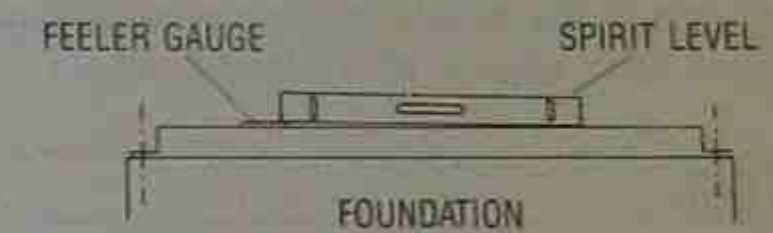
Fig. 3-5 Using a feeler gauge to determine adjustments.
