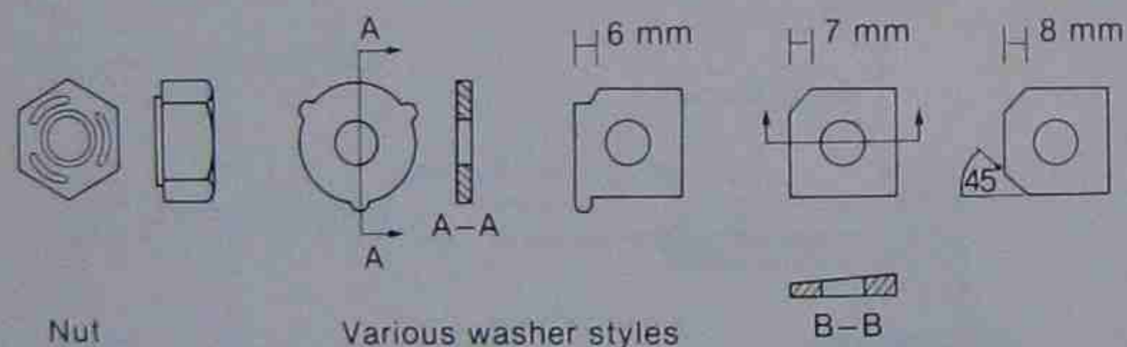
Fig. 5.4 Nuts and washers for use with HSFG bolts
