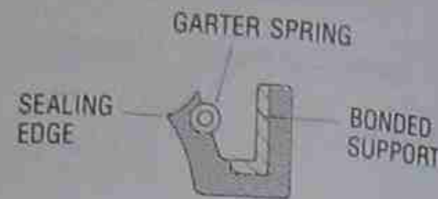
Fig. 9-59 The principles of bonded construction.
