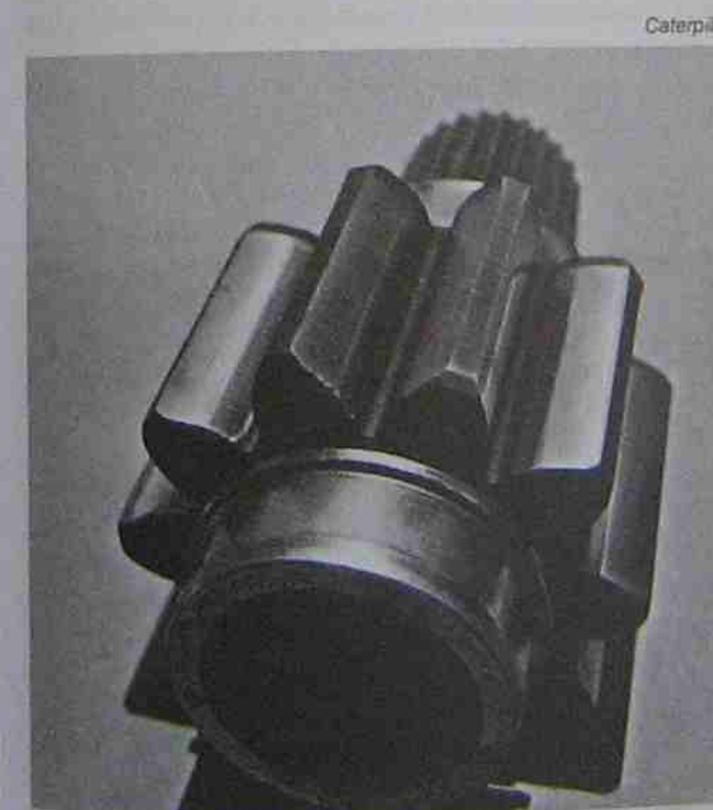
Fig. 7-60 Abrasive wear patterns.
