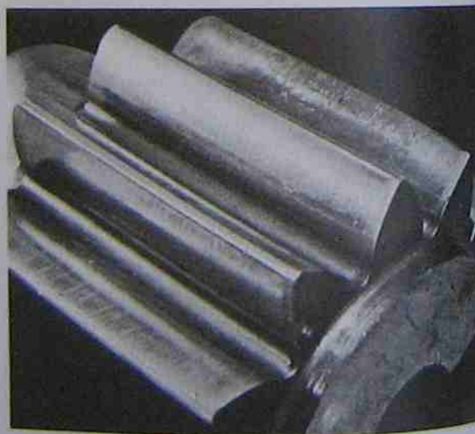
Fig. 7-58 Normal wear under light to moderate loads.
