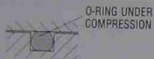
Fig. 9-12 A typical arrangement of a static sealing O-ring.
