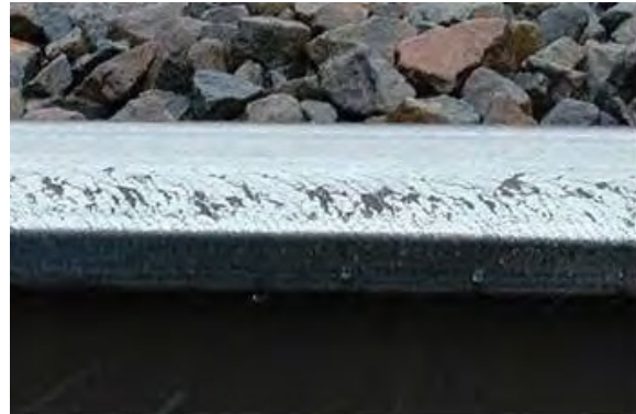
Severe Checking with Spalling
