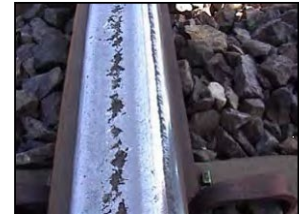
Severe Rail Center Spalling
