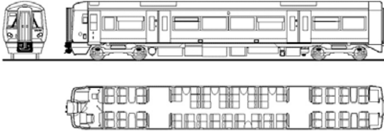
Figure 3.1: Technical drawing of a wagon from an Electrostar EMU operated in United Kingdom
