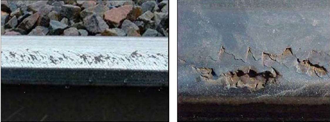
Severe Flaking with Head Checking
