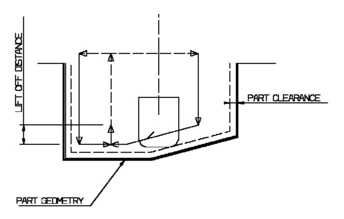
Lead-in, Lift-off and Attack for Recess Turning
