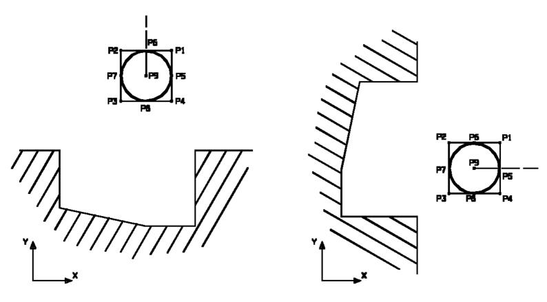
The tool output point is dependent on the machine axis system.
