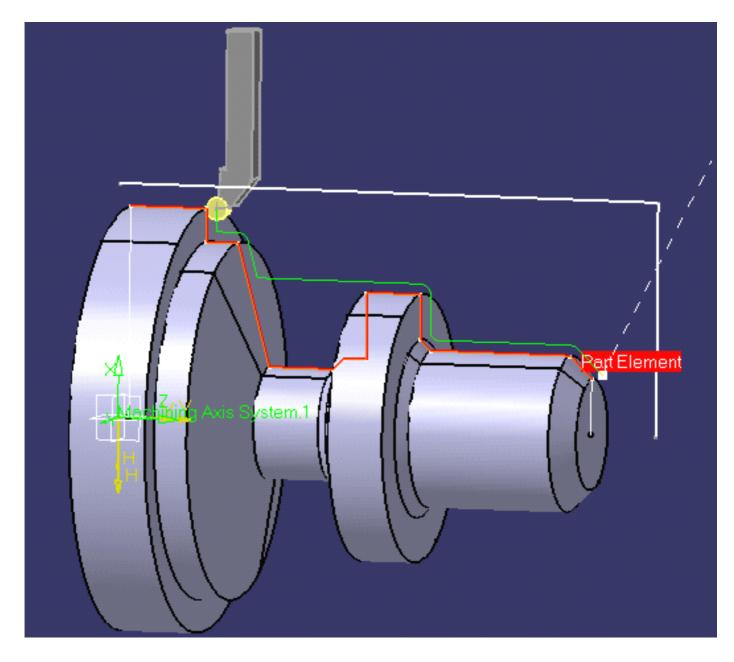
Click OK to exit the replay mode and return to the Profile Finish Turning dialog box. **5.** Click OK to create the operation in the program.
