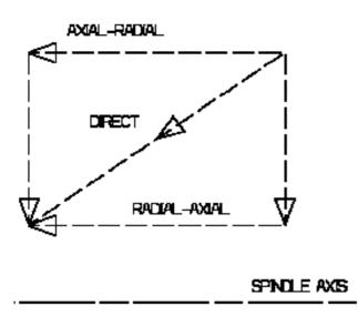
Linking macros, which comprise retract and approach motion can also be used on roughing operations.
