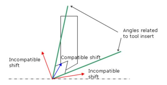
The shift direction must be inside the limit angles defined on the tool insert otherwise a collision may occur. In collision cases, the collision is on the first pass, not on the last passes of the toolpath.
