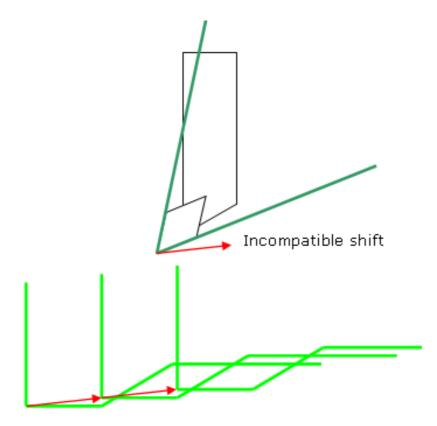
The parallel contour toolpath is in collision because the shift does not respect the tool insert angle on the right side.
