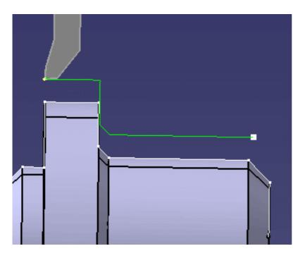
• **End limit offset**: distance with respect to the end element (only if end element is a line or a curve, and when In or Out is set for end element positioning).
