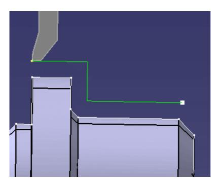
• Axial part offset: specifies a virtual displacement of the part profile along the spindle axis direction.
