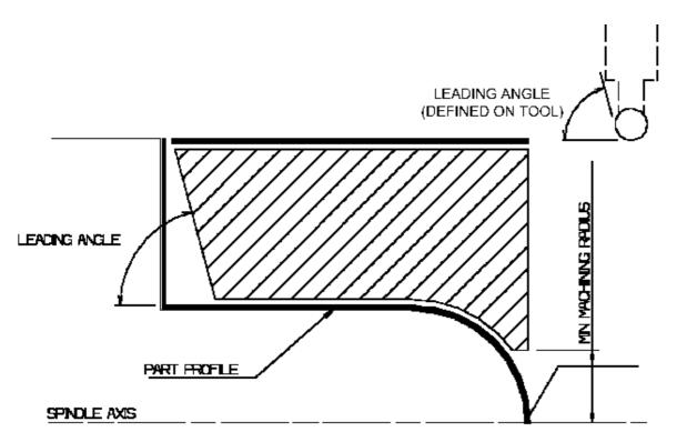
Maximum Machining Radius (for internal machining)
