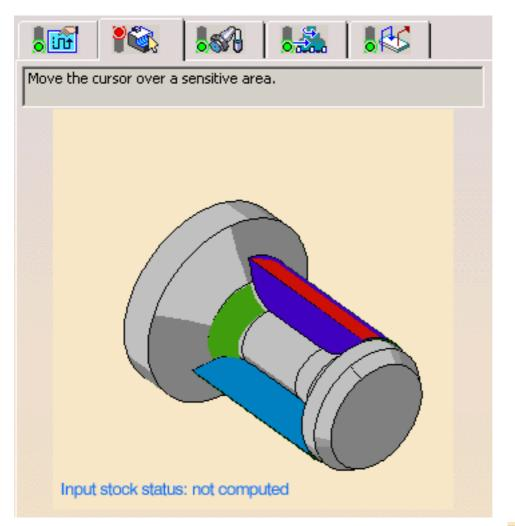
**6.** Select the **Update Input Stock** command by either clicking the icon **input stock status** field in the sensitive icon. The stock is computed and the corresponding sketch profile is displayed in the viewer.
