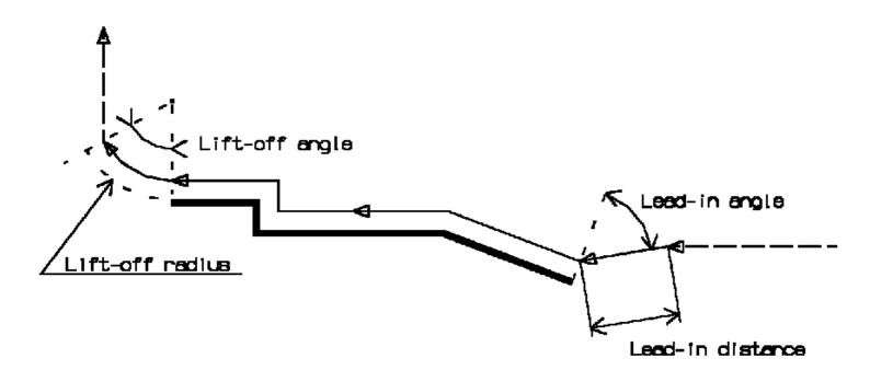
Linear lead-in and circular lift-off (Profile Finish Turning)
