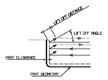
For Longitudinal or Face Rough Turning, lift-off occurs:
