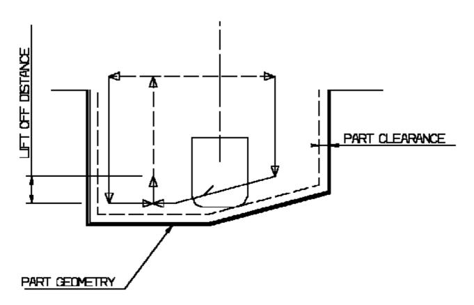
Plunge and Lift-off for Ramp Recess Turning
