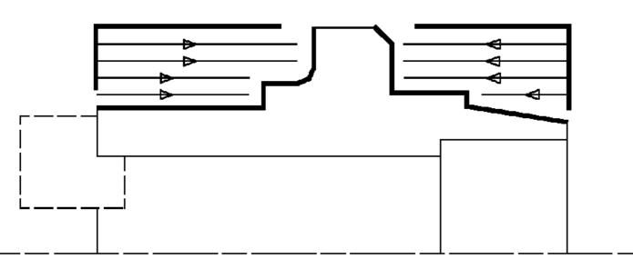
Orientation and Location settings determine the way the program closes the area to machine using radial, axial, axialradial or radial-axial relimitation.
