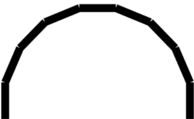
Figure 6-5. Acceptable 180° turn made gradually from 22.5° segments
