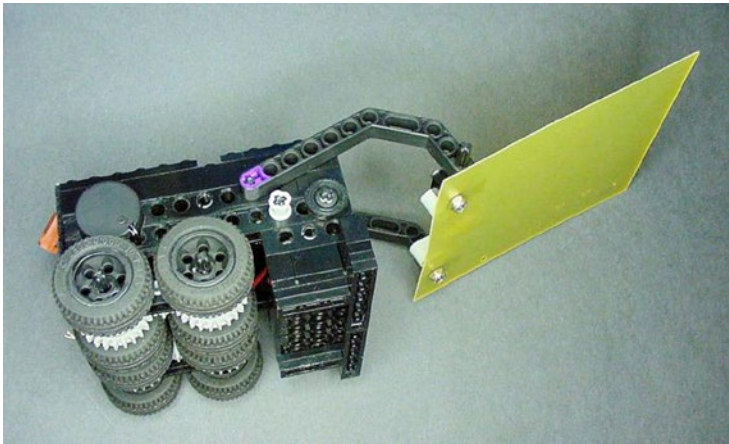
Figure 19-8. A mini-sumo robot with eight wheels selected for maximum pushing
