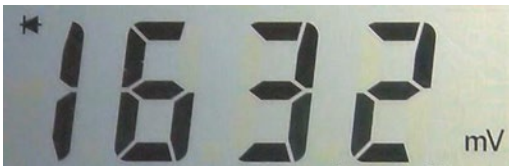
Figure 10-17. Multimeter displaying normal LED value
