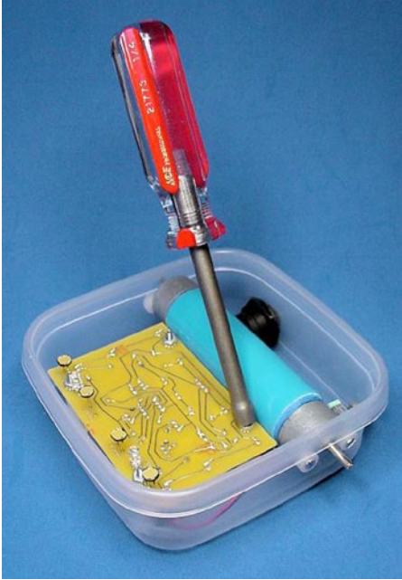
Figure 24-28. Nutdriver tightening nuts onto standoff screws
