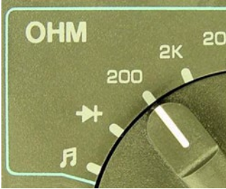
Figure 8-6. Multimeter dial set to lowest ohm range
