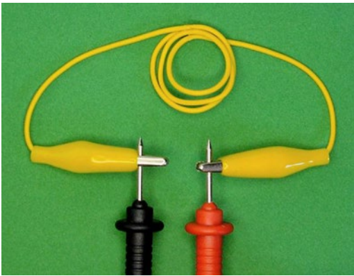
Figure 8-11. Making a connection with alligator jumper leads
