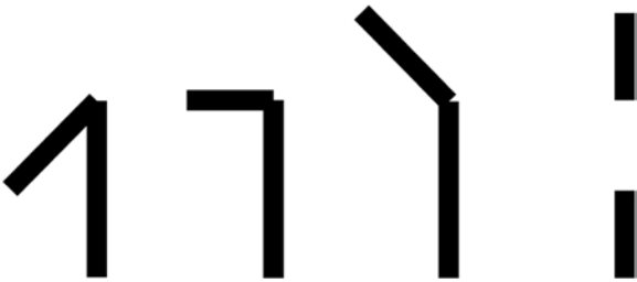
Figure 6-4. Unacceptably sharp turns: (left to right) 135°, 90°, and 45°. (far right) broken line
