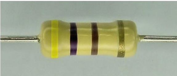
Figure 5-7. Color bands of yellow, violet, brown, and gold (470 at 5% Tolerance)
