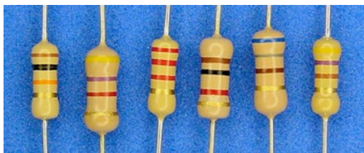
Figure 11-11. Resistor values for experimenting: from 10,000 \Omega down to 470 \Omega
