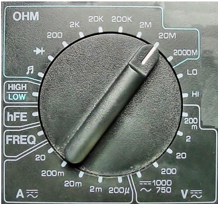
Figure 4-7. Dial with groups of manual range settings
