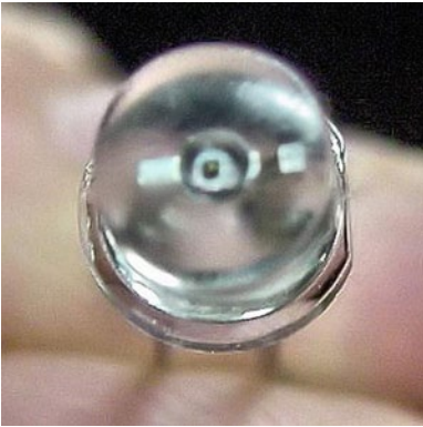
Figure 10-9. View of a reflector cup and die
