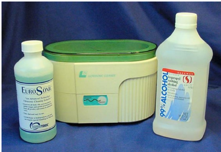
Figure 19-15. Ultrasonic cleaner (middle) with cleaning solution (left) and 99% isopropyl alcohol (right)
