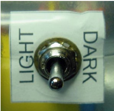
Figure 25-3. A printed piece of paper inserted inside the container for labeling the line-following switch
