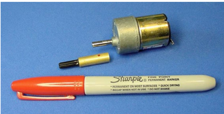
Figure 20-18. Marking desired location for the setscrew hole on a coupler using a fine-point permanent marker
