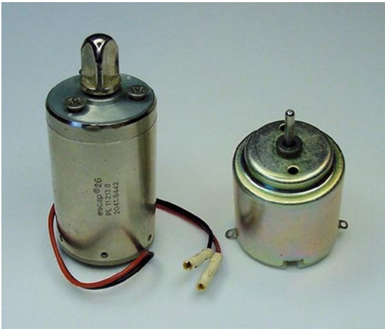
Figure 17-20. Escap motor (left) and toy motor (right)
