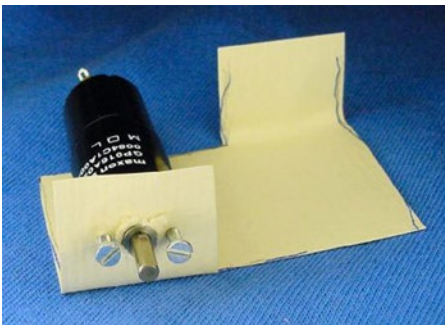
Figure 24-3. Design with folded paper before cutting complex metal shapes
