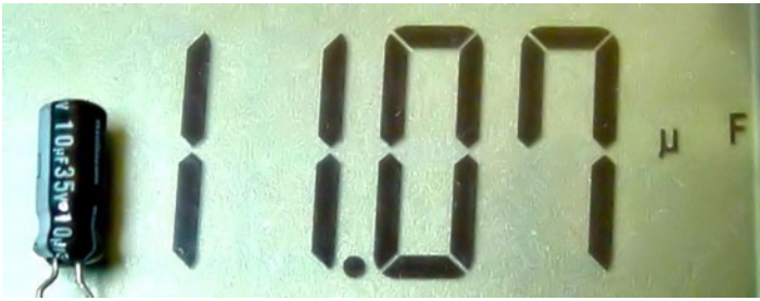
Figure 5-9. A multimeter shows the capacitor marked 10 \mu\text{F} is actually 11 \mu\text{F}
