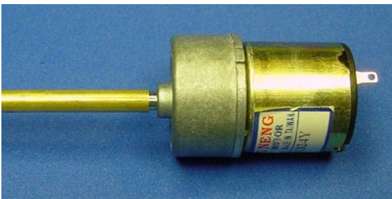
Figure 20-6. Motor shaft inserted into \frac{3}{16} -inch diameter tubing
