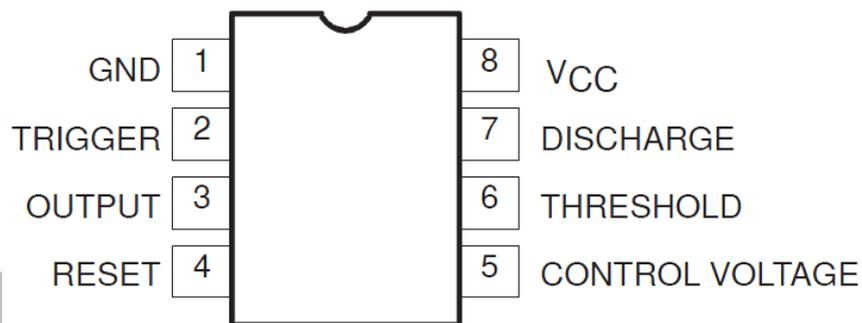
Fig: Pin diagram of IC 555
