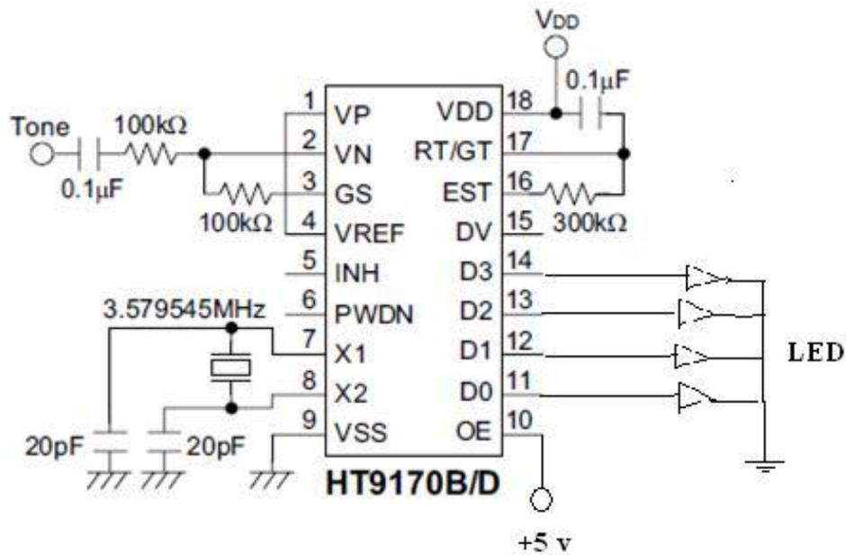
Fig: Interfacing Mobile with DTMF IC
