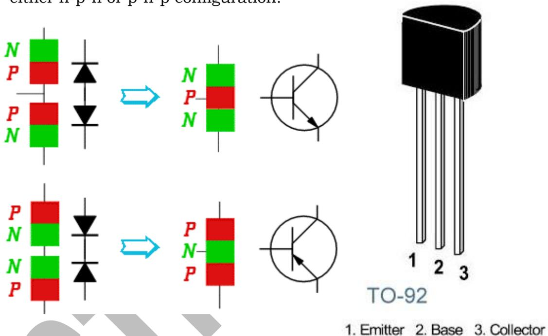
The middle, or *base*, region between the junctions is typically very narrow. The other regions, and their associated terminals, are known as the *emitter* and the *collector*. A small current injected through the junction between the base and the emitter changes the properties of the base-collector junction so that it can conduct current even though it is reverse biased. This creates a much larger current between the collector and emitter, controlled by the base-emitter current.
