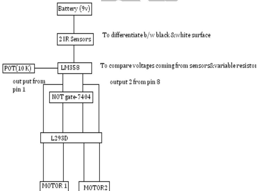
**Working:** The power supply given to the circuit through battery (9 volt). IR sensors sense the light, and if it is placed on a white surface transmitter send the light signal to the receiver by
