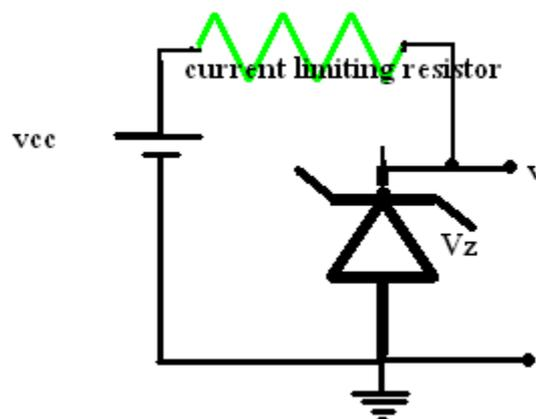
**NOTE:** If current limit resistor is not connected or it is not of proper value, then it causes heating of the zener diode. So remember about this before touching zener diode. If the input voltage is less than  $V_z$  then output voltage will be zero (ideally).
