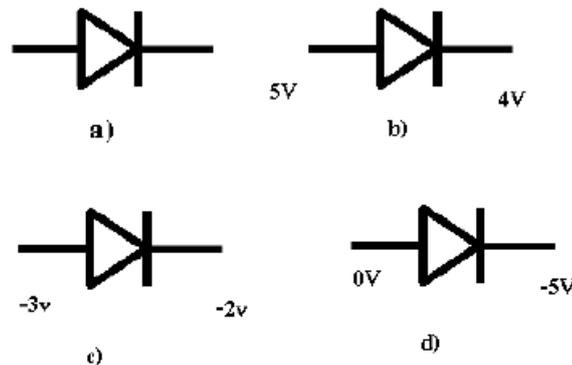
From the above figure try to find out which diodes are forward biased and which are reversed biased. You can see that a) is represents symbol of a diode b), d) are forward biased and c) is reverse biased(voltage at the P N junction should be greater than N junction by .7V).
