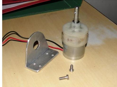
DC Geared Motor with Motor clamp
