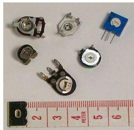
PCB mount [trimmer](#) potentiometers, or "trimpots", intended for infrequent adjustment.
