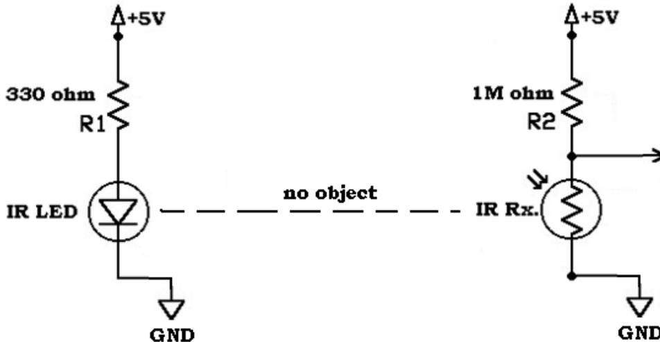
When no object is there in between the IR Tx. – Rx. Pair, complete light goes to the receiver. But it gets blocked when an object comes in between.
