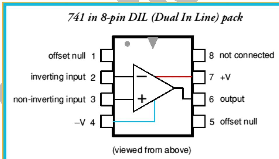
Power supply voltage  $\pm 3V$  to  $\pm 18V$
