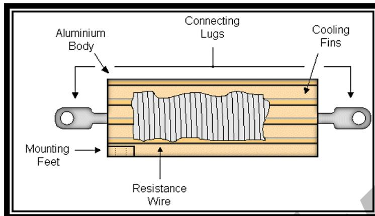
Wire wound resistor types are prefixed with a "WH" or "W" notation (eg WH10 $\Omega$ ) and are available in the WH Aluminum Cladded package ( $\pm 1\%$ ,  $\pm 2\%$ ,  $\pm 5\%$  &  $\pm 10\%$  tolerance) or the W Vitreous Enameled package ( $\pm 1\%$ ,  $\pm 2\%$  &  $\pm 5\%$  tolerance) with power ratings from 1W to 300W or more.
