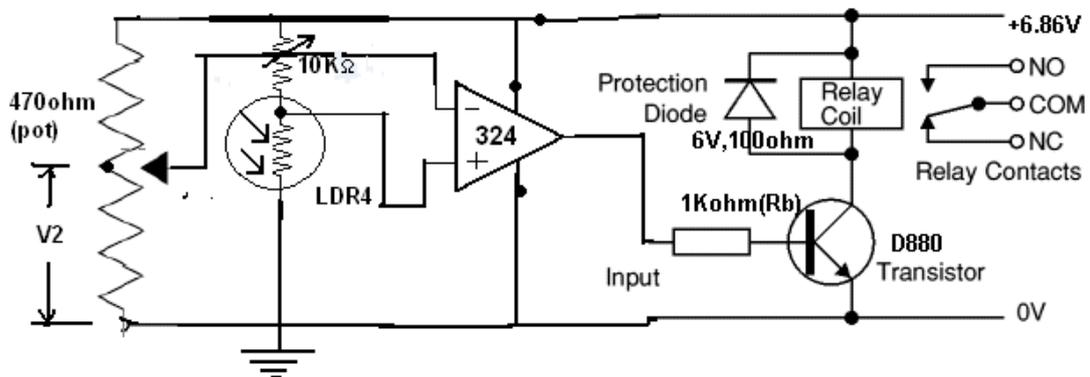
This circuit is used to turn ON light or any equipment if the light intensity is below a level. This level is set by 470ohm pot (i.e,  $V2$  is the reference). You can make the same circuit using power transistor, but difference between two.
