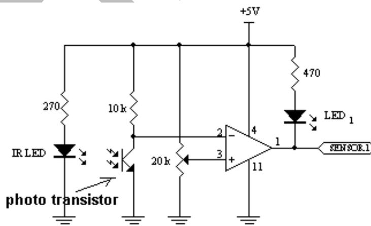
Here when light is not there then the resistance of transistor will be high, so the  $V_{-}(\text{pin}2) > V_{+}(\text{pin}3)$  making output of comparator LOW. That is when no reflection from ground or any obstacle on the IR. When light is there then the resistance will be very less and
