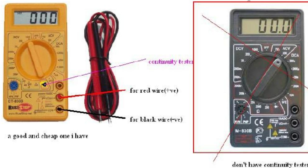
Suppose if you want to measure output voltage of an adapter, see what is the maximum voltage of adapter (mostly around 15V). Then put the needle to 20V (a voltage greater than 15V). A display of '1' on multimeter means that it is not able measure the quantity in that position of the needle.
