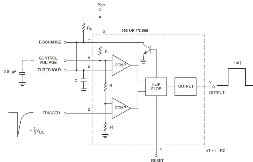
Fig: Monostable Operation
