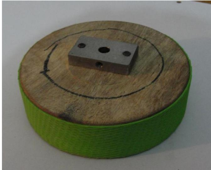
Tires with Hub for robot (Rear and Front view):
