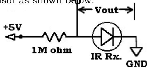
As we always check the output relative to ground terminal, also, as ir light falls on the receiver, its resistance decreases, so the output voltage is measured across receiver decreases. You can check it on multimeter connecting the output of the circuit to positive/red lead of the multimeter and other terminal to the ground reference.
