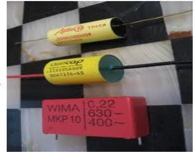
6. **Polyester:-** These type of capacitor has high tolerance and these types of capacitors are used in blocking, bypassing, filtering, coupling and decoupling, interference suppression in low voltage circuit
