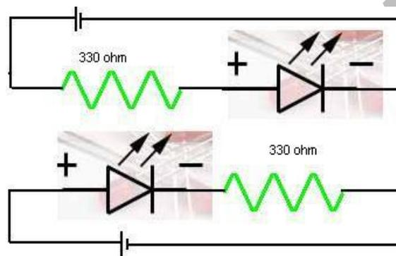
What is the difference when u connects resistor at anode side and resistor at cathode side. There is a difference in case of 7-segment displays.
