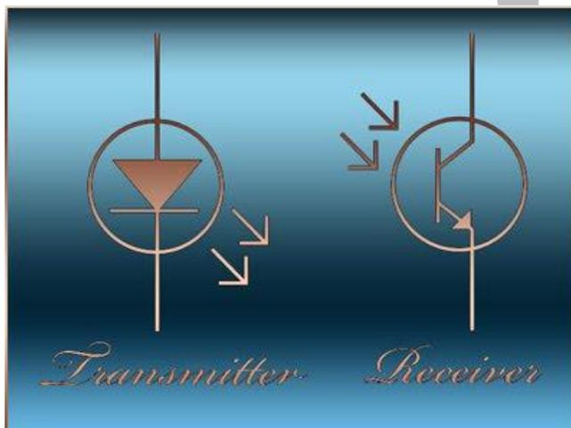
So, for transmitter, we consider an IR light source with outward arrows indicating that it emits IR radiations and inward arrows for IR receiver showing it as an IR light detector.
