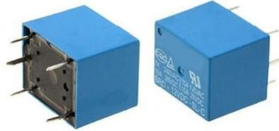
Relay is an electromagnetic device which works on magnetic field. The only difference between a switch and a relay is that switch operates when given a manual input whereas relay on the other hand triggers when given an input electrical signal on its 2 input terminals. Relay is also called an electromagnetic switch. If you apply proper low voltage on one side the metal will get contacted. Following figure shows an SPDT Relay and its terminals.
