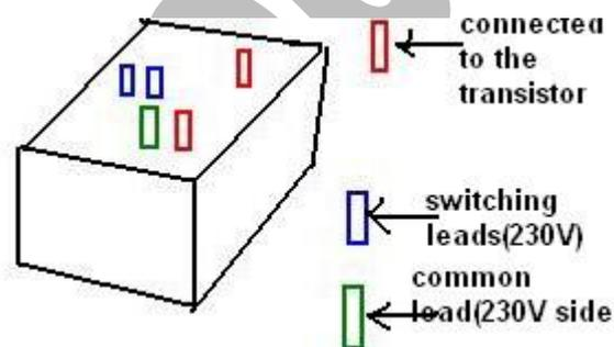
Here it is a small relay representation (a diagram of relay i have). The other side of the relay can be 230V or even 5V (no restriction), but we normally get 230V relay, means voltage $\leq$ 230 (on the 230V side). You can use this in the last stage of a line follower(assume that line follower has more than 2 LDR's), when last sensor go out of the line, you can use relay mechanism to provide Vcc to the other lead of the motor so that motor start to rotate backward.
