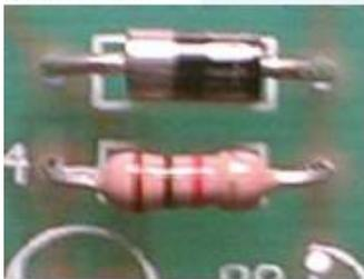
Above figure shows how to bend the leads of a diode and a resistor so that a properly inserted into breadboard or PCB. But remember not to bend too close to body. But there are different diodes LED, IRLED, Photo Diode, and Zener Diode. But in robotics we use LED, IR LED's, and Photo Diodes. Diode and Zener diodes are used, but rarely.
