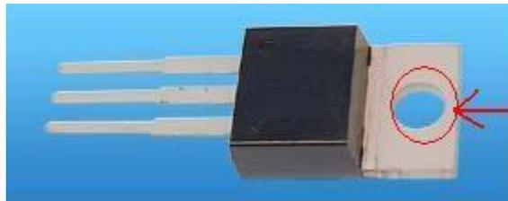
position for screwing the heat sink
