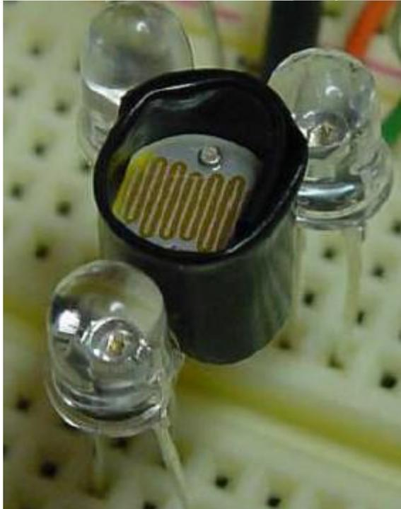
Above figure shows how LED is placed with LDR. Here LDR is covered because we want light reflections from ground only, not from sides of LED. Also cover the LED so that the light will move pointed, so that reflection will directly go to LDR. When you attach
