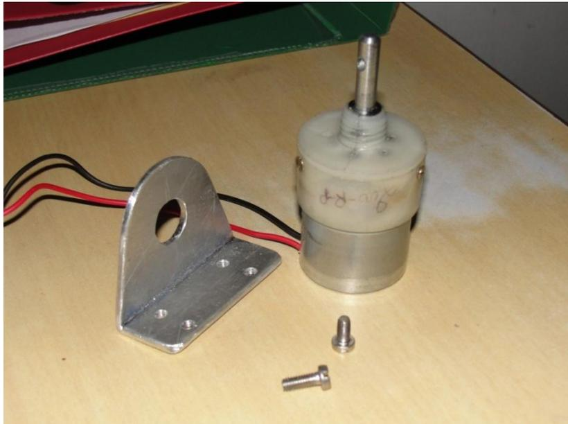
Fig: Metallic Dc Geared Motors (100/60 RPM)
