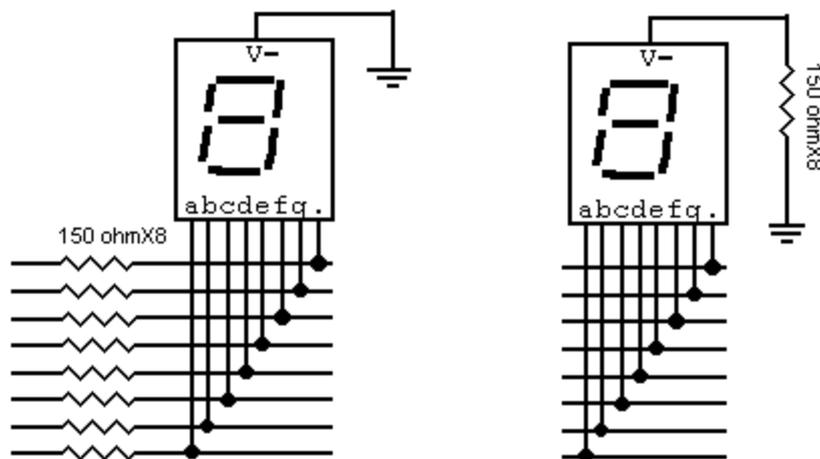
See in the above diagram, you can see that resistance is connected at common cathode only. There is a difference between two. 7Segment display consist of 7 led's. Connecting a resistor in series with every LED and connecting a resistor in series with all LED's
