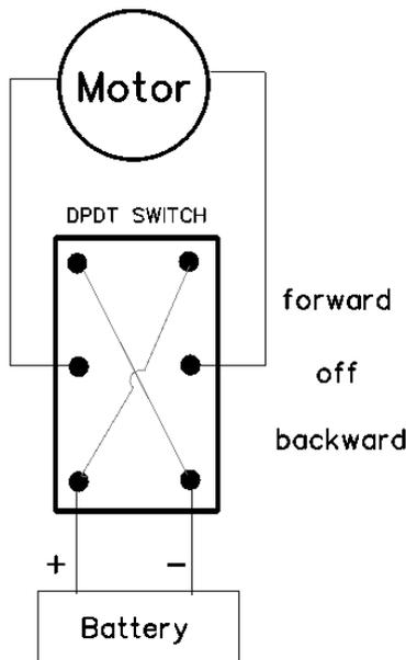
**Note:** we need at least 6 terminal switch (DPDT) to forward, reverse and stop the motor as shown in picture below
