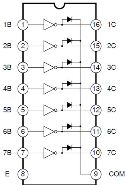
It accept 5 volt signal as input and can drive 7 motor in ON-OFF , 7 relay and high power lamps
