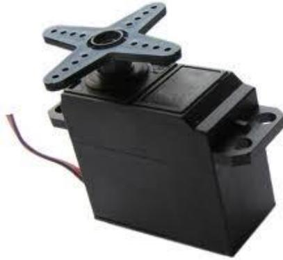
The shaft typically does *not* rotate freely round and round like a DC motor, but rather can only turn 200 degrees or so back and forth.
