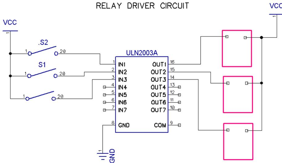
In these circuit input can be given from any Digital ic / Microcontroller / Switches / Computer Parallel port etc . Do practise on this circuit before using ULN2003 with other IC.
