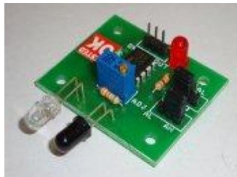
Above method helps in detecting the object by reflection from the surface. In this case, in normal condition, no IR light passes to the receiver, but as the object comes in front IR light is reflected from the object and passes to the receiver.
