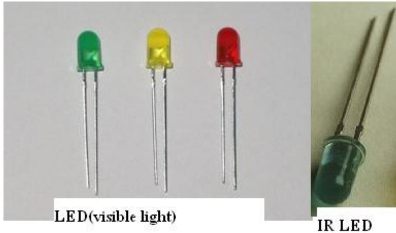
LED has two leads- cathode and anode. They are identified by the length of the lead. Cathode lead is of lesser length. But I have seen some LED's with manufacturing defect having cathode lead longer. So in order to identify the cathode of the LED see the figure below. In that you can see that cathode is of broader filament. I got some white LED's of cathode of small filament. So this convention can be right or wrong. Check LED in both ways to see that LED is good.
