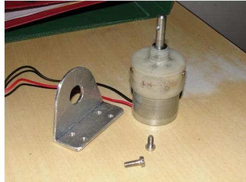
DC Geared Motor with Motor clamp
