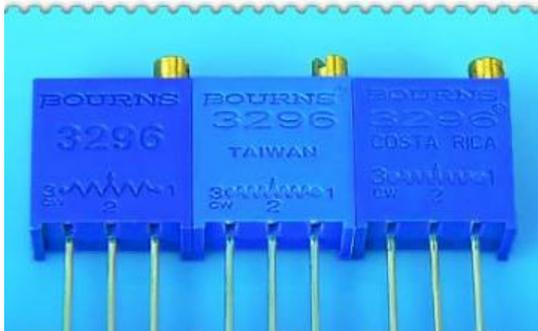
High Precision Variable Resistors 10 Ohm
