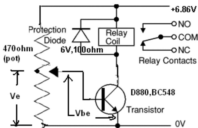
This circuit is used to turn on or turn off relays. Suppose if you use an LDR and a series resistor to turn ON and OFF light in your room, if the intensity of the light become LOW.
