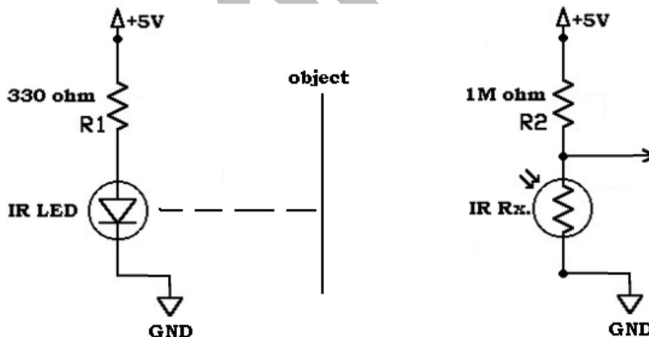
**Output from IR Sensor:** As the output comes in the form of varying voltage, so, this could be given to a comparator such as: LM358, LM741, LM324, etc. or to an Analog to Digital Converter or an IC NE555 in monostable mode or astable mode.
