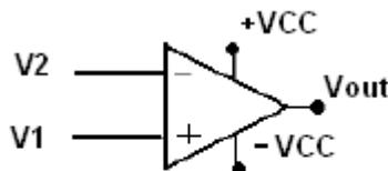
Above figure shows the general circuit diagram of a general comparator. If  $V1 > V2$  then  $V_{out} = +V_{cc}$  and if  $V1 < V2$  then  $V_{out} = -V_{cc}$ . Suppose if  $V1 = V2$ , then output will be  $+v_{cc}$  or  $-v_{cc}$  theoretically. But practically no such condition exist, because an operational amplifier has a gain of  $10^6$ , so there is no condition exist.
