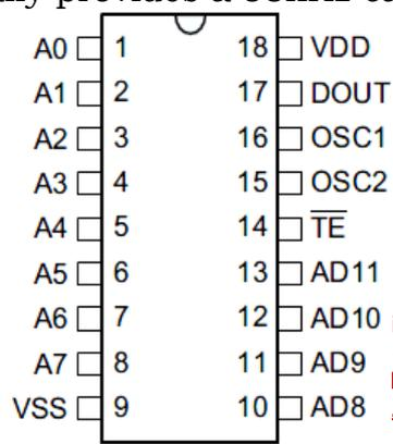
Pin Diagram of HT12E (Encoder)
