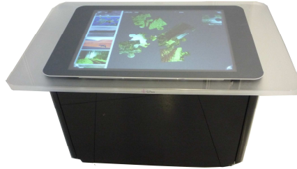
Figure 1. The Microsoft Surface was used for the evaluation of different interaction techniques for touch devices.
