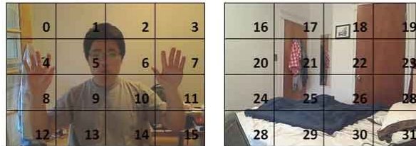
Figure 4. Each image is divided into 16 states resulting in 32 states across two camera views
