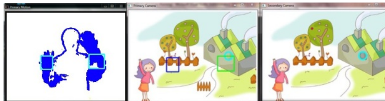
Figure 7. Hidden Paintings : The interface contains windows that display two versions of a picture* and tracking results. The detected hand locations (cyan) are shown overlaid onto the binary version of the motion energy image. The tracked locations of the left and right hands are mapped to corresponding positions in the original version of the picture (blue and green rectangle). The goal of the user is to move the rectangles onto the objects that do not appear in the other version of the picture, here the fence and the red apple. (* The original picture was obtained from Google Image Search and manipulated with image editing software to create a version with “hidden” objects.)
