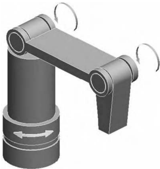
FIGURE 14.7 The articulated configuration.
