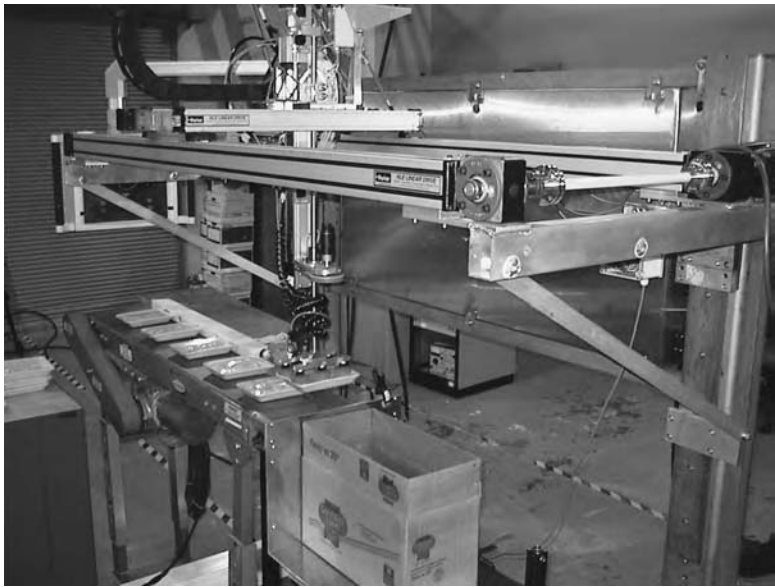
FIGURE 14.15 Case packer cartesian robot. (Courtesy of CAMotion, Inc.)
