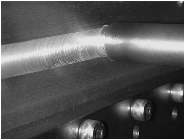
FIGURE 17.12 Friction stir weld.
