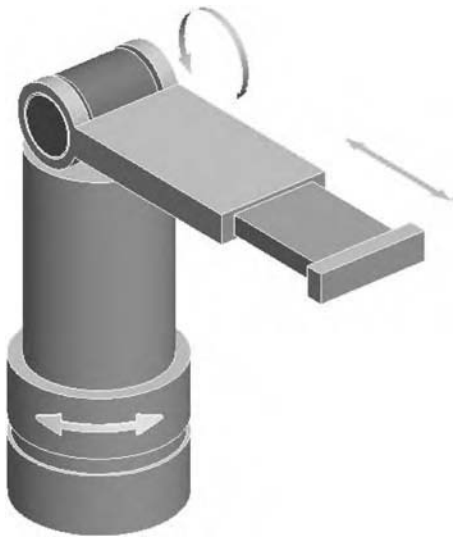
FIGURE 14.5 The spherical configuration.
