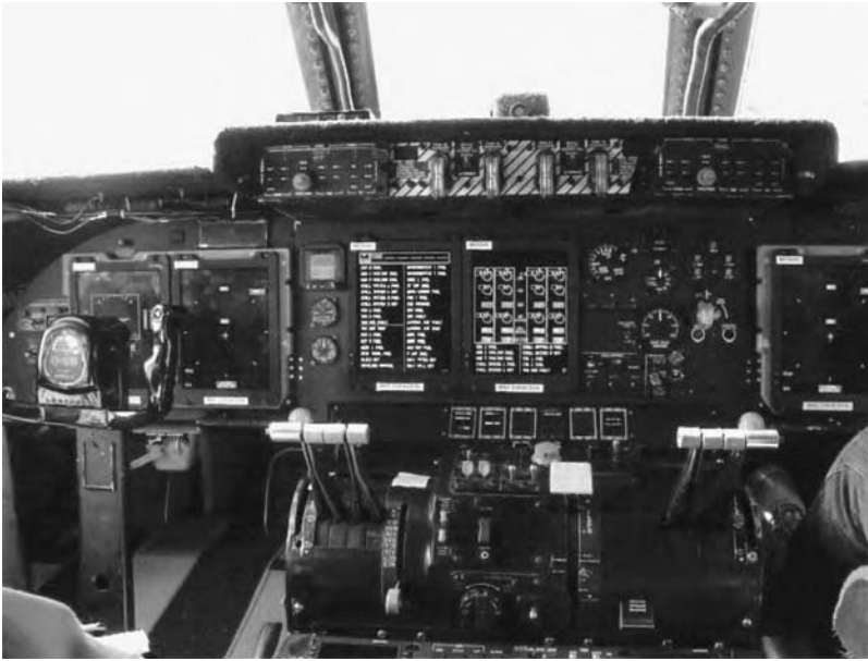
FIGURE 12.6 Navigation displays in the U.S. Air Force C-5 transport showing flat-panel displays in front of each pilot; vertical situation display outboard and horizontal situation display inboard. Waypoints are entered on the horizontally mounted control-display unit just visible aft of the throttles. In the center of the instrument panel are status and engine displays and backup analog instruments. (Photo courtesy of Honeywell, Copyright 2004.)
